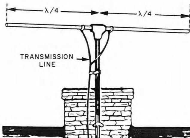
Figure 2-9.—Dipole antenna.
