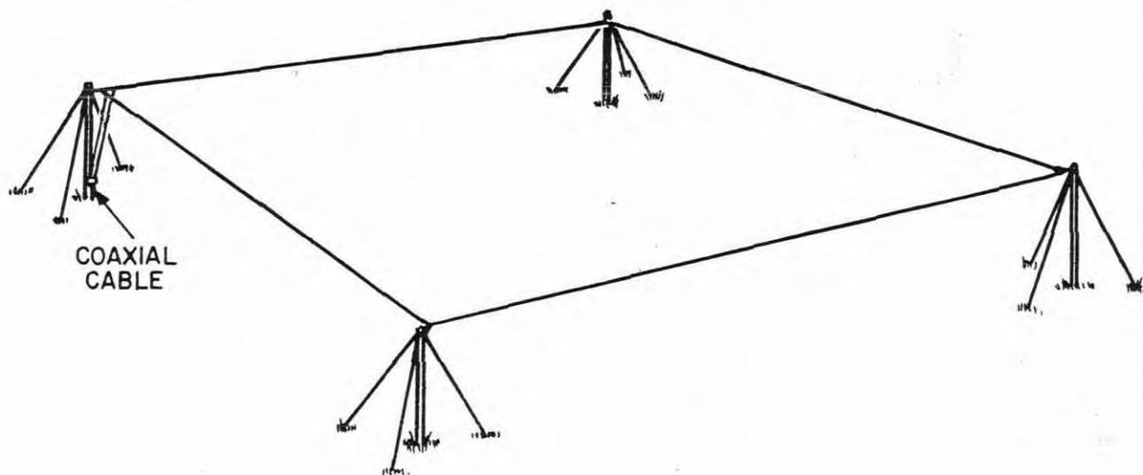
Figure 2-15.—A rhombic antenna.
