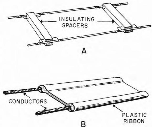
Figure 2-1.—Parallel pair transmission lines.
