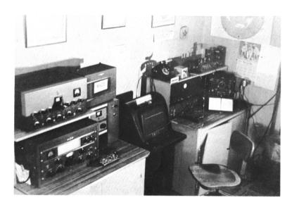
One of the better known RTTY stations is W6CG, formerly W9CSB of Chicago. Bud uses a Viking II for an exciter on the low frequencies, and has a 450 T final to help his signals along. He is active on CD RTNET as well as the SC 2 meter RTNET.
