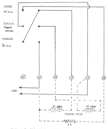
Series or Parallel switching of Printer Coils in Model 26
