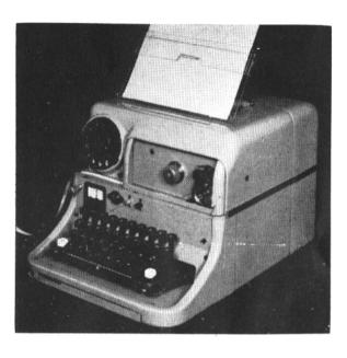
BRNO, CZECHOLOVAKIA—Simplicity and ease of maintenance characterize a tape-style teletypewriter which features a continuously rotating type wheel. Complete separation of electrical and mechanical components is a chieved in this design by sealed, self-contained units which plug in or clamp on inside the machine housing.
