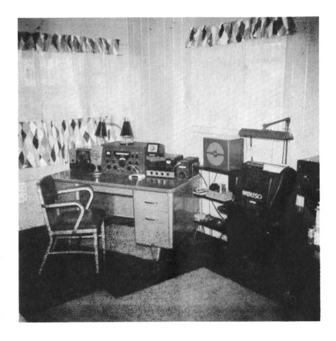
Have enclosed a picture of the shack. Left to right — Ranger, Collins 75-A3, Viking 6N2, BC-459 VFO for 6 and 2 meters, Model 26 Antennas are an 8/8 long john Telrex yagis on 2 meters, 3/3 Telrex on 6, Dipole on 80 and 40 and Vertical ground plane on 20, 15 and 10.
