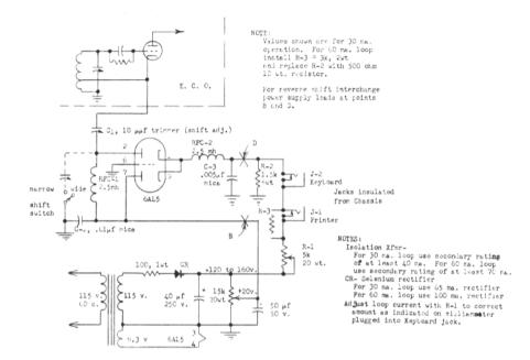
I have drawn it in to show the method of connection of this addition. To switch back to wide shift, it is only necessary to throw the switch to take out the added capacity. This same idea can be used to give several pre-set shift widths or to give pre-set shift widths for each band. The only adjustments necessary are:
