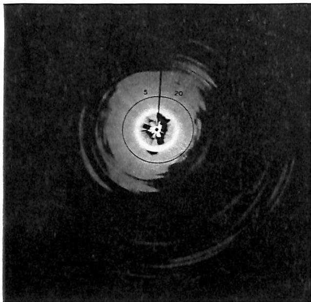
FIGURE 2.—Solid mass is broken up by FTC and tracking of moving targets is made comparatively easy.
