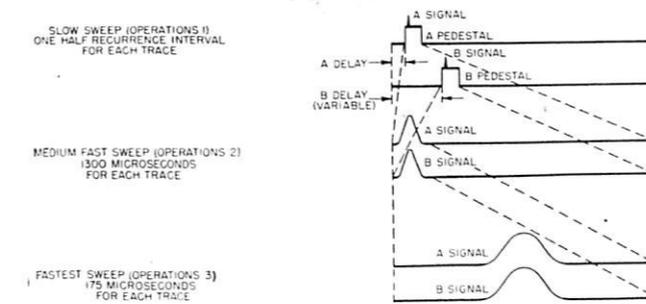
FIGURE 2.—Graphical representation of a signal on the three different sweep speeds available. Position 4 of the operations switch eliminates the trace separation.
