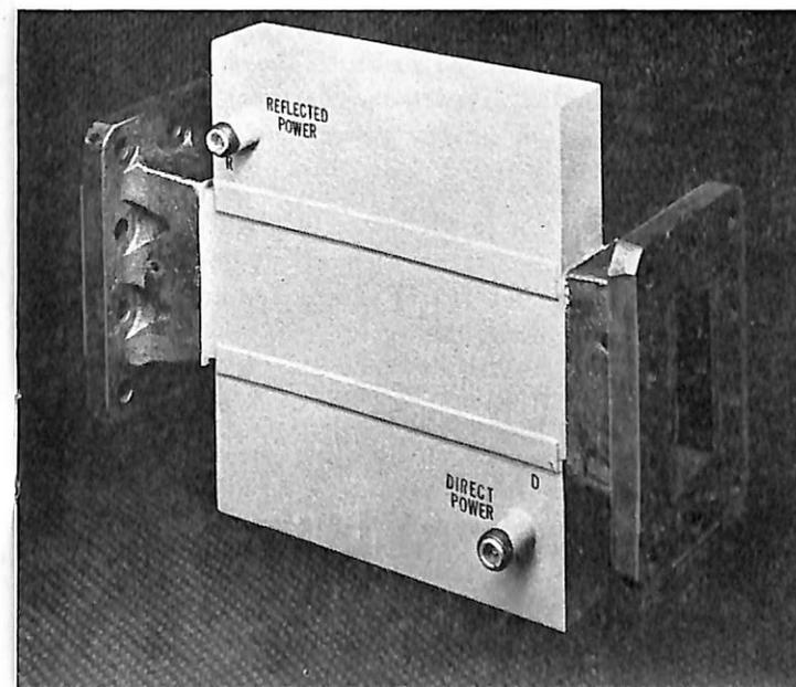
This bi-directional coupler can be used on  $S_s$ -band, radars, having 1-1/2" x 3" waveguide transmission lines and where 27 db coupling is required. Similar couplers can be made using other values of coupling. Different values of coupling are used with various models of radars to enable the same echo boxes to be used.
