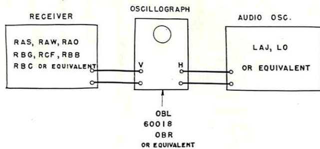
FIGURE 2—Block diagram indicating connections for the method of calibrating audio oscillators by the use of WWV modulated frequencies.
