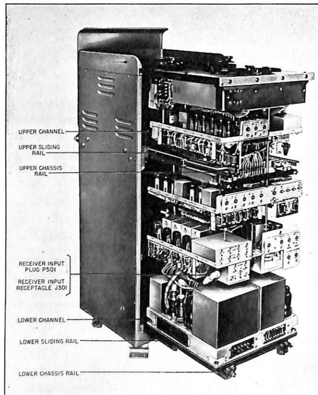
FIGURE 5.—The entire chassis, including the top panel, may be slid on rails out of the cabinet.
