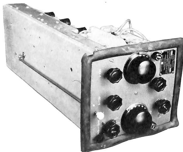
FIGURE 3.—Photograph showing remotely controlled switch for FTC circuit. The control shaft for the switch runs up the underside of the chassis.
