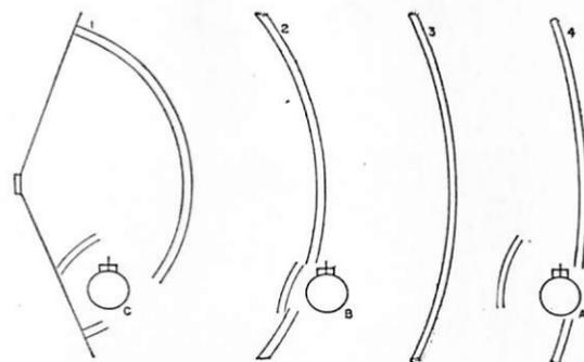
It should be noticed that although MCC decreases the directivity of the projector in the vertical plane, it does not affect the horizontal pattern. Thus we are able to achieve the advantages of maintaining close contact and still retain bearing accuracy.
