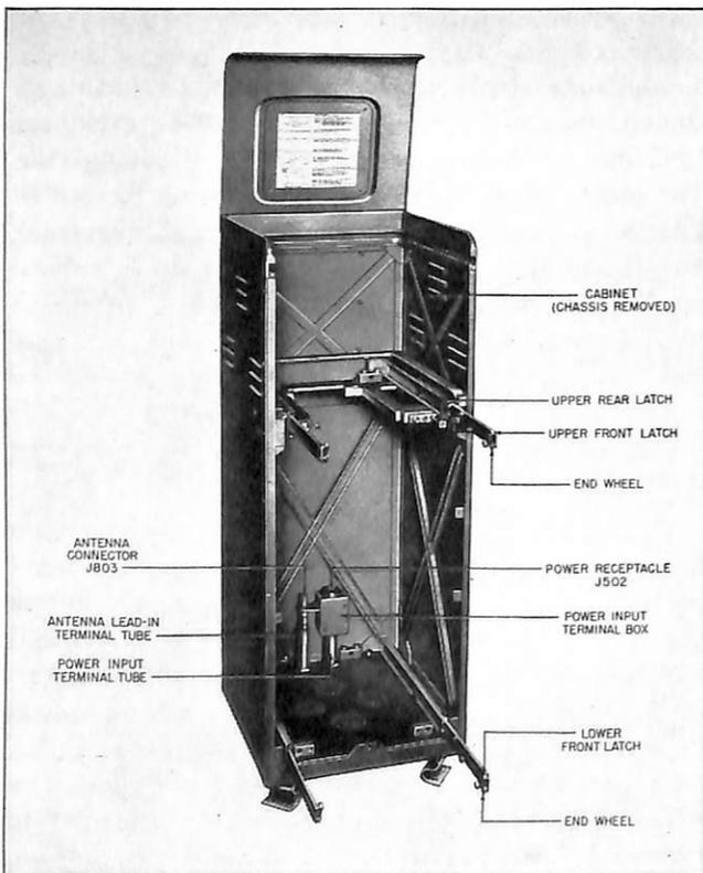
FIGURE 4.—The chassis may be removed and serviced while power and antenna remain attached.
