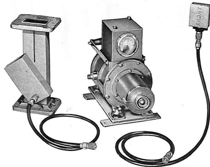
From left to right: CABV-47AAN directional coupler, CABV-14ABA-1 echo box and CABV-66AJG pickup dipole. This type directional coupler is for use with S-band radars having 1-1/2" x 3" wave guide transmission line. It may be seen that in this case the auxiliary wave guide section is fastened to the longest side of the main wave guide and is set at an angle. The auxiliary line fitting will connect to a flexible cable for coupling to the echo box.
