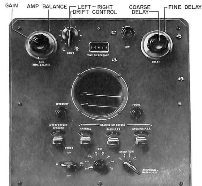
FIGURE 1.—Improved control panel of DBE Loran indicates time difference directly in microseconds.
