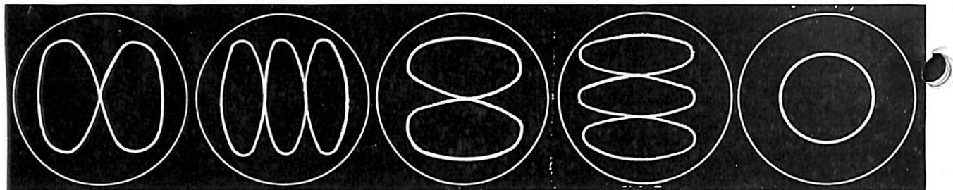
FIGURE 3.—Common Lissajous figures used in frequency determination. (a) Frequency on vertical plates equal to twice frequency on horizontal plates. (b) Frequency on vertical plates equal to three times frequency on horizontal plates. (c) Frequency on vertical plates equal to 1/2 time frequency on horizontal plates. (d) Frequency on vertical plates equal to 1/3 of frequency on horizontal plates. (e) Frequencies equal.
