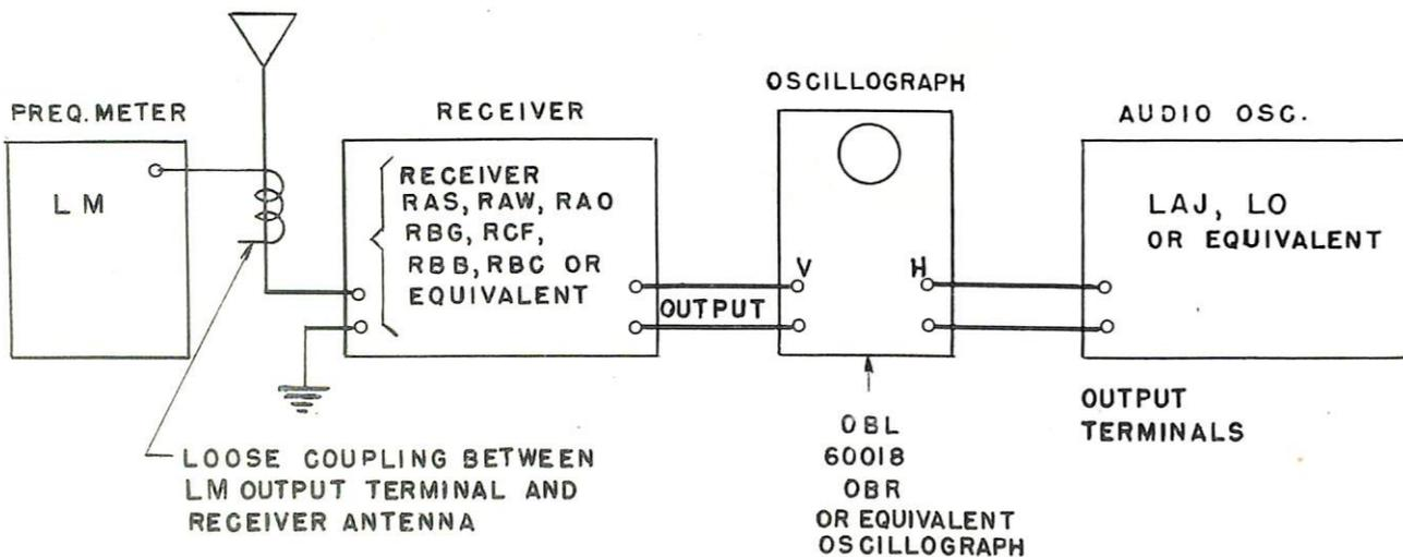
FIGURE 1.—Block Diagram showing the use of standard pieces of Navy test equipment to check the frequency difference between WWV and the LM calibrator crystal.
