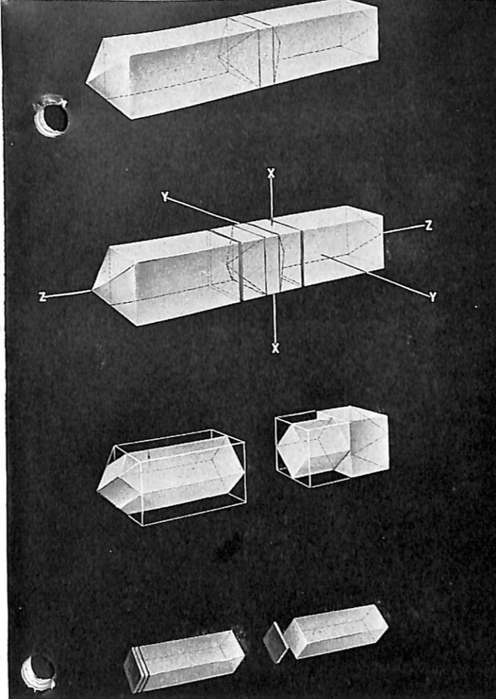
Steps in the formation of the finished crystal. The crystal is grown onto "planted" caps. Final plates are cut at 45 degrees to the X and Y axis and normal to the Z axis.
