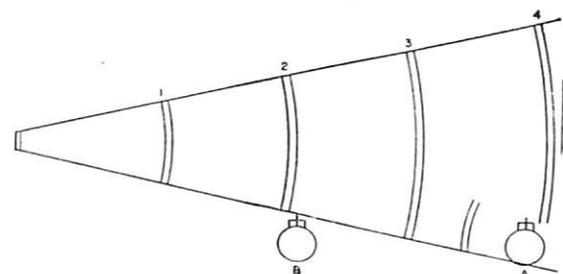
hit by the beam, and some sound energy will be reflected. However, if the submarine is at position B, the sound beam will pass over, and no energy will be reflected. It is clear, therefore, that as the projector approaches the target, a point will be reached where the transmitted sound will pass over it.
