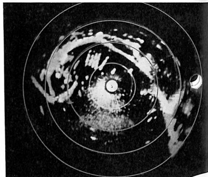
When a larger capacitor value is switched into the RC circuit almost all sea return is eliminated.
