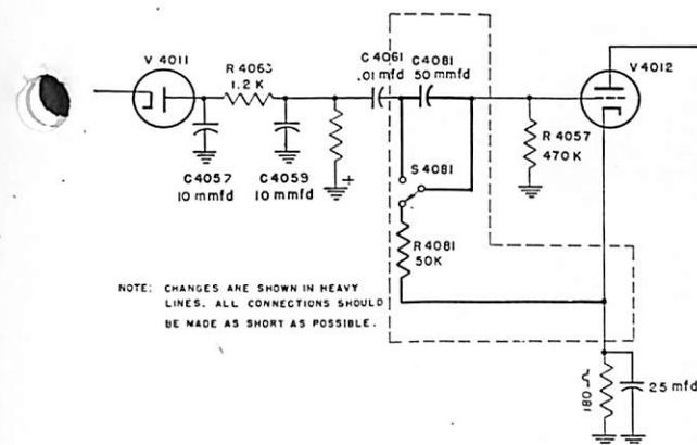
FIGURE 4.—Schematic diagram for incorporating FTC circuit.
