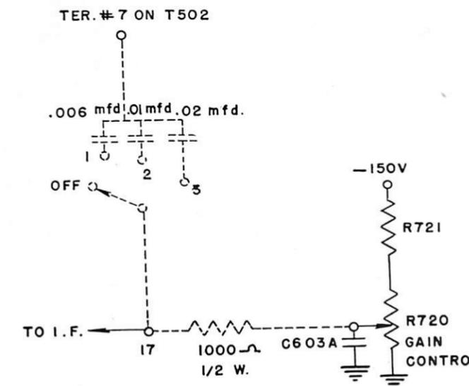
FIGURE 2—Schematic diagram of the STC circuit. Added portions are indicated by dotted lines.
