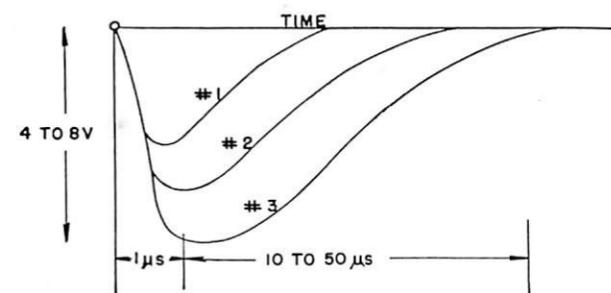
FIGURE 1—Curves illustrating voltages that are applied to the i-f strips of the receiver to accomplish sensitivity time control. The curves shown are for three different capacitor values.
