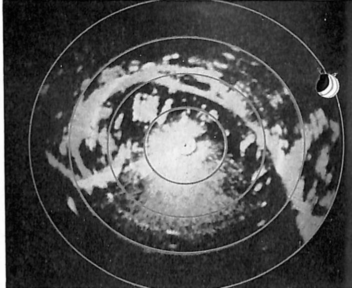
(Above)—PPI scope without STC showing considerable sea return. (Below)—Effect on scope picture when sensitivity time control is introduced.
