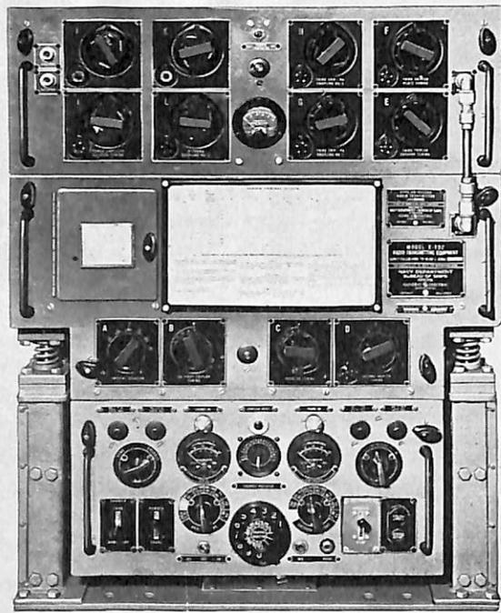
Front panel of the TDZ Transmitter. Note the telephone dial and channel indicator on the bottom panel.
