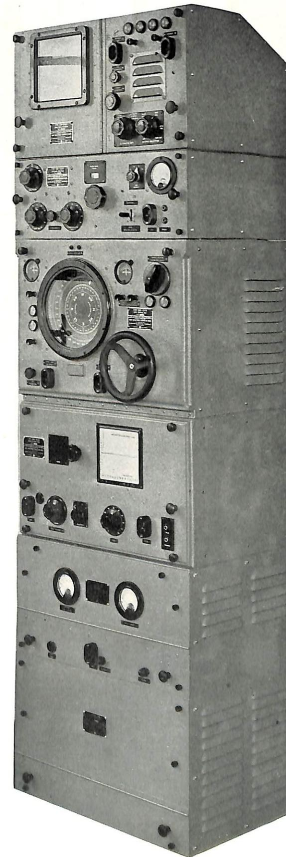
Forward torpedo room sonar stack
