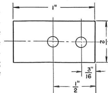
FIGURE 4.—Dimensions of asbestos pad.
