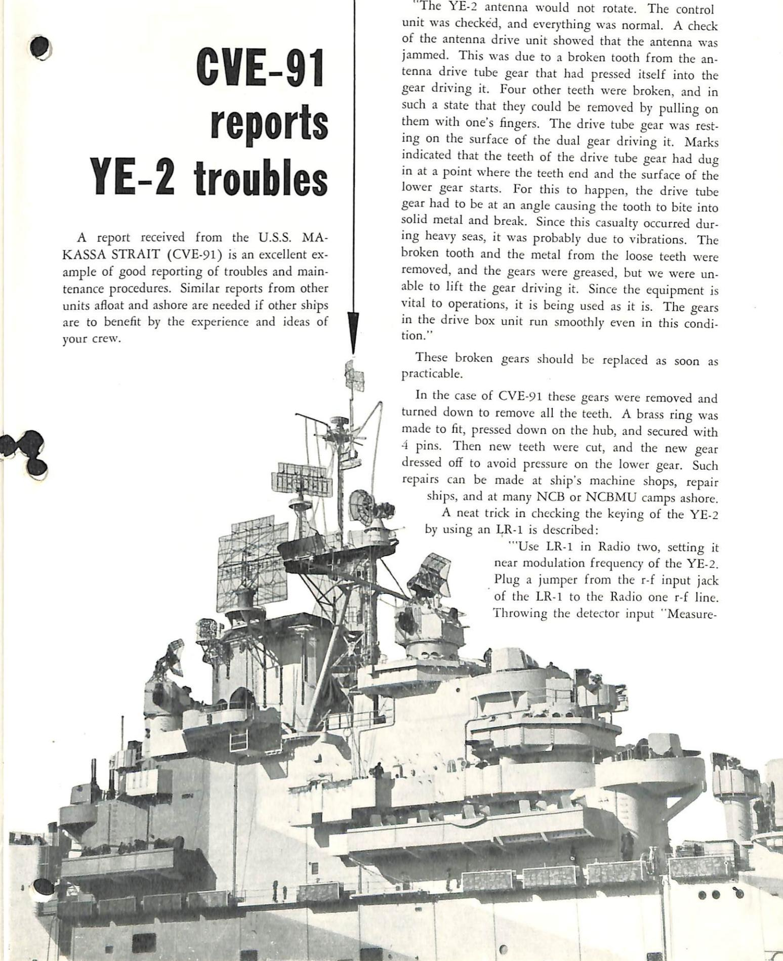
Match" switch to "Match", we can check the YE-2 keying by plugging a head set into the audio output of the frequency meter and listening to the beat note of the LR-1 against the modulation frequency.
