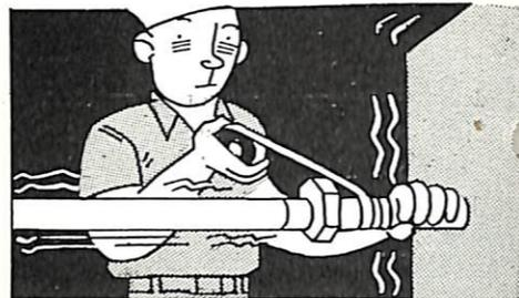
the pulse cable. If the job is not well done, the system will radiate power which will interfere with adjacent radio equipment. Protect the cable from any crushing which might loosen the inner conductor from the first layer of rubber. When air enters the line, it can start corona. Check the bonding of the outer shield of the cable to the ship's structure. Make sure the cables do not run too closely to hot vacuum tubes.
