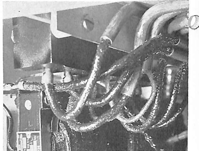
TBM-10 Modulator Unit before and after tropicalization. Note that all cloth covered wires to the modulator transformer T-405 have been attacked by fungus growth.
