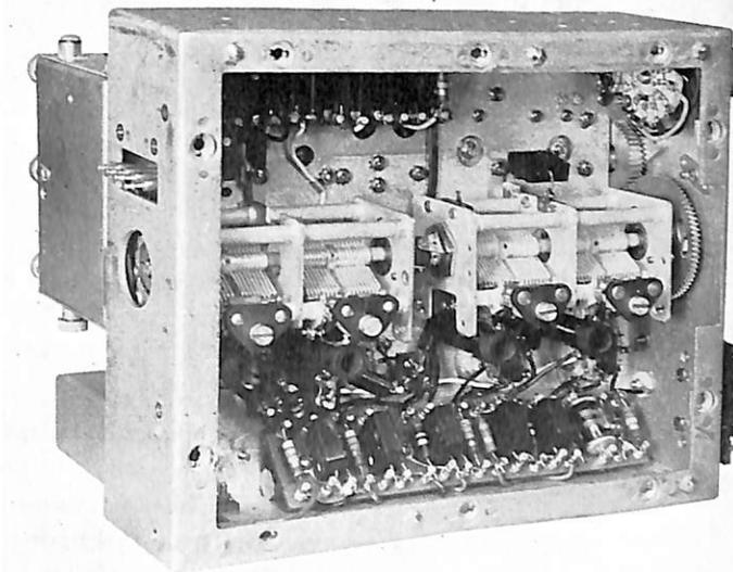
Rugged construction is exemplified by this RDZ pre-selector chassis.
