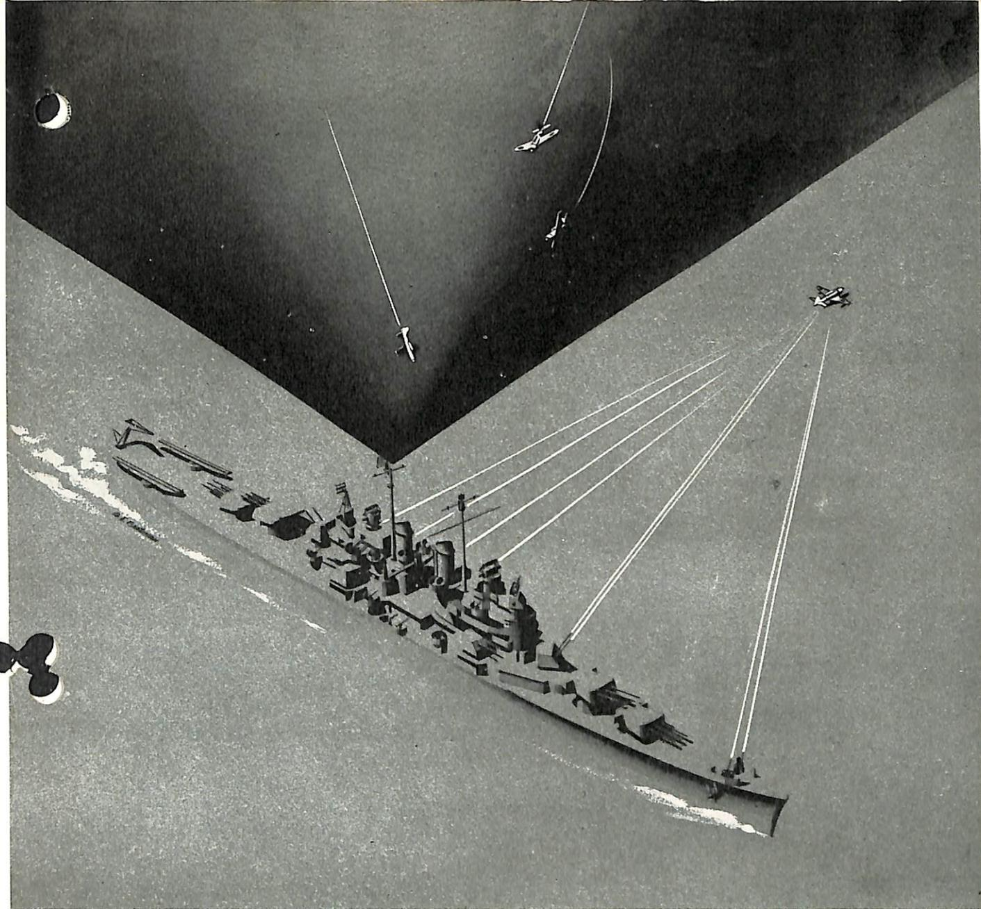
*SG radar is converted into Zenith Watch by this modified antenna reflector and r-f feed. The antenna pedestal is not affected.*
