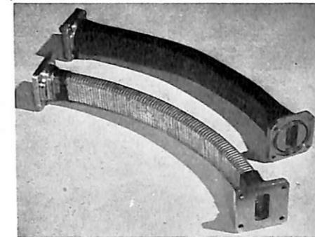
Sections of flexible waveguide simplify the problem of emergency repairs.
