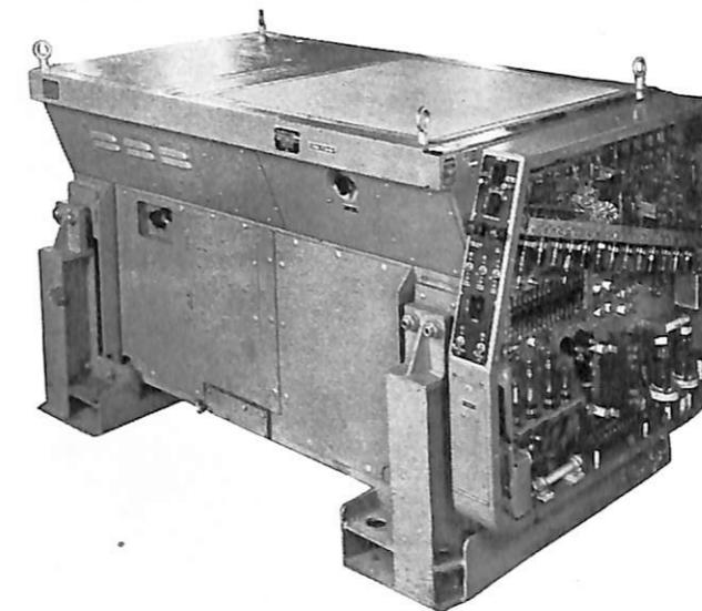
Oblique View of VG Remote Indicating Equipment with end cover removed.
