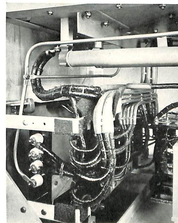
*Right side of bottom deck of a TBM-10 Modulator Unit before and after the tropicalization treatment. This is new equipment being unpacked and treated before going into service with the fleet.*
