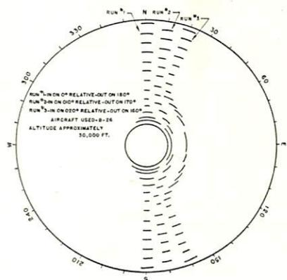
*Drawing made from a Zenith-Watch Scope showing the presentation of three different plane runs. The first run passed directly overhead; in the other two the plane passed the antenna to starboard.*
