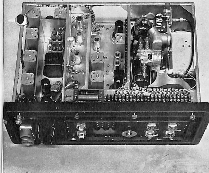
Compact, miniature construction packs a lot of radio in a small package in the Model MAR.
