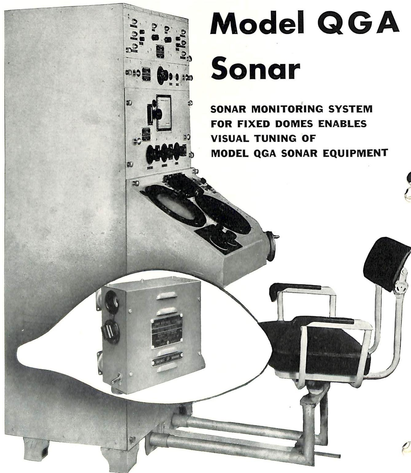
■ A method of "seeing" if the frequency of the driver is adjusted for maximum transmitted signal and if the transmitted signal level is normal has been designed by the Bureau of Ships for ships having model QGA sonar equipment.
