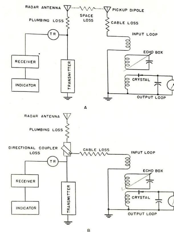
FIGURE 5.—Two methods of feeding the echo box are illustrated above. Note that when the directional coupler is used, the plumbing loss is not present.
