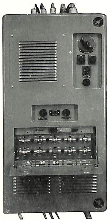
A front view of the driver unit shows how controls and switches are recessed in the equipment. Dropping door provides easy access to all fuses.
