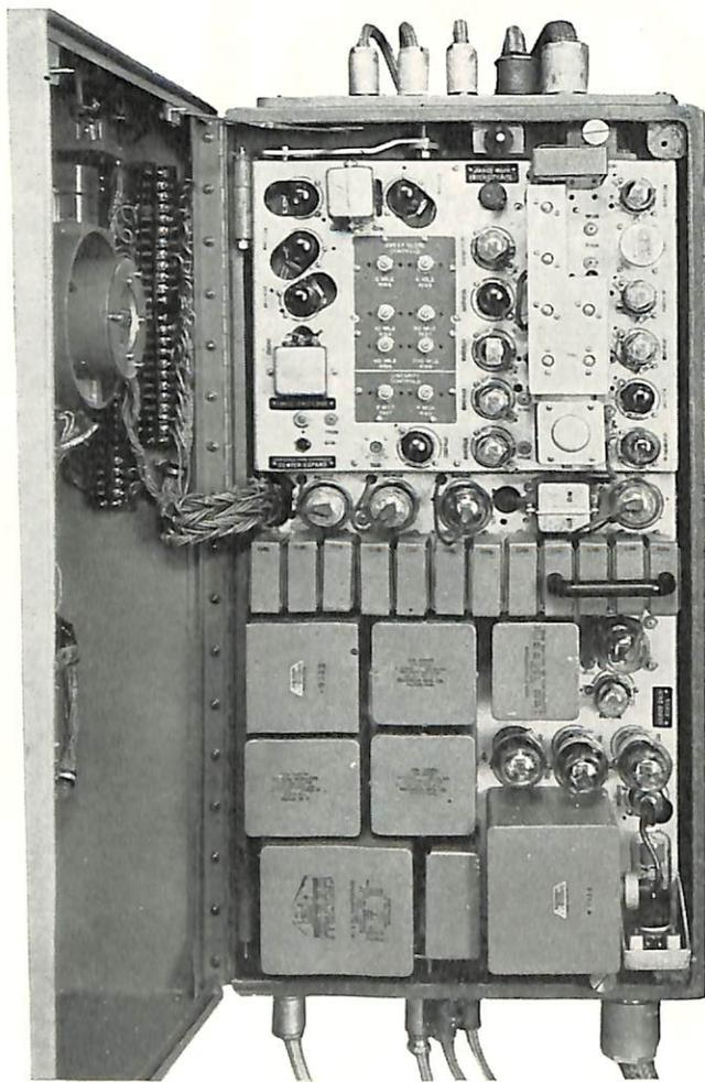
The front panel of the driver unit, when opened, presents a neat arrangement and easy accessibility to all tubes and screwdriver controls.
