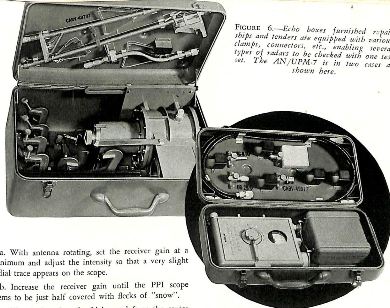
FIGURE 6.—Echo boxes furnished repair ships and tenders are equipped with various clamps, connectors, etc., enabling several types of radars to be checked with one test set. The AN/UPM-7 is in two cases as shown here.
