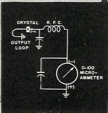
FIGURE 2.—Schematic diagram of the echo box.
