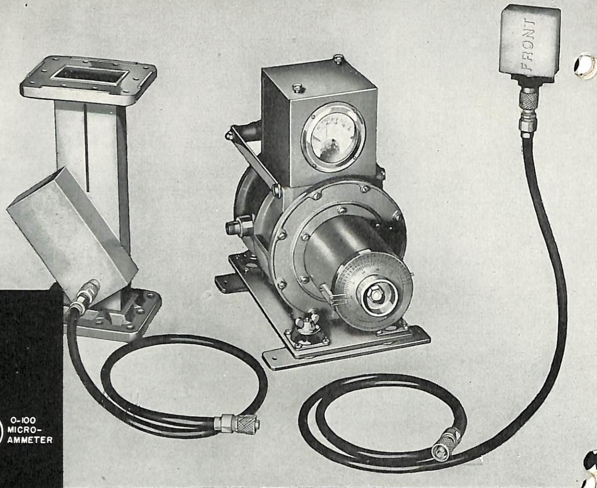
FIGURE 1.—One model echo box test set, the OBU-3, is shown with a directional coupler to the left and a pickup dipole to the right.
