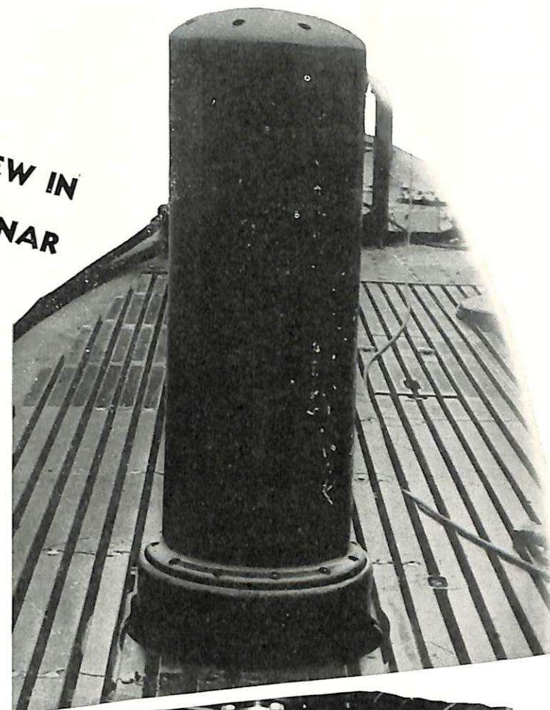
Specifically designed for submarine warfare and including in the installation many of the newer advancements of sonar equipment formerly supplied as field changes or as modifications to the original sonar installation, Model WFA Echo Ranging—Listening—Sounding Equipment, manufactured by the Submarine Signal Company, offers a good example of some of the modern advancements that have been made in submarine sonar during the present war.
