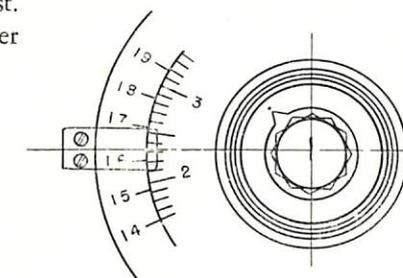
FIGURE 3.—A section of the echo box tuning dial. Outer dial moves one division when inner dial is turned one complete revolution. Reading above would be approximately 1623.
