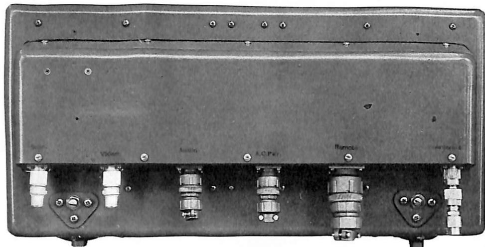
Rear view of the Model RDZ cabinet showing the cable filter blister and location of the various cable connectors. The blister cover can be removed from the back to provide access to the filter components, or the complete filter may be removed through the front of the cabinet.
