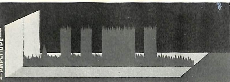
FIGURE 1.—Three-dimensional representation of a conventional telegraph signal.
