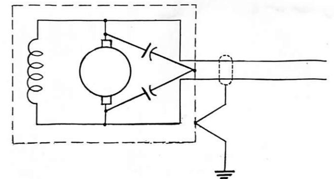
FIGURE 1—Simple filter consisting of small capacitors connected between brushes and motor frame.
