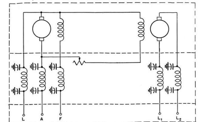
FIGURE 3—All external connections to this motor-generator unit are filtered.
