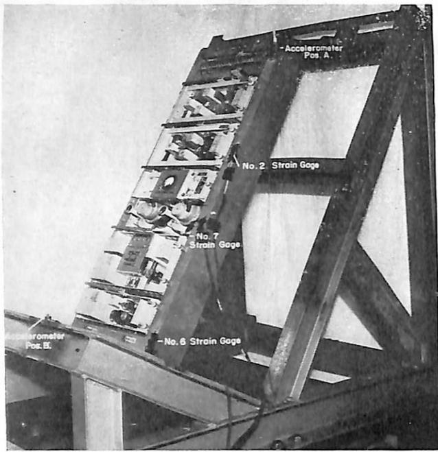
Typical arrangement of jigs and gauges for shock-testing equipment with the medium-weight shock-testing machine.
