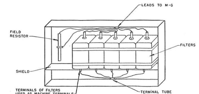
FIGURE 4—Arrangement of components inside shield case of filter unit.
