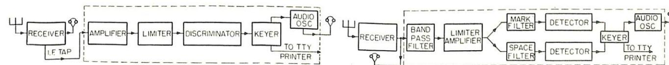
FIGURE 6.—Arrangement of FSK receiver-converter for operation direct from the IF amplifier of a receiver which has been modified for the purpose.
