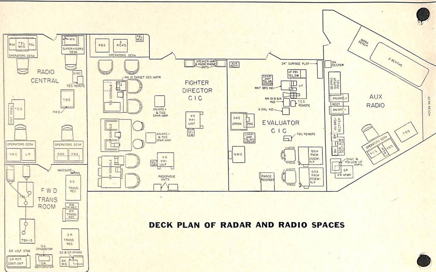
**DECK PLAN OF RADAR AND RADIO SPACES**
