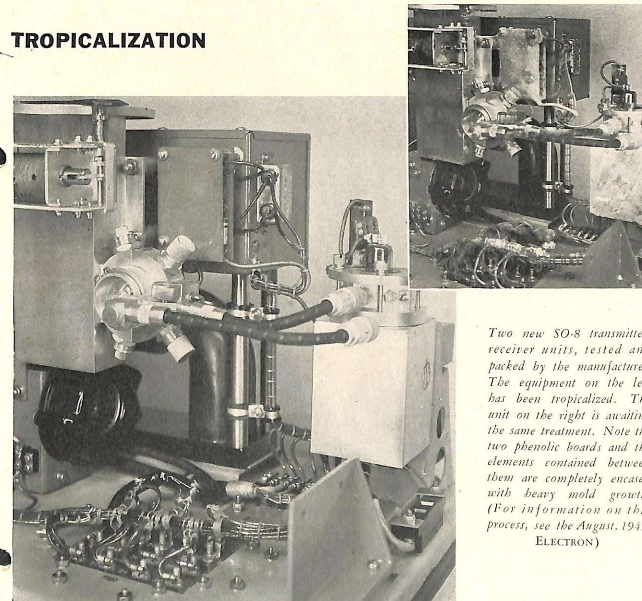
*Two new SO-8 transmitter-receiver units, tested and packed by the manufacturer. The equipment on the left has been tropicalized. The unit on the right is awaiting the same treatment. Note the two phenolic boards and the elements contained between them are completely encased with heavy mold growth. (For information on this process, see the August, 1945, ELECTRON)*
