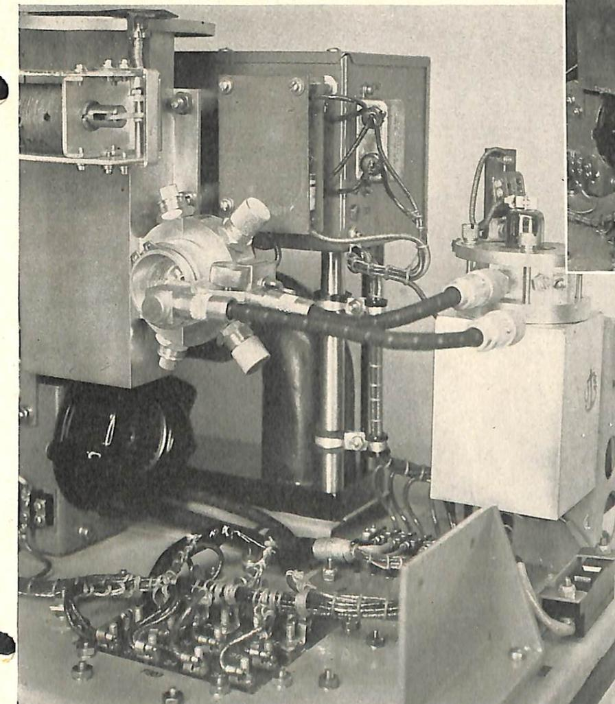
*Two new SO-8 transmitter-receiver units, tested and packed by the manufacturer. The equipment on the left has been tropicalized. The unit on the right is awaiting the same treatment. Note the two phenolic boards and the elements contained between them are completely encased with heavy mold growth. (For information on this process, see the August, 1945, ELECTRON)*
