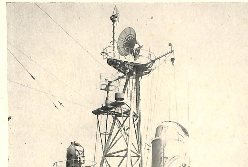
The usual radio and radar antennas have been retained on the foremast. Additional VHF antennas bristle from the yardarm and all around the mast giving a Christmas-tree effect. TBS and low-frequency DBM-1 spinners are stacked one above the other, outrigged forward of the mast. Antenna trunks and whips sprout from every deck house.
