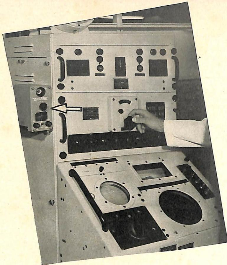
■ With the new Retractable Dome Tuning Indicator equipment now in production, most sonar gear having a streamlined dome will be magic-eye tuned. This new tuning indicator is designed for use with echo-ranging equipment installed with either the 50-inch or 54-inch retractable domes.
