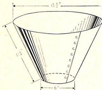
There is ample clearance between the tube and shield to absorb gunfire shock without physical contact. This shield with its simplicity and ease of installation has eliminated completely a troublesome situation.
