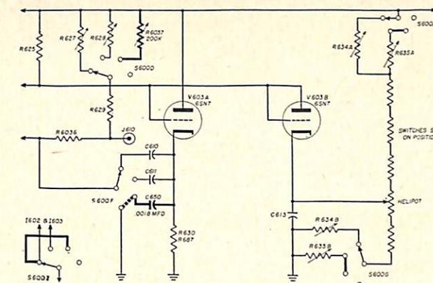
FIGURE 1—Circuit showing 80-mile range step. Heavy lines indicate new wiring, and the dotted line indicates a connection removed.
