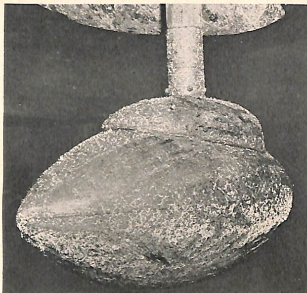
Fish type dome showing moderate amount of calcaereous growth before cleaning.
