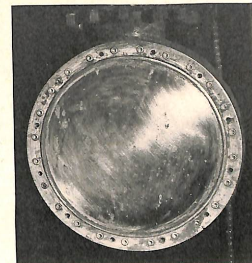
Projector face has been cleaned by some sort of abrasive, probably steel wool, as indicated by the deep scratches in the metal surface.
