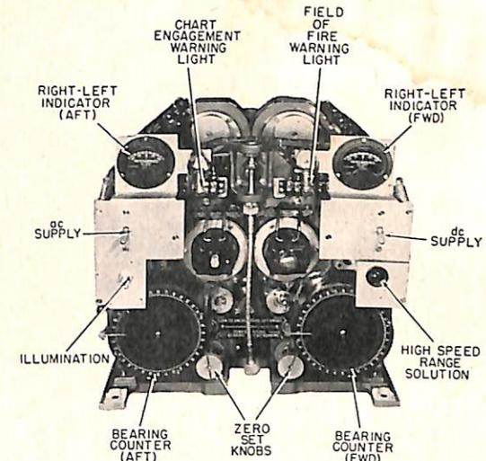
FIGURE 6—Azimuth drive unit of the computer—front view, covers removed.
