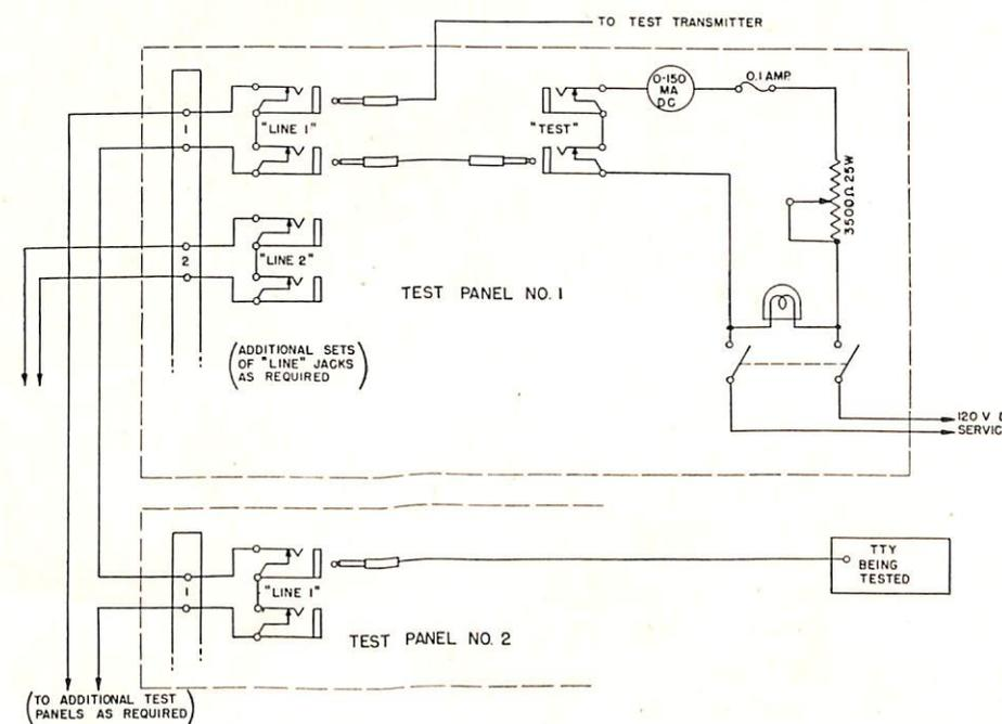
Schematic of one of the test panels, showing external wiring and patching required for multiple testing.
