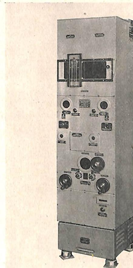
FIGURE 4—Mechanical computer stack. From top to bottom, in order, are the rectifier unit, range-rate assembly, triangle solver, and power unit.
