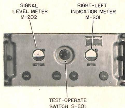
FIGURE 3—Right-left indicating bearing deviation indicator main unit.
