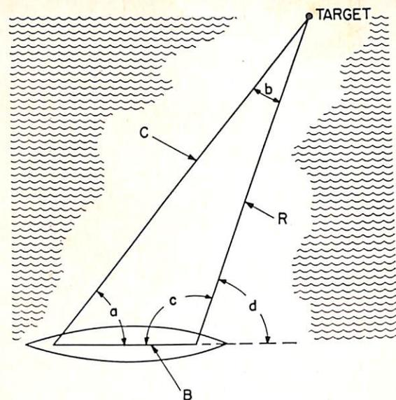
FIGURE 8—Typical triangle to be solved by the computer. Angle  $a$  is the after hydrophone bearing, angle  $d$  the forward bearing, angle  $b$  the target angle, side  $B$  the baseline, and side  $R$  the range line from the forward hydrophone to the target.
