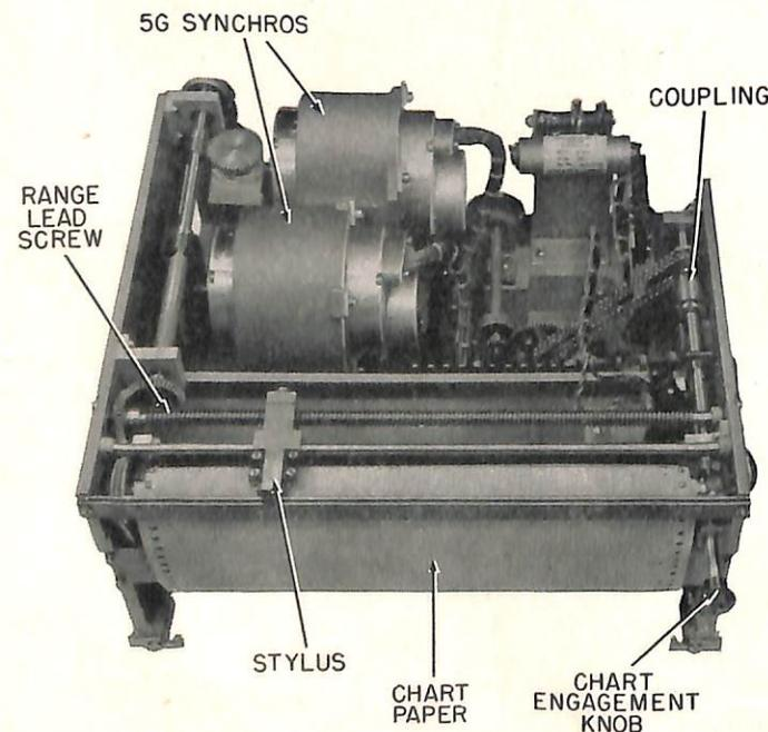
*Exposed view of range recorder unit of the computer, showing major components.*
