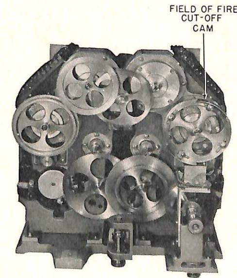
FIGURE 7—Azimuth drive unit of the computer—rear view, covers removed.
