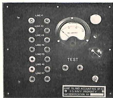
Closeup of one of the TTY test panels which provides 7 tie lines to other work benches.
