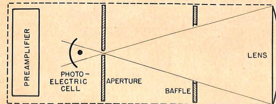
FIGURE 4—Cross section diagram of detector optical system and p-e cell.
