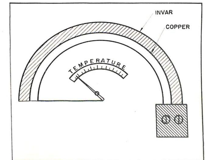
FIGURE 7—Principle of bimetallic thermometer.
