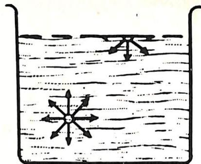
FIGURE 3—Surface tension of a liquid results from uncancelled molecule forces at the surface.
