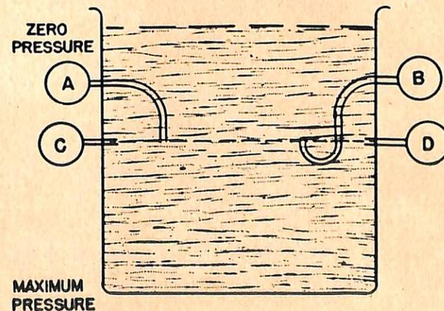
FIGURE 5—Pressure acting on a molecule of a liquid of uniform temperature is the same in any direction.
