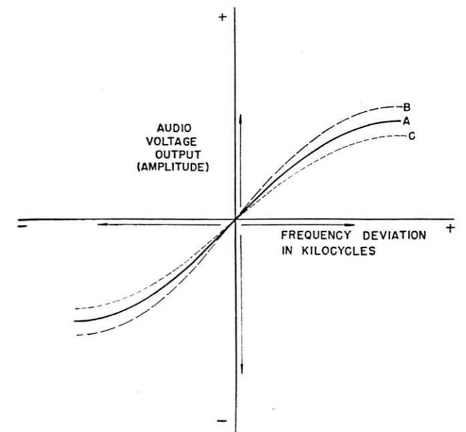
FIGURE 2—Characteristic curves for standard discriminator circuit. Curve A represents standard i-f signal amplitude; curves B and C show the effects of changing the magnitude of i-f signal.
