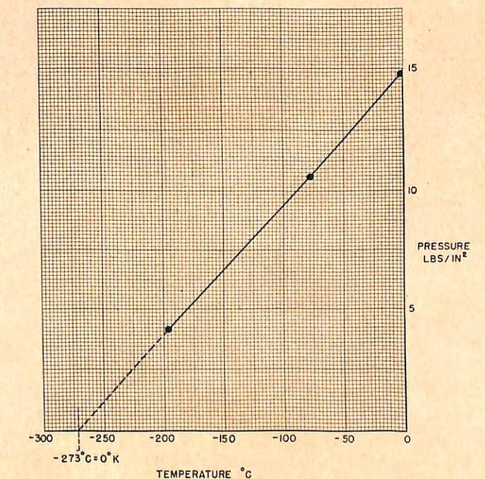
FIGURE 6—Experimental determination of absolute zero temperature.
