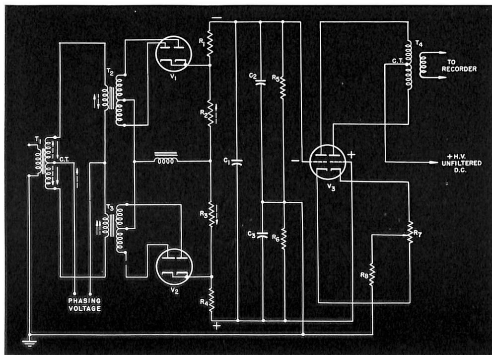
FIGURE 6—Simplified schematic diagram of discriminator.
