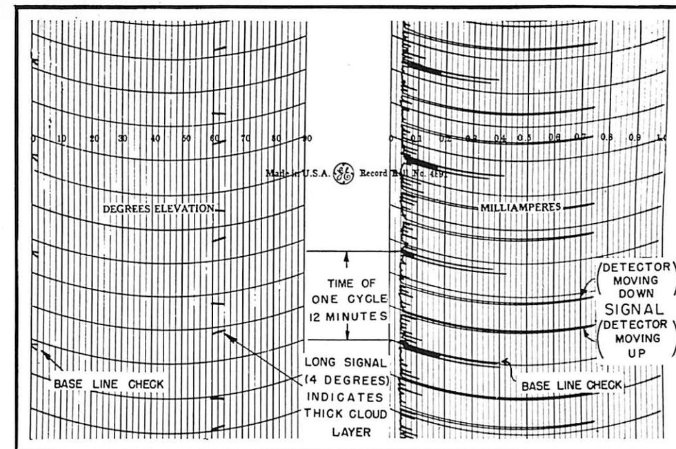
FIGURE 7—Typical graphs made by ceilometer recorder.
