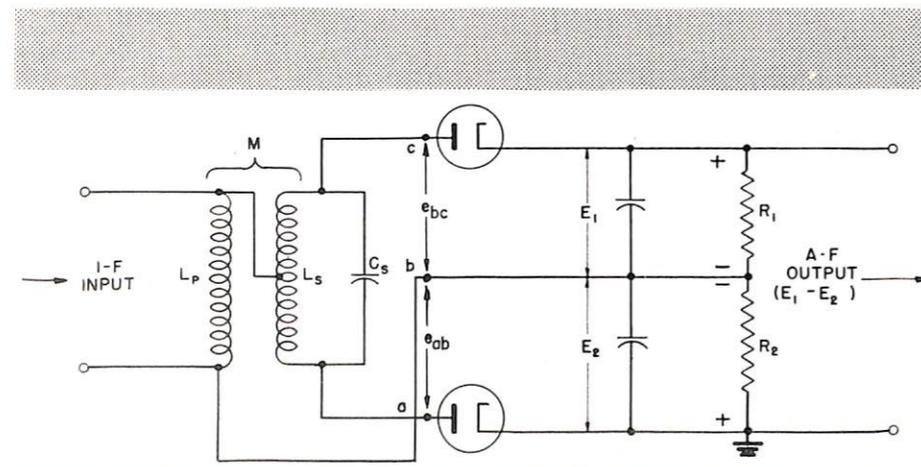
FIGURE 1—Standard discriminator circuit. This circuit is sensitive to both AM and FM and must therefore be preceded by a limiter circuit.
