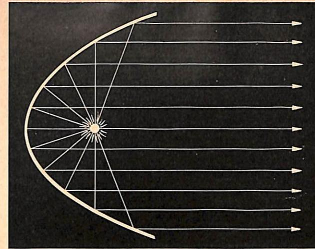
FIGURE 3—Action of a parabolic reflector and a point source of light located at the focal point.
