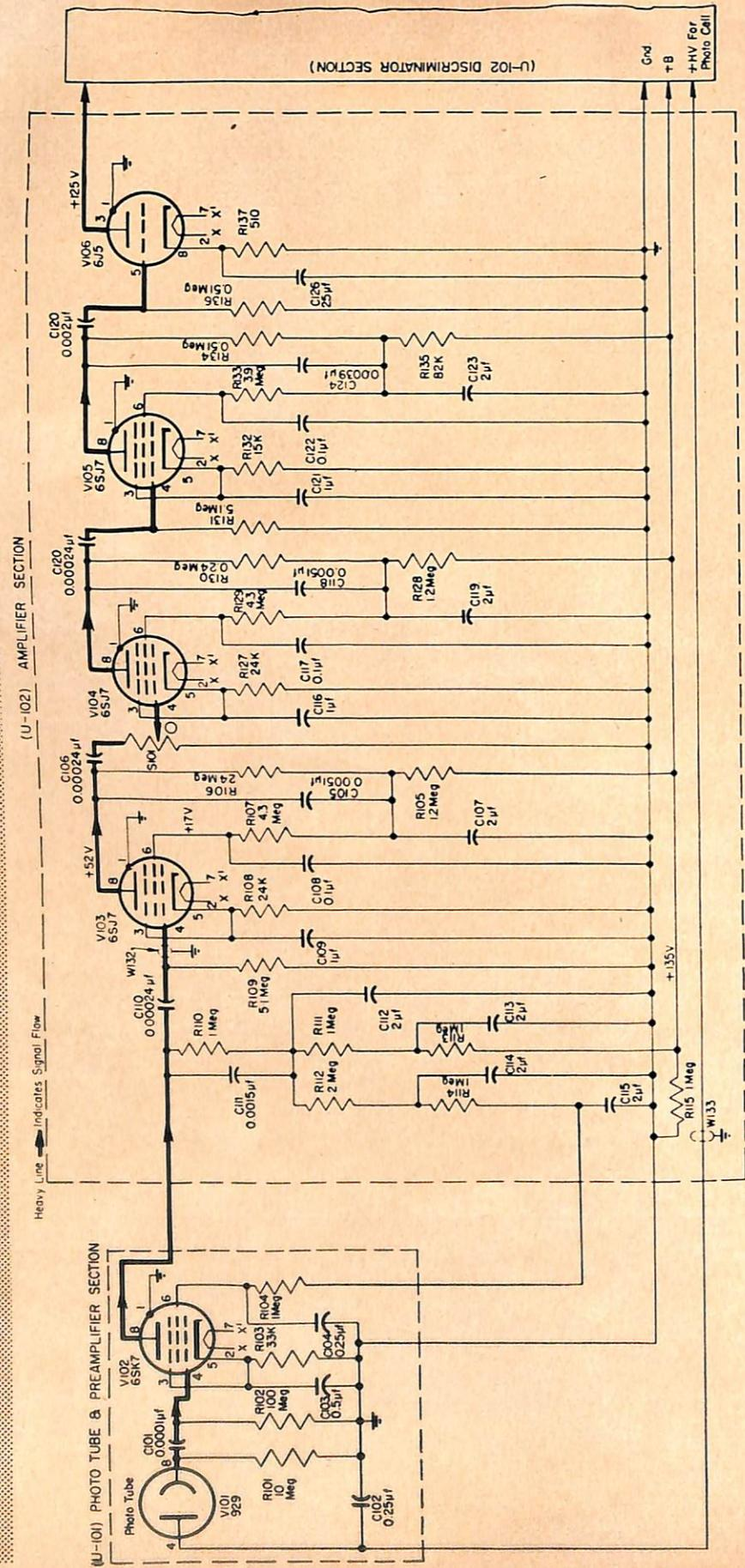
FIGURE 5—Schematic diagram, pre-amplifier and amplifier.
