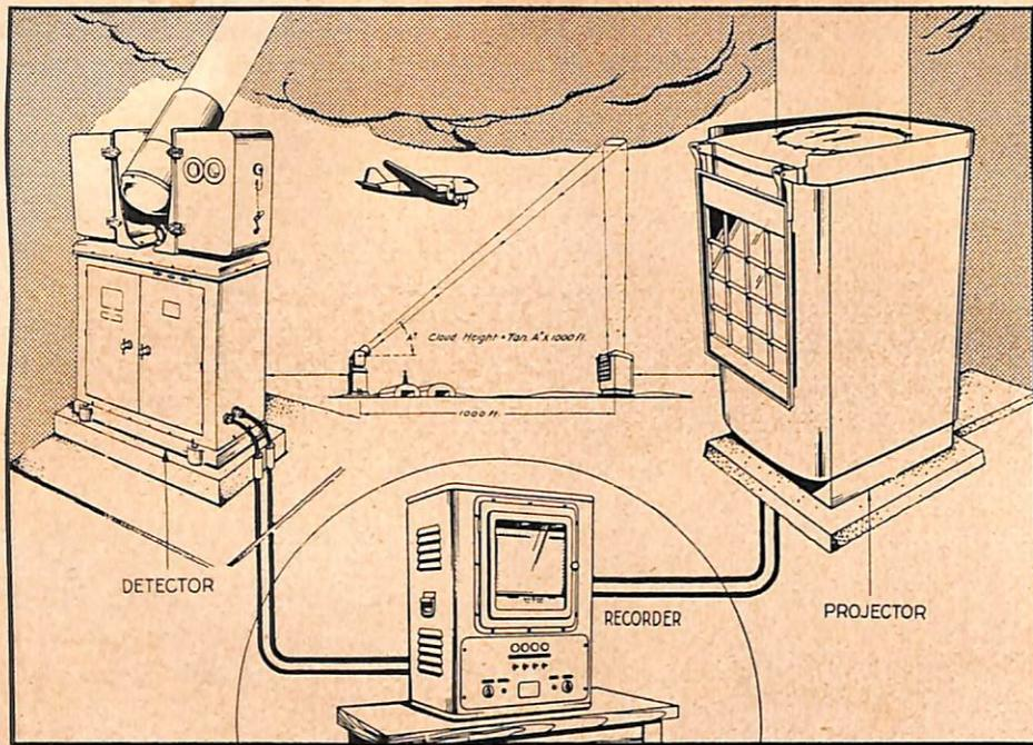
FIGURE 2—Ceilometer equipment AN/GMQ-2. Schematic layout.
