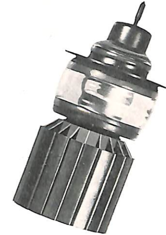
An experimental-type grounded-grid r-f power amplifier tube. Fins are provided to aid in dissipating heat.
