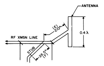
ADJUST STUB ATTACHMENT POINT & STUB SHORTING BAR FOR LOWEST VSWR.
