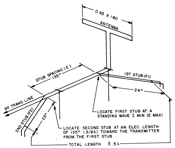
ADJUST THE STUB SHORTING BARS FOR LOWEST VSWR (STUB LENGTHS SPECIFIED ARE MEDIAN VALUES)
