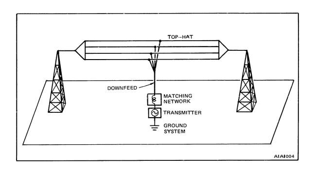
Figure 1-3. Simplified VLF Transmitting Antenna
