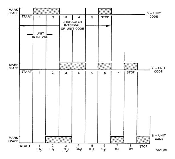
Figure 1-1. Comparison of Transmission Format of Letter A Using 5-, 7-, and 8- Unit Code Systems
