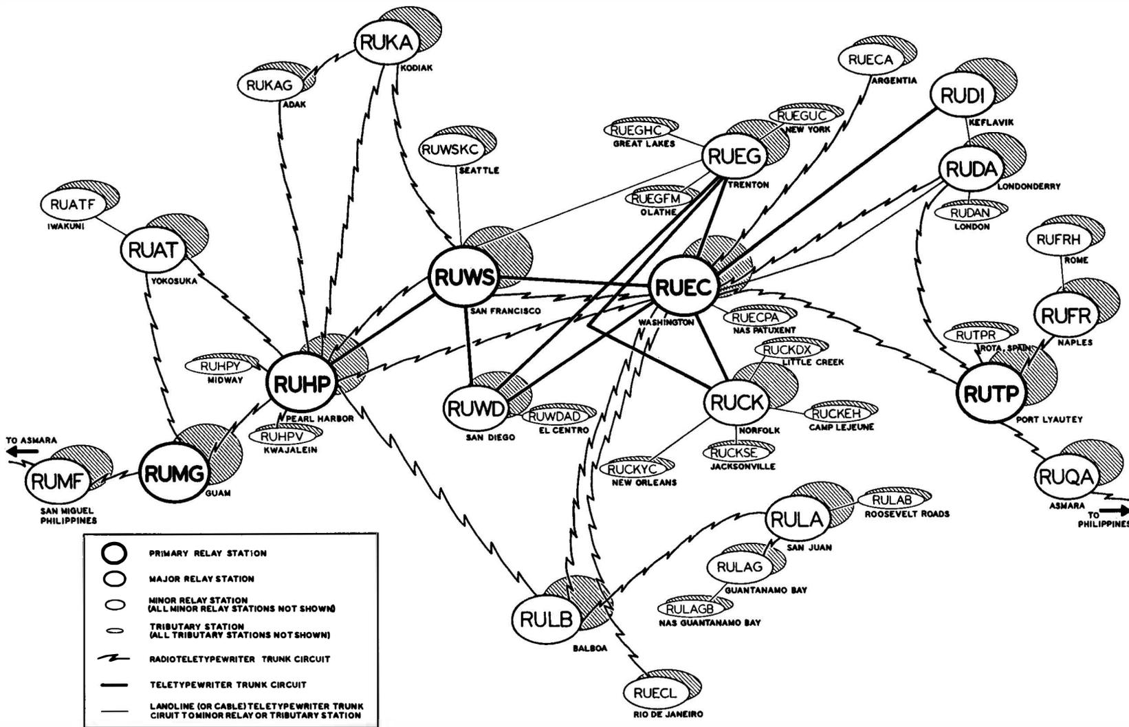
Figure 11-1. —U.S. naval teletypewriter tape relay system.
