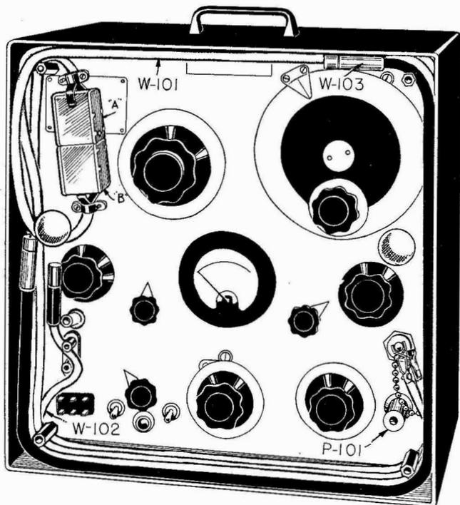
Figure 7-12—Method of Stowing Interconnecting Cable (W-101), Output Test Cord (W-102), Patch Cord (W-103), and Concentric Plug (P-101) on Panel of the Signal Generator
