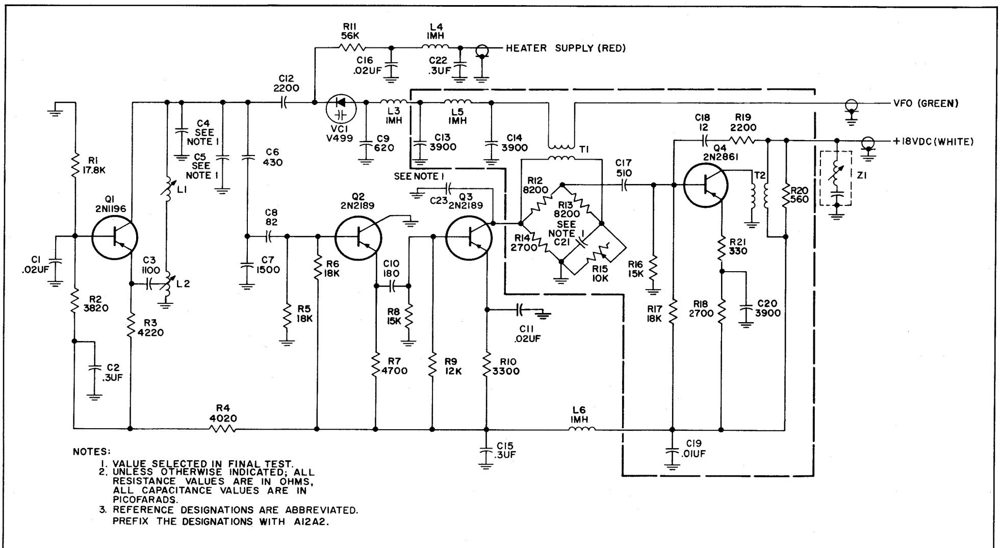
Figure 7-14. Variable Frequency Oscillator Submodule A12A2, Schematic Diagram
