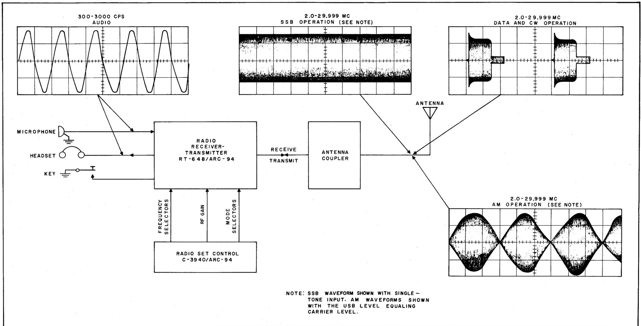
Figure 4-3. Radio Set AN/ARC-94, Block Diagram with Input and Output Waveforms
