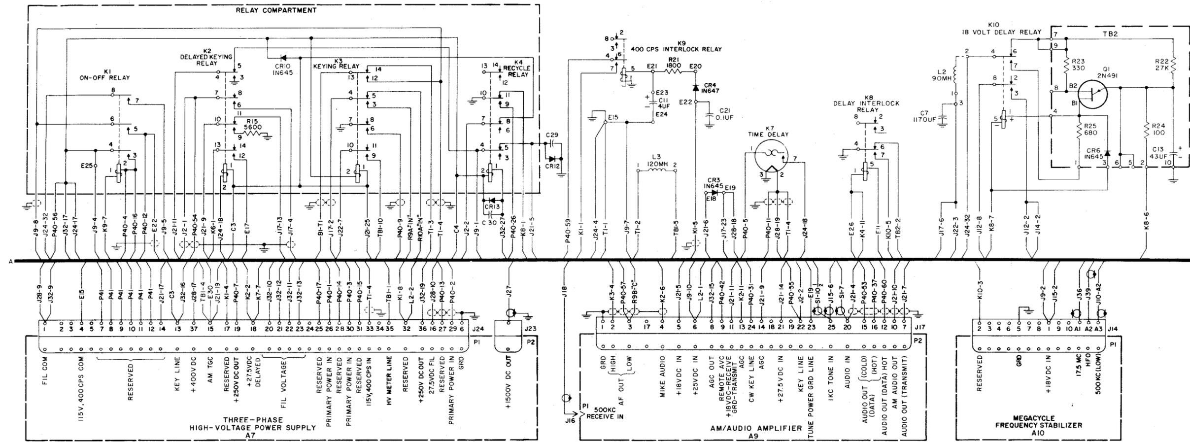
Figure 7-1. Radio Receiver-Transmitter RT-698/ARC-102 Chassis, Schematic Diagram (Sheet 2 of 3)
