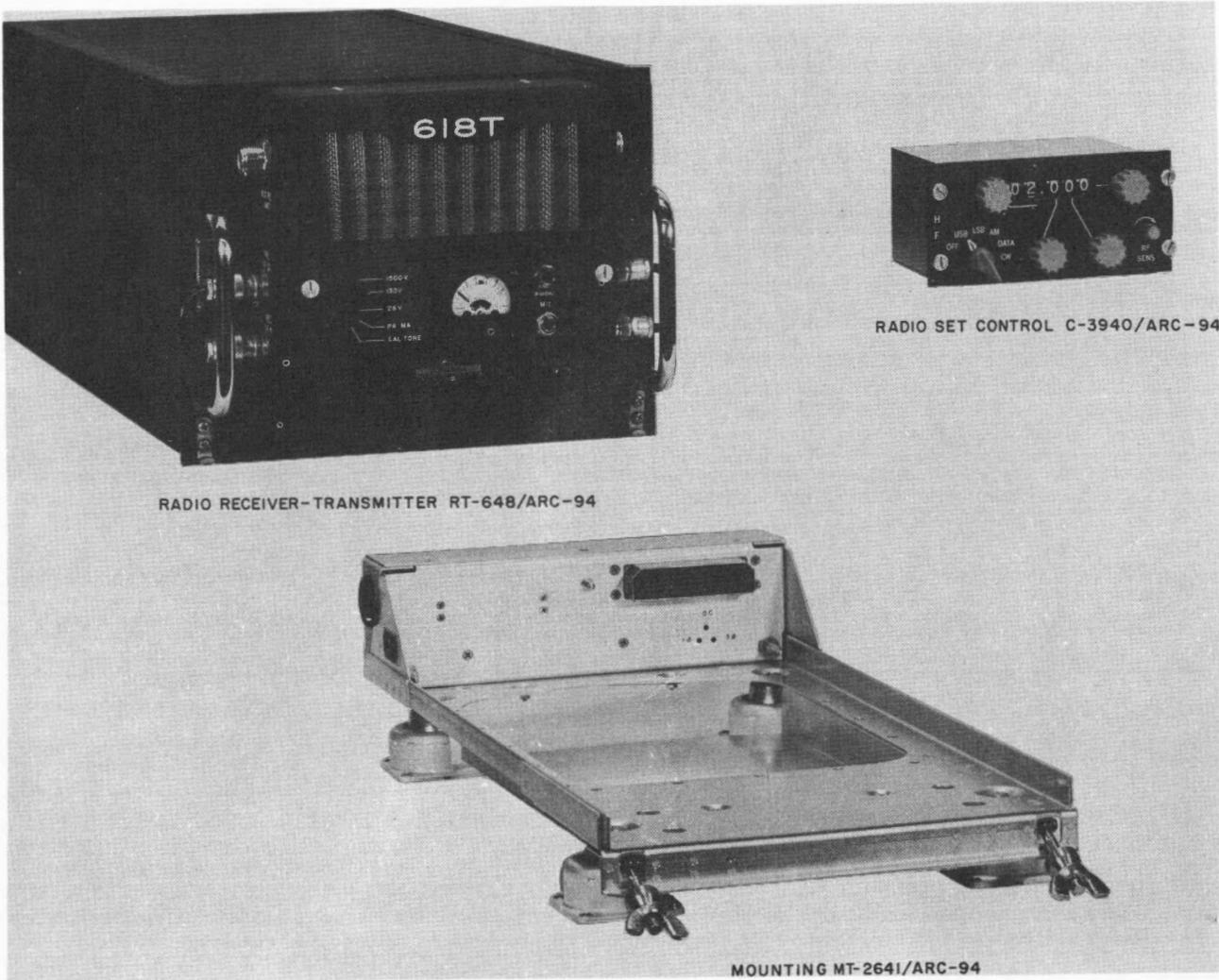
Figure 1-1. Radio Set AN/ARC-94
