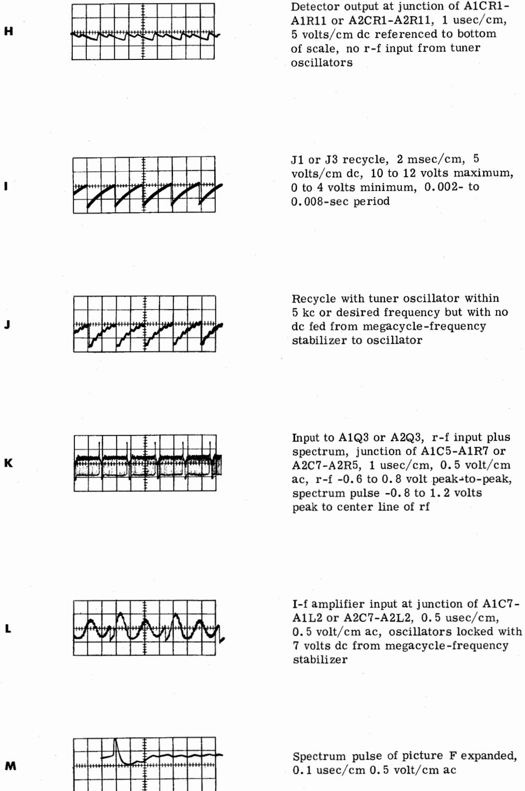
Figure 6-22. Megacycle-Frequency Stabilizer Module A10, Waveforms (Sheet 2 of 2)
