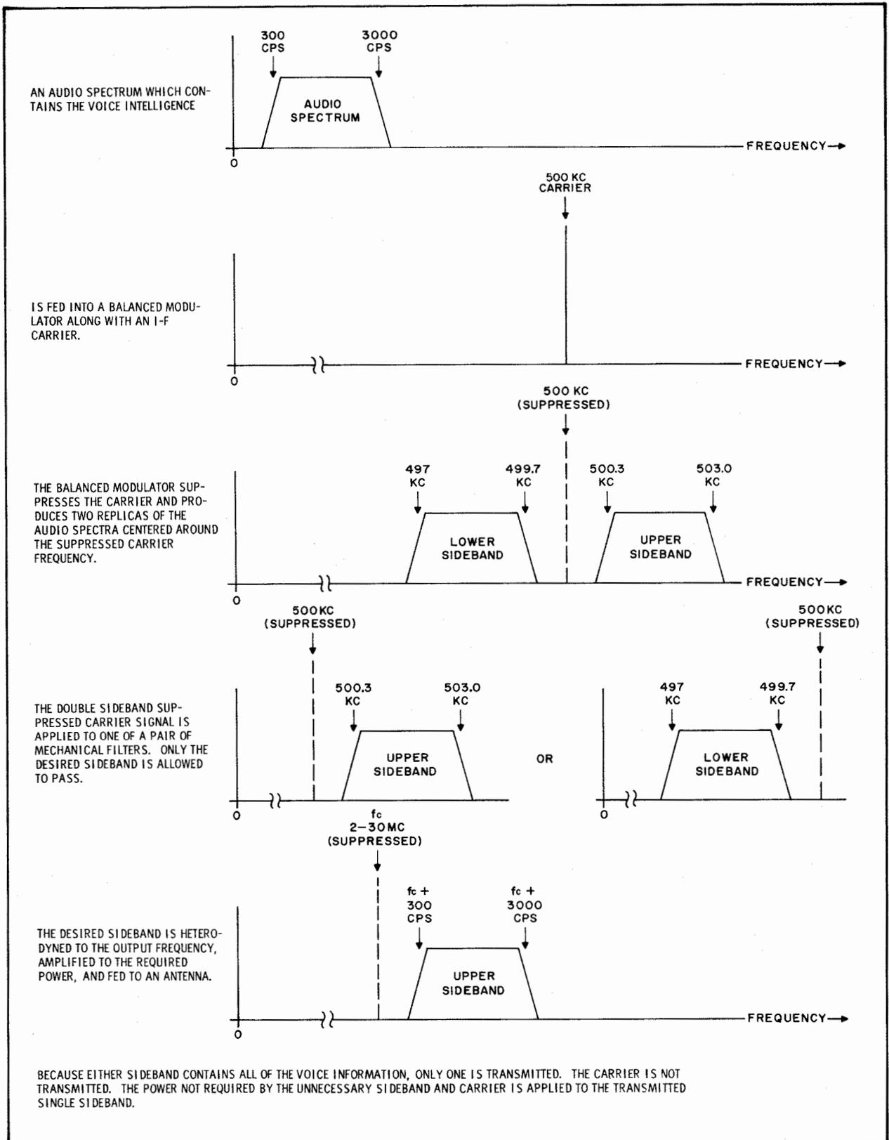
Figure 4-2. SSB Signal Development
