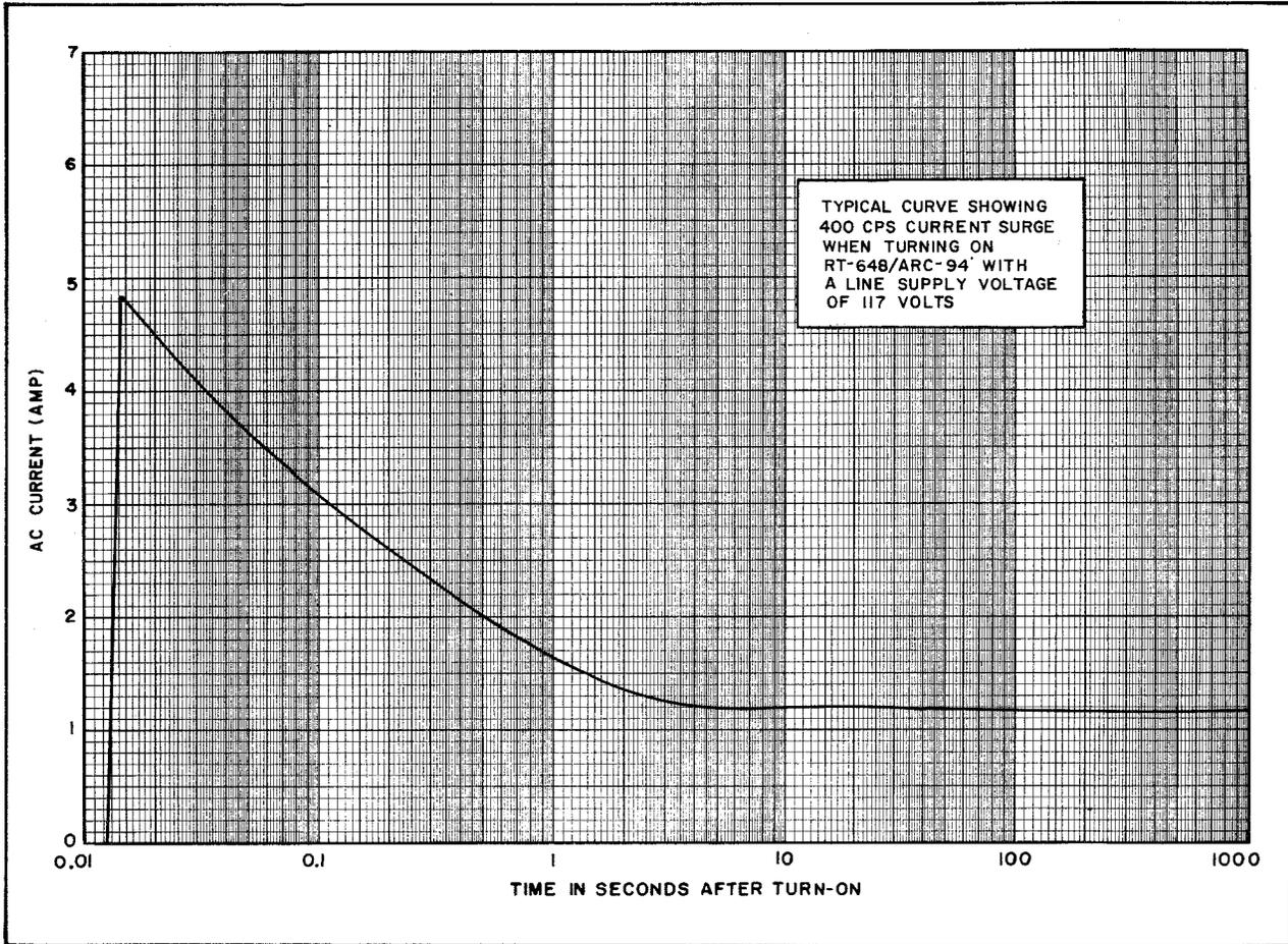
Figure 1-5. Typical A-C Turn-On Surge Current
