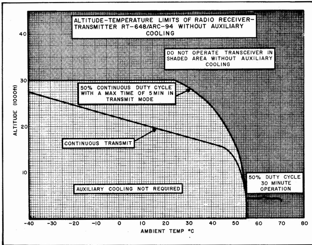
Figure 3-7. Altitude-Temperature Limits
