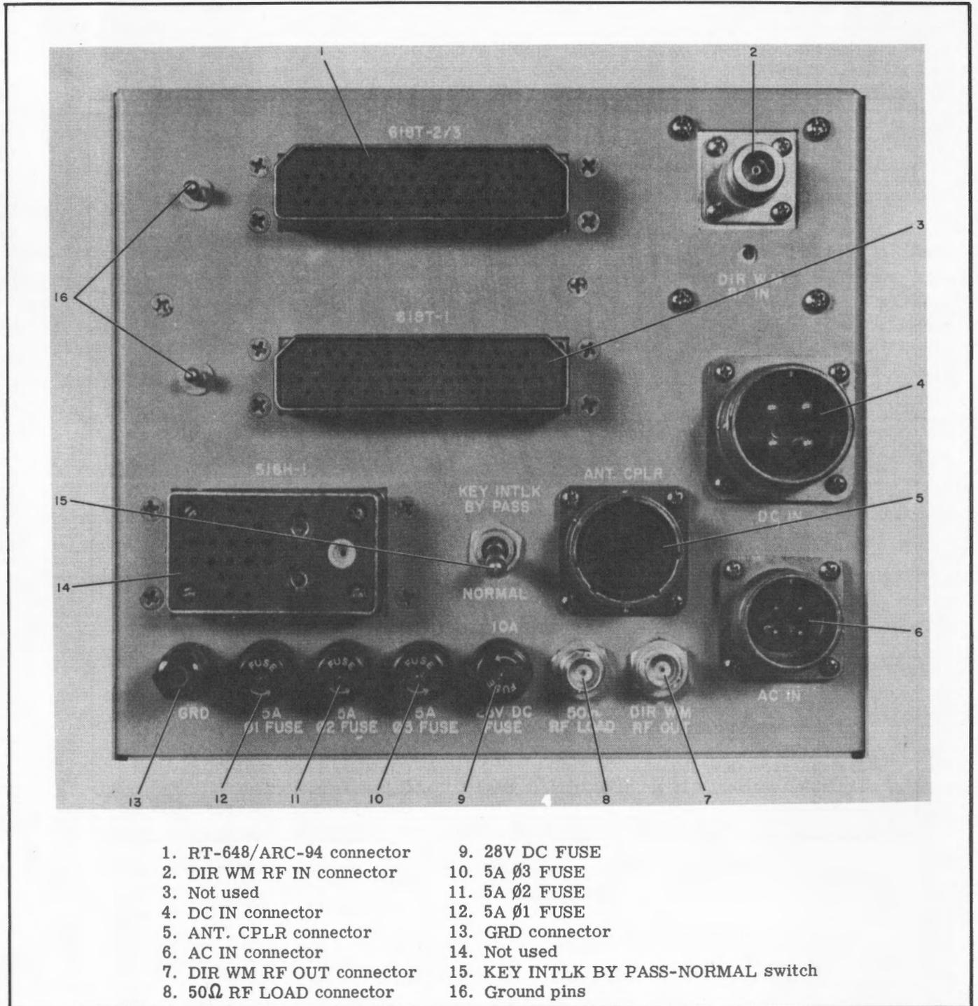
Figure 2-2. Radio Set Test Harness 678P-1, Top Panel
