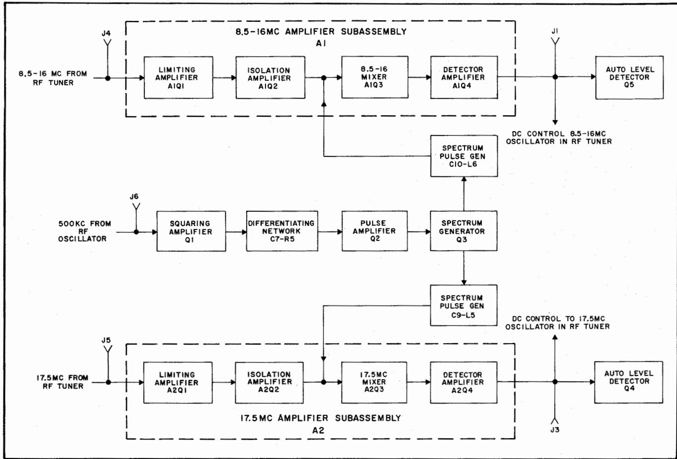
Figure 4-19. Megacycle-Frequency Stabilizer Module A10
