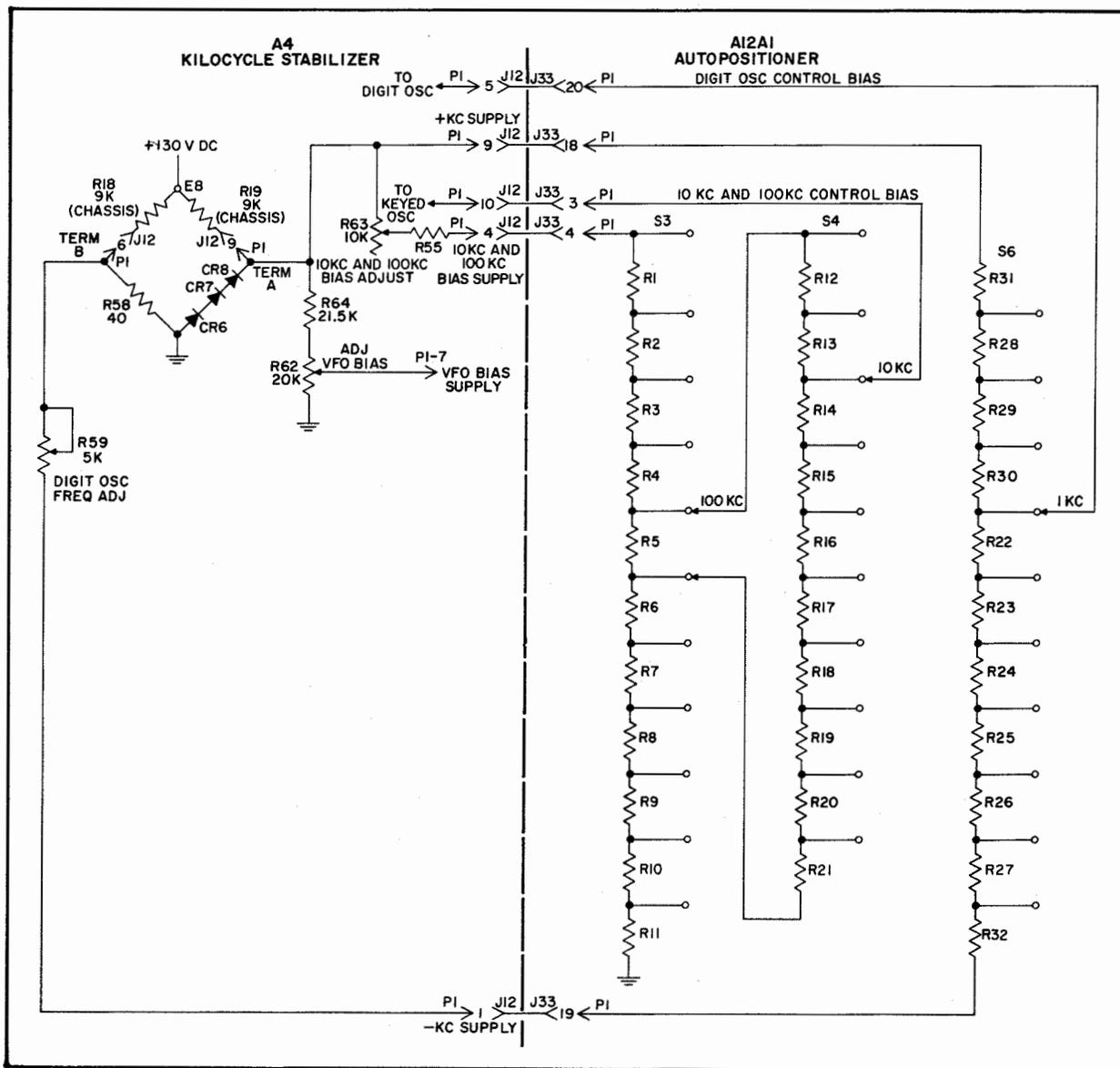
Figure 4-15. Voltage-Stabilizing Bridge Circuit, Simplified Schematic Diagram
