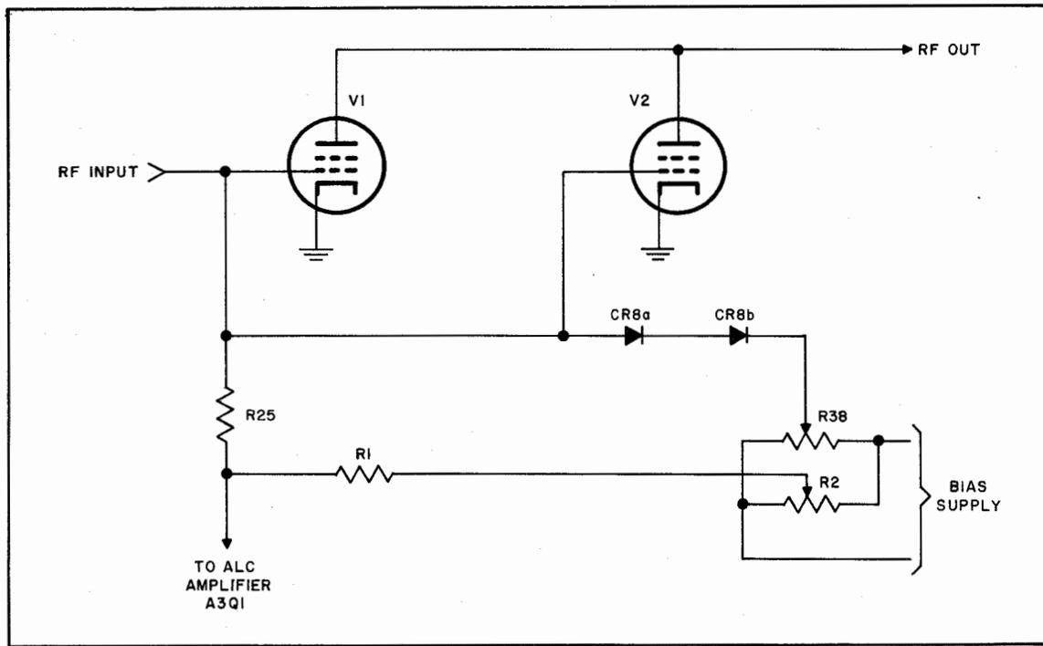
Figure 4-21. PEP Limiter, Simplified Schematic Diagram
