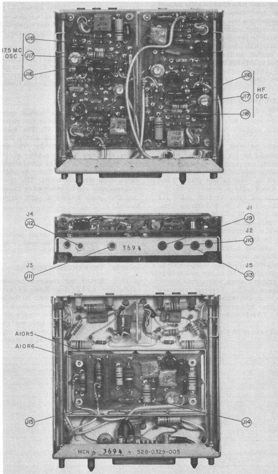
Figure 6-22A. Megacycle-Frequency Stabilizer Module A10 (Collins P/N: 528-0329-005)
