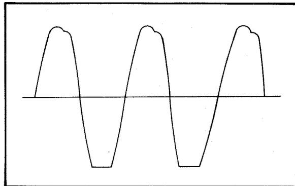
Figure 6-19. Audio Amplifier Distortion Measurement
