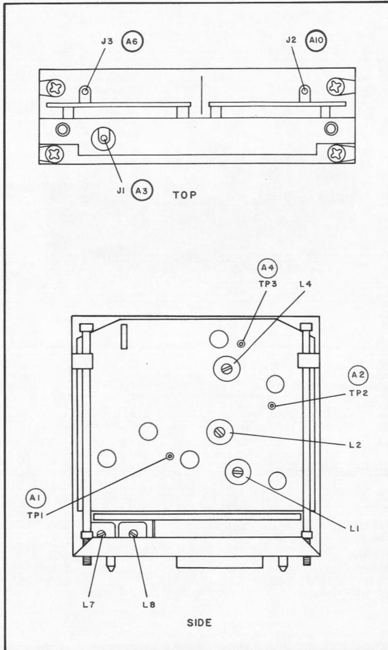
Figure 6-3. Frequency Divider Module A1, Location of Test Points
