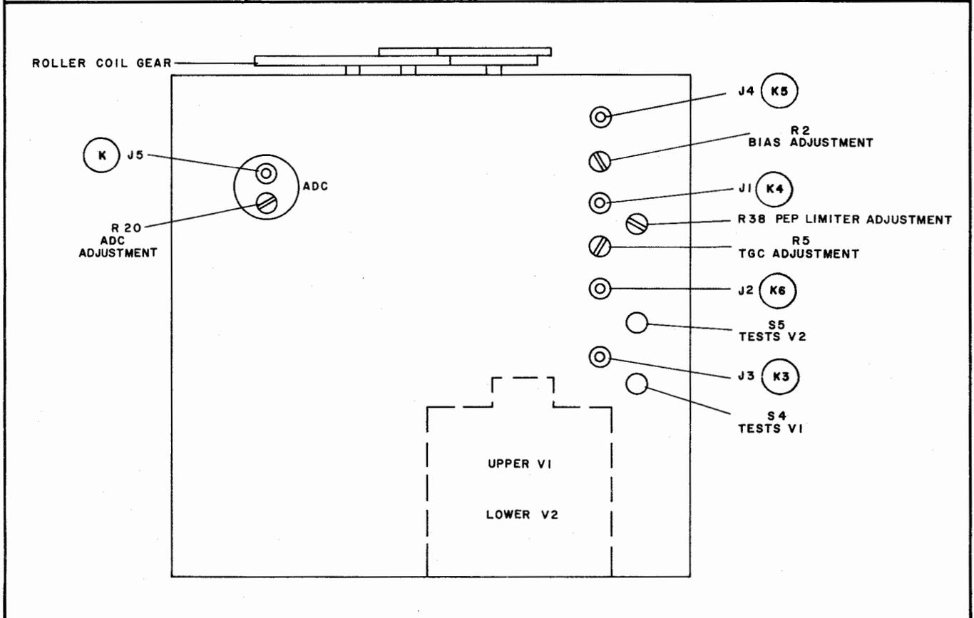
Figure 6-24. Power Amplifier Module A11, List and Location of Test Points
