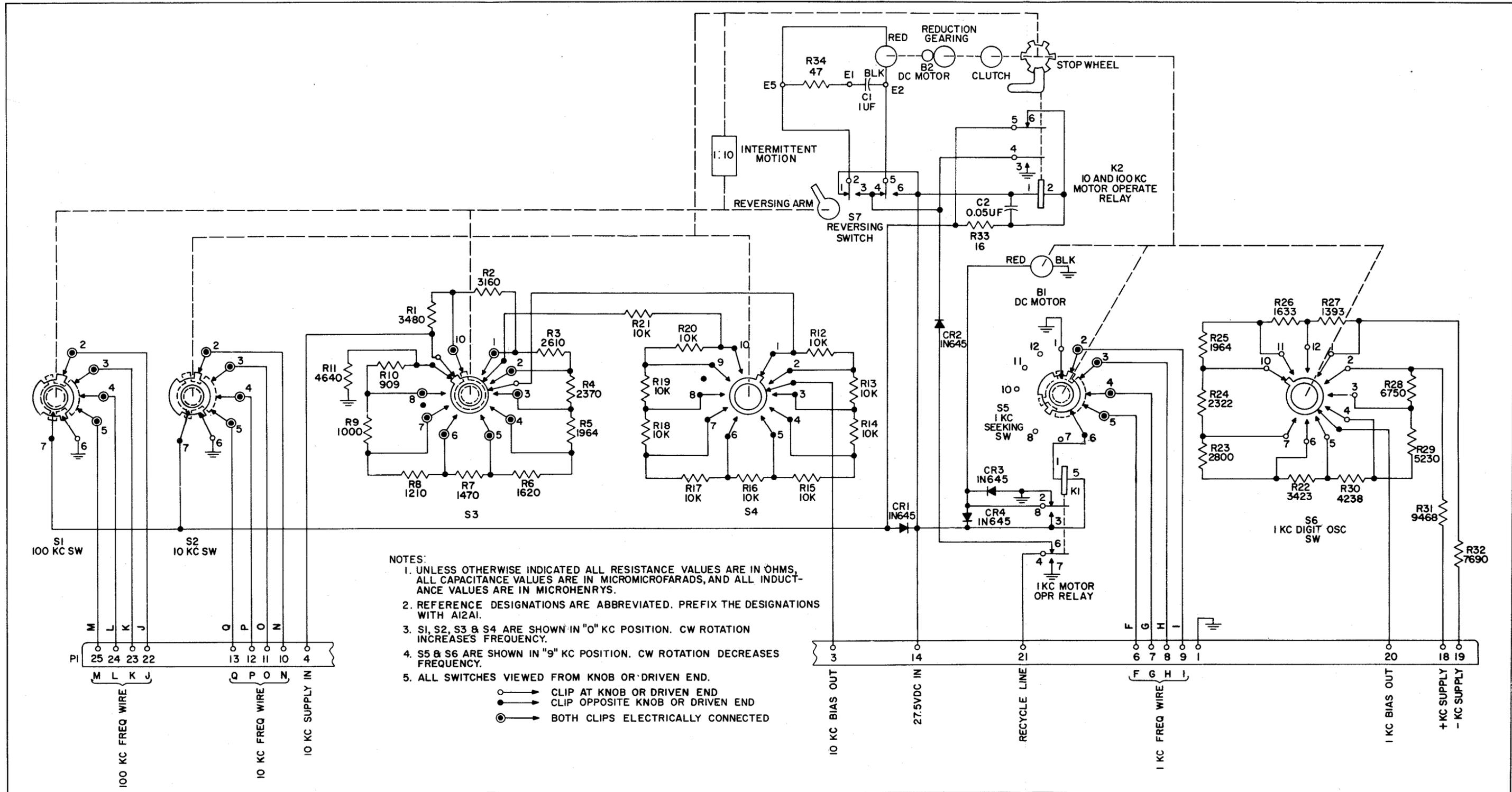
Figure 7-13. Autopositioner Submodule A12A1, Schematic Diagram
