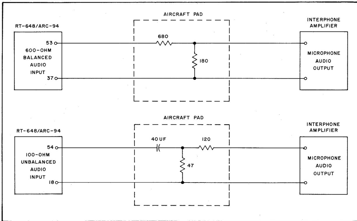
Figure 3-14. Typical Microphone Input Connections
