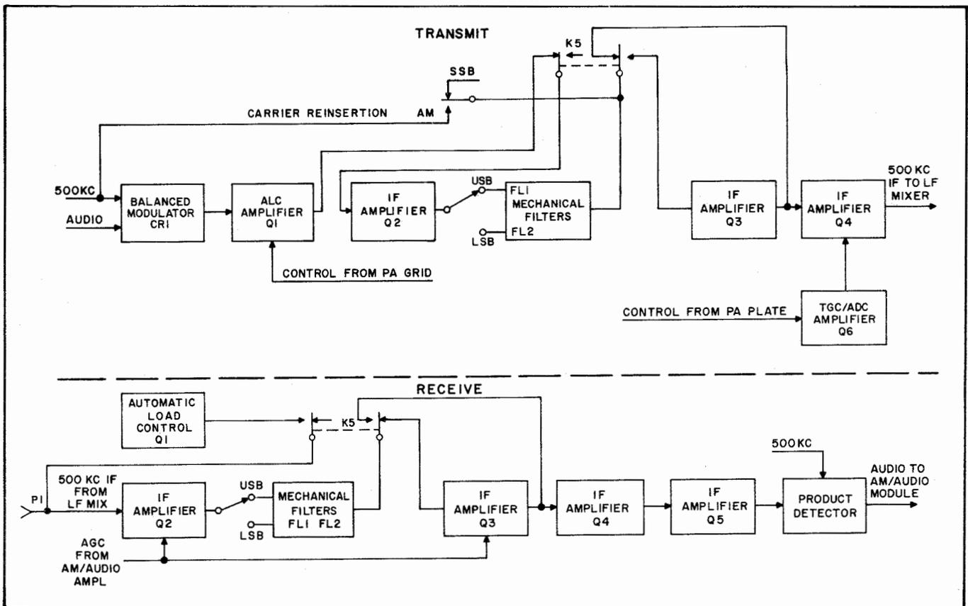
Figure 4-10. I-F Translator Module A3, Block Diagram
