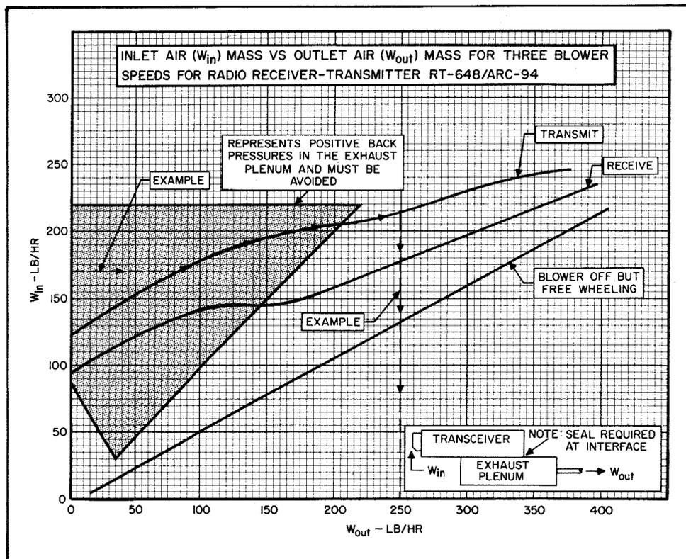
Figure 3-12. Inlet Air Mass Vs Outlet Air Mass
