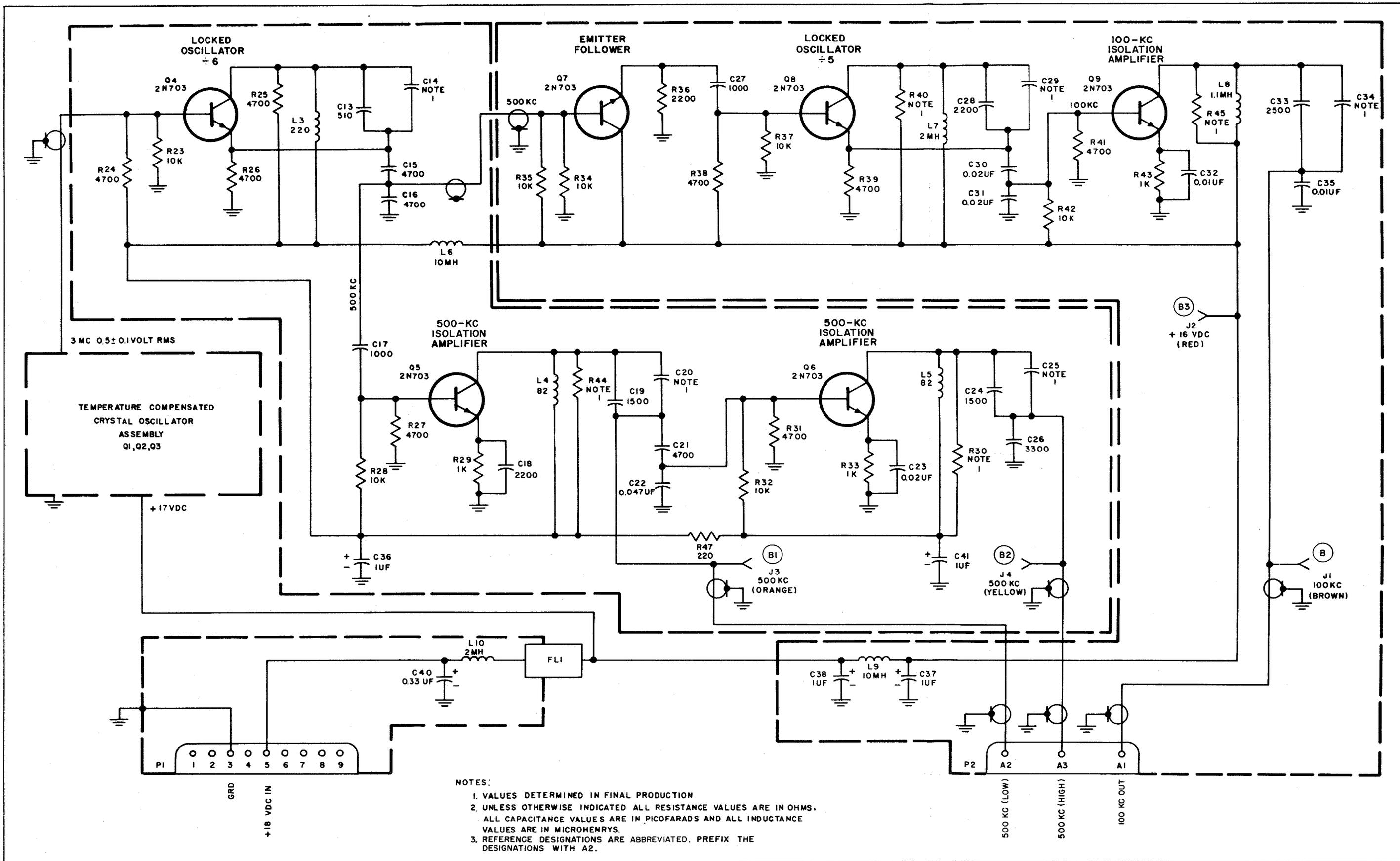
Figure 7-3. R-F Oscillator Module A2, Schematic Diagram
