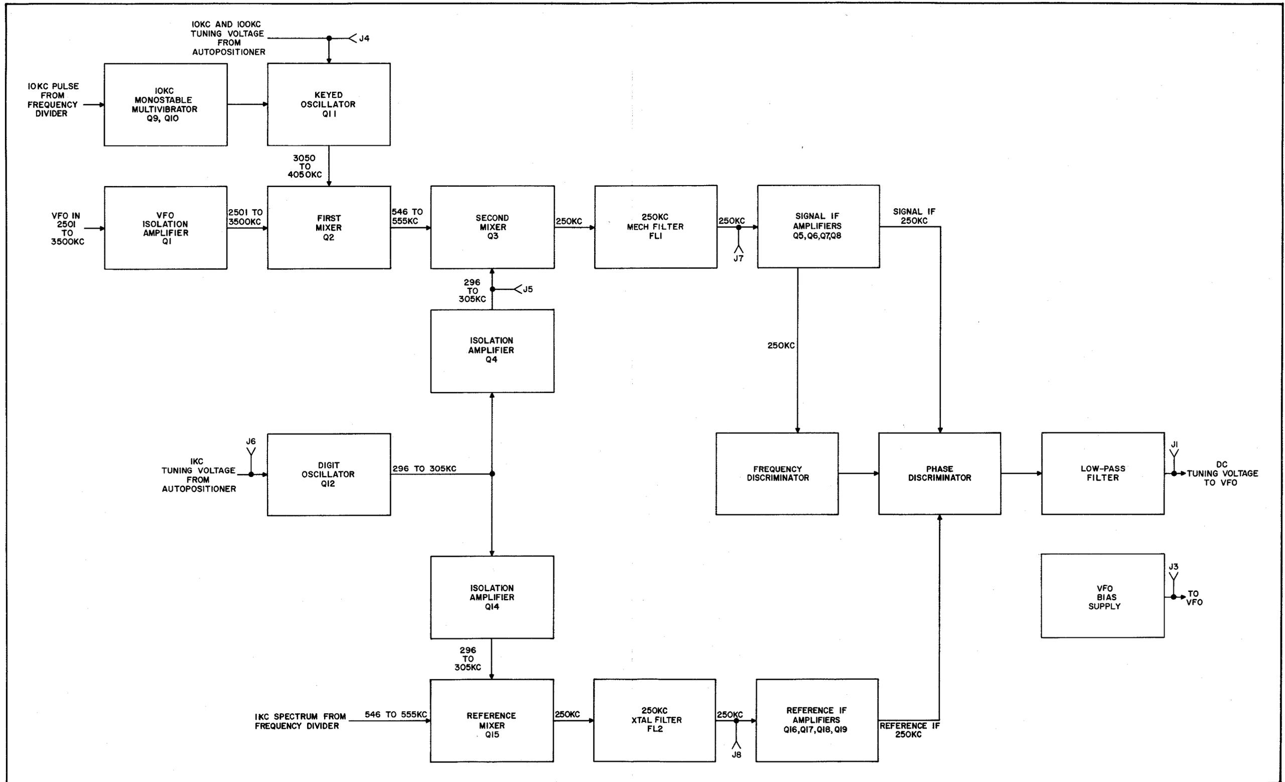
Figure 4-14. Kilocycle-Frequency Stabilizer Module A4, Block Diagram
