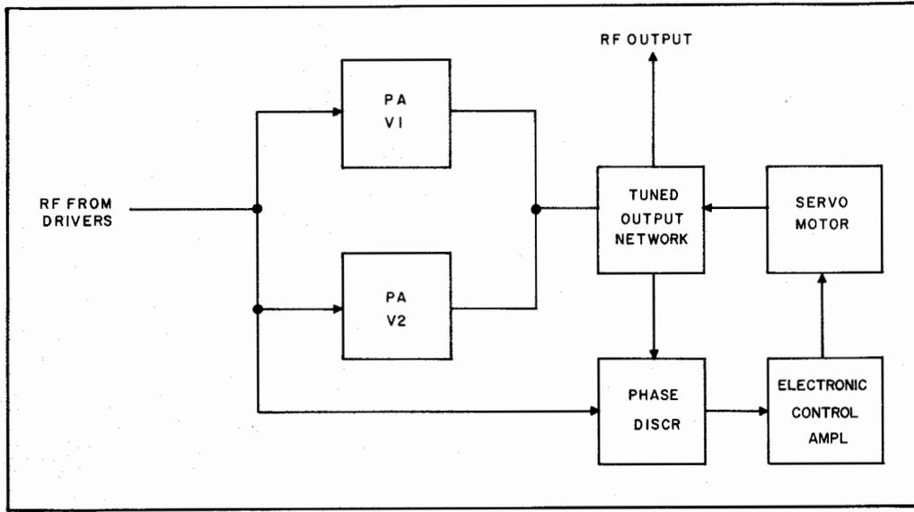
Figure 4-20. Power Amplifier Module A11, Block Diagram
