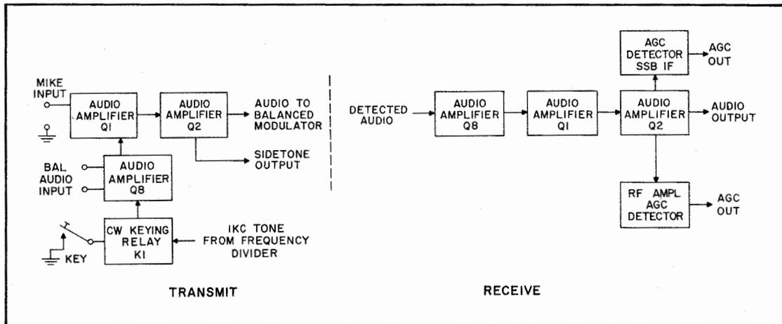
Figure 4-17. Audio Amplifier Stages in AM/Audio Amplifier Module A9, Block Diagram
