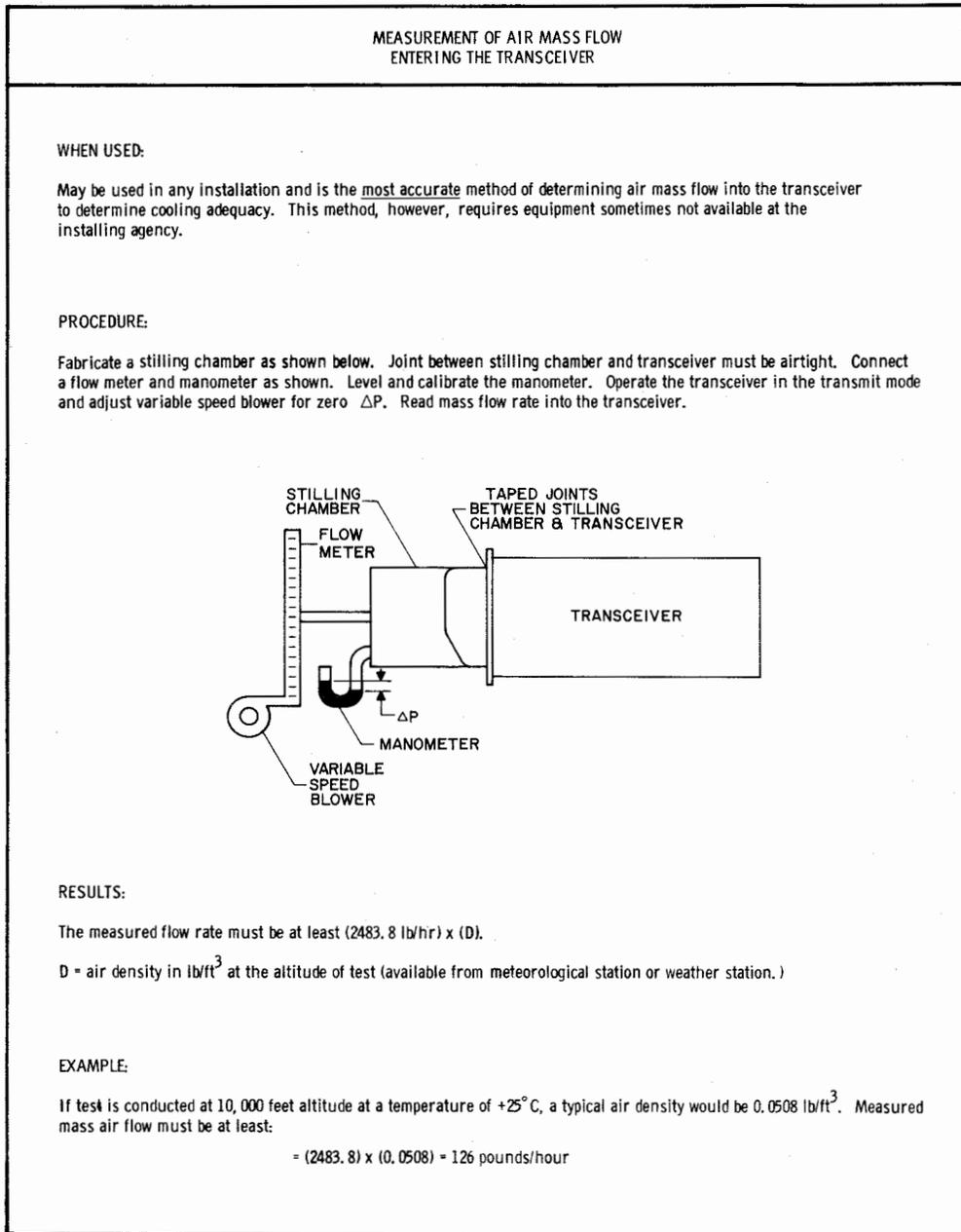
Figure 3-8. Measurement of Air Mass Flow Entering
