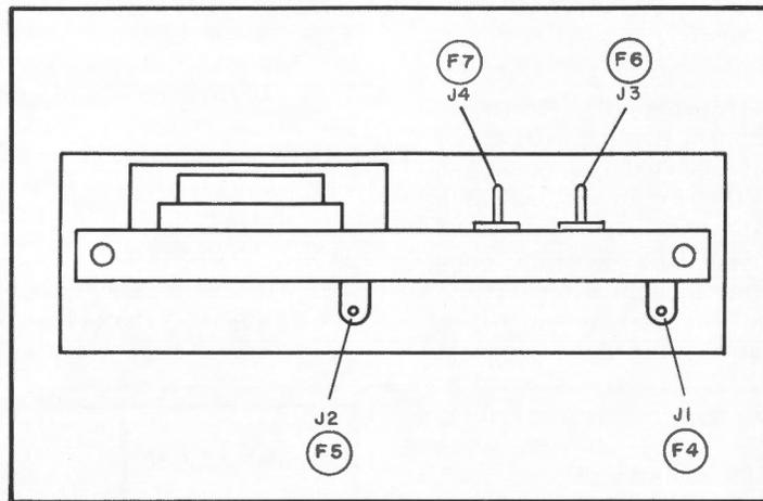
Figure 6-15. Electronic Control Amplifier Module A6, Location of Test Points
