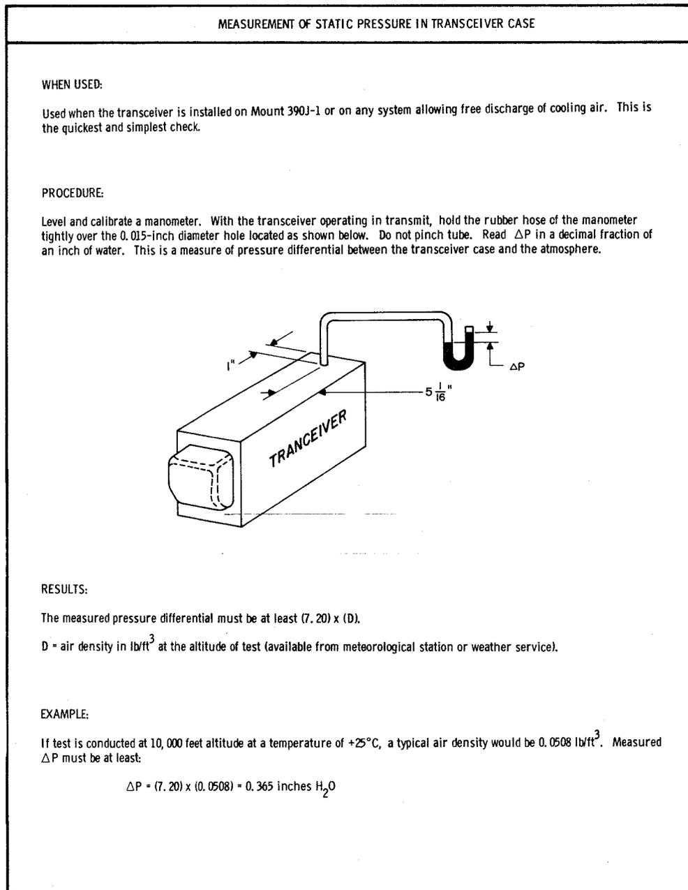
Figure 3-9. Measurement of Static Pressure in Radio Receiver-Transmitter RT-648/ARC-94 Case
