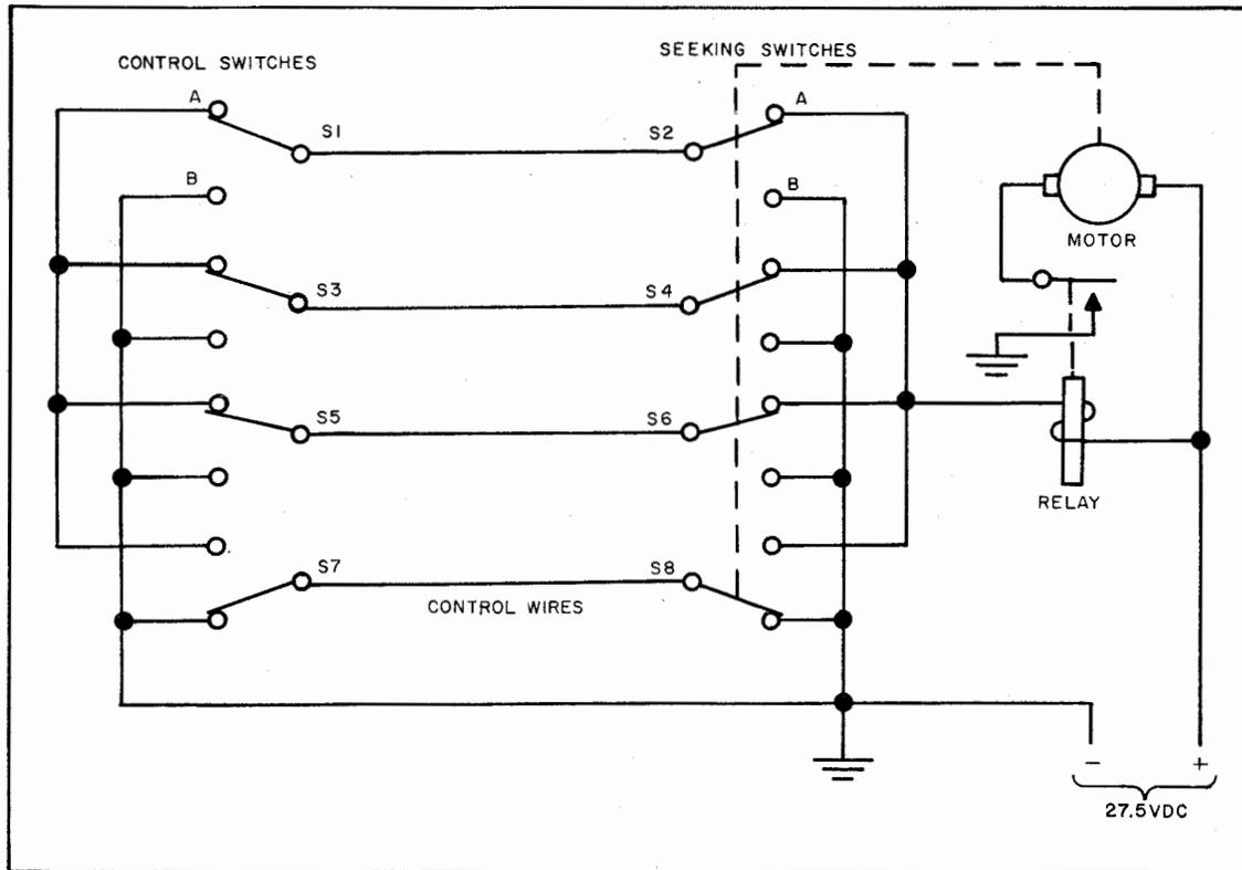
Figure 4-26. Frequency Control System, Simplified Schematic Diagram
