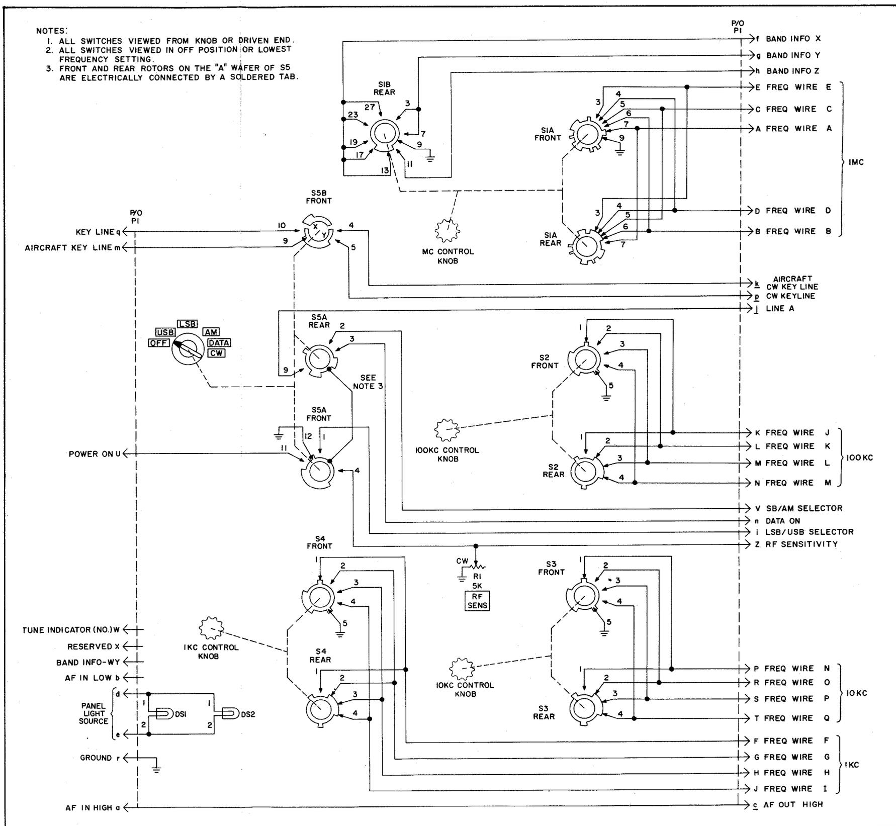
Figure 7-15. Radio Set Control C-3940/ARC-94, Schematic Diagram
