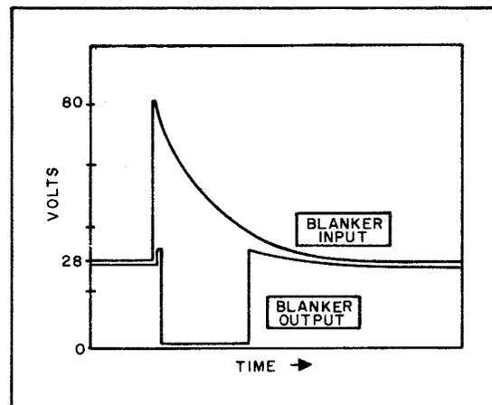
Figure 4-16. Transient Blanker
