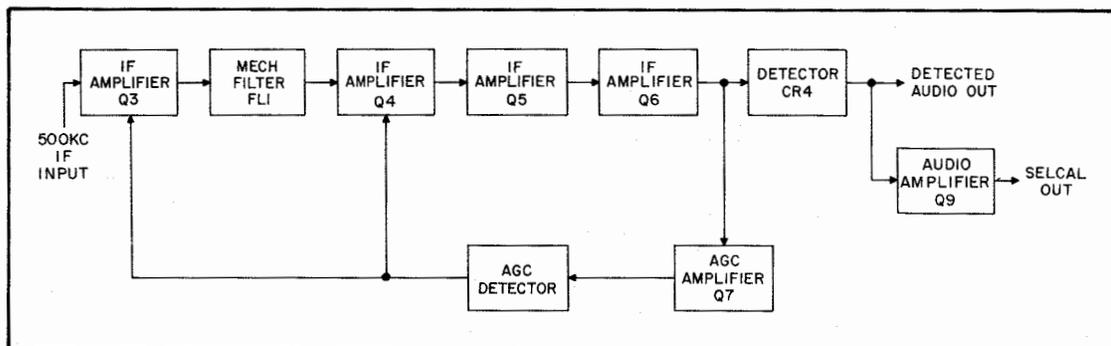
Figure 4-18. AM/Audio Amplifier Module A9, Block Diagram
