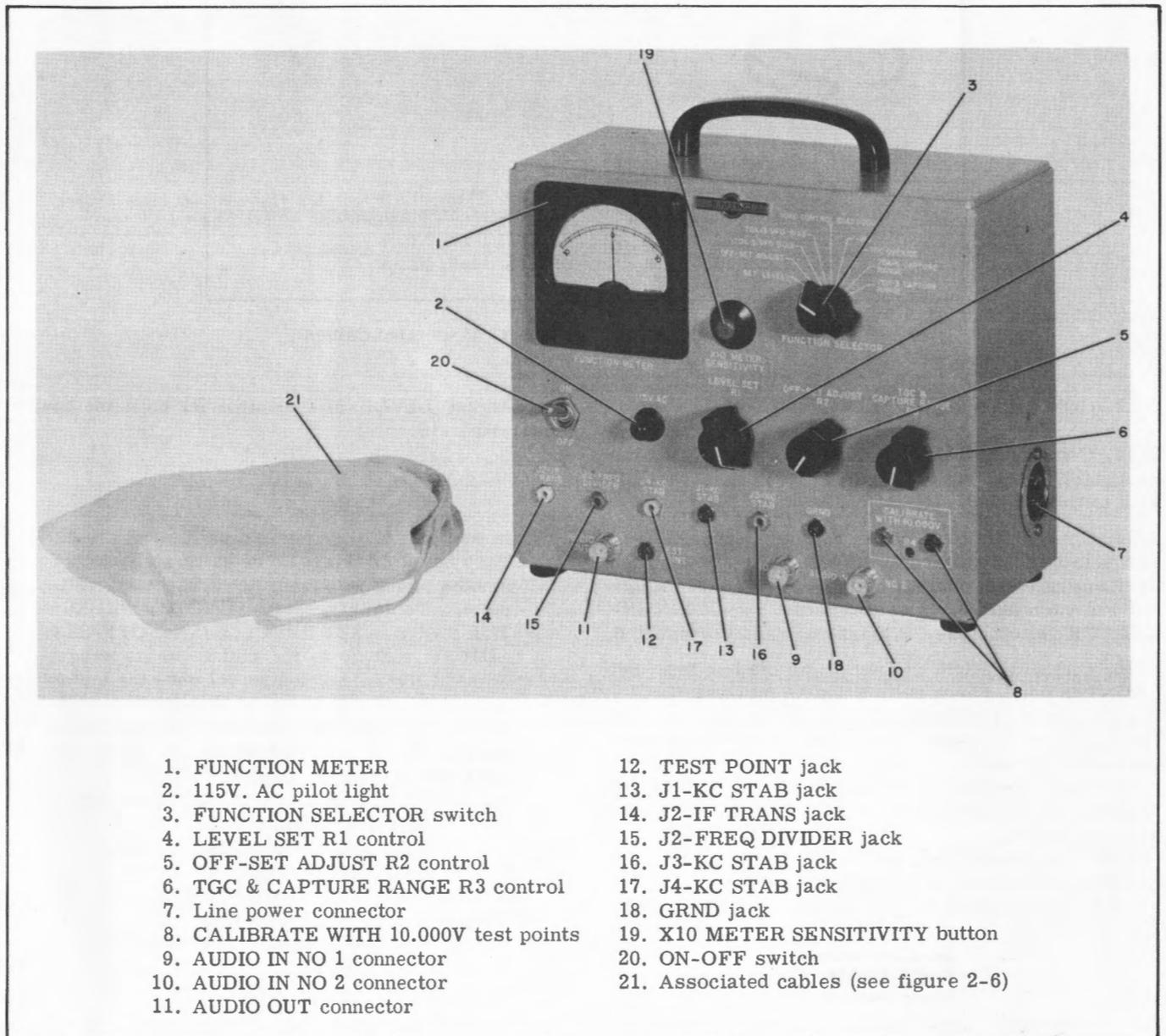
Figure 2-5. Radio Test Set 678Z-1, Front Panel
