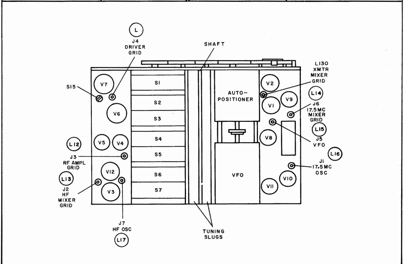
Figure 6-27. RF Translator Module A12, List and Location of Test Points
