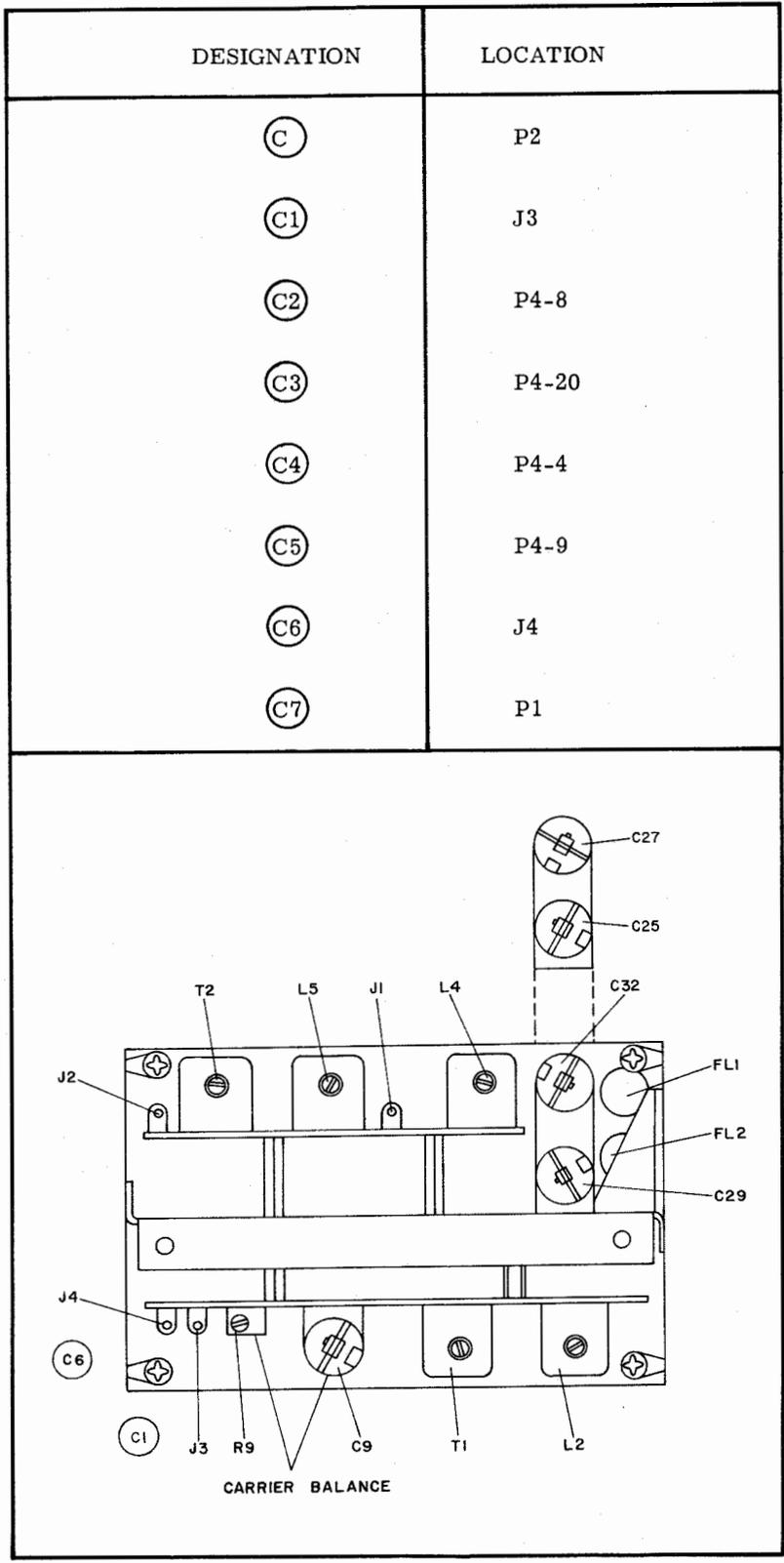
Figure 6-8. I-F Translator Module A3, List and Location of Test Points
