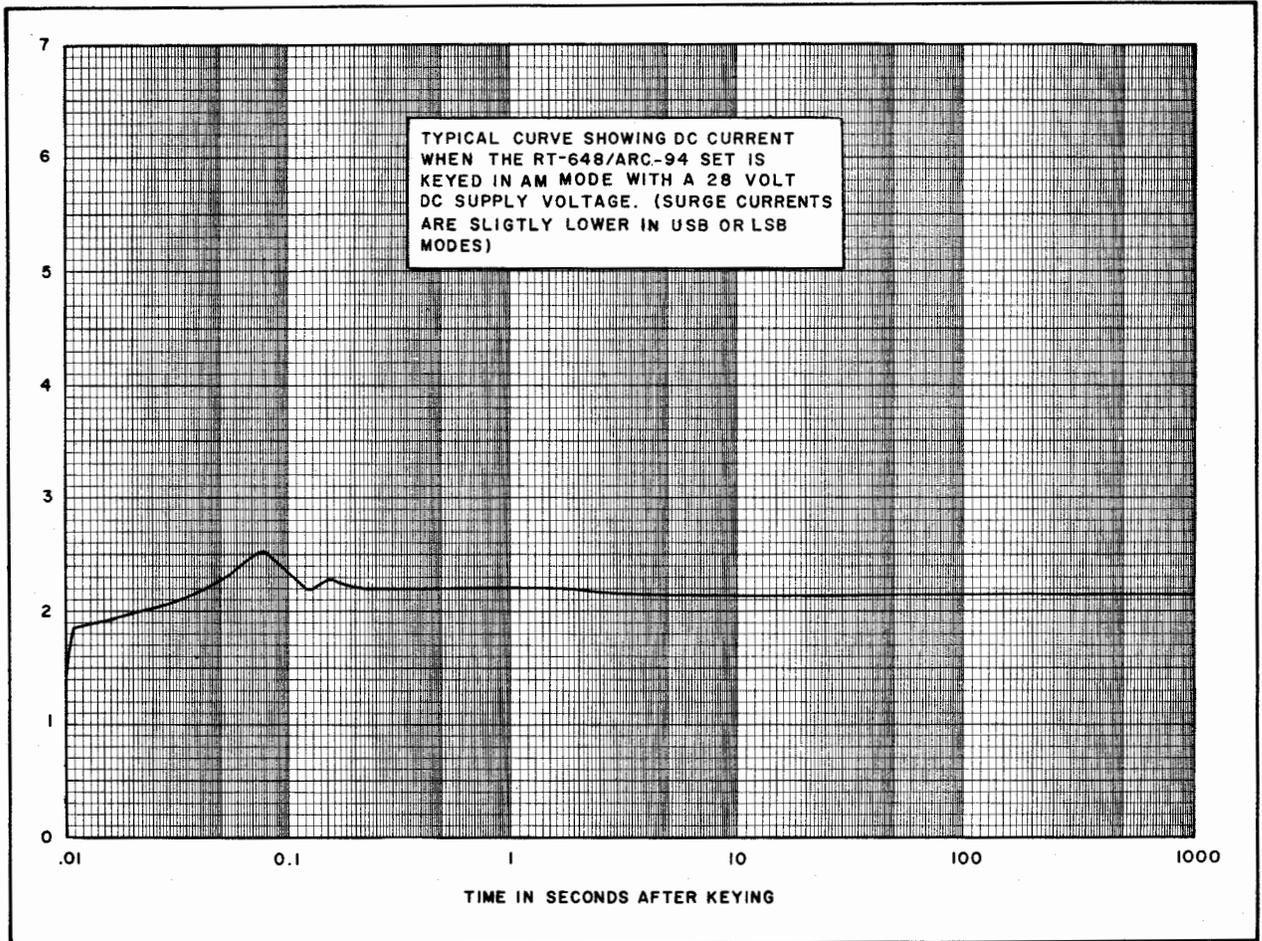
Figure 1-4. Typical D-C Transmitter Keying Surge Current
