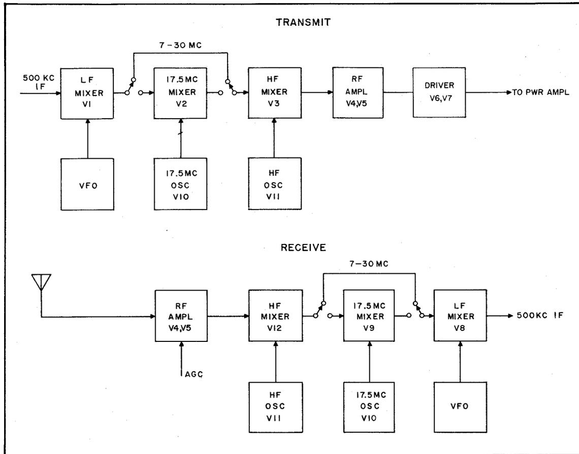
Figure 4-23. R-F Translator Module A12, Block Diagram
