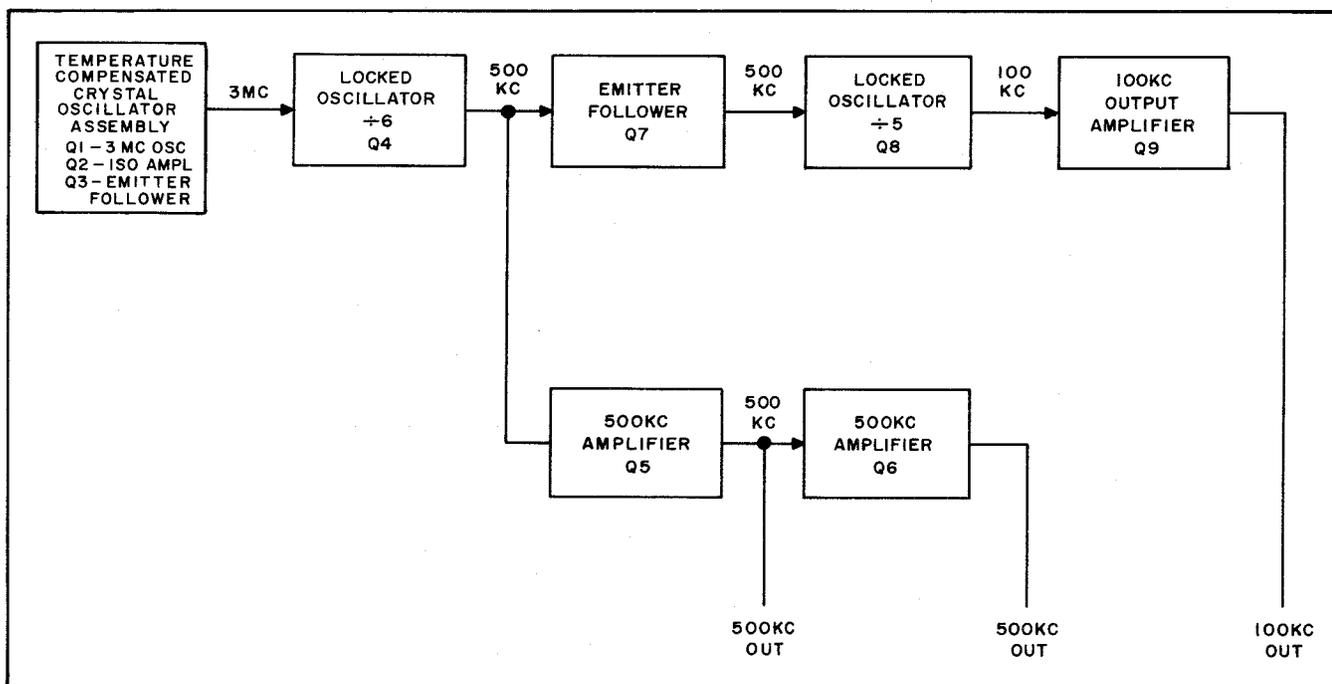
Figure 4-9. R-F Oscillator Module A2, Block Diagram
