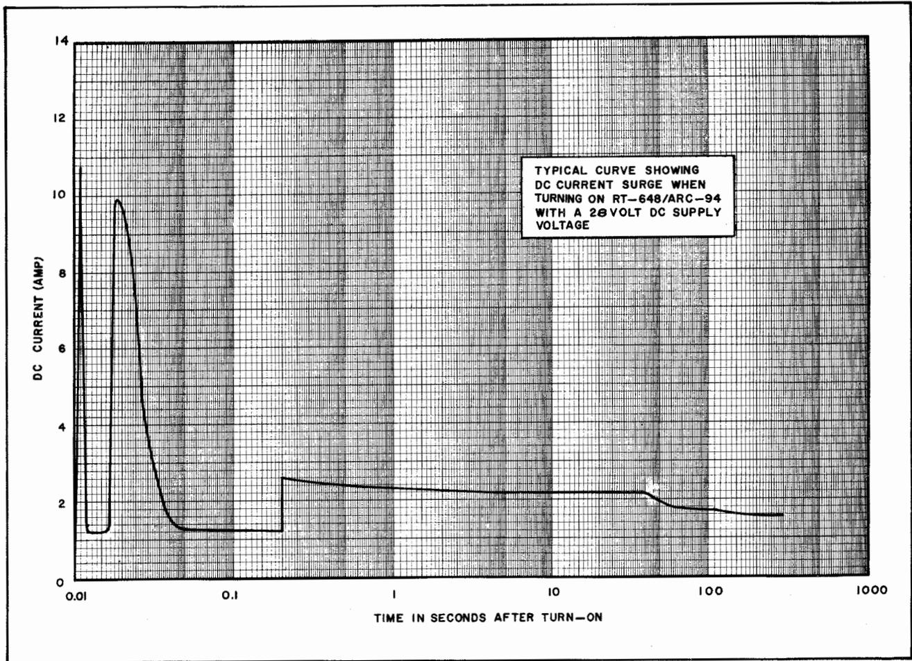
Figure 1-3. Typical D-C Turn-On Surge Current
