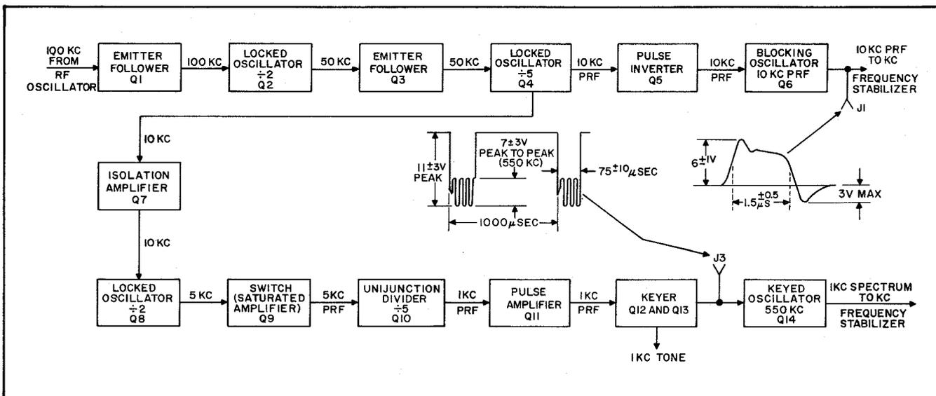
Figure 4-8. Frequency Divider Module A1, Block Diagram
