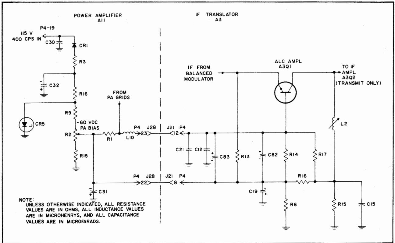
Figure 4-12. Automatic Load Control, Simplified Schematic Diagram
