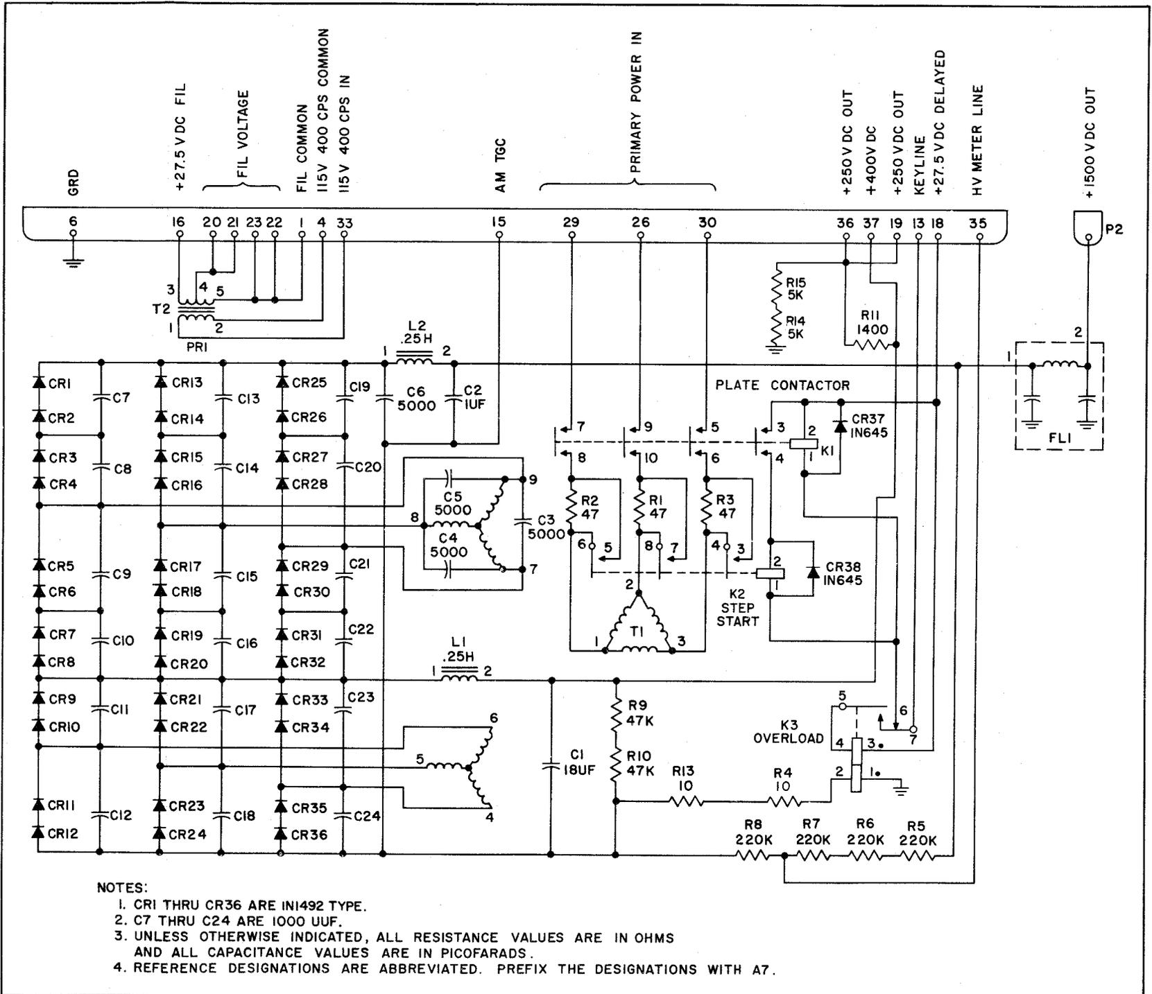
Figure 7-8. Three-Phase High-Voltage Power Supply Module A7, Schematic Diagram
