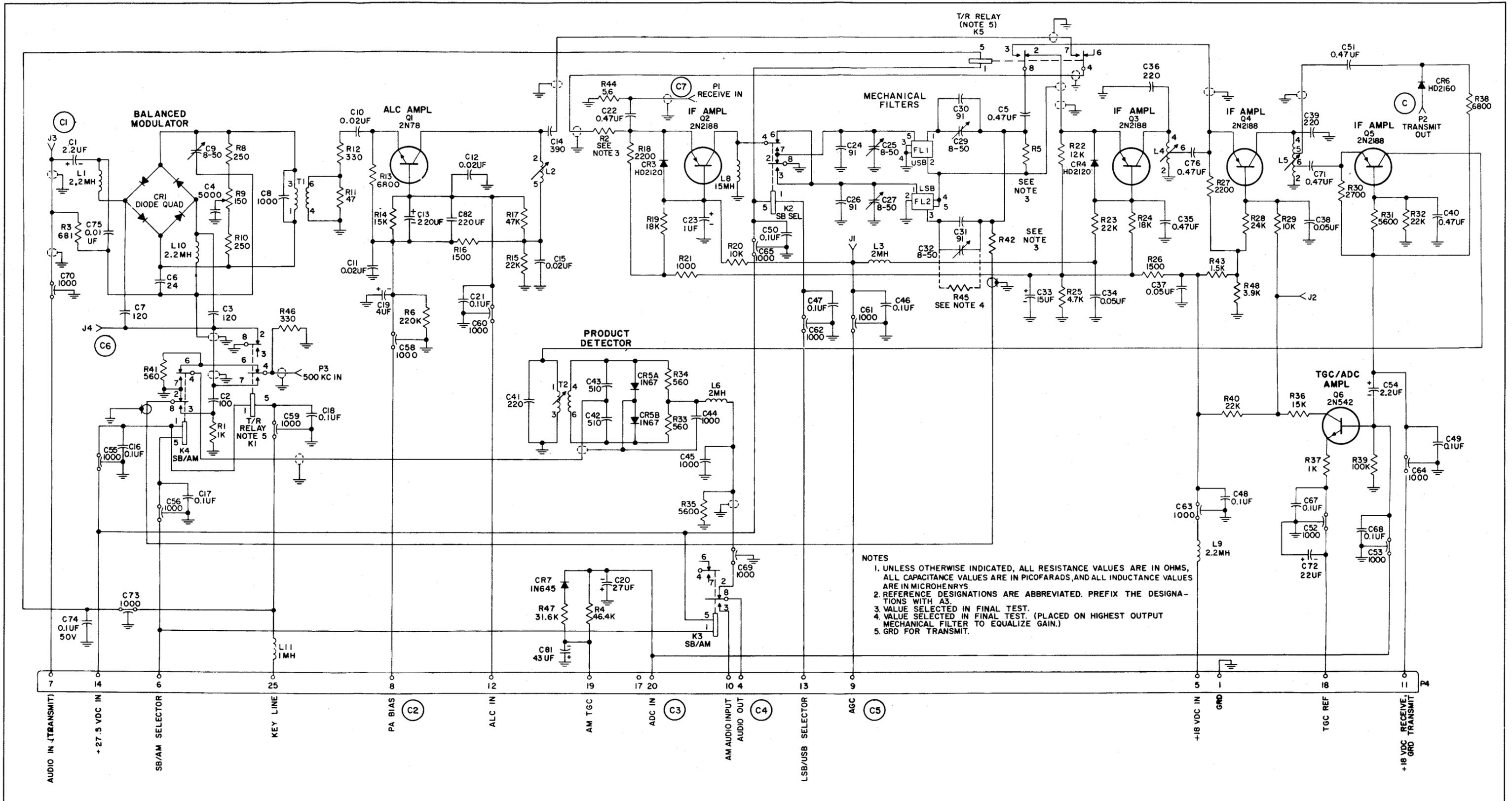
Figure 7-4. I-F Translator Module A3, Schematic Diagram
