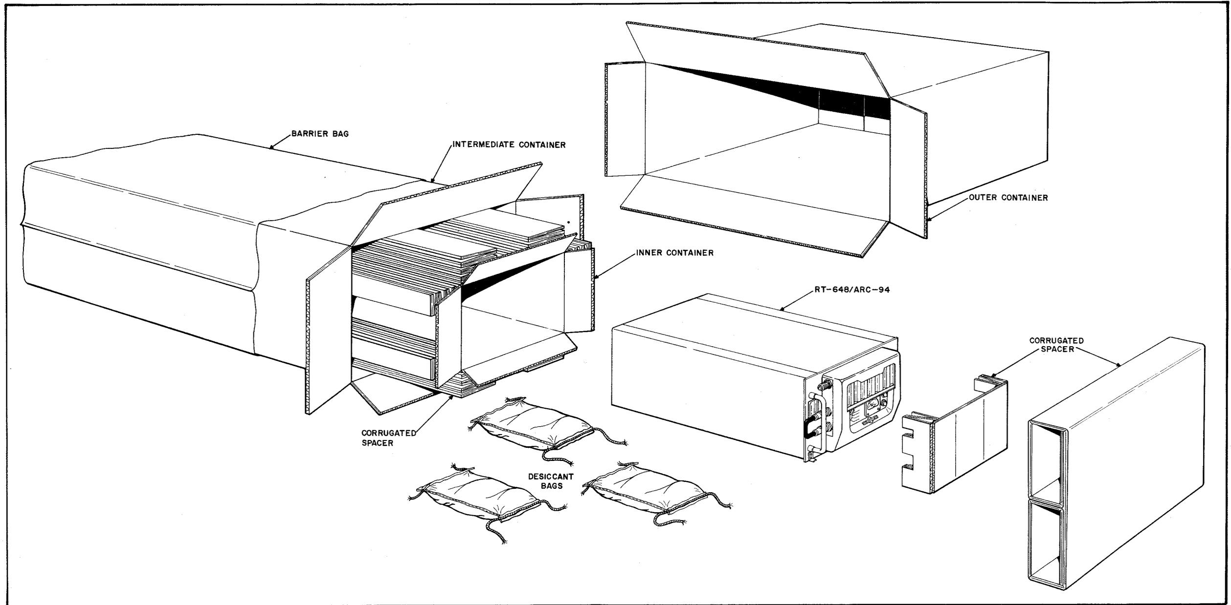
Figure 3-3. Packaging Details, Radio Receiver-Transmitter RT-648/ARC-94
