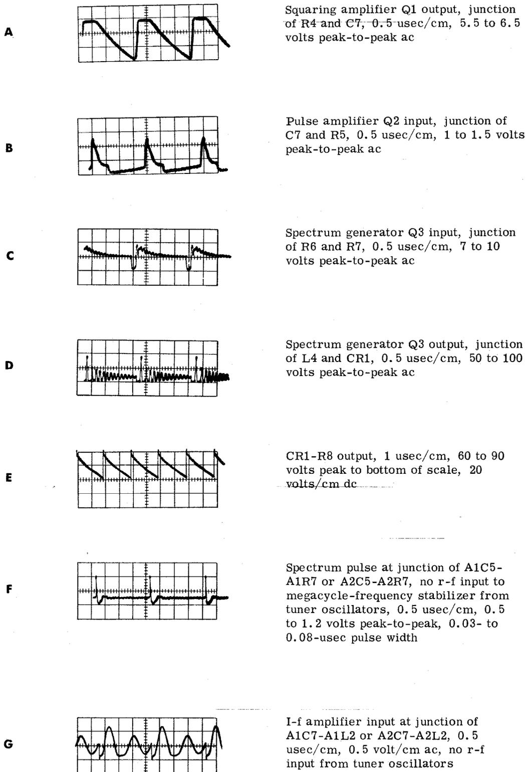
Figure 6-22. Megacycle-Frequency Stabilizer Module A10, Waveforms (Sheet 1 of 2)
