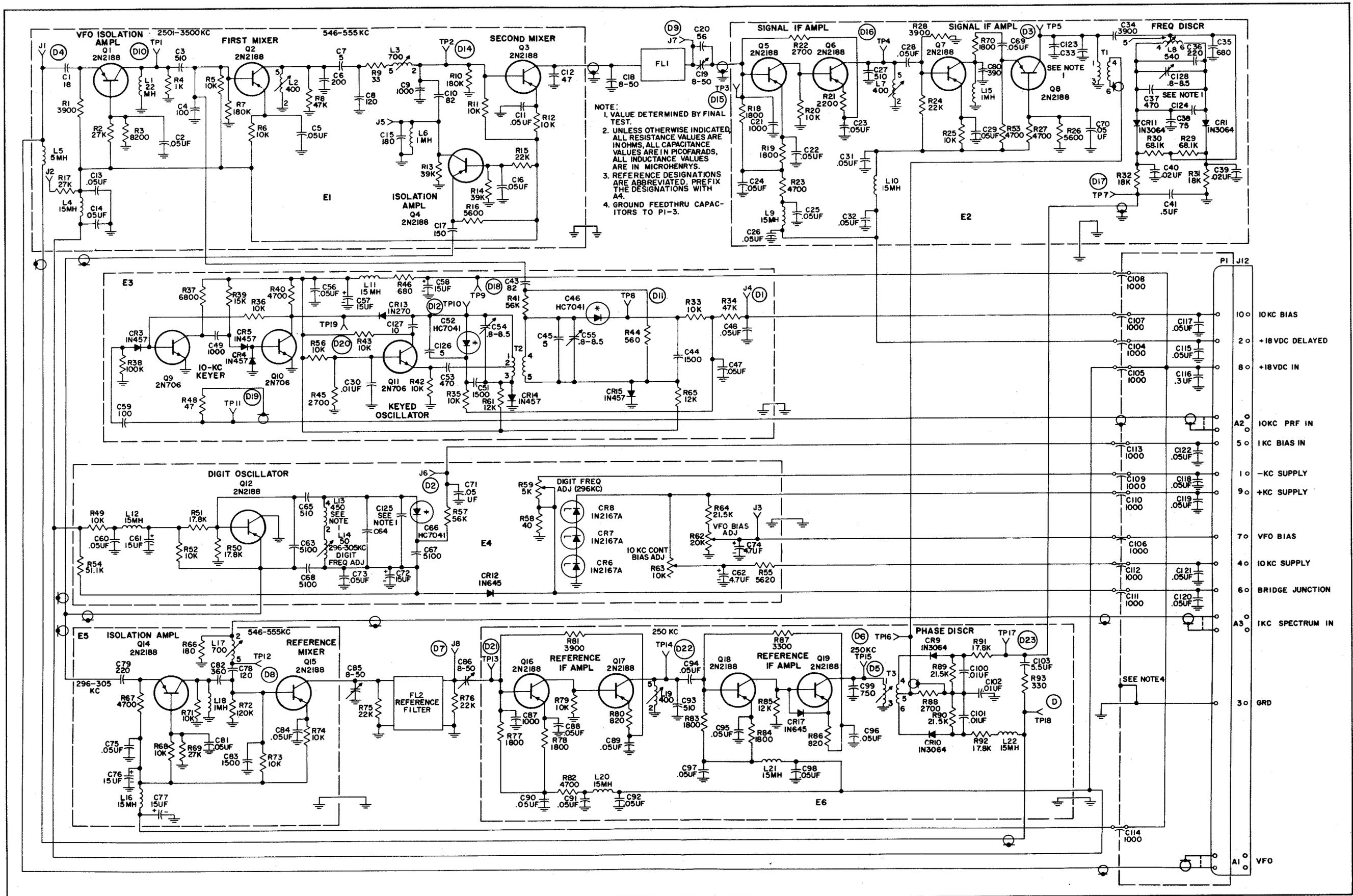
Figure 7-5. Kilocycle-Frequency Stabilizer Module A4, Schematic Diagram
