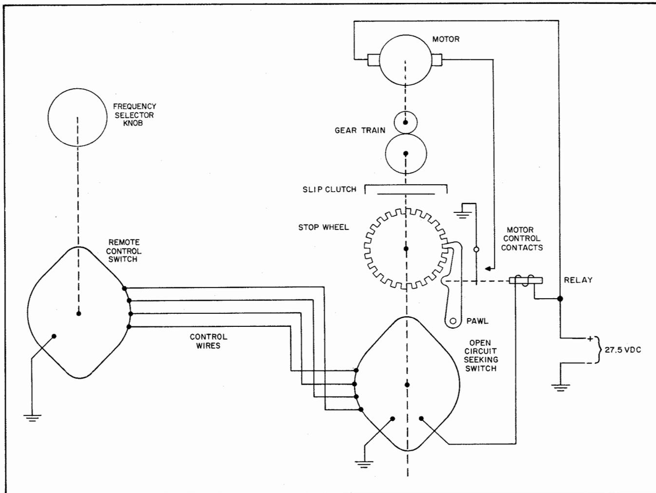
Figure 4-25. Autopositioner System, Basic Elements, Simplified Schematic Diagram
