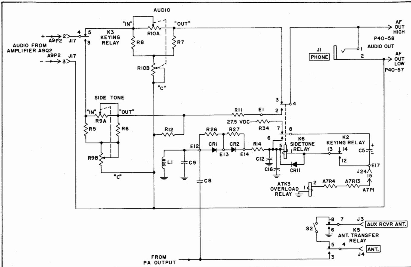
Figure 4-6. Sidetone Circuits, Simplified Schematic Diagram
