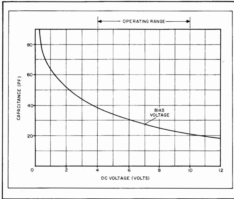
Figure 4-24. Typical Characteristics of Voltage-Sensitive Capacitor
