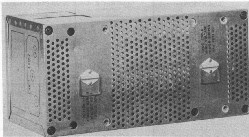
**THREE-PHASE HIGH-VOLTAGE POWER SUPPLY MODULE**
