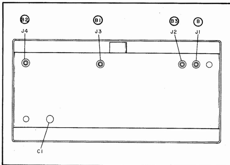
Figure 6-6. R-F Oscillator Module A2, Location of Test Points
