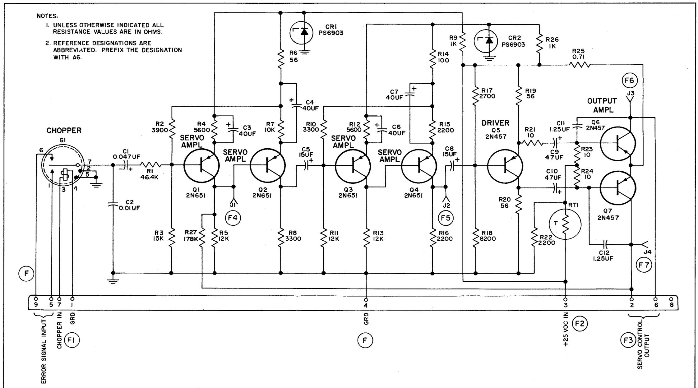
Figure 7-7. Electronic Control Amplifier Module A6, Schematic Diagram
