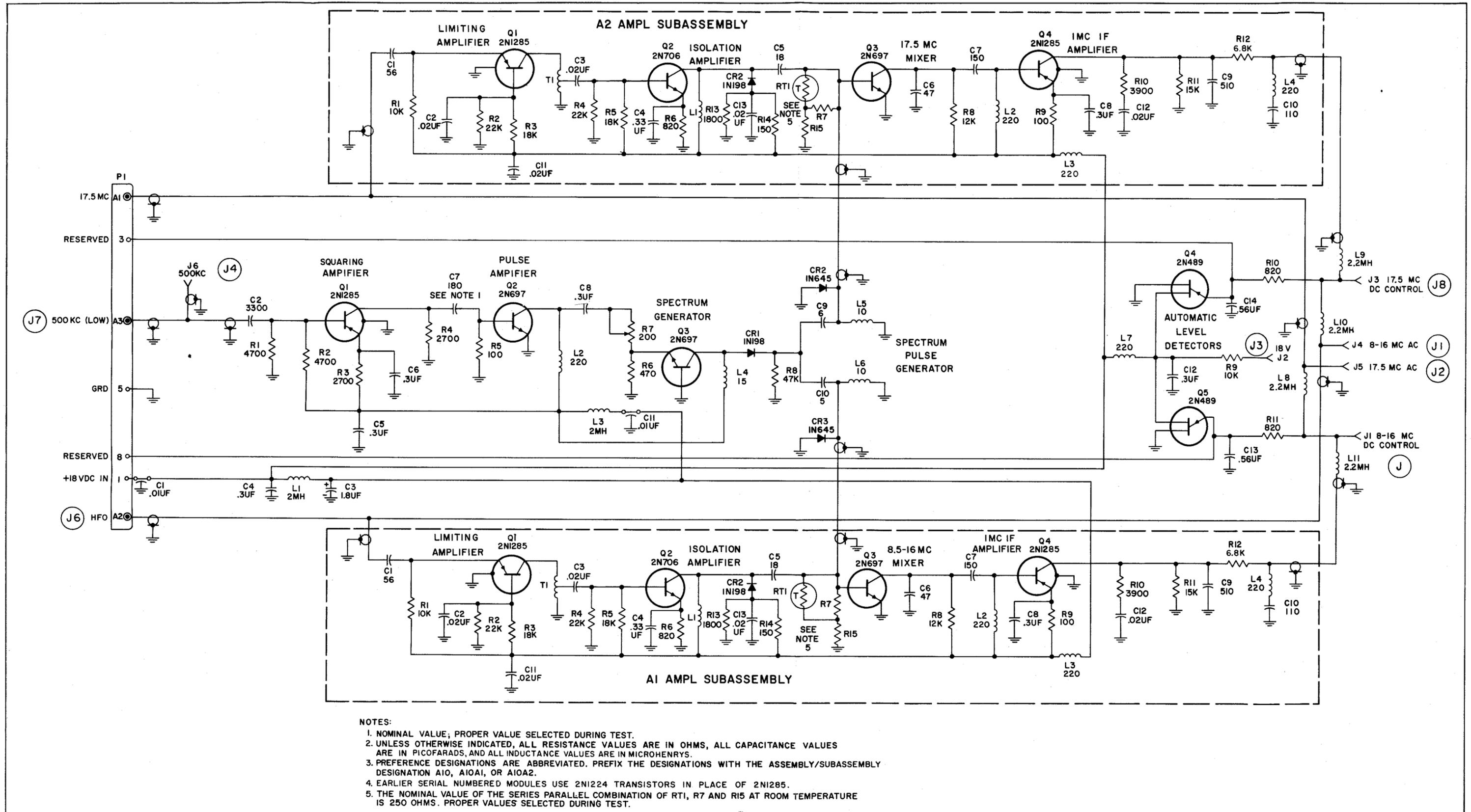
Figure 7-10. Megacycle-Frequency Stabilizer Module A10 (Collins P/N: 544-9289-005), Schematic Diagram
