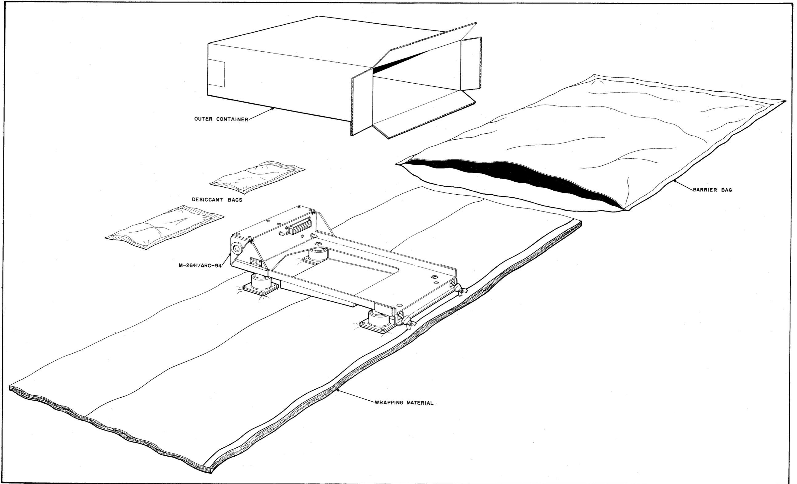
Figure 3-2. Packaging Details, Mounting MT-2641/ARC-94
