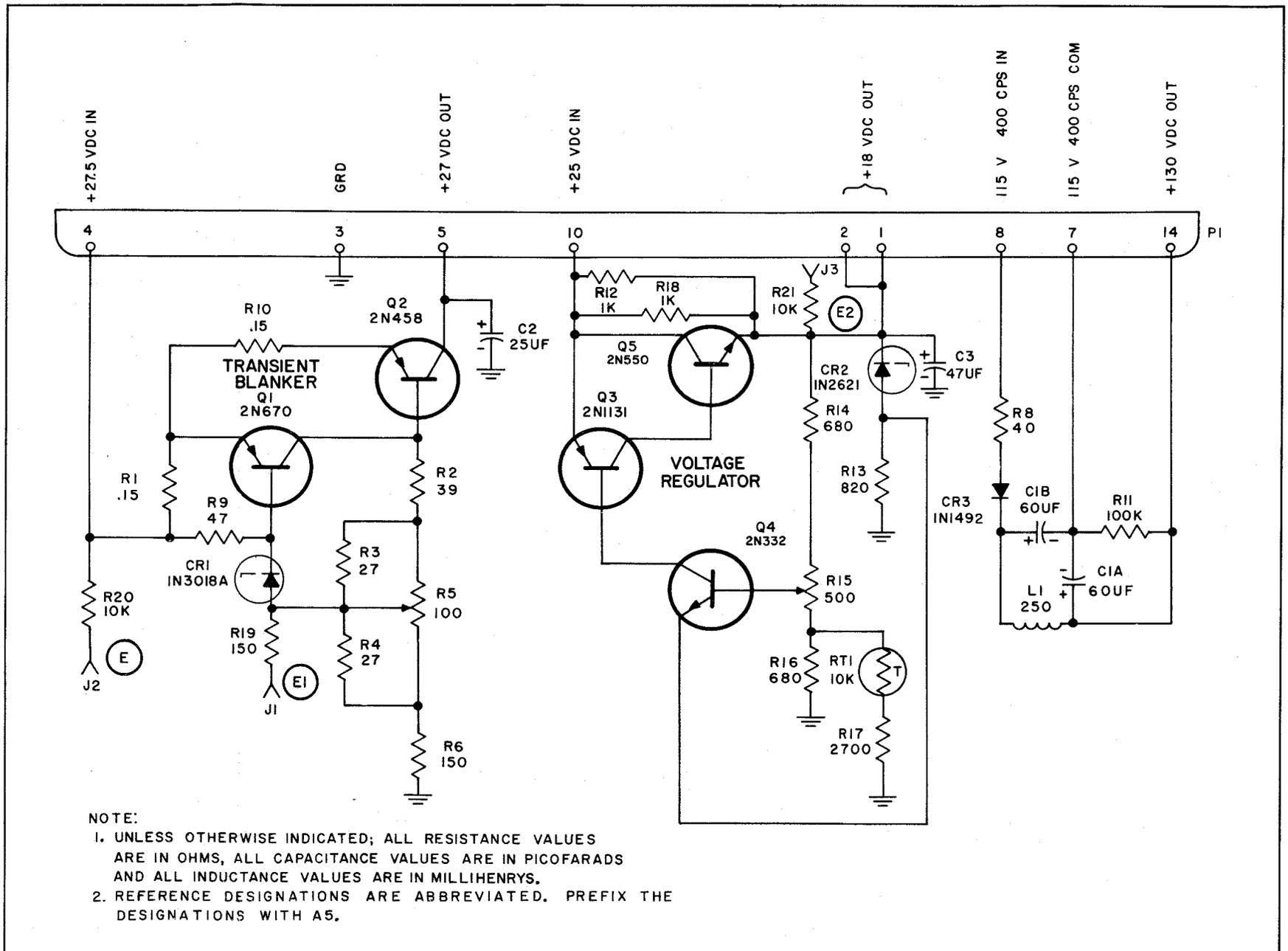
Figure 7-6. Low-Voltage Power Supply Module A5, Schematic Diagram
