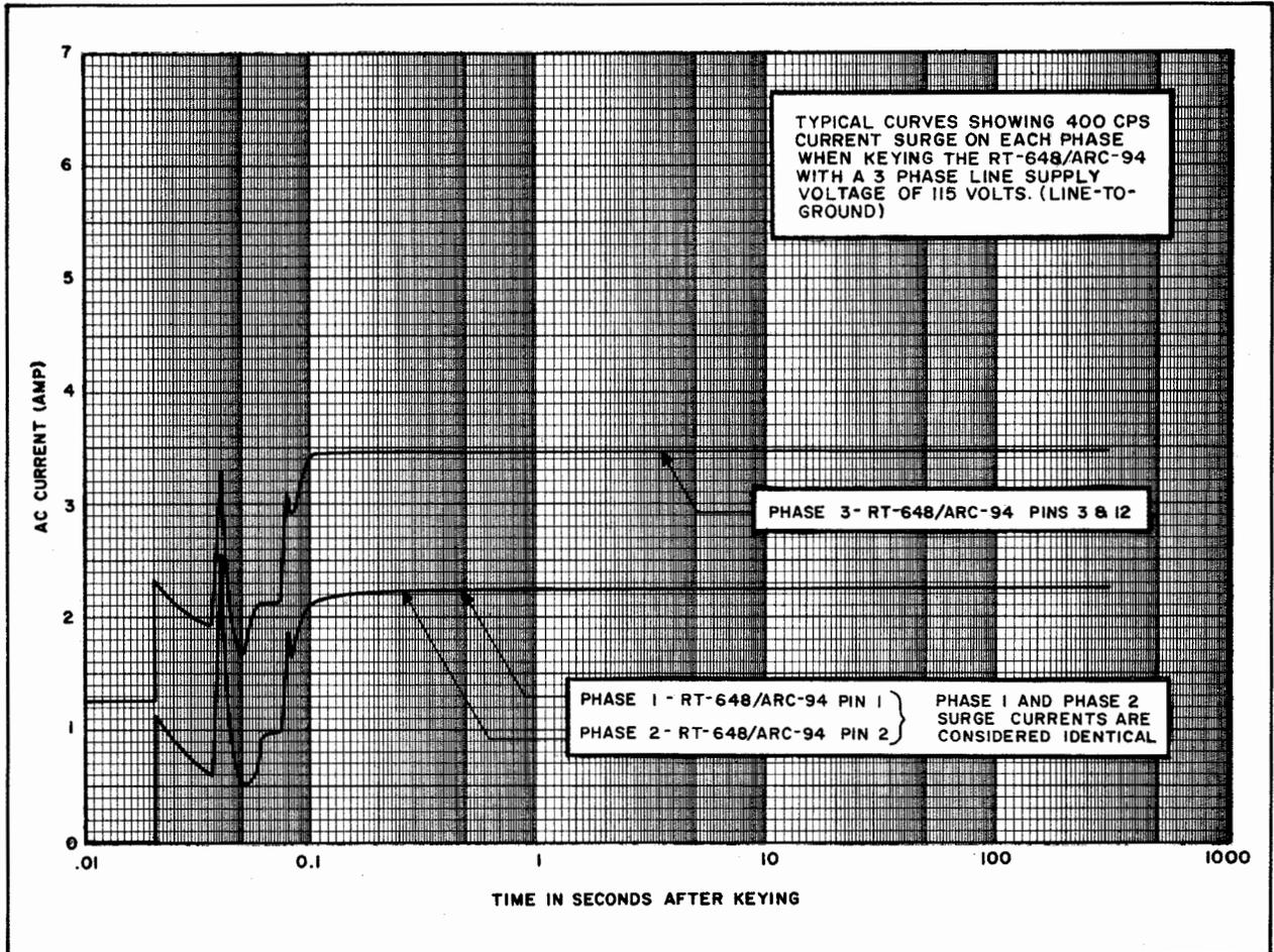
Figure 1-6. Typical A-C, Three-Phase, Transmitter Keying Surge Current
