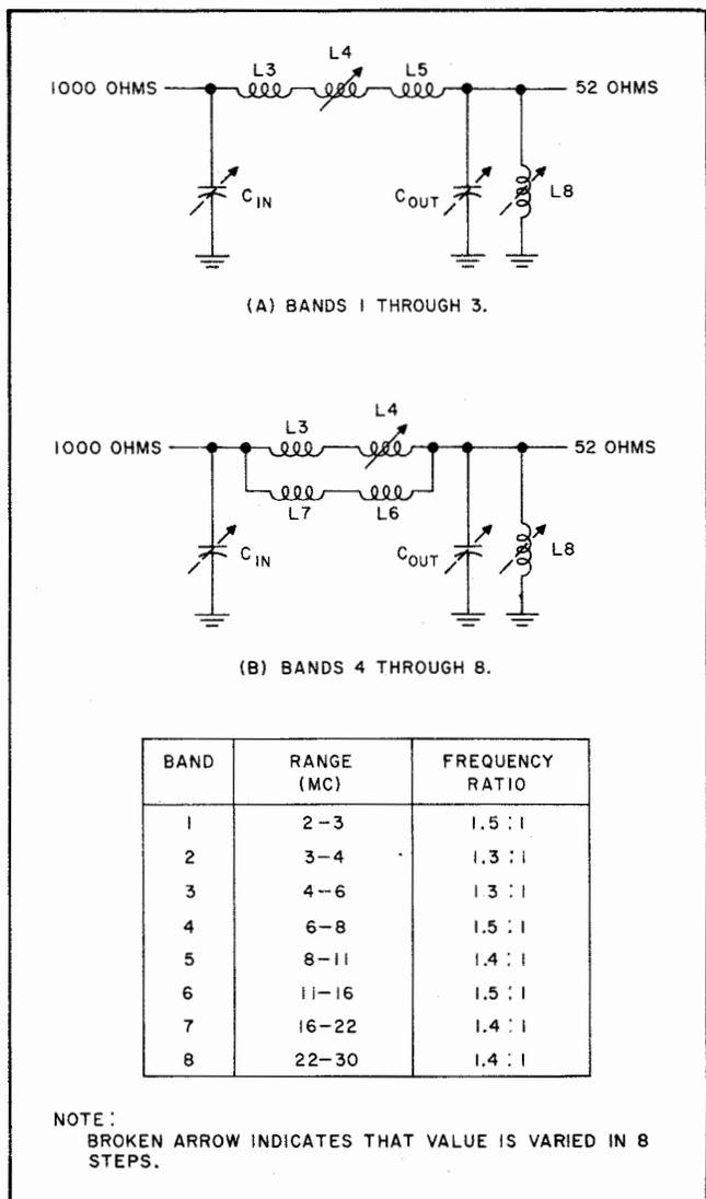
Figure 4-22. Power Amplifier Module A11, Simplified Schematic Diagram of Output Network
