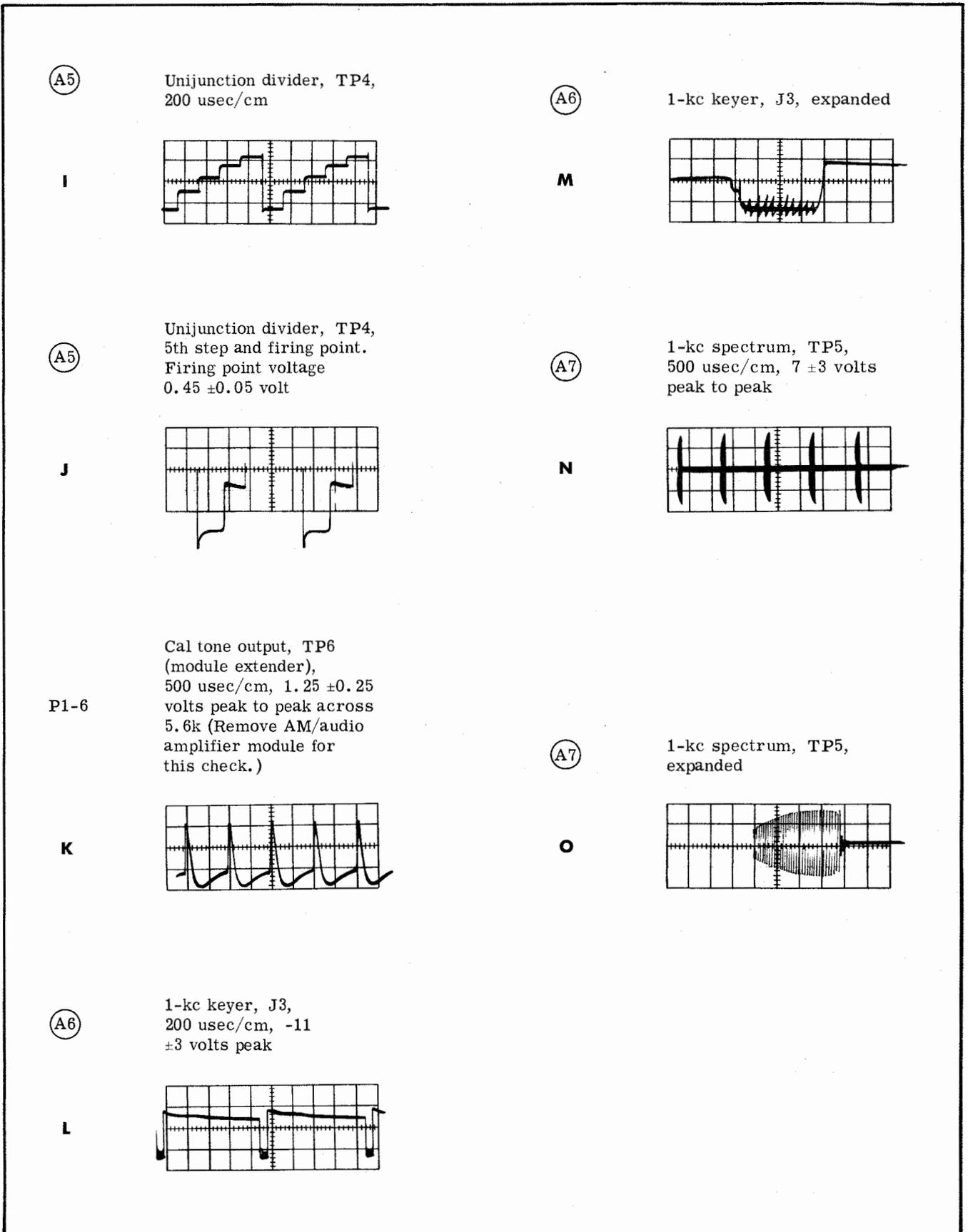
Figure 6-4. Frequency Divider Module A1, Waveforms (Sheet 2 of 2)
