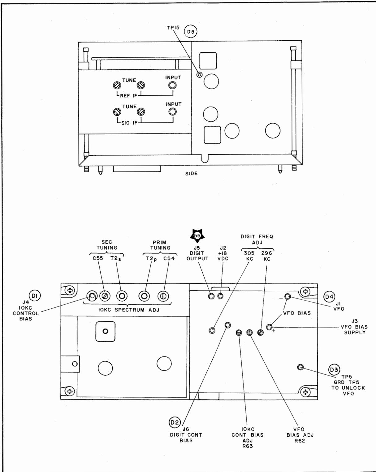
Figure 6-10. Kilocycle-Frequency Stabilizer Module A4, Location of Test Points
