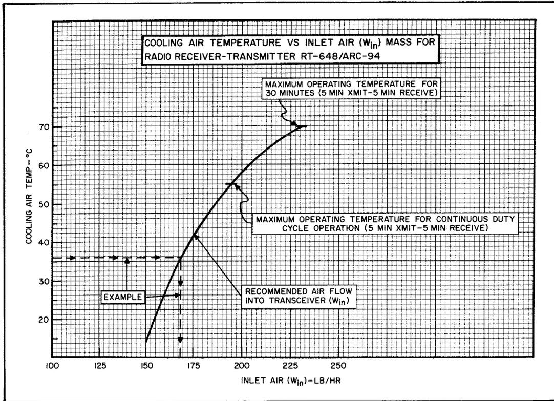
Figure 3-11. Air Temperature In Vs Inlet Air Mass
