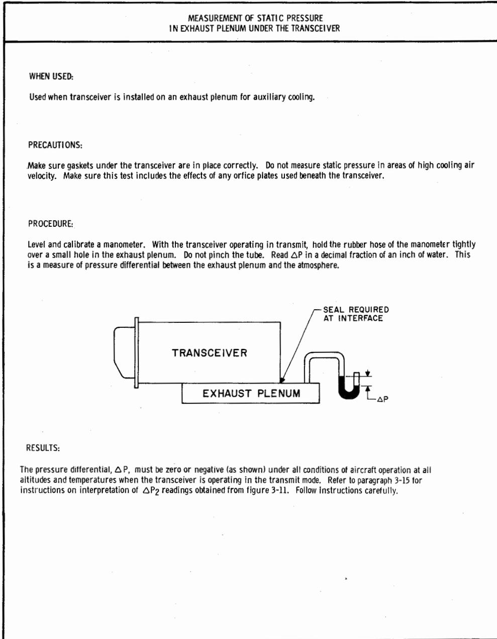
Figure 3-10. Measurement of Static Pressure in Exhaust Plenum Under Radio Receiver-Transmitter RT-648/ARC-94
