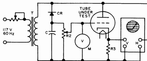
Figure 2-83. Circuit To Display Plate Current-Voltage Characteristic of a Triode Tube
