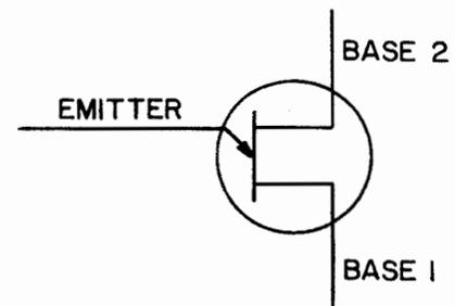
Figure 2-103. Unijunction Transistor
