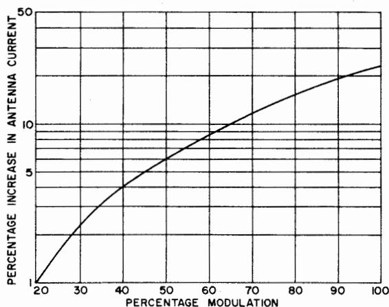
Figure 2-75. Antenna Current Increase with Amplitude Modulation
