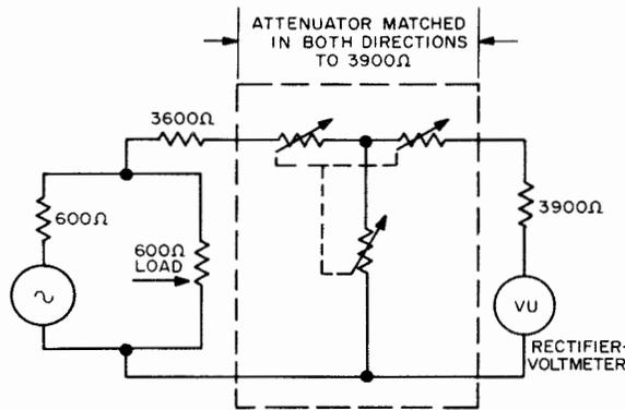
Figure 2-31 Schematic Circuit of a Volume-Level Indicator for Measuring Audio-Frequency Power in the Transmission of Speech and Music, Showing Connections to a Calibrating Circuit
