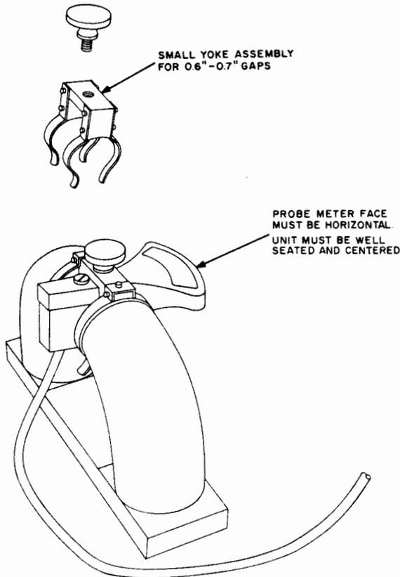
Figure 2-121. Magnetic Flux Density Adapter in Use
