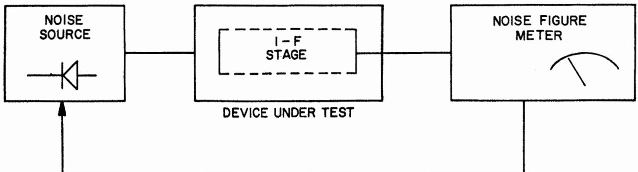
Figure 2-126. Noise Figure Measurement
