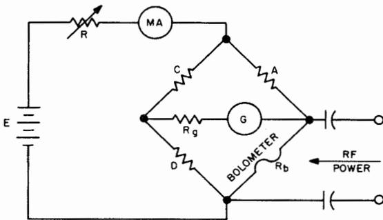
Figure 2-38. Basic Bolometer Bridge Circuit
