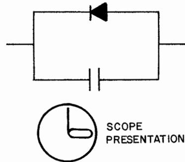
Figure 2-65. Diode Check
