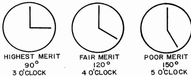
Figure 2-64. Transistor Check-Single Junction
