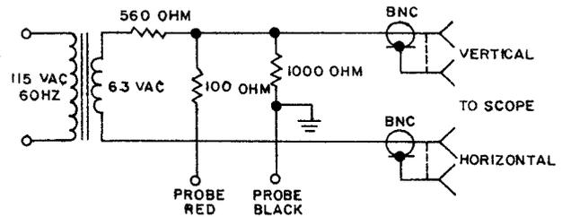
Figure 2-62. In-Circuit Tester Schematic Diagram
