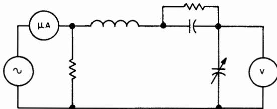
Figure 2-29. Simplified Q-Meter Connection for Measuring Large Capacitances
