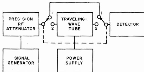
Figure 2-85. Traveling-Wave Tube Test Arrangement
