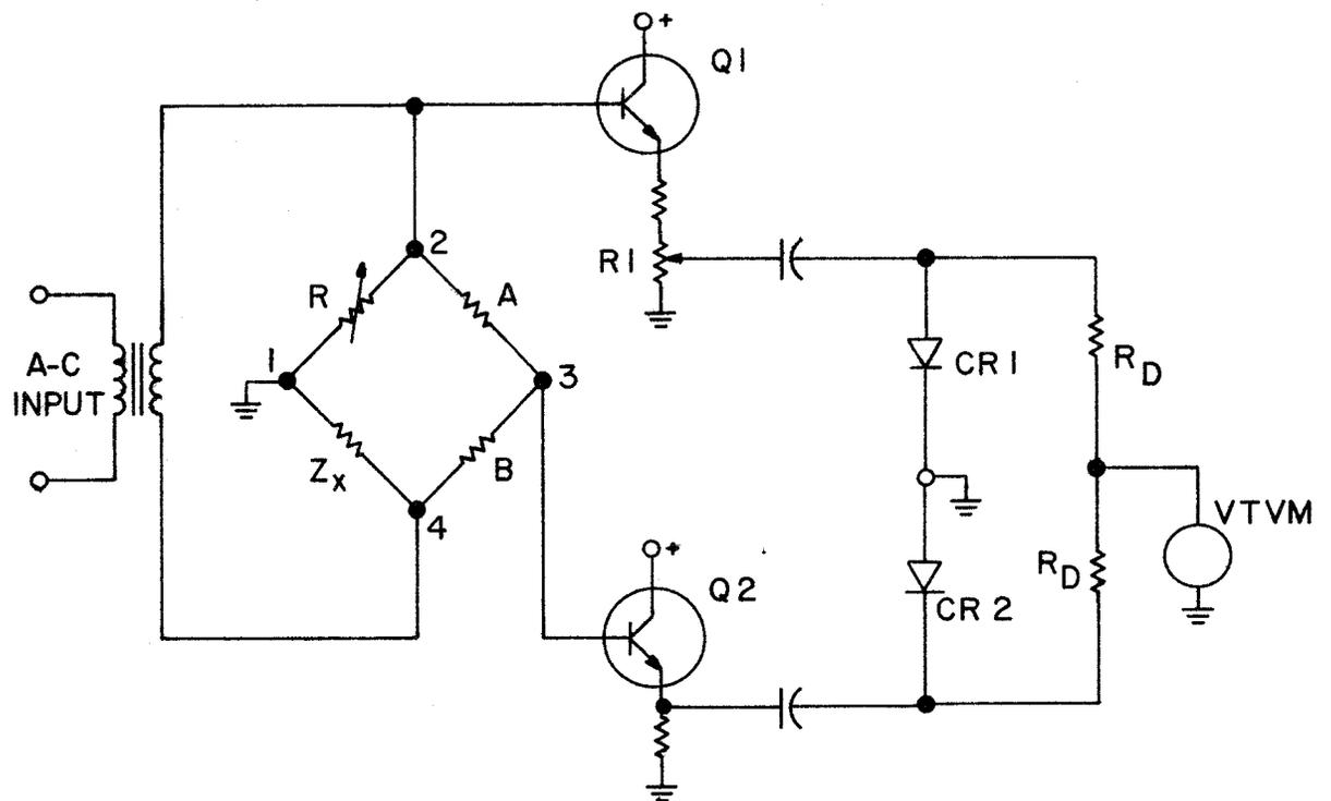
Figure 2-17. Vector Bridge Phase Angle Determination
