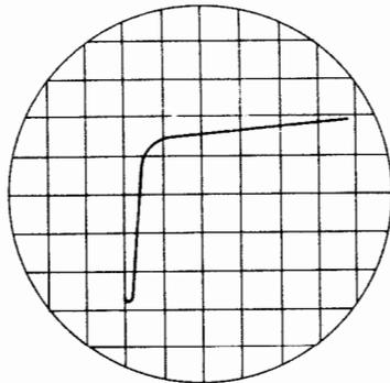
Figure 2-92. Typical Collector Current-Voltage Curve
