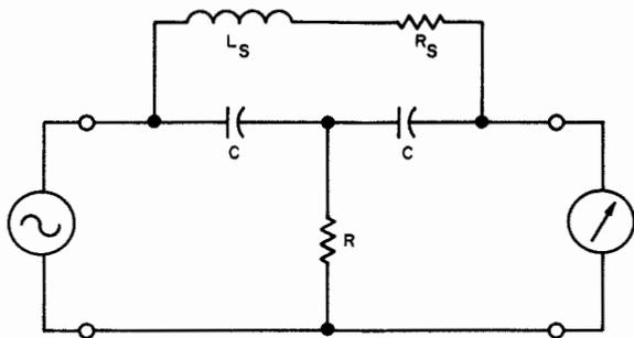
Figure 2-14. A Null Instrument Utilizing a Bridged-T
