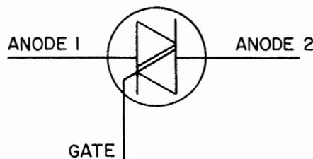
Figure 2-100. Gate-Controlled Full-Wave AC Silicon Switch
