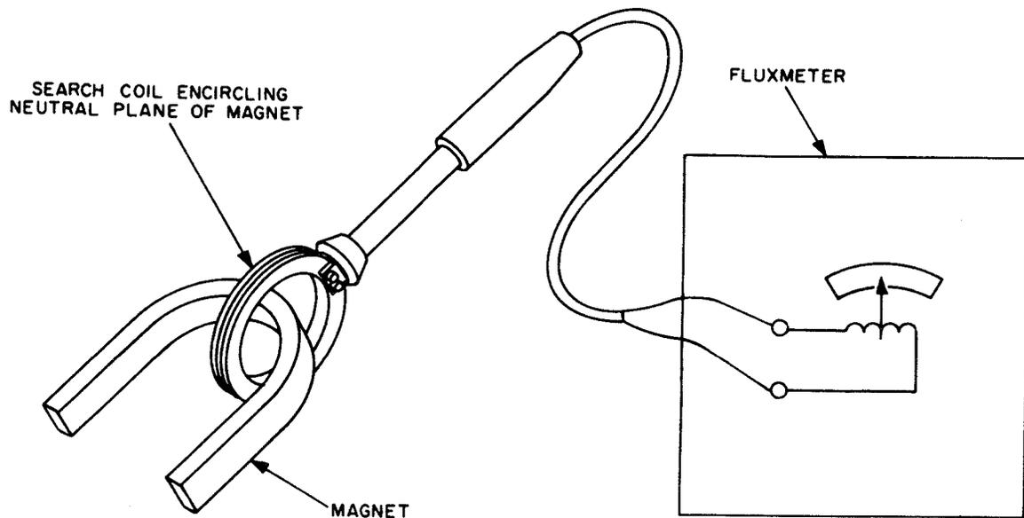
Figure 2-122. Search-Coil in Neutral Plane of Magnet
