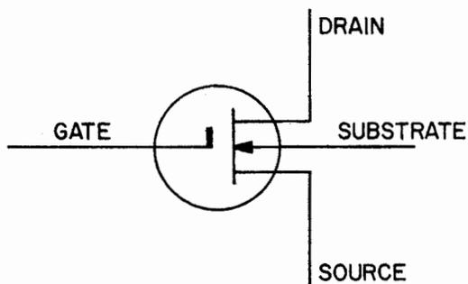
Figure 2-108. MOSFET (Depletion/Enhancement Type)
