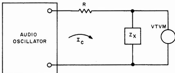
Figure 2-19. Constant-Current Impedance Measuring Method
