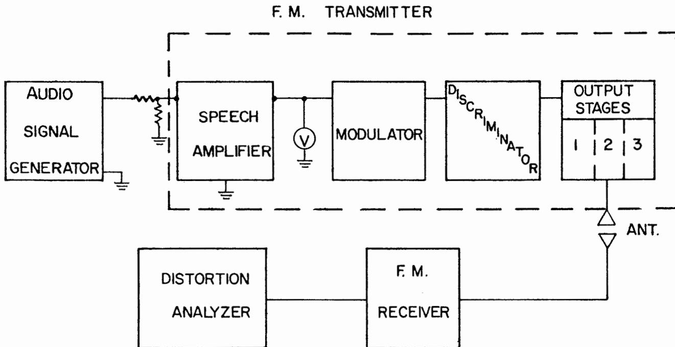
Figure 2-81. FM Deviation and Harmonic Distortion Test Set-Up
