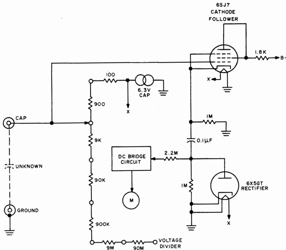
Figure 2-3. Capacitance-Measuring Section Taken from a Typical Reactance Type Electronic Volt-Ohm-Capacitance Milliammeter
