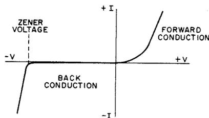
Figure 2-97. Zener Diode Characteristic Pattern
