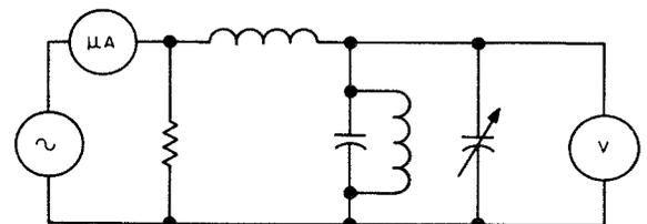
Figure 2-27. Simplified Q-Meter Circuit, Parallel
