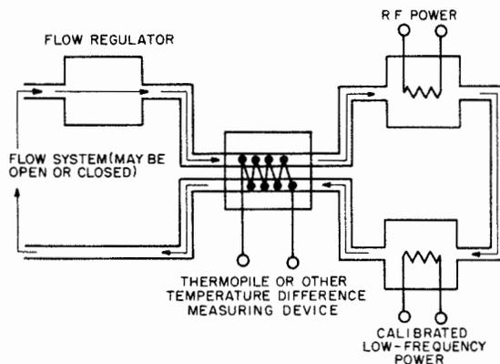
Figure 2-52. Generalized Flow Calorimetric System Using Substitution at Low-Frequency Power
