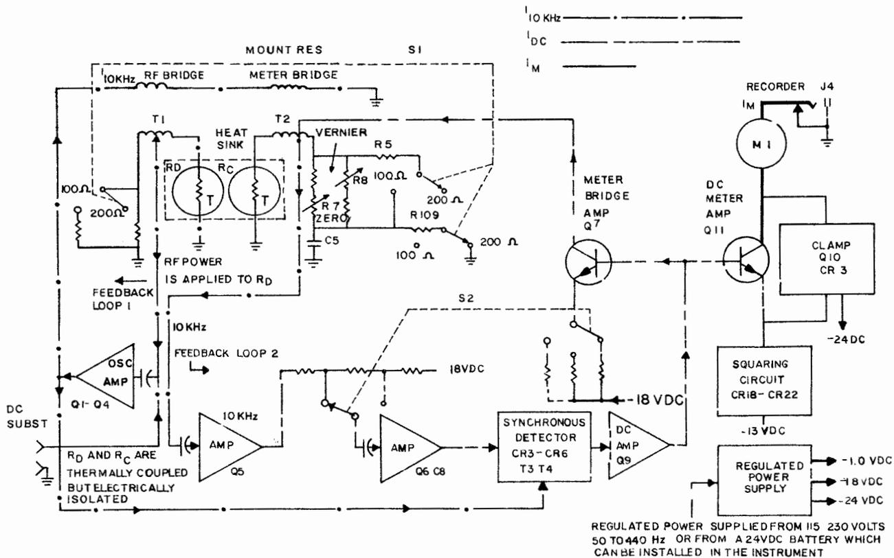
Figure 2-47. Power Meter Block Diagram
