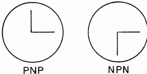
Figure 2-69. Distinction Between PNP and NPN Transistors
