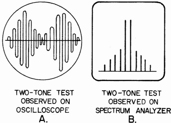
Figure 2-80. Examples of Ideal Two-Tone Test Waveform
