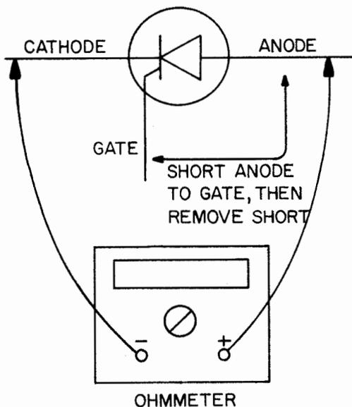
Figure 2-99. Testing an SCR with an Ohmmeter
