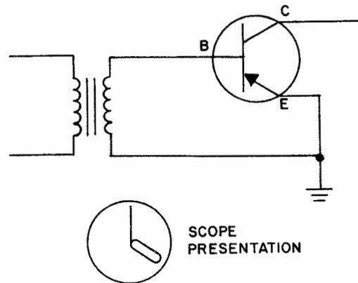
Figure 2-66. Transistor Check-Base to Emitter
