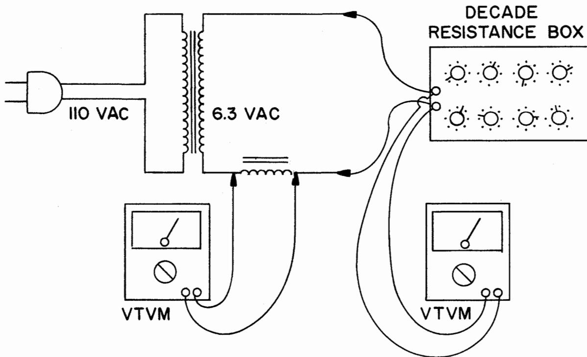
Figure 2-5. Determining Inductance with a VTVM and Decade Resistance Box
