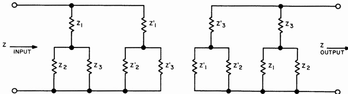
Figure 2-15. Input and Output Impedances of Twin-T at Balance
