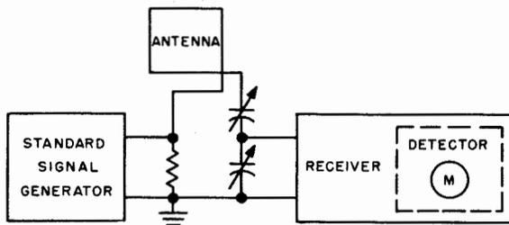
Figure 2-119. Substitution Method of Determining Field Strength
