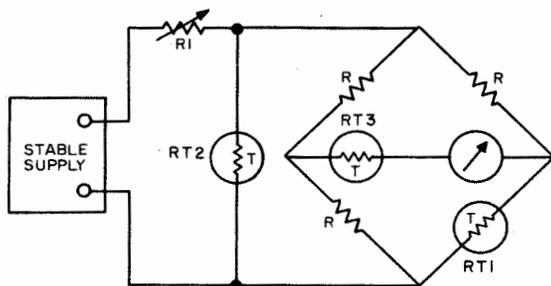
Figure 2-43. Simplified Diagram of a Two-Disk Thermistor Bridge
