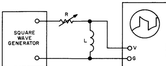
Figure 2-24. Square Wave Technique for L Measurement
