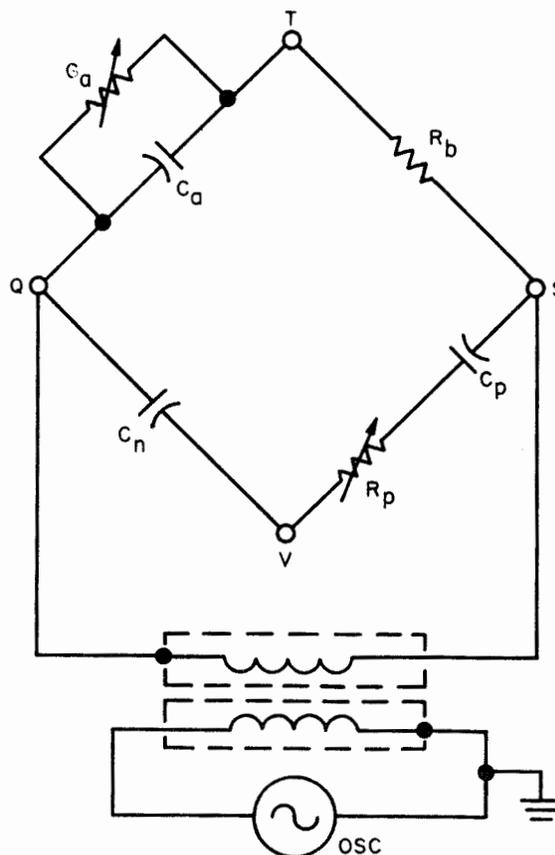
Figure 2-10. Substitution Bridge Schematic
