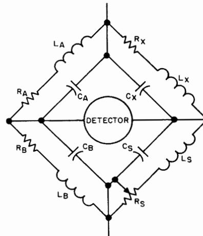
Figure 2-8. Resistance-Ratio Bridge Residual Elements
