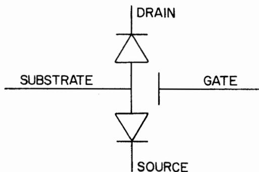
Figure 2-111. MOSFET (Enhancement Type) Equivalent Circuit
