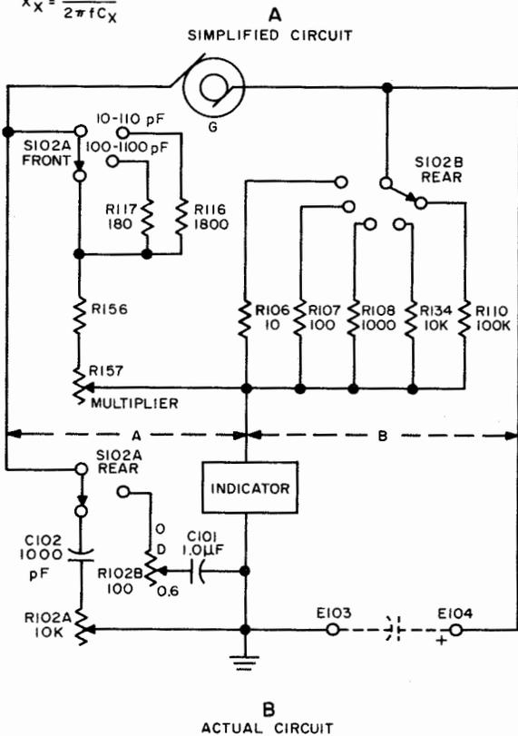
Figure 2-2. Capacitor Bridge Measuring Circuit
