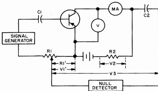
Figure 2-90. Transistor Beta-Test Circuit
