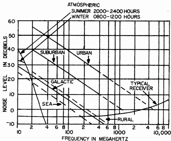
Figure 2-117. Median Values of Average Noise Power Expected From Various Sources (Omni-Directional Antenna Near Surface).
