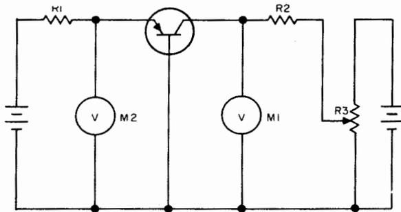
Figure 2-89. Transistor Punch-Through Voltage ( $V_{PT}$ ) Test Circuit
