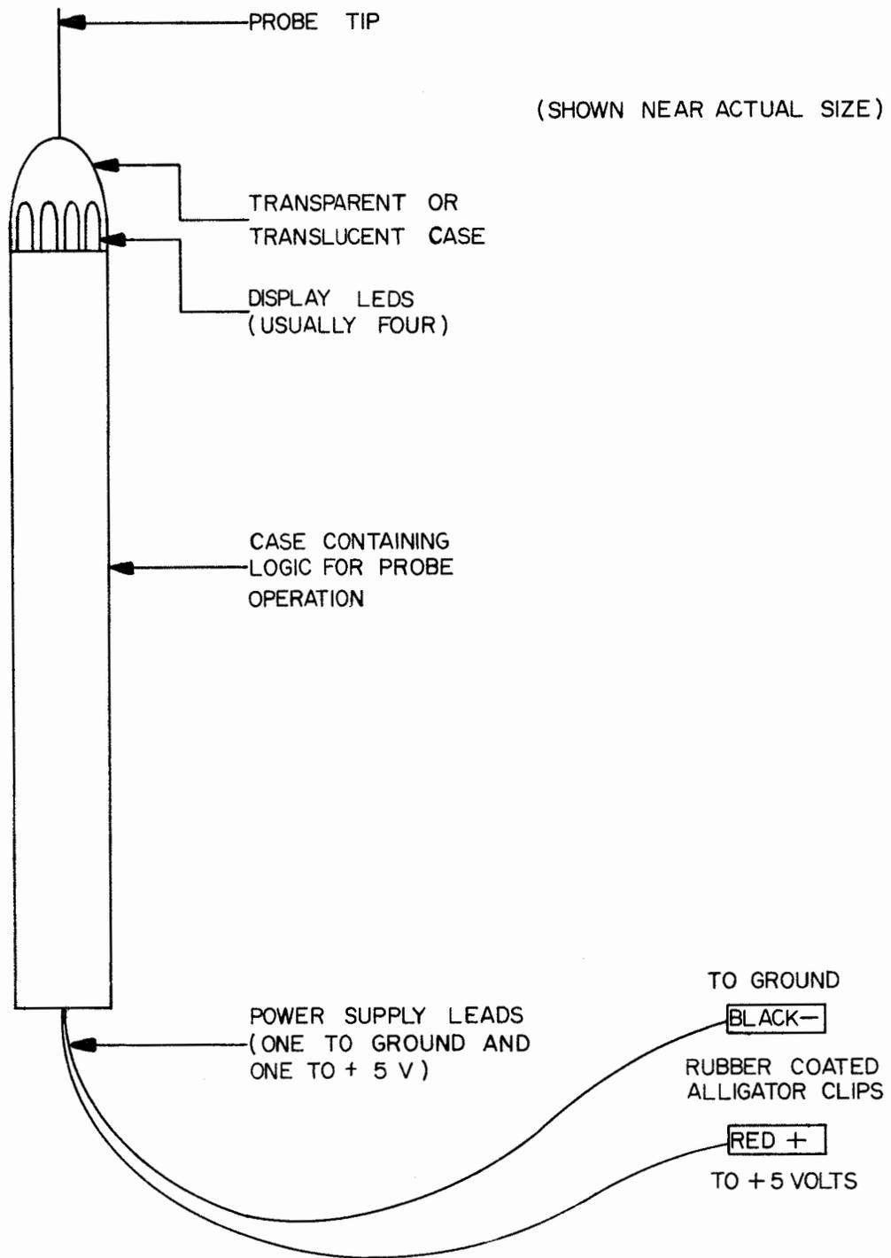
Figure 2-113. Typical Logic Probe
