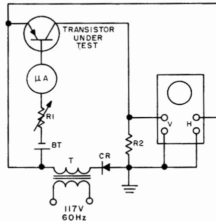
Figure 2-91. Circuit To Display Collector Current-Voltage Curve
