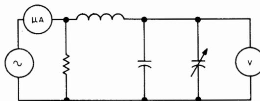
Figure 2-28. Simplified Q-Meter Connection for Measuring Small Capacitances
