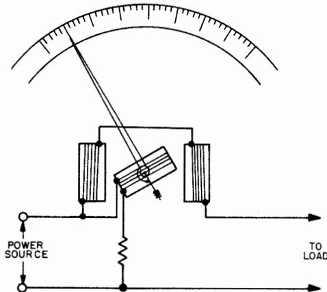
Figure 2-34. Mechanical Equivalent of the Electrodynamic Wattmeter
