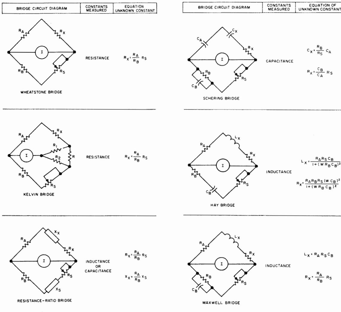
Figure 2-6. Basic Bridge Circuits
