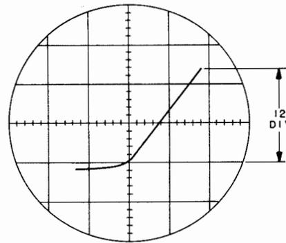
Figure 2-94. Typical Characteristic Curve of a Silicon Diode
