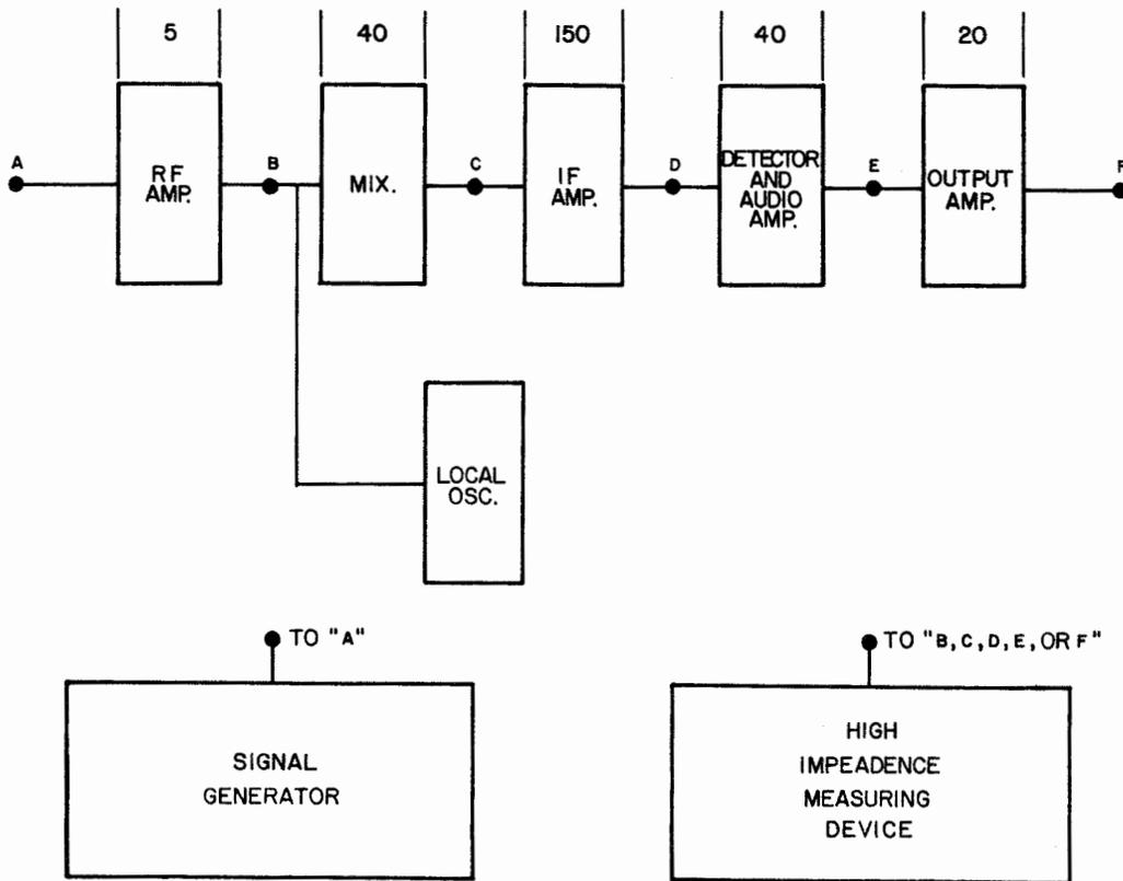
Figure 2-127. Superheterodyne Receiver Stage Gain
