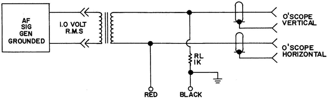
Figure 2-73. Tester Using 1.0-Volt Source
