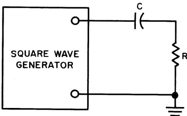
Figure 2-22. Square Wave Technique for R or C Measurement
