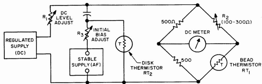
Figure 2-44. Simplified-Diagram of V Bridge
