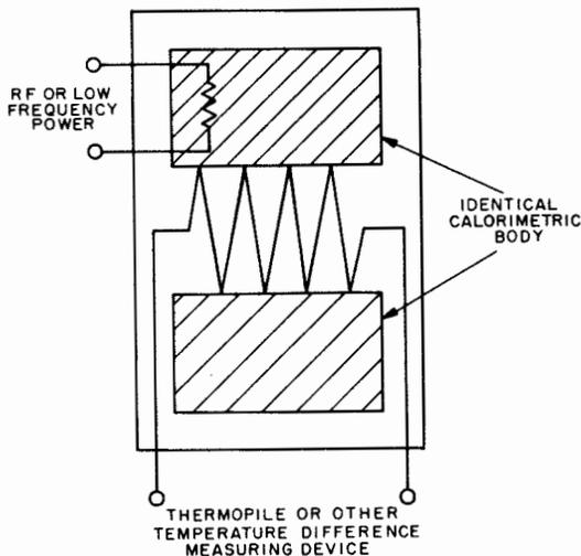
Figure 2-50. Twin Calorimetric System
