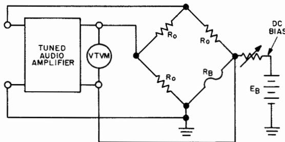
Figure 2-45. Self-Balancing Bridge Circuit
