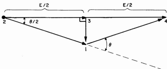
Figure 2-18. Vector Bridge Phasor Diagram
