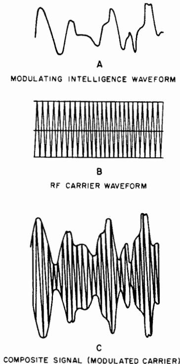
Figure 2-76. RF Carrier Amplitude Modulated by a Complex Waveform
