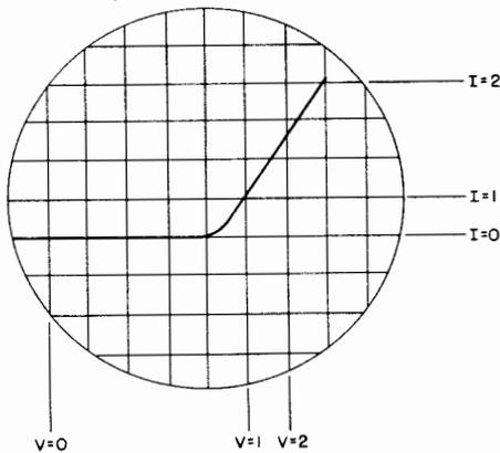
Figure 2-84. Oscilloscope Presentation of Triode Tube Plate Current-Voltage Characteristic
