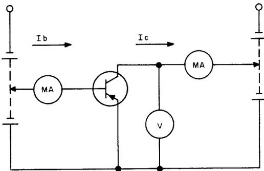
Figure 2-87. Transistor Direct-Current Gain Test
