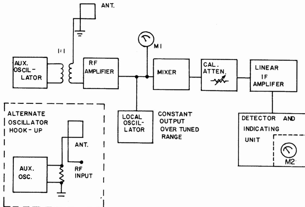
Figure 2-118. Standard Antenna Method for Measuring Field Strength
