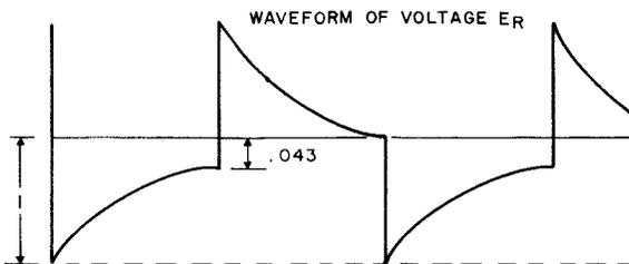
Figure 2-23. Waveform of Voltage,  $E_R$
