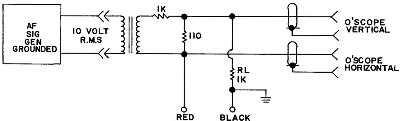
Figure 2-74. Tester Using 10.0-Volt Source
