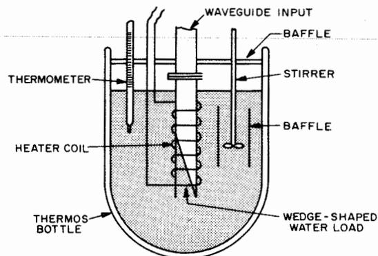
Figure 2-49. NBS Adiabatic Calorimeter
