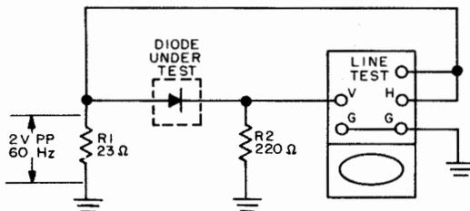
Figure 2-93. Display Circuit Used with Oscilloscope OS-8C/U
