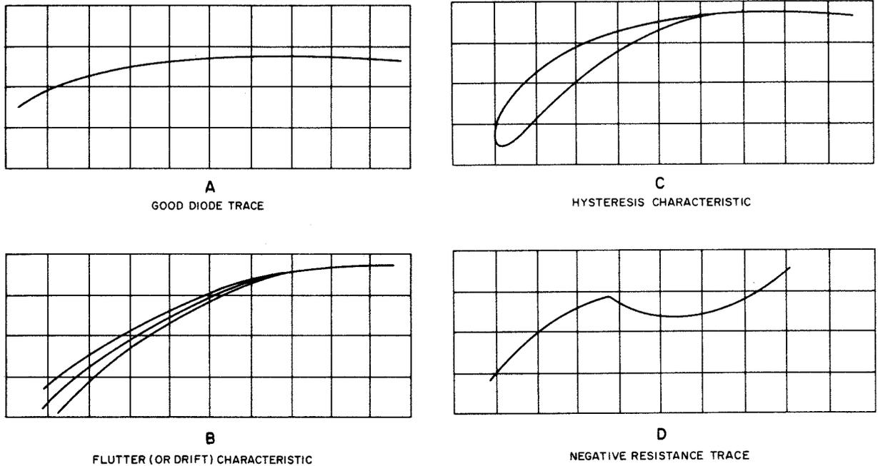
Figure 2-95. Diode Reverse Current-Voltage Characteristics
