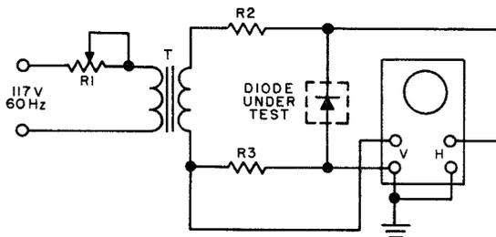
Figure 2-96. Semiconductor Diode Test Circuit
