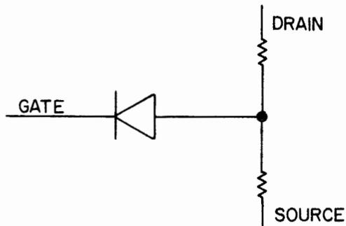
Figure 2-107. P Channel JFET Equivalent Circuit
