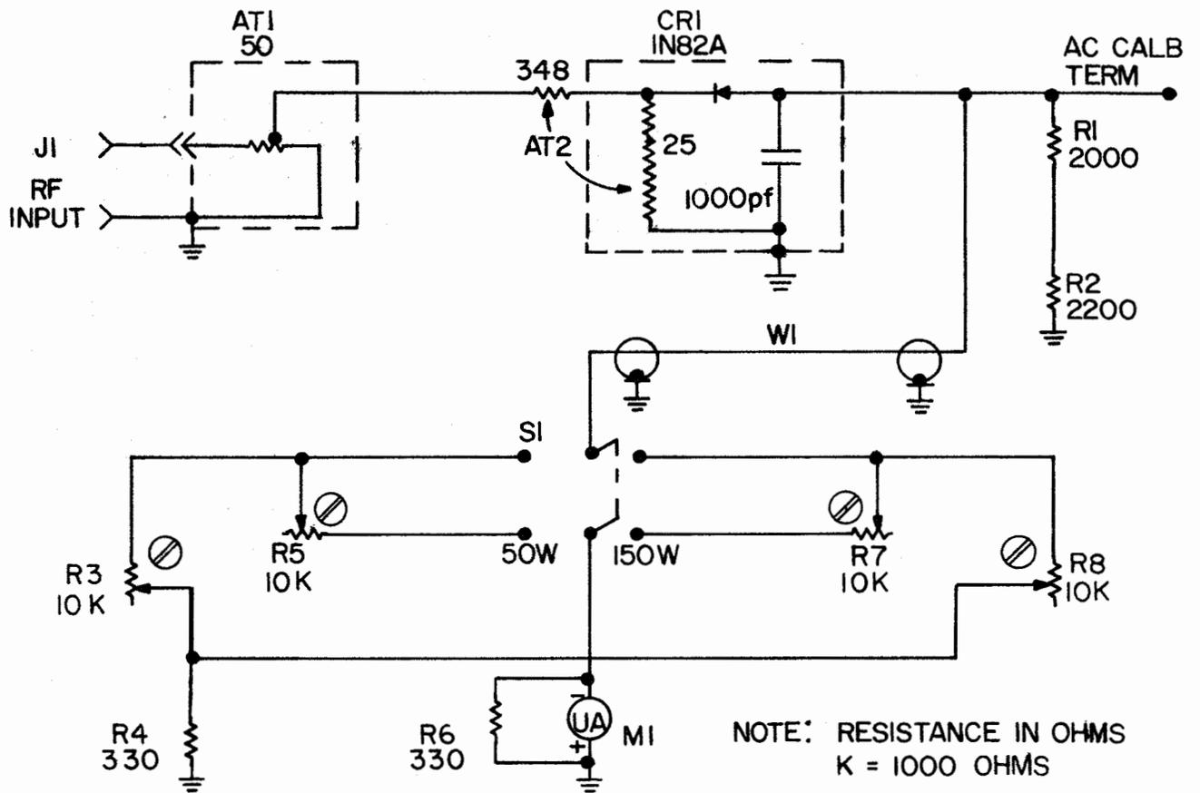
Figure 2-36. VHF-UHF Wattmeter
