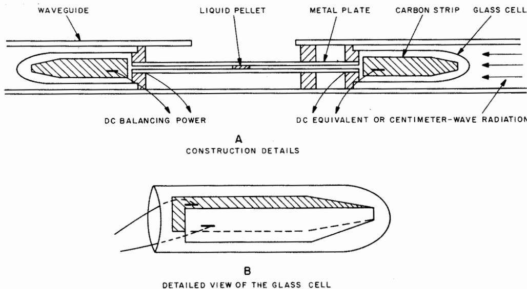
Figure 2-51. Differential Air Thermometer-Type Calorimeter
