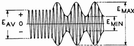
Figure 2-77. RF Amplitude Percentage Modulation
