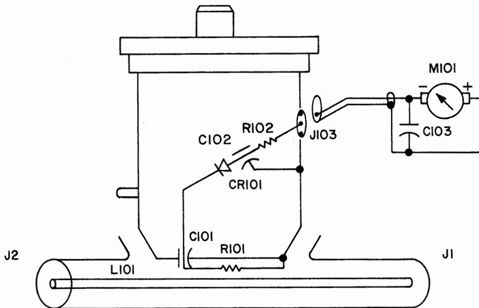
Figure 2-37. Typical In-Line Wattmeter
