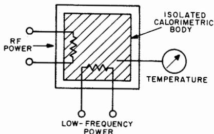
Figure 2-48. Generalized Static Calorimeter Using Low-Frequency Power Substitution
