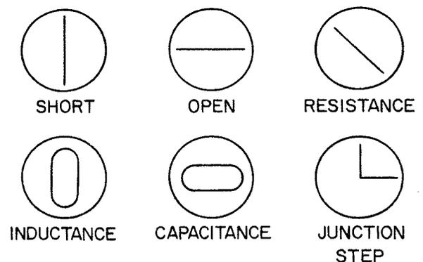
Figure 2-63. Typical Oscilloscope Displays
