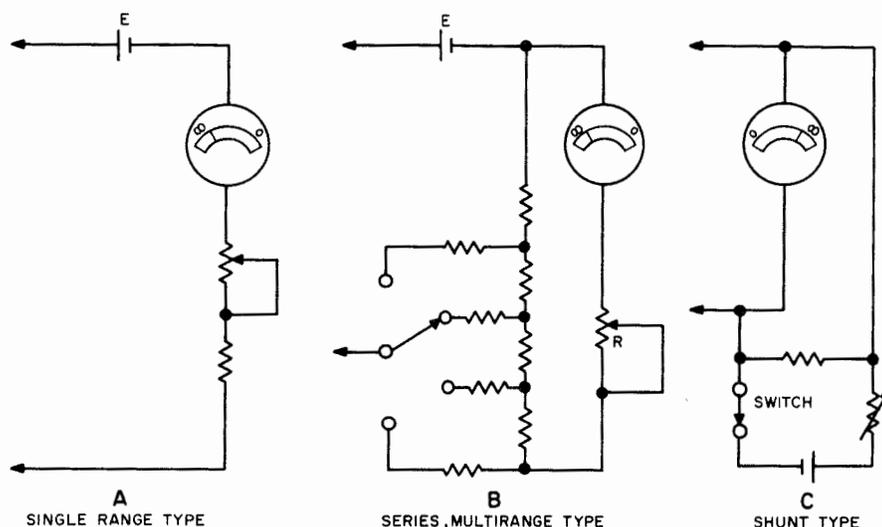
Figure 2-1. Basic Ohmmeter Circuits
