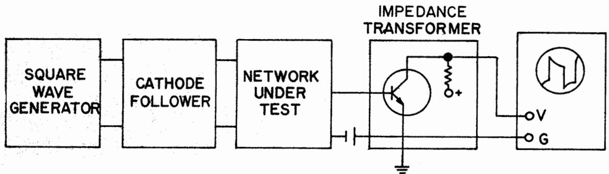
Figure 2-21. Square Wave Impedance Measurement Test Arrangement
