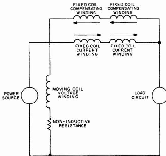
Figure 2-33. Electrical Equivalent of Compensated Electrodynamic Wattmeter
