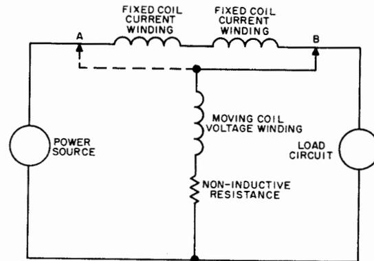
Figure 2-32. Electrical Equivalent of the Electrodynamic Wattmeter
