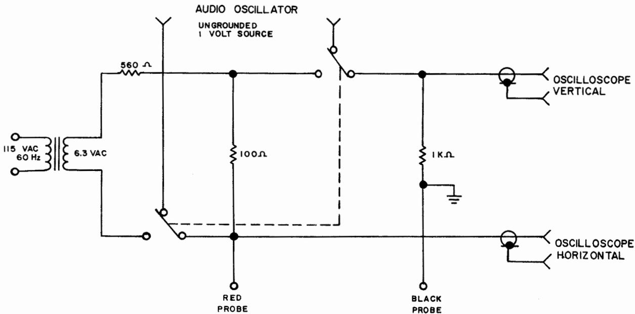
Figure 2-72. Modified In-Circuit Tester (Schematic Diagram)
