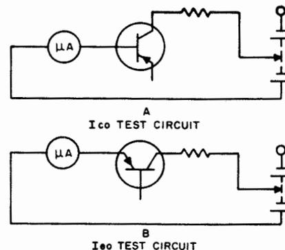
Figure 2-86. Collector Leakage Current Test Circuit
