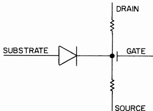
Figure 2-109. MOSFET (Depletion/Enhancement Type) Equivalent Circuit
