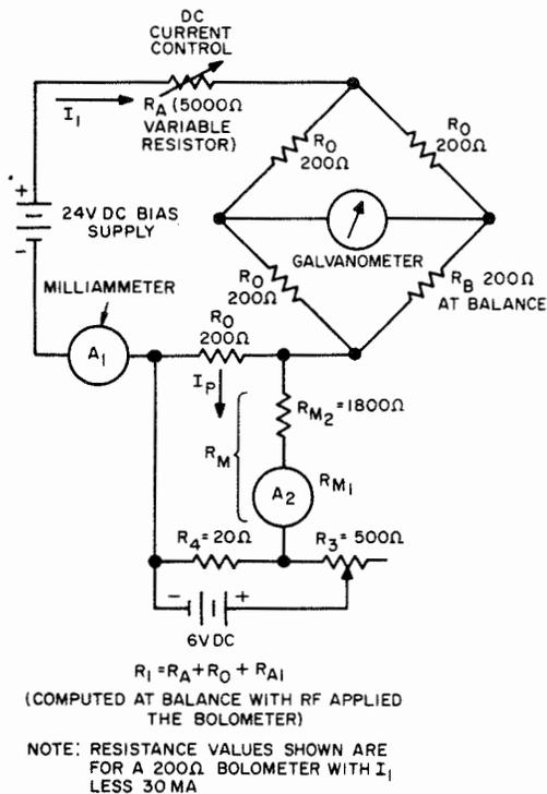
Figure 2-40. Potentiometer Bridge
