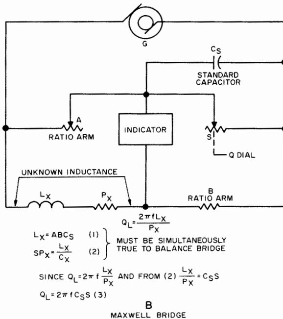
Figure 2-4. Basic Bridge Circuits Used for Inductance Measurements
