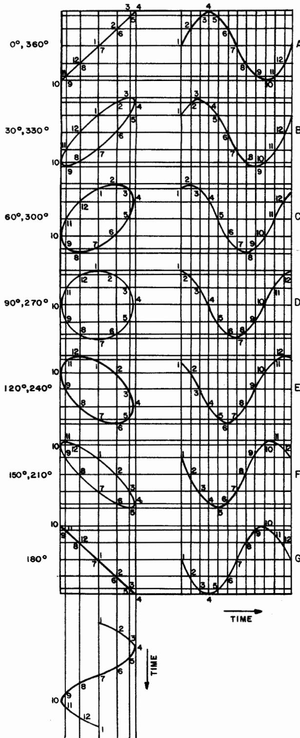
Figure 2-59. Lissajous Patterns of A 1:1 Ratio, Showing Effect on Phase Relationships
