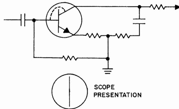
Figure 2-67. Transistor Check-Base to Collector
