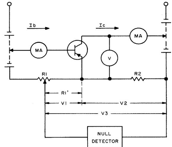
Figure 2-88. Direct Reading Transistor Direct-Current Gain Tester
