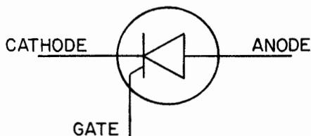
Figure 2-98. SCR Active Elements
