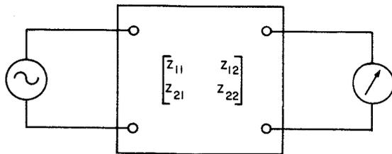
Figure 2-11. Generalized Four Terminal Network
