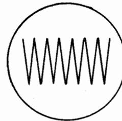
Figure 2-60. Undistorted Transmitter Output Signal
