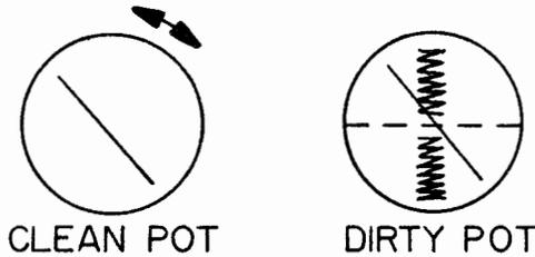
Figure 2-68. Potentiometer Noise Check
