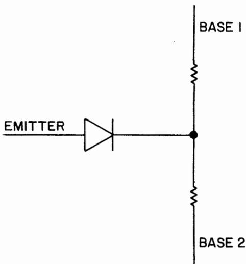
Figure 2-104. Unijunction Transistor Equivalent Circuit
