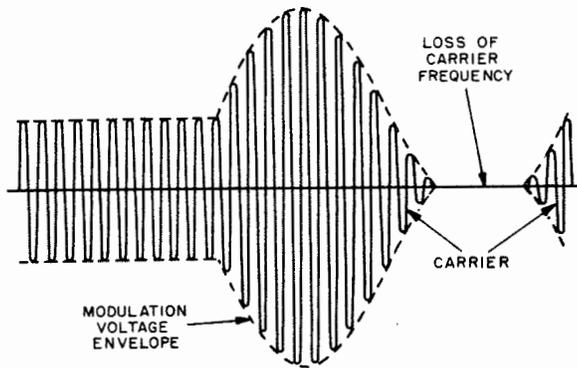
Figure 2-79. Overmodulated RF Carrier
