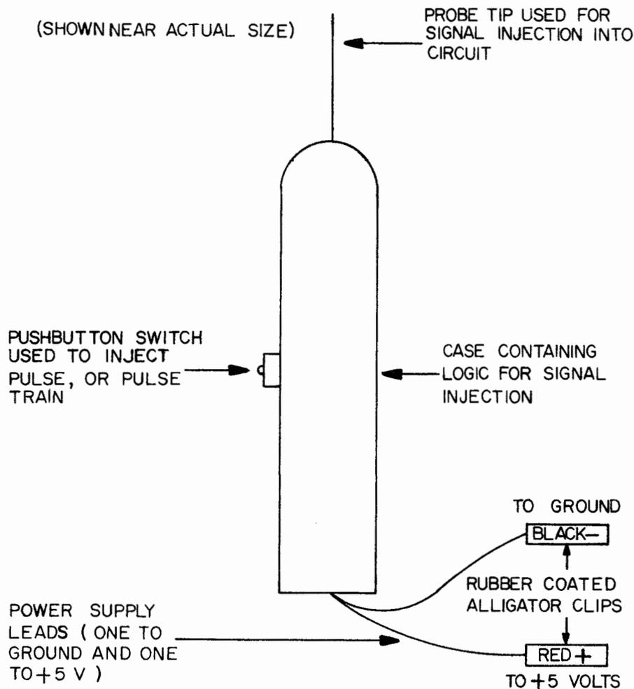
Figure 2-112. Logic Pulse Generator
