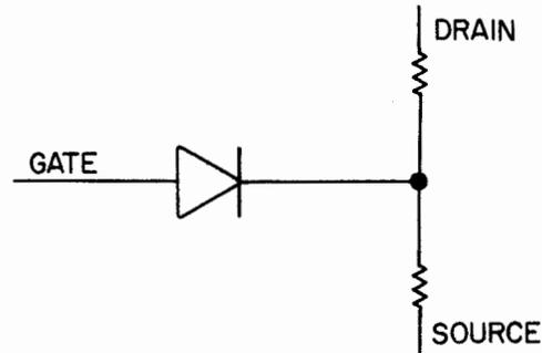
Figure 2-106. N Channel JFET Equivalent Circuit
