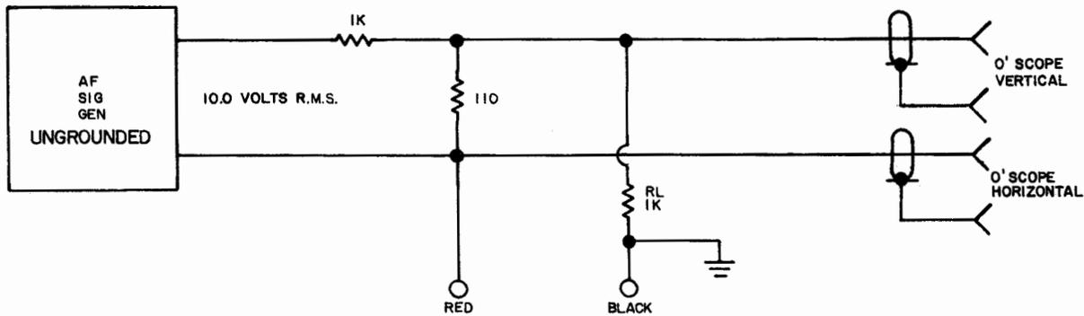
Figure 2-71. Tester Using 10.0 Volt Source
