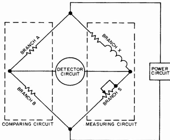
Figure 2-7. General Bridge Circuit Configuration
