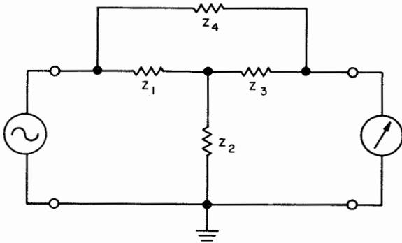
Figure 2-13. Bridged-T Bridge
