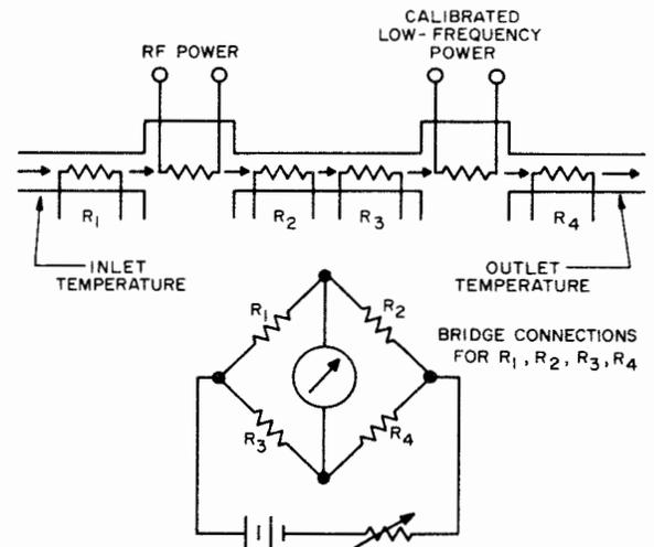
Figure 2-53. Generalized Balanced Flow Calorimeter
