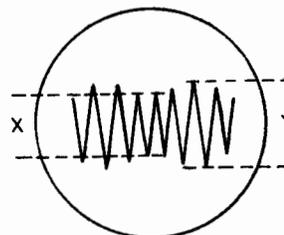
Figure 2-61. Distorted Transmitter Output Signal
