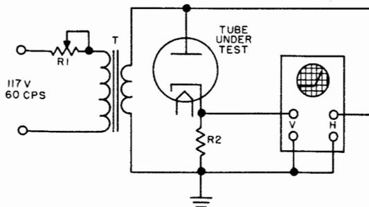
Figure 2-82. Circuit To Display Plate Current-Voltage Characteristic of a Diode Tube
