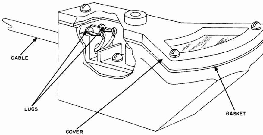
Figure 2-120. Probe Meter
