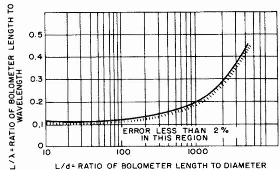
Figure 2-46. Relation Between Bolometer Wire Dimensions and Wavelength for Small Substitution Error
