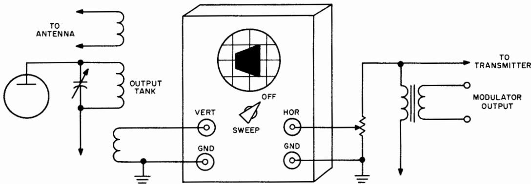
Figure 2-78. Trapezoidal Modulation Patterns
