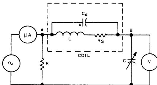
Figure 2-26. Simplified Q-Meter Circuit, Series
