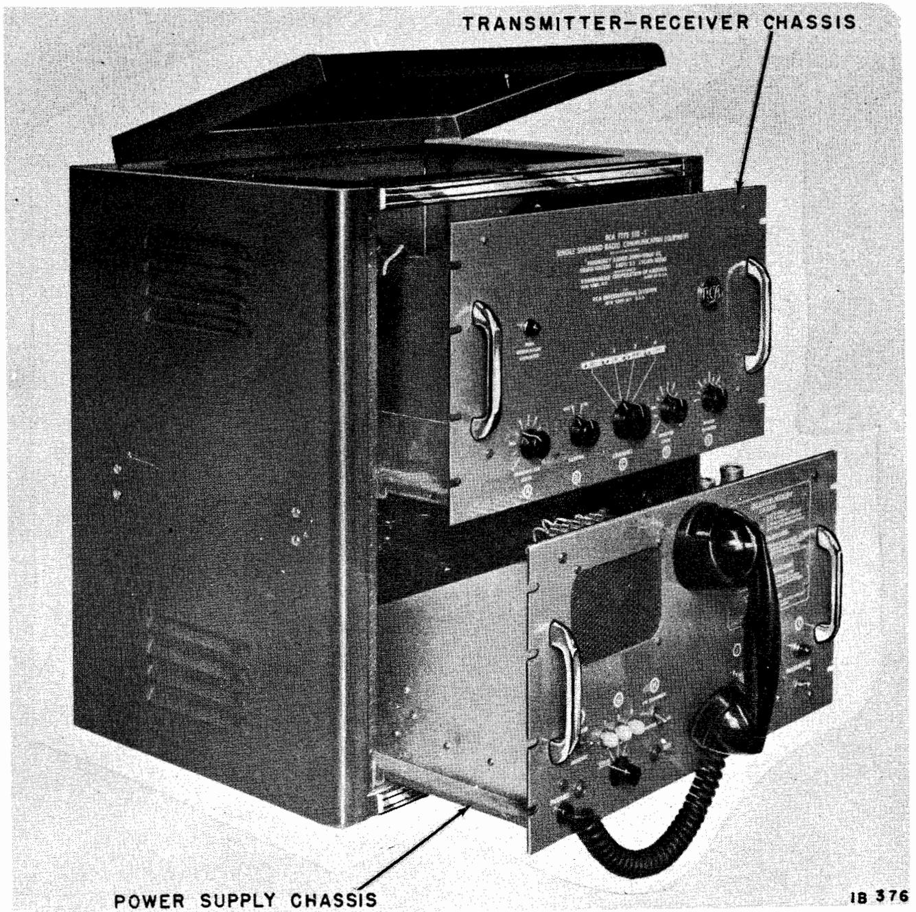
**Figure 3. Cabinet Top Raised and Chassis Withdrawn**
