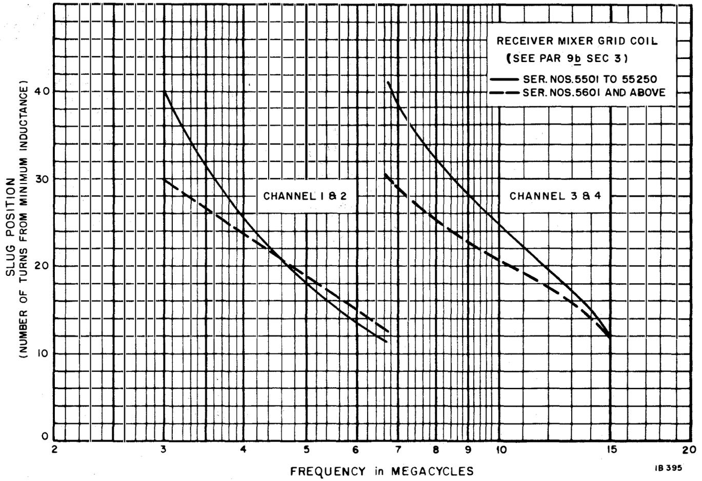
**Figure 27. Slug Position of Receiver Mixer Grid Coils**
