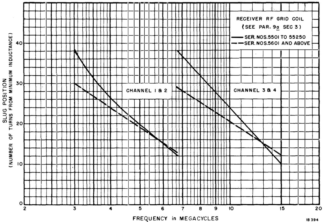
Figure 26. Slug Position of Receiver RF Coils
