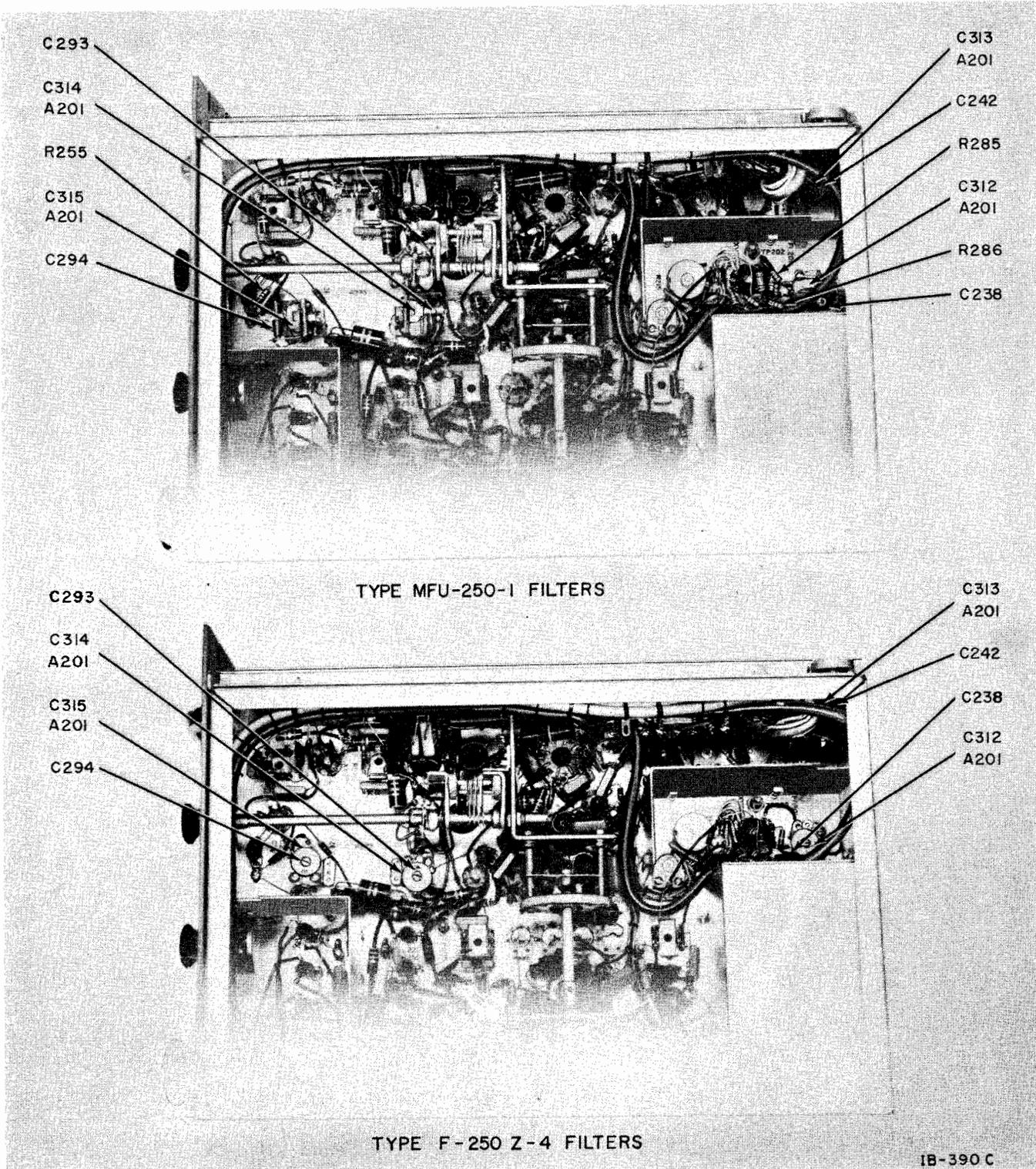
Figure 21C. Transmitter-Receiver, Components Used with Mechanical Filters, Equipments Serial Nos. 5601 and above
