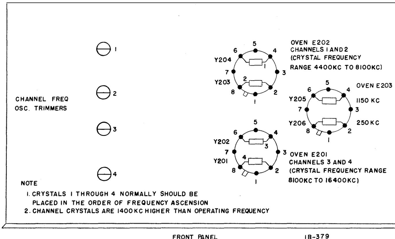
Figure 9. Crystal Ovens, Top View, Cover Removed
