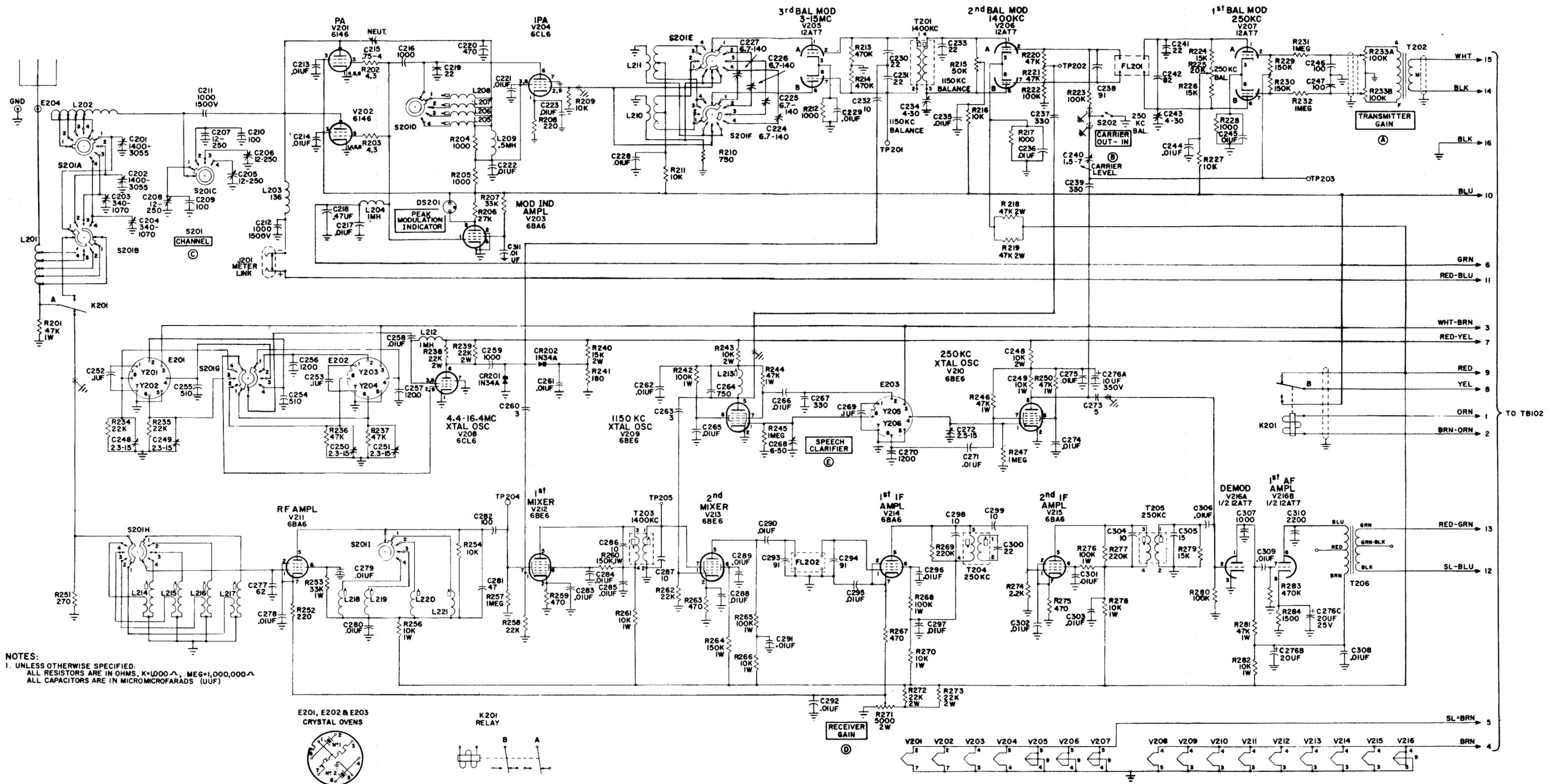
Figure 29A Transmitter-Receiver Schematic (Serial Numbers 5501 to 55250)
