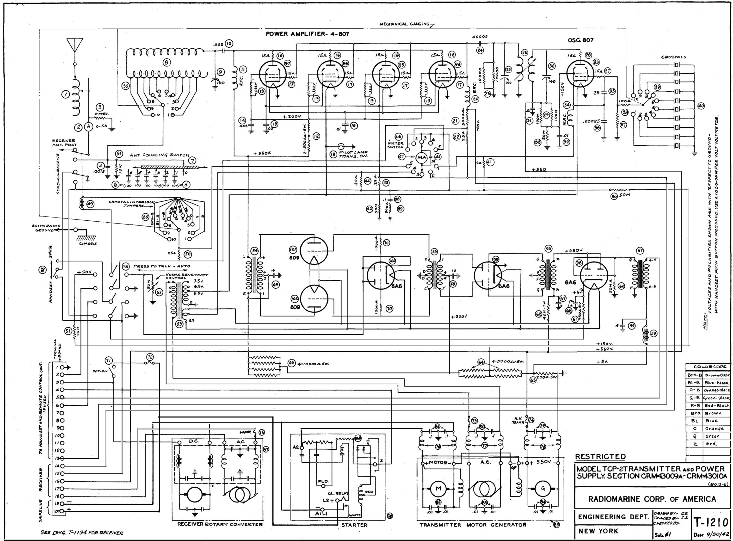
NOTE: VOLTAGES AND POLARITIES SHOWN ARE WITH RESPECT TO GROUND - WITH HANDSET PUSH BUTTON PRESSED. USE A 1000-OHM PER VOLT METER.
