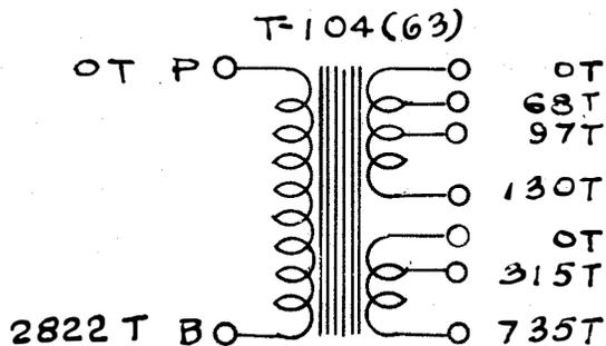
MODEL TCP & TCP-1 TRANSFORMERS (ALSO TCP-2)
