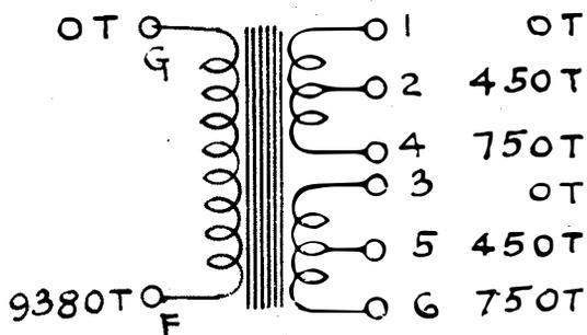
NOTE: NUMBERS IN BRACKETS ARE SYMBOL DESIGNATIONS ON SCHEMATIC DWGS. NUMBERS WITH "T" FOLLOWING INDICATE NO. OF TURNS
