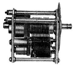
Fig. 34 96J Autotune Singleturn Unit Left Side View
