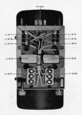
Fig. 66 High Voltage Dynamotor-Bottom View
