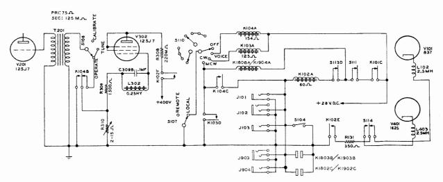
Fig. 15 Emission Selection and Carrier Control Circuits (Dwg. No. 500 1456 00B)
