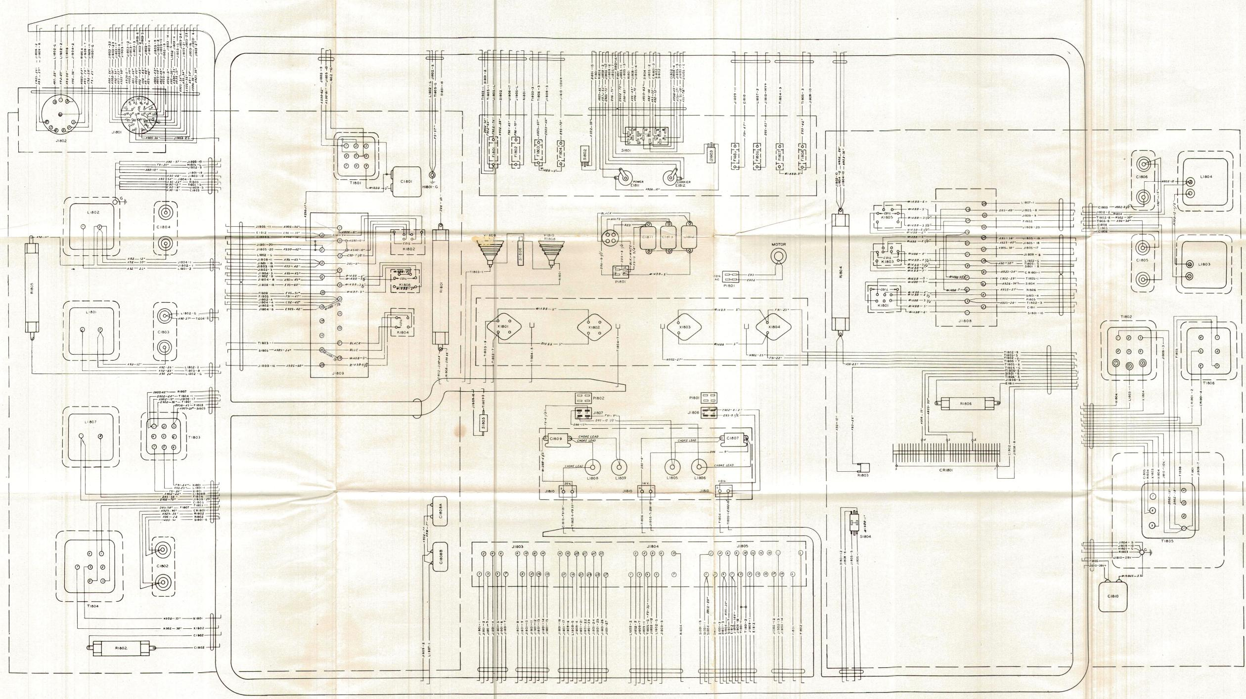
FIG. 101 TYPE COL-211101 MOTOR-GENERATOR-RECTIFIER POWER UNIT PRACTICAL WIRING DIAGRAM (Dwg. No. 500 4446 00F)
