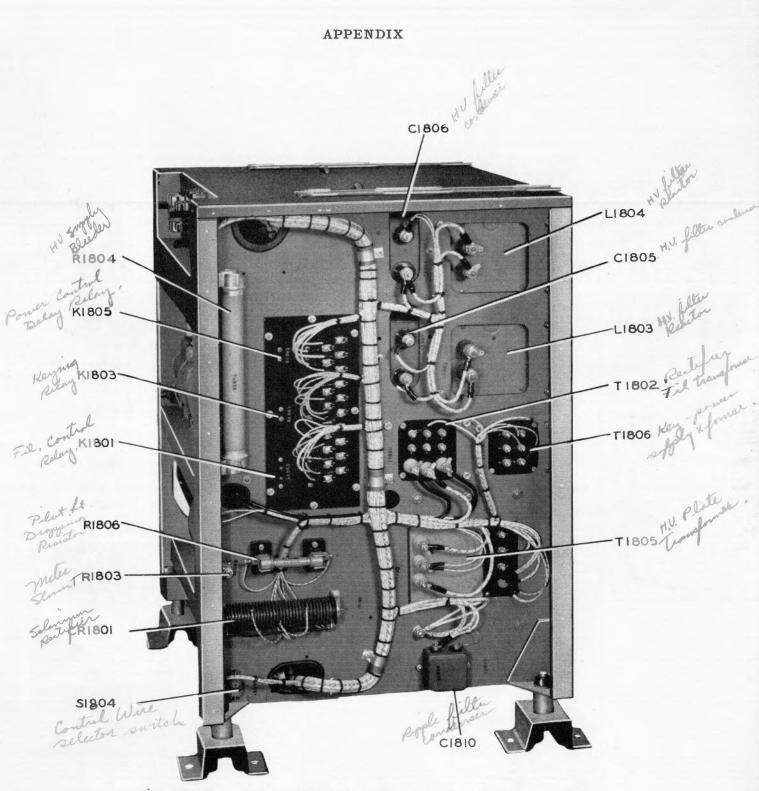
Fig. 60 Type COL-211101 Motor-Generator-Rectifier Power Unit Right Side Open View
