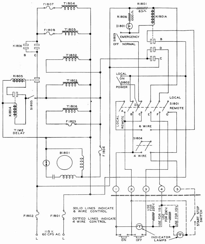
Fig. 11 Simplified Power Control Circuits for A.C. Power Unit (Dwg. No. 500 1458 00B)
