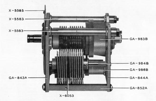
Fig. 75 96J Autotune Singleturn Unit-Right Side View
