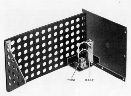
Fig. 52 Dummy Low-Frequency Oscillator Unit-Side View
