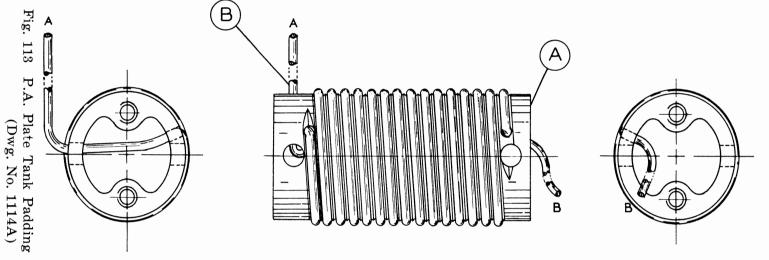
P.A. Plate Tank Padding Inductor L114 (Dwg. No. 1114A)
