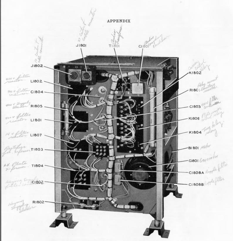
Fig. 61 Type COL-211101 Motor-Generator-Rectifier Power Unit Left Side Open View
