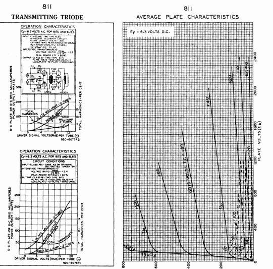
D-C PLATE(Ib)OR D-C GRID(IC) MILLIAMPERES
