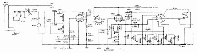
Fig. 21 Low Frequency R-F Circuits (Dwg. No. 500 1460 00C)
