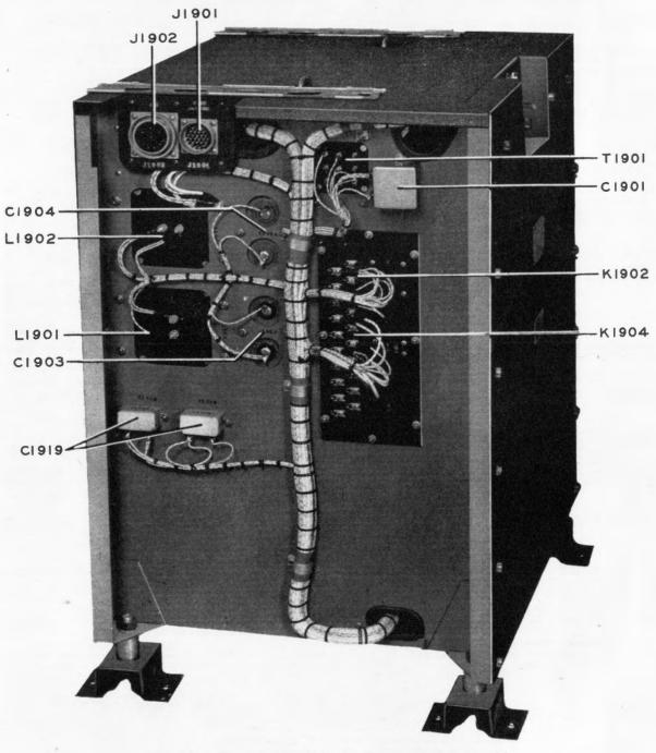
Fig. 65 Type COL-211102 Dynamotor Assembly Left Side Open View
