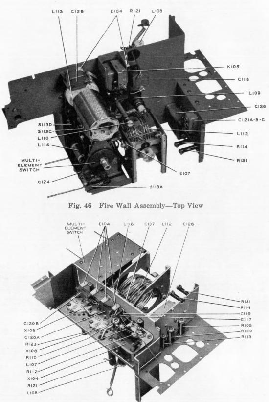
Fig. 47 Fire Wall Assembly-Bottom View
