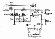
Fig. 20 CFI Oscillator Circuit (Dwg. No. 500 0221 00A)
