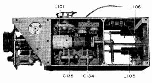
Fig. 32 High Frequency Oscillator
