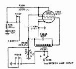
Fig. 19 MCW Oscillator Circuit (Dwg. No. 500 0219 00A)
