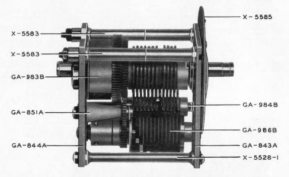
Fig. 74 96J Autotune Singleturn Unit-Left Side View
