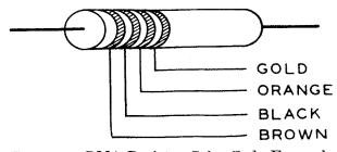
Fig. 123 RMA Resistor Color Code Example (Dwg. No. 500 0242 00A)
