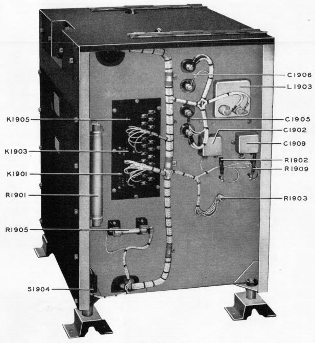
Fig. 64 Type COL-211102 Dynamotor Assembly Right Side Open View
