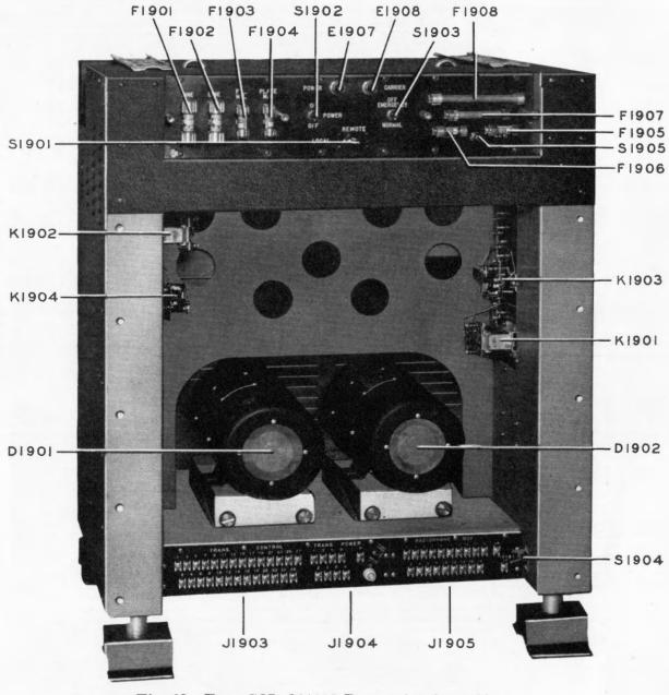
Fig. 63 Type COL-211102 Dynamotor Assembly Front Open View
