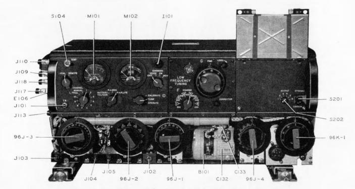
Fig. 41 Type COL-52286 Transmitter Unit-Front Open View
