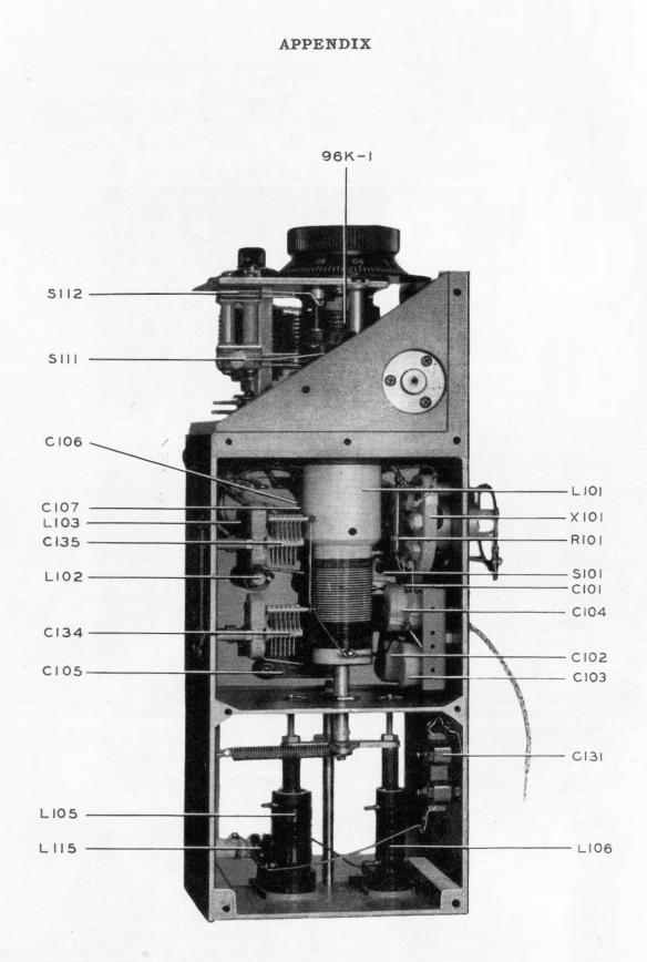
Fig. 44 High-Frequency Oscillator-Side Open View
