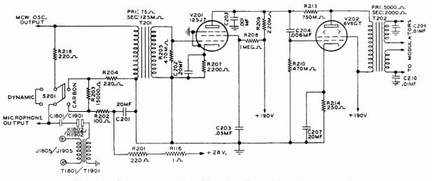
Fig. 16 Speech Amplifier Circuits (Dwg. No. 500 1453 00A)
