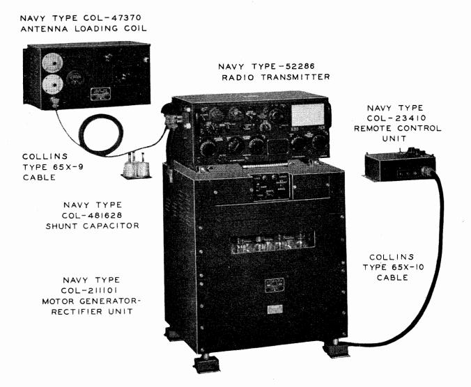
Fig. 1 Complete TCZ Equipment Navy Type COL-211101 Power Unit Shown
