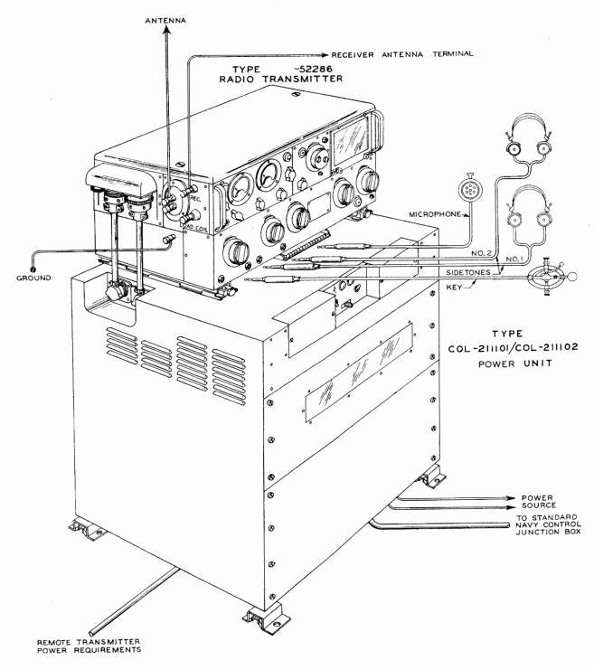
Fig. 28 Simplified TCZ Installation Diagram (Dwg. No. 500 1474 00D)
