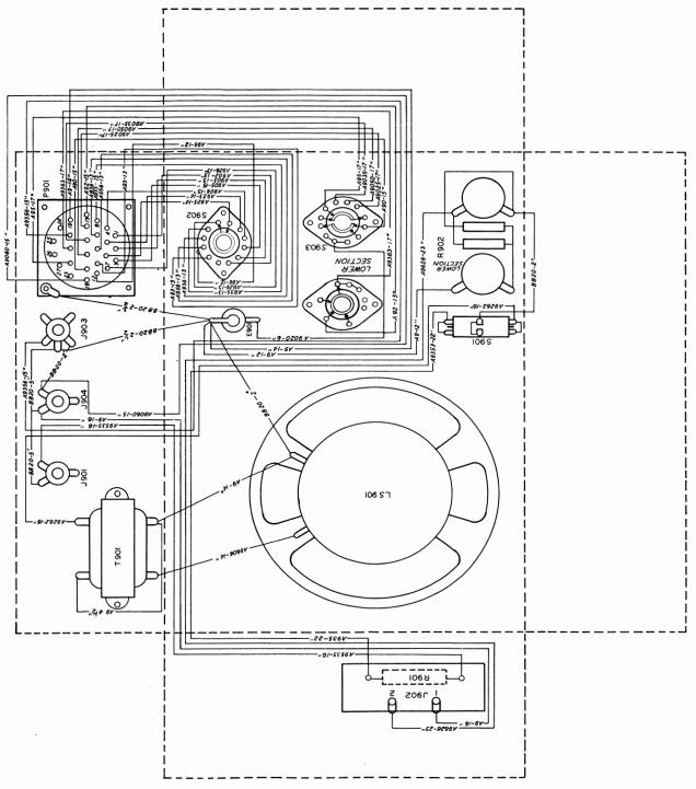
Fig. 103 Type COL-23410 Remote Control Unit Practical Wiring Diagram (Dwg. No. K1064C)
