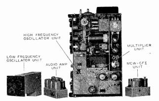
Fig. 4 Type -52286 Transmitter Top View Open—Units Removed
