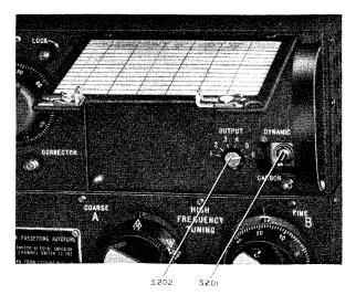
Fig. 30 Microphone Switch and Sidetone Amp. Gain Control
