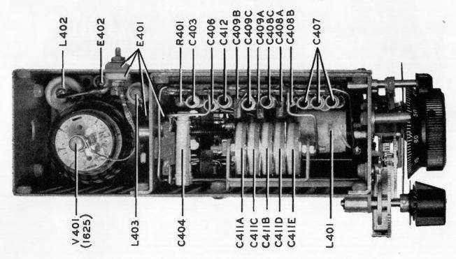
Fig. 49 Low-Frequency Oscillator Unit-Top Open View
