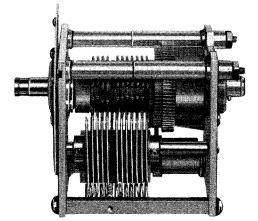
Fig. 35 96J Autotune Singleturn Unit Right Side View
