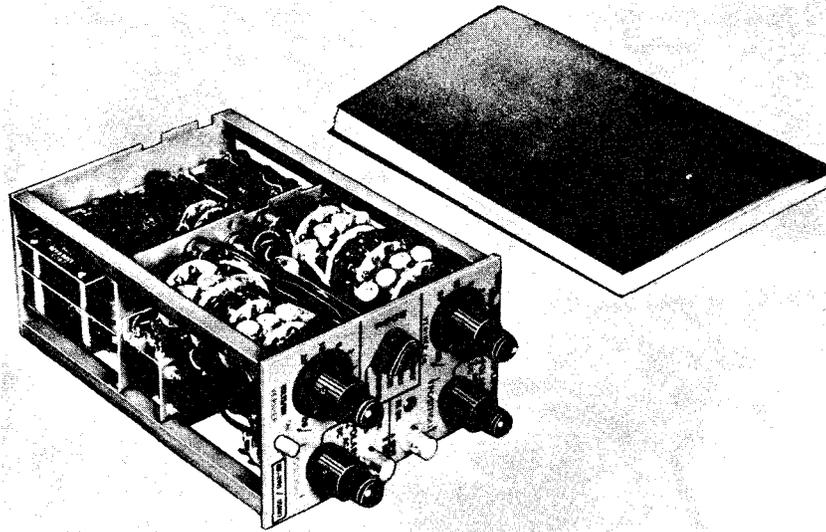
OSCILLOSCOPE SUB-ASSEMBLY. VERTICAL CHANNEL,
