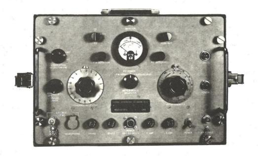
A portable, special purpose equipment used to supply radio frequency signals to Radio Receiving Set AN/ARR-26 and AN/ARR-26A during test and alignment procedures. Output of the equipment is indicated by a meter, calibrated controls, and selector switches.
