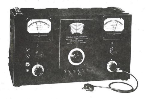
A portable, general purpose, laboratory instrument used for the measurement of sensitivity, selectivity, fidelity overload, distortion, automatic gain control, image and intermediate frequency rejection ratios, and noise and stage gain characteristics. Test results are indicated on a motor-driven direct-reading linear scale.
