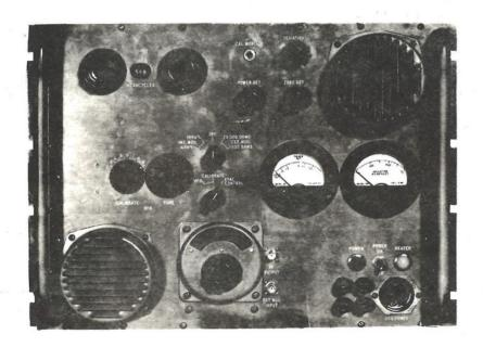
A portable, special purpose equipment designed to furnish RF test signals at an accurately adjustable frequency and power level. This equipment is used in testing AN/ARW-56. The generator includes provisions for both external and internal frequency modulation. Indication is in decibels by means of a thermistor bridge circuit, and in megacycles per second on a calibrated tuning control.
