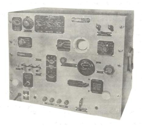
A rack-panel mounted unit suitable for use as a conventional signal generator but designed specifically for Loran application. Internally and externally modulated pulse and continuous signals are available. Master and slave pulses may be independently controlled in amplitude and the slave may be delayed by variable amounts from the master pulse. Primary application is to Loran maintenance and repair work.
