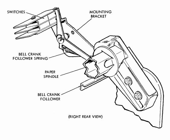
Figure 45 - Paper Out Contacts (Friction Feed)
