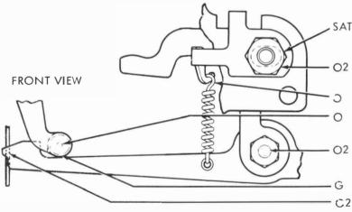
2.09 Transfer Lever Mechanism
