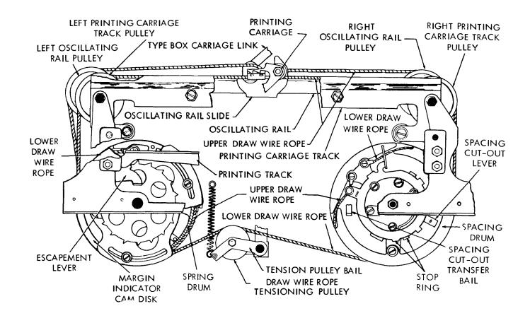
Figure 18 - Draw Wire Rope and Drums
