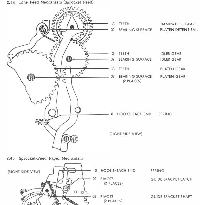
0 HOOKS-EACH END SPRING PACK PIN AND SPRING G SPROCKET WITH STEEL PINS CAVATIES (22 PLACES) G LIGHT COAT SPROCKET WITH DELRIN PINS NOTE: BEFORE ATTEMPTING TO DISASSEMBLE ON PIN CONTACTING THE 153700 PLATEN HUB, SEE DISASSEMBLY SURFACE OF CAM. AND REASSEMBLY INSTRUCTIONS IN THE DO NOT PACK WITH APPROPRIATE SECTION. GREASE
