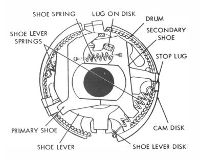
Figure 9 - Three Stop Clutch
