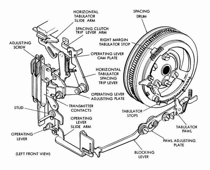
Figure 47 - Horizontal Tabulation Mechanism
