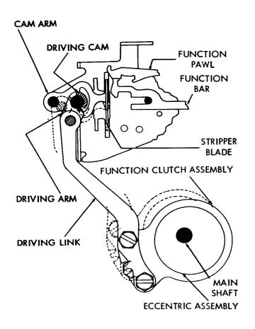
Figure 36 - Stripper Blade Mechanism
