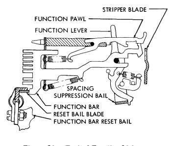
Figure 34 - Typical Function Linkage (Unselected)
