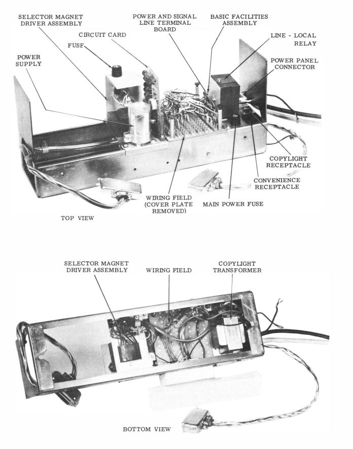
Figure 1 - Typical Electrical Service Unit for 35 KSR Set
