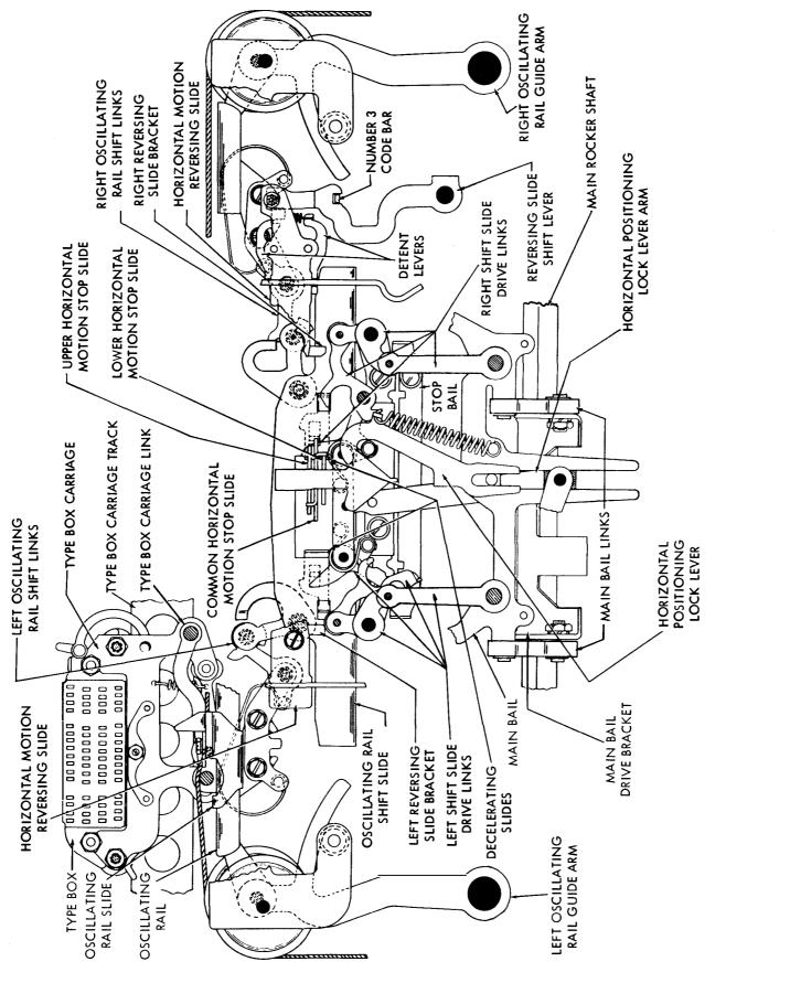
Figure 23 - Horizontal Positioning Mechanisms
