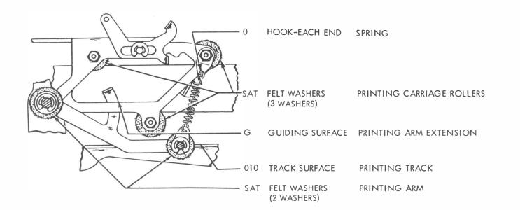
2.03 Type Box Carriage Mechanism
