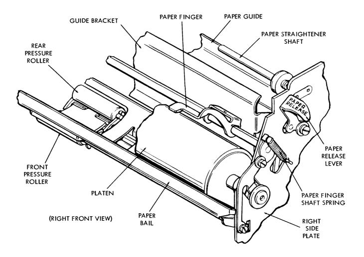
Figure 43 - Friction Feed Platen Mechanism
