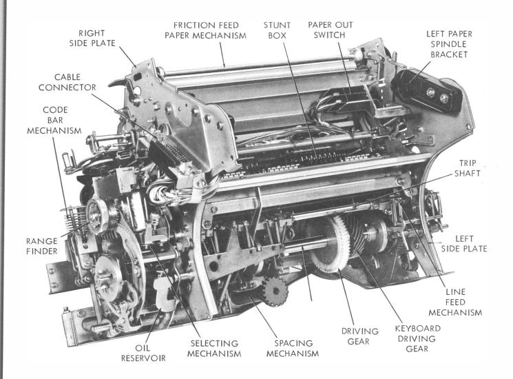
Figure 3 - 35 Typing Unit (Friction Feed) (Right Rear View)
