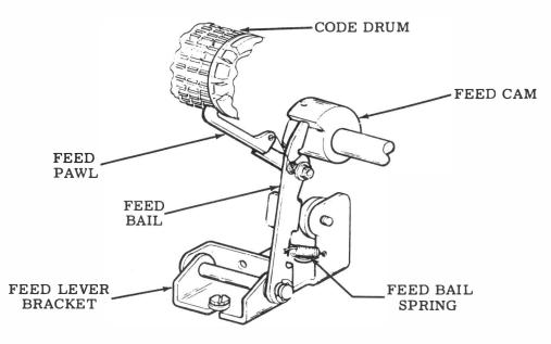
Figure 8 - Feed Mechanism
