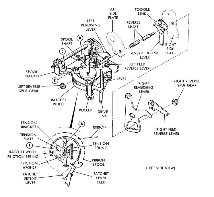
Figure 28 - Ribbon Feed and Reverse Mechanisms
