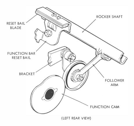
Figure 32 - Reset Bail Mechanism
