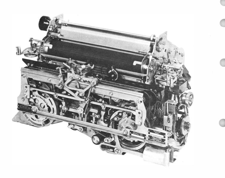
Figure 1 - 35 Typing Unit - Friction Feed
