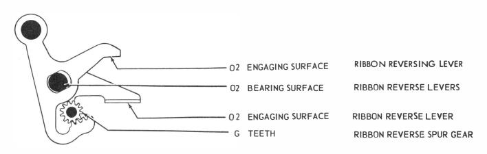
2.13 Vertical Positioning Mechanism (Right Side)
