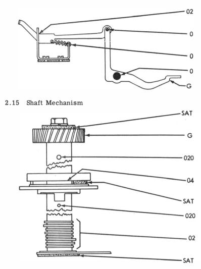
2.16 Intermediate Gear Mechanism
