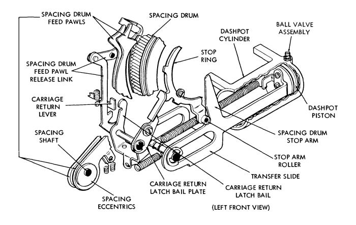
Figure 38 - Carriage Return Mechanism
