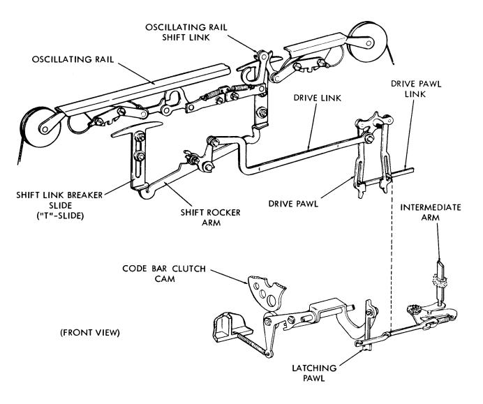
Figure 19 - Shift Mechanism
