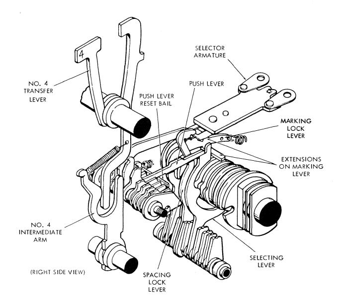
Figure 13 - Selecting Mechanism and Transfer Mechanism
