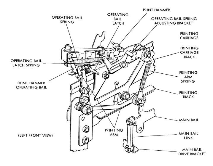
Figure 25 - Print Hammer and Carriage
