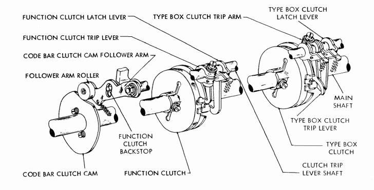
Figure 22 - Clutch Trip Mechanisms
