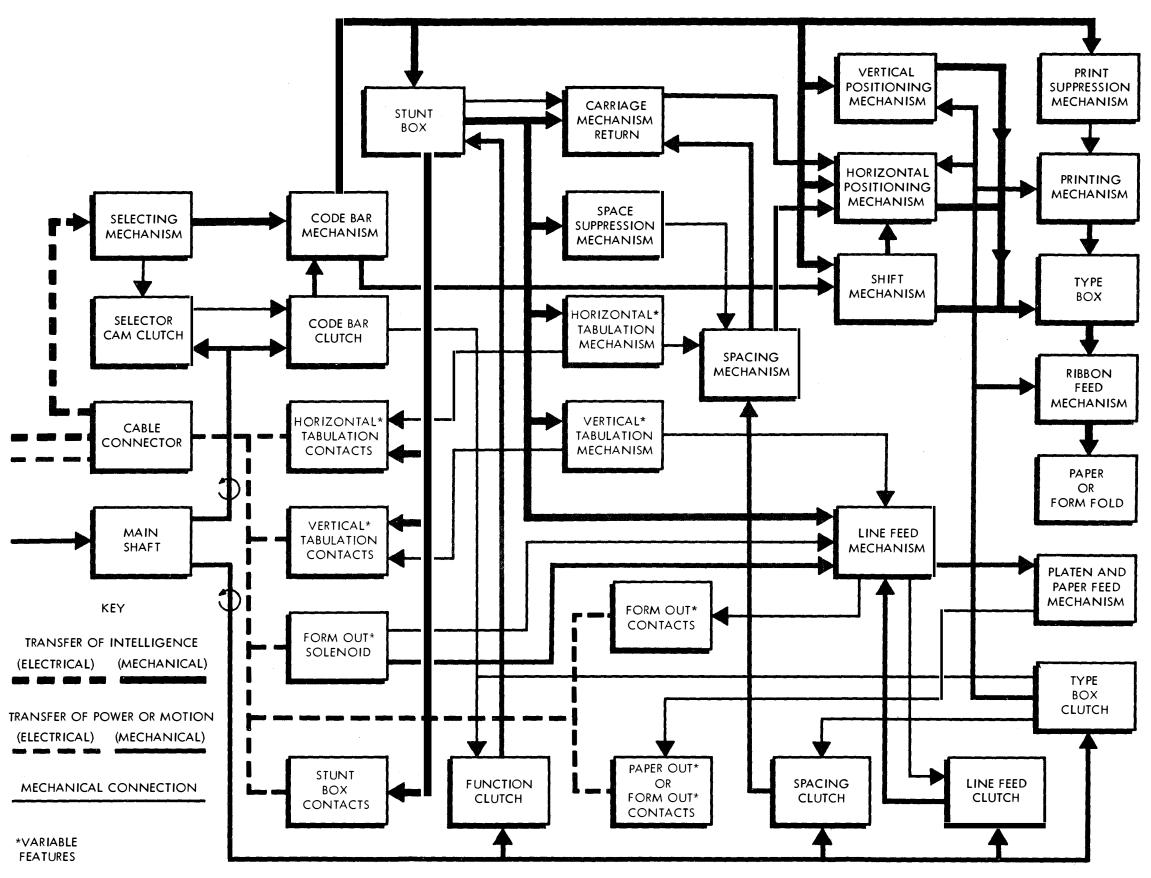
Figure 7 - 35 Typing Unit Block Diagram
