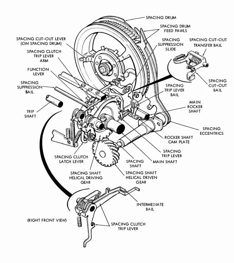
Figure 27 - Spacing Mechanism
