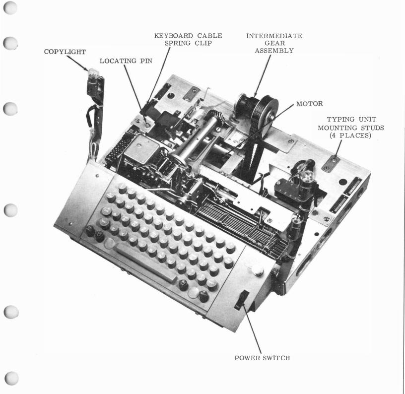
Figure 3 - 35 Keyboard for Wall Mounted Send-Receive Sets
