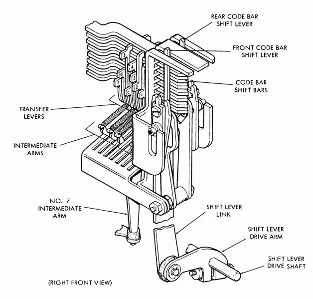
Figure 14 - Code Bar Mechanism
