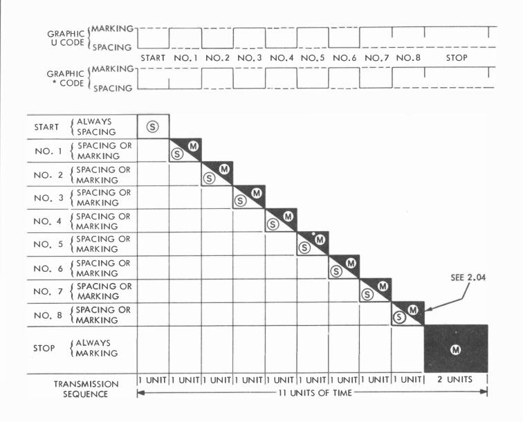
Figure 5 - 11.0 Unit Transmission Pattern Signaling Code
