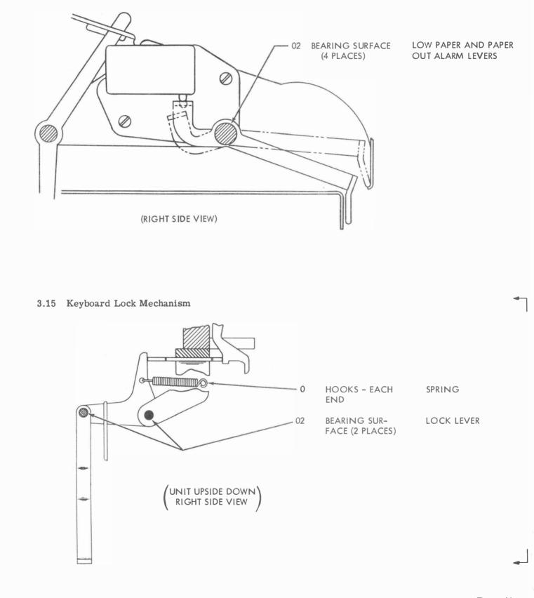
3.14 Low Paper and Paper Out Alarm Mechanism (Sprocket Feed)
