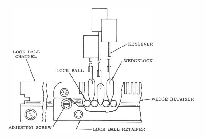
Figure 6 - Wedgelock Mechanism
