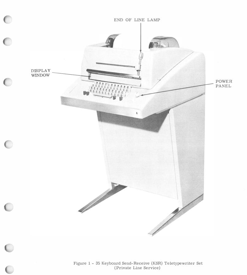
Figure 1 - 35 Keyboard Send-Receive (KSR) Teletypewriter Set (Private Line Service)
