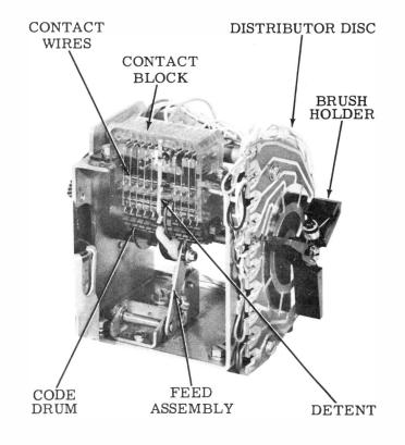
Figure 3 - Answer-Back Mechanism (Rear View)
