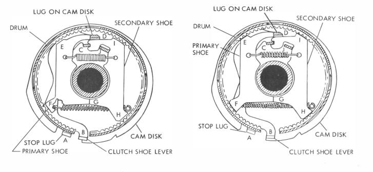
Figure 10 - One Stop Clutch (Disengaged)
