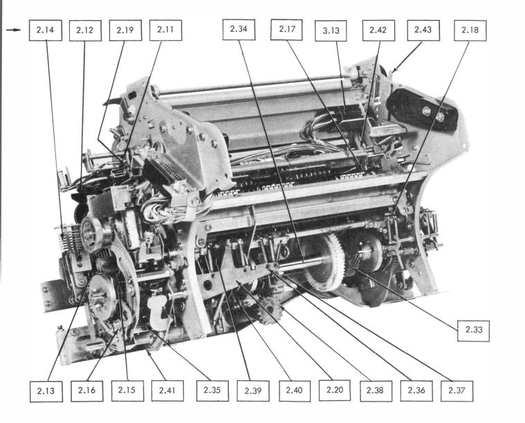
Figure 2 - 35 Typing Unit (Friction Feed), Right Rear View
