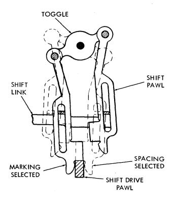
Figure 20 - Shift Mechanism Positioning
