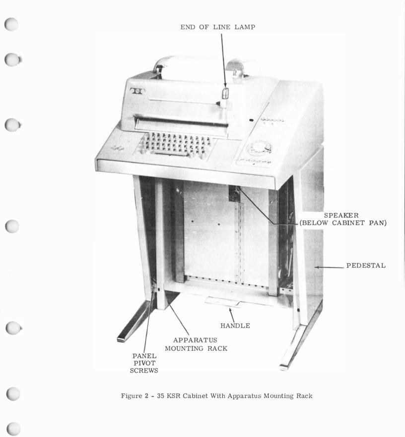
Figure 2 - 35 KSR Cabinet With Apparatus Mounting Rack
