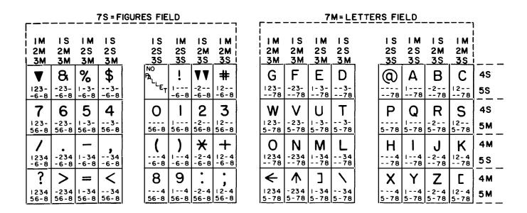
Figure 17 - Type Box Pallet Arrangement
