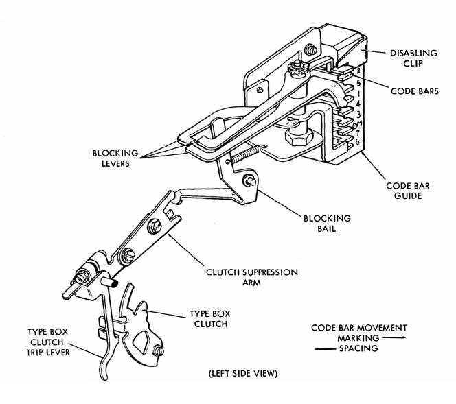
Figure 26 - Print Suppression Mechanism
