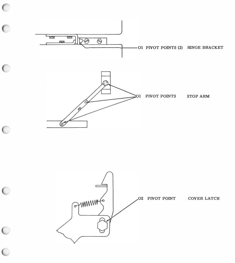
2.03 Upper and Lower Cover Hinge and Latch, Wall Mounted Cabinet
