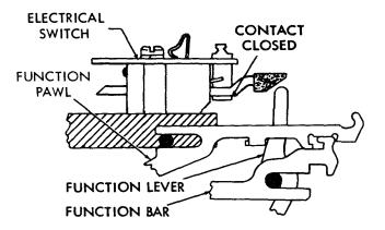
Figure 42 - Typical Box Contact (Selected)
