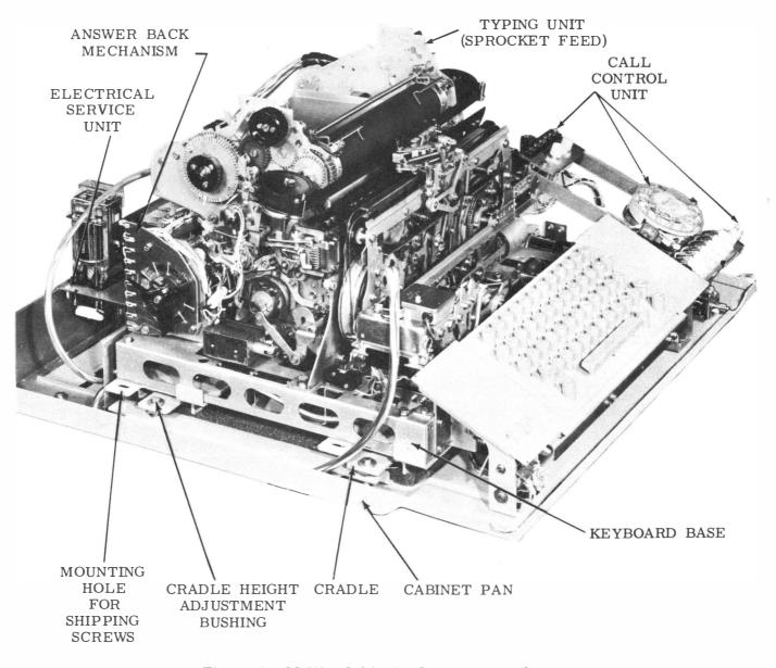
Figure 4 - 35 KSR Cabinet - Cover Removed
