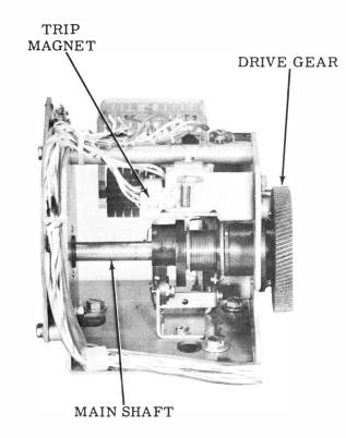
Figure 4 - Answer-Back Mechanism (Front View)
