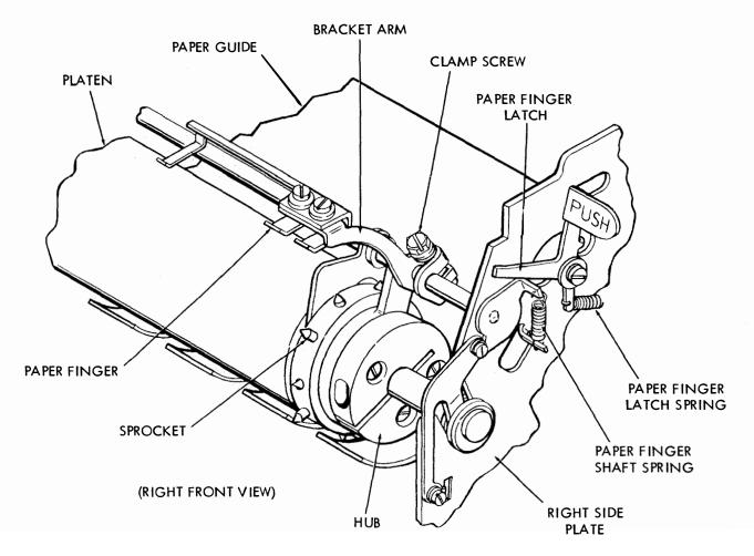
Figure 44 - Sprocket Feed Platen Mechanism
