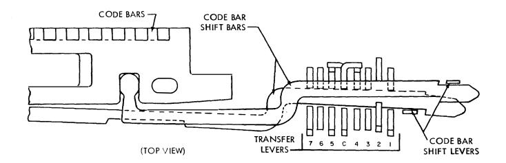
Figure 15 - Code Bar Shift Bar Positioning
