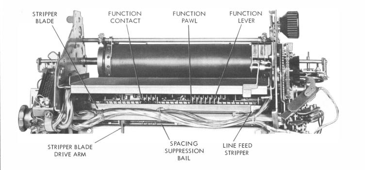
Figure 31 - Stunt Box Installed in Sprocket Feed Typing Unit (Rear View)
