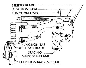
Figure 35 - Typical Function Linkage (Selected)
