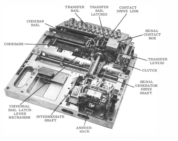
Figure 2 - 35 Keyboard for Send-Receive Sets (Rear View)
