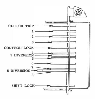
Figure 11 - Codebar Arrangement With Even Parity
