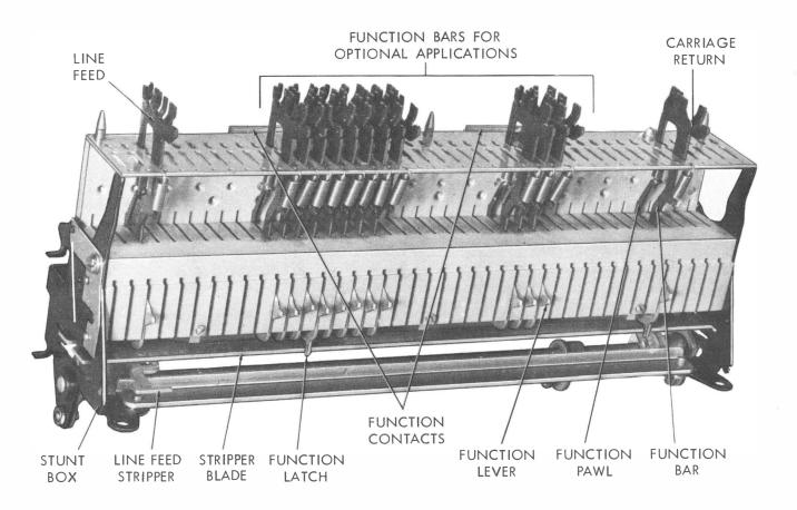
Figure 30 - Typical Stunt Box (Bottom View)
