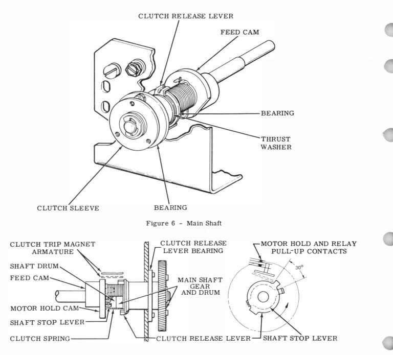
Figure 7 - Spring Clutch
