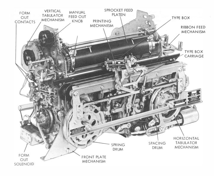
Figure 4 - 35 Typing Unit (Sprocket Feed) (Left Front View)
