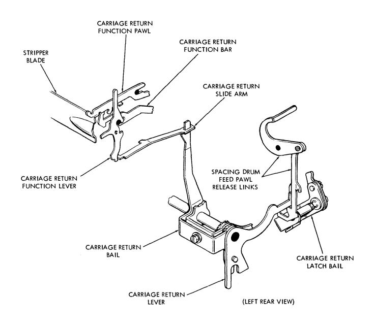
Figure 37 - Carriage Return Function Mechanism
