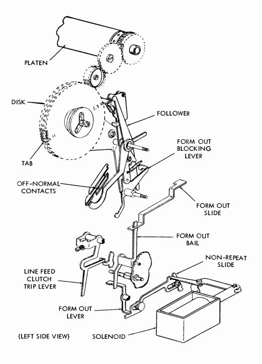
Figure 49 - Form Out Mechanism (Sprocket Feed)
