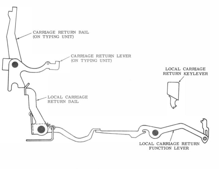
Figure 10 - Local Carriage Return Mechanism
