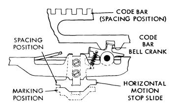
Figure 24 - Stop Slide Positioning
