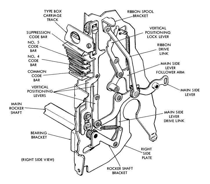
Figure 21 - Right Side Plate Mechanisms
