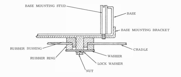
Figure 6 - Base Isolator Assembly
