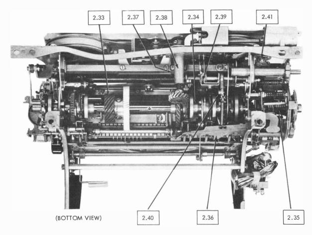
2.33 Main Shaft (Clutches, Gears, etc.) (Bottom View)
