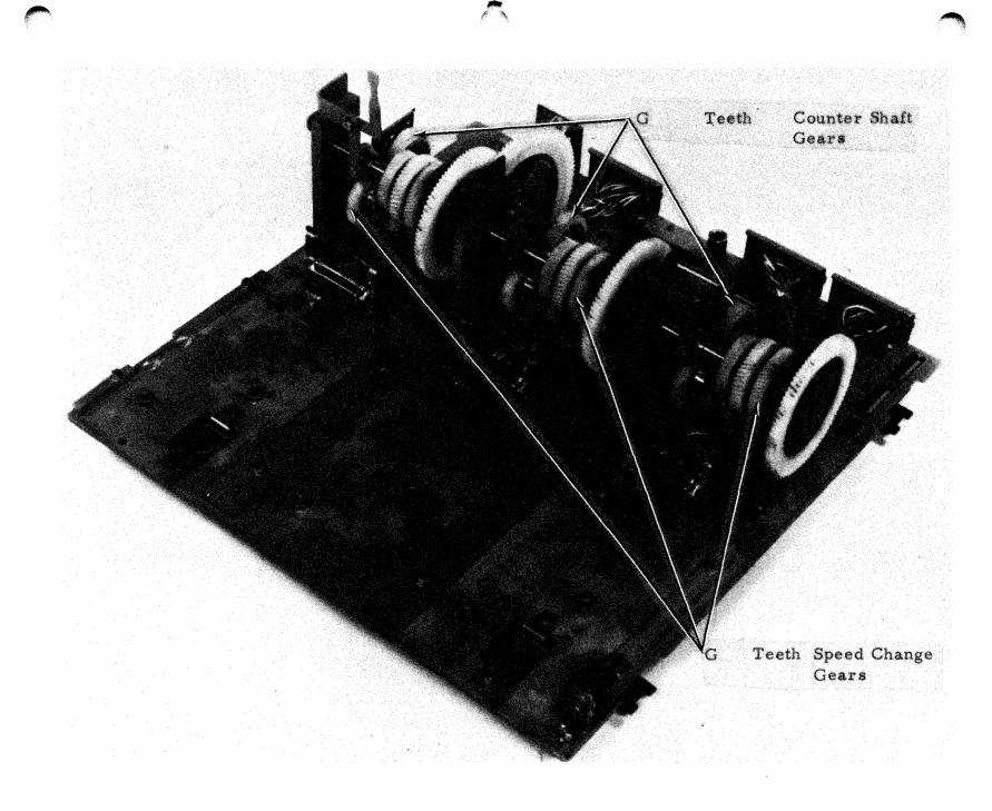
Figure 4-36. Drive Gears and Speed Change Gears - Multicontact Multiple Mounting Bases (Variable Speed)
