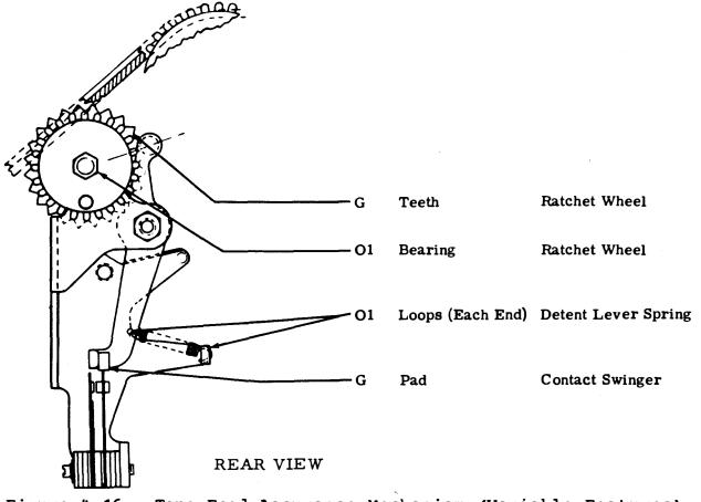
Figure 4-16. Tape Feed Assurance Mechanism (Variable Features)
