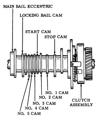
Figure 3-14. Clutch Camshaft Assembly
