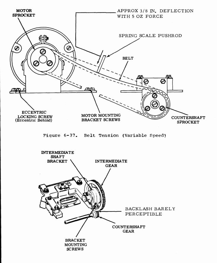
Figure 6-38. Intermediate Gear - Countershaft Gear Backlash
