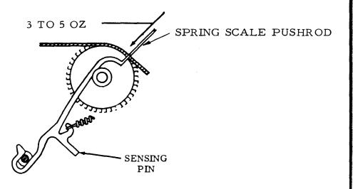
Figure 6-24. Sensing Pin Spring
