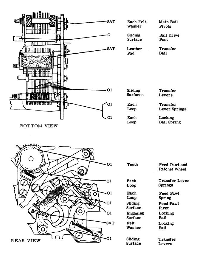
Figure 4-15. Transfer Mechanism
