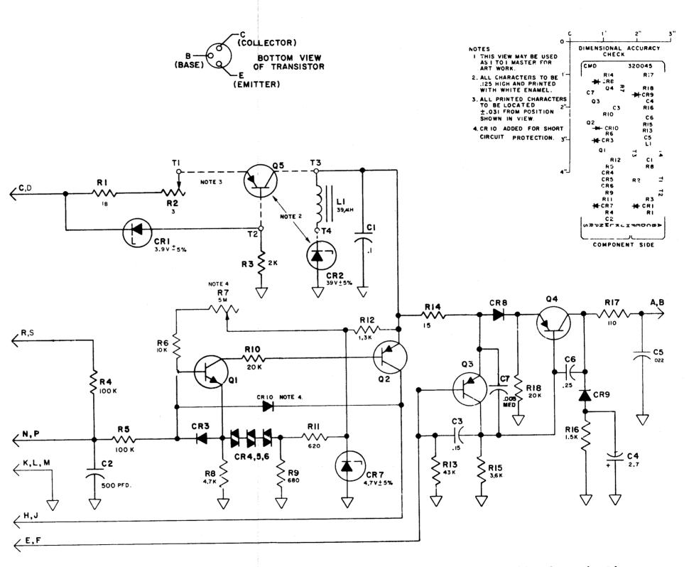
Figure 5-15. Clutch Magnet Driver 321991 Schematic Diagram (Sheet 2 of 2)
