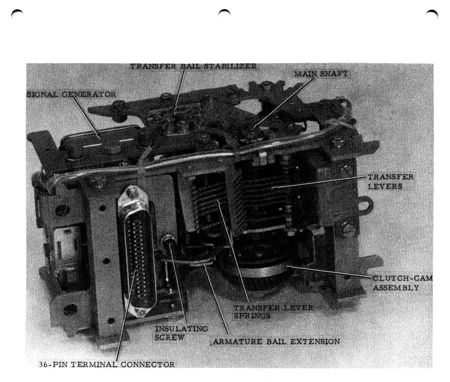
eccentrics, and a clutch. Motor power to the shaft is obtained from an external source and is controlled by the clutch and the clutch trip magnet assembly.
