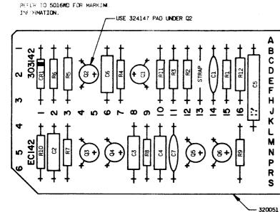
ALPHA NUMERIC CONVERSION CHART NUMERICAL CONVERSION FOR STAMPING 15 PT. CARDS WHEN USED WITH 36 PT. CONNECTOR ON CIRCUIT WHEN INSERTED WHEN INSERTED BOARD IN UPPER HALF IN LOWER HALF OF CONNECTOR OF CONNECTOR 22 A В 2 23 24 3 С D 4 25 5 26 F 27 F 6 н 7 28 8 29 J ĸ 9 30 10 31 L 11 м 32 N 12 33 13 P 34 14 R 35 15 S 36
