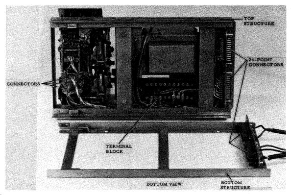
Figure 1-11. Transmitter Distributor Base - Multicontact, Single Mounting Structural View (Transmitter Distributor and Motor Unit in Place)
