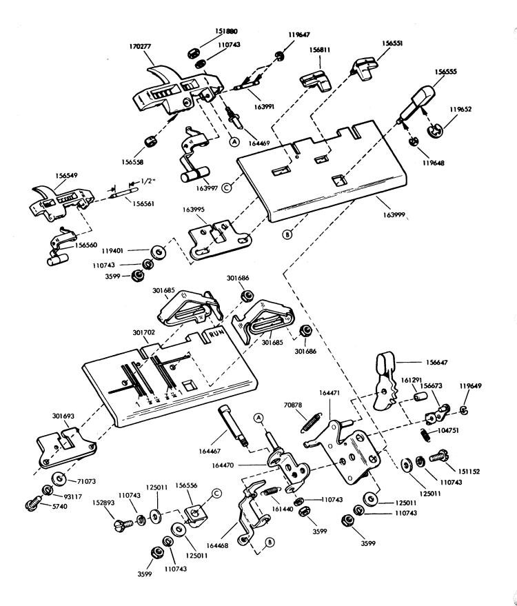
Figure 7-17. Tape Guide Plate Mechanisms (Sheet 3 of 3)
