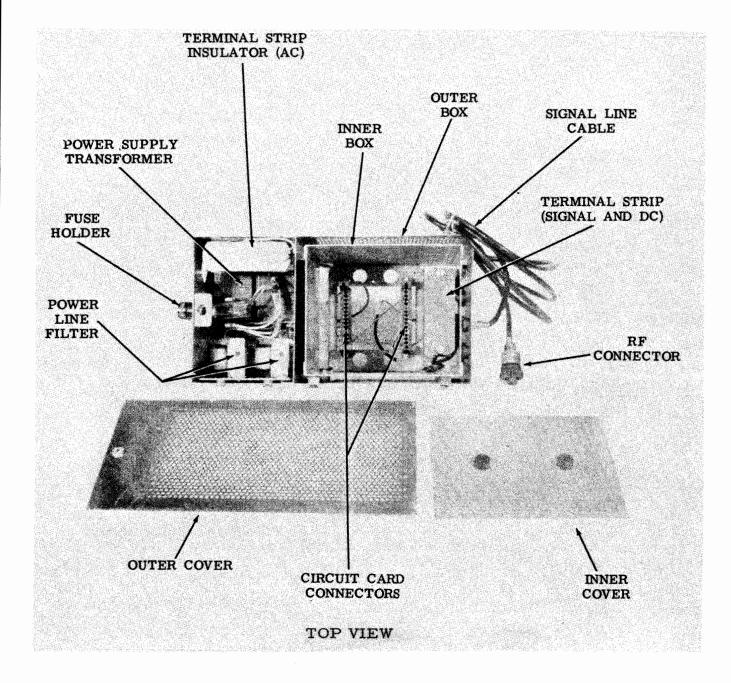
Figure 3-23. Typical Parts of an ESA - Double Box Construction (Sheet 1 of 2)
