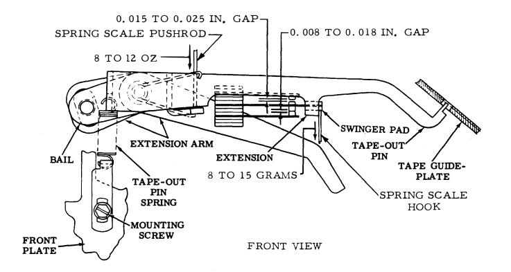
Figure 6-52. Tape-Out Contact and Tape-Out Bail Torsion Spring
