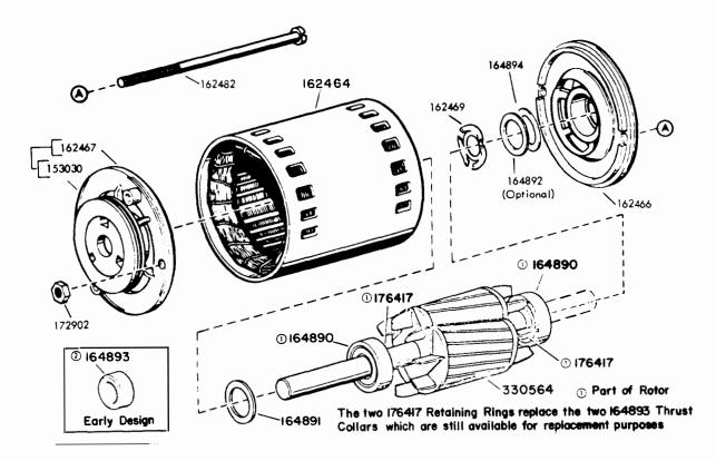
Figure 7-39. Synchronous Motor Assembly 151795 (Standard) -Used on LMU3 and LMU38
