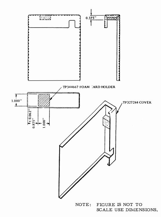
Figure 8-2. Circuit Card Hold-Down Installation for ESA TP326792 (Sheet 2 of 2)
