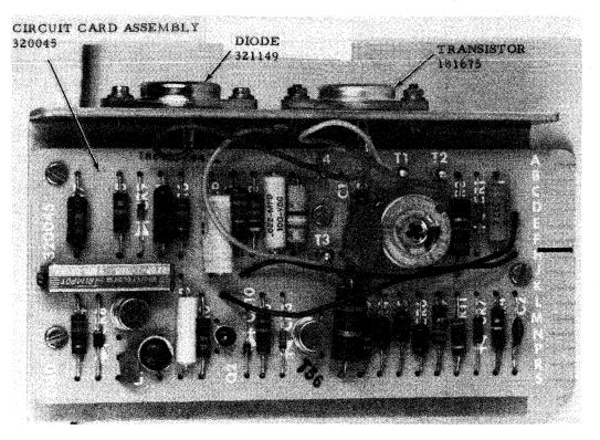
Figure 3-26. Clutch Magnet Driver TP321991 for Low-Level Operation
