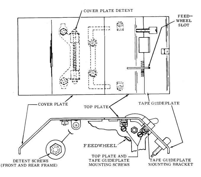
Figure 4-1. Transmitter Distributor Plate Removal Details
