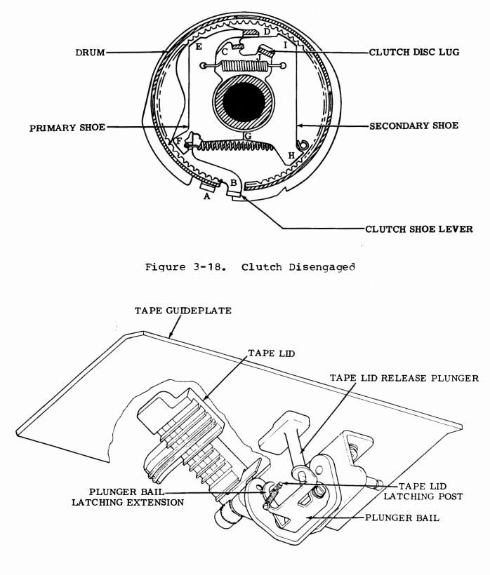
Figure 3-19. Tape Lid Mechanism - Bottom View
