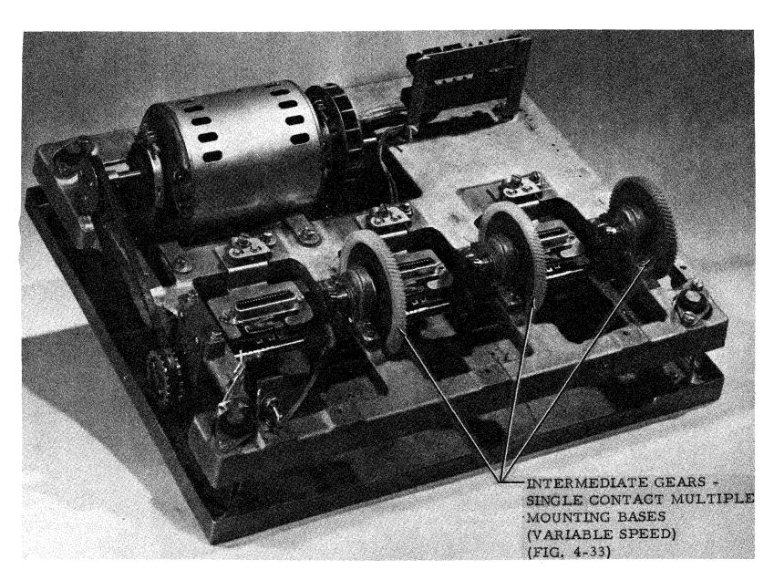
Figure 4-32. Single Contact Multiple Mounting Bases (Variable Speed)
