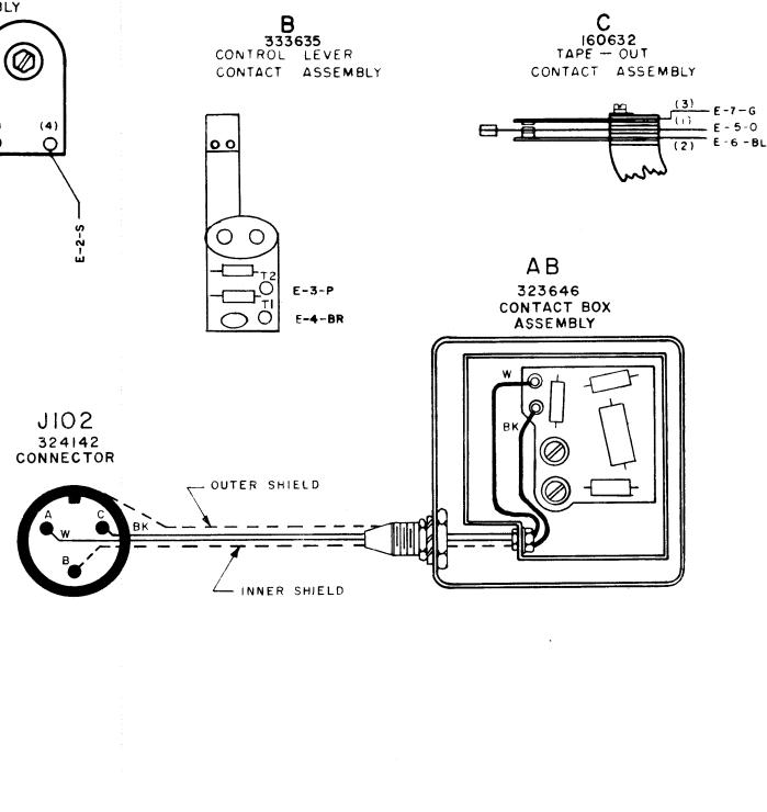
Figure 5-10. Transmitter Distributor Unit LXD37, 38 Wiring Diagram
