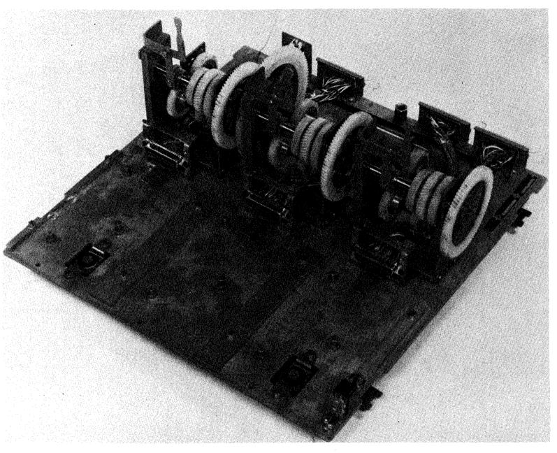
Figure 1-16. Transmitter Distributor Base - Multicontact, Multiple Mounting (Variable Speed)
