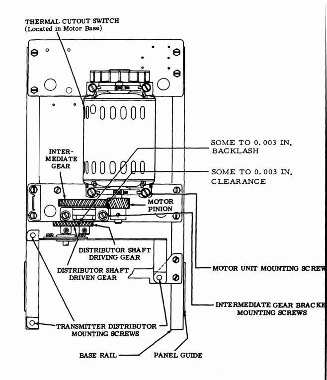
Figure 6-40. Intermediate Gear Assembly and Motor Pinion
