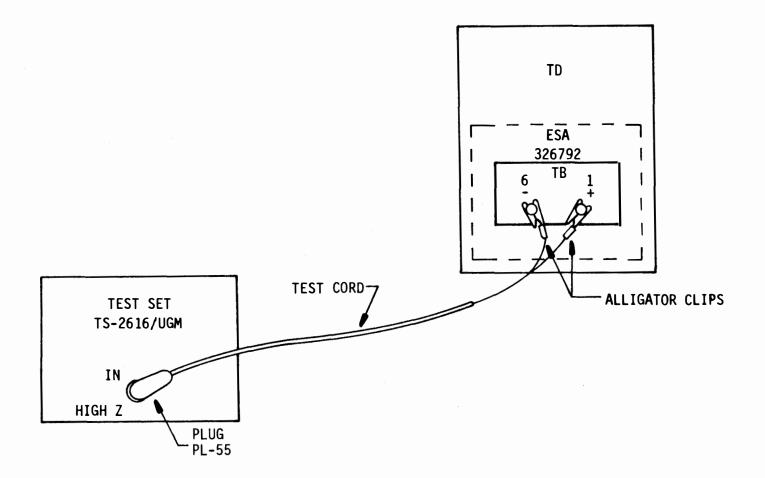
Figure 4-3. TD Test Setup (Low-Level)
