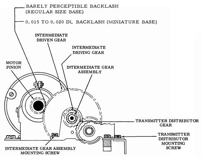
Figure 6-33. Transmitter Distributor Gear and Intermediate Shaft Assembly
