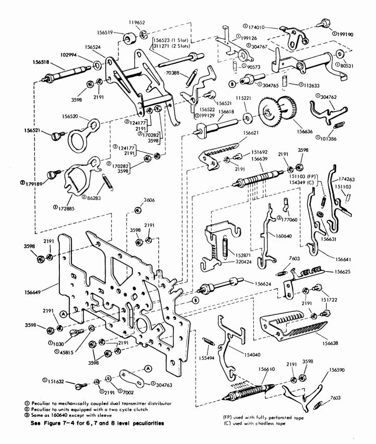
Figure 7-1. Front Plate Mechanism (Sheet 1 of 3)
