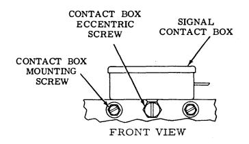
Figure 6-31. Signal Contacts - Electrical
