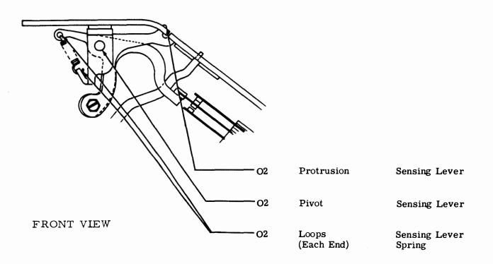
Figure 4-19. Tape Lid Sensing Lever (Variable Features)
