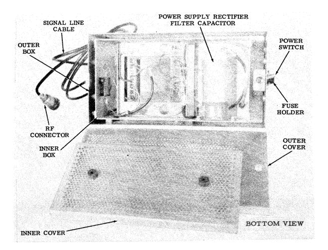
Figure 3-23. Typical Parts of an ESA - Double Box Construction (Sheet 2 of 2)
