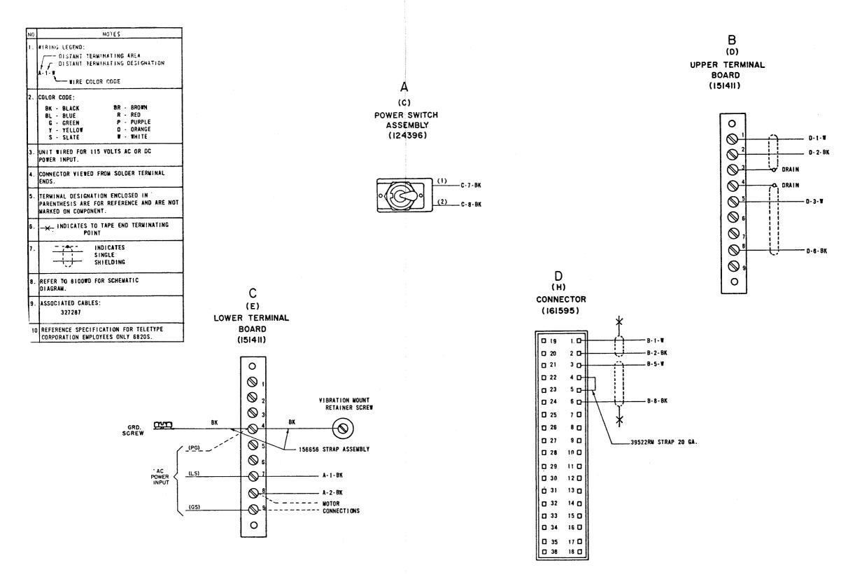
Figure 5-11. Transmitter Distributor Base LXDB20 Wiring Diagram
