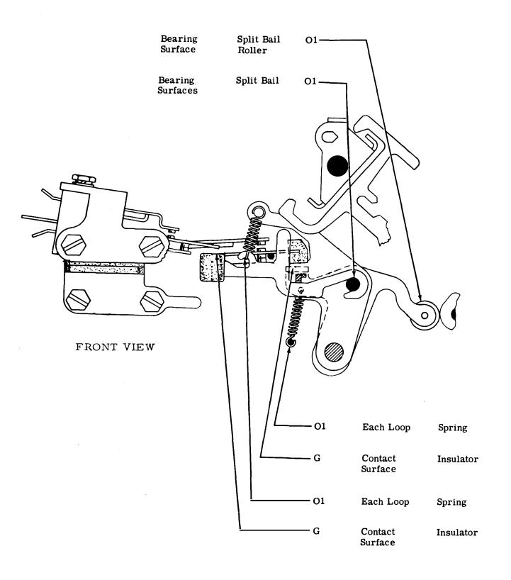
Figure 4-18. Code Reading Contacts (Variable Features)
