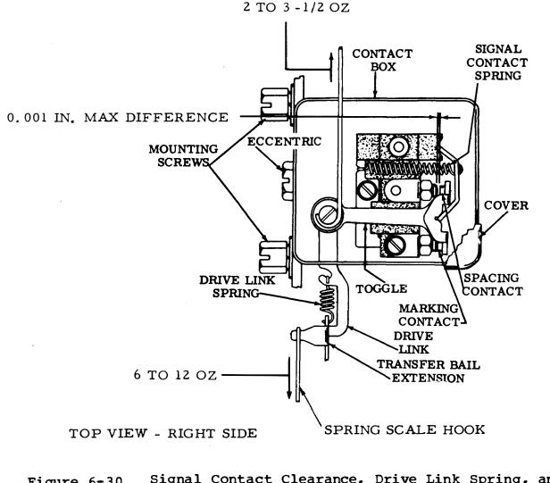
Figure 6-30. Signal Contact Clearance, Drive Link Spring, and Signal Contact Spring
