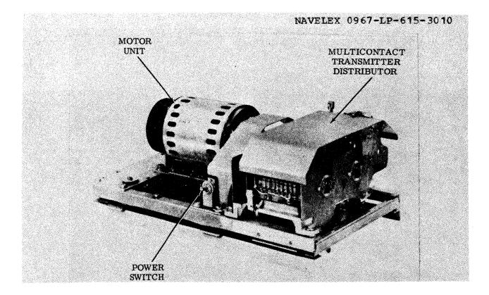
Figure 1-10. Transmitter Distributor Base - Multicontact, Single Mounting (Transmitter Distributor and Motor Unit in Place)
