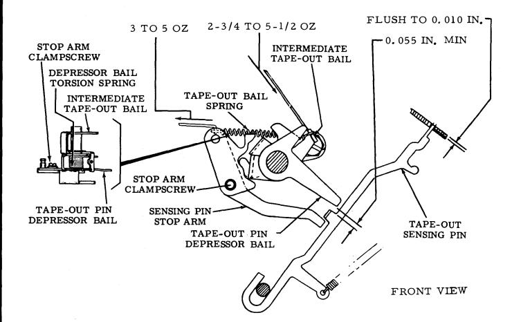
Figure 6-17. Tape-Out Sensing Pin, Depressor Bail Torsion Spring, and Intermediate Tape-Out Bail Spring
