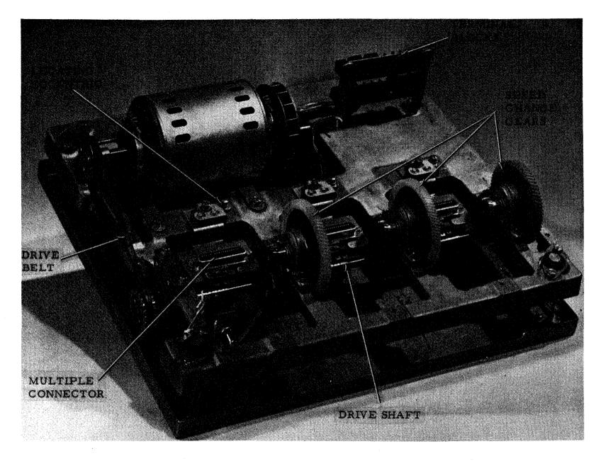
Figure 1-14. Transmitter Distributor Base - Single Contact, Multiple Mounting (Variable Speed)
