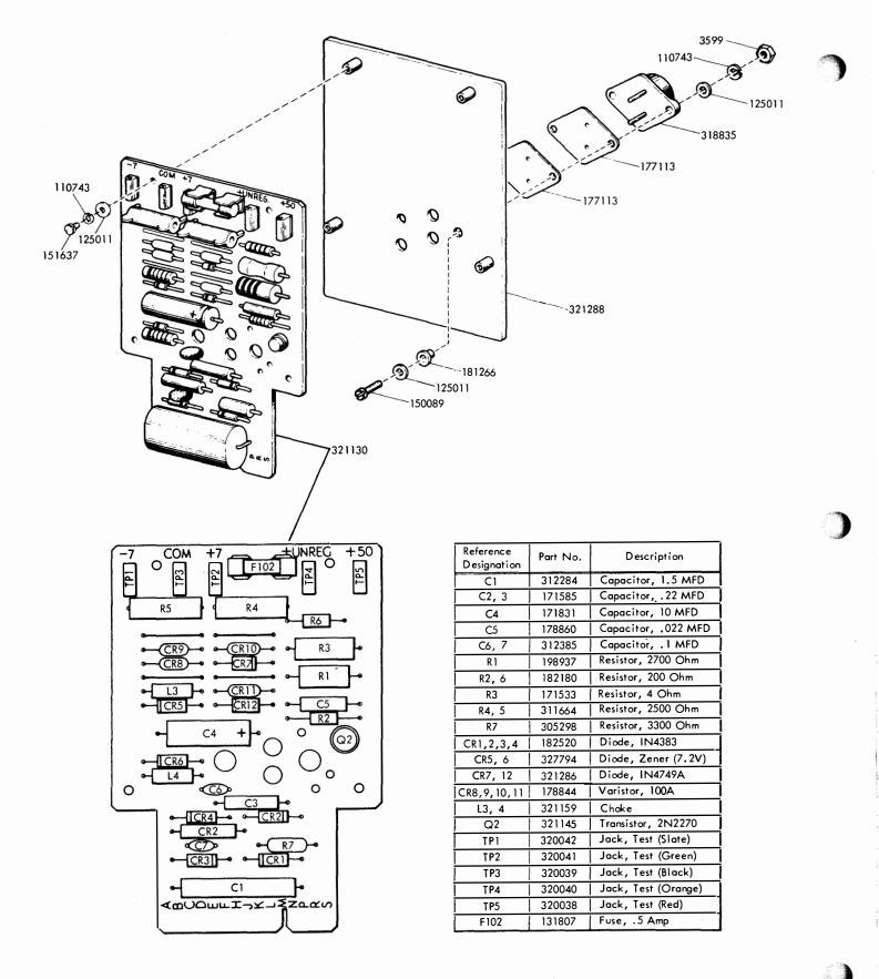
Figure 7-52. Power Supply Circuit Card 321290 (0.5 Ampere)
