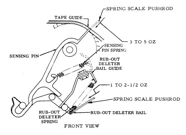
Figure 6-68. Sensing Pin Spring and Rub-Out Deleter Bail Spring
