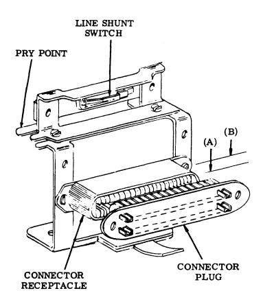
Figure 6-47. Line Shunt Switch
