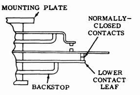
Figure 6-54. Normally-Closed Contacts - Backstop
