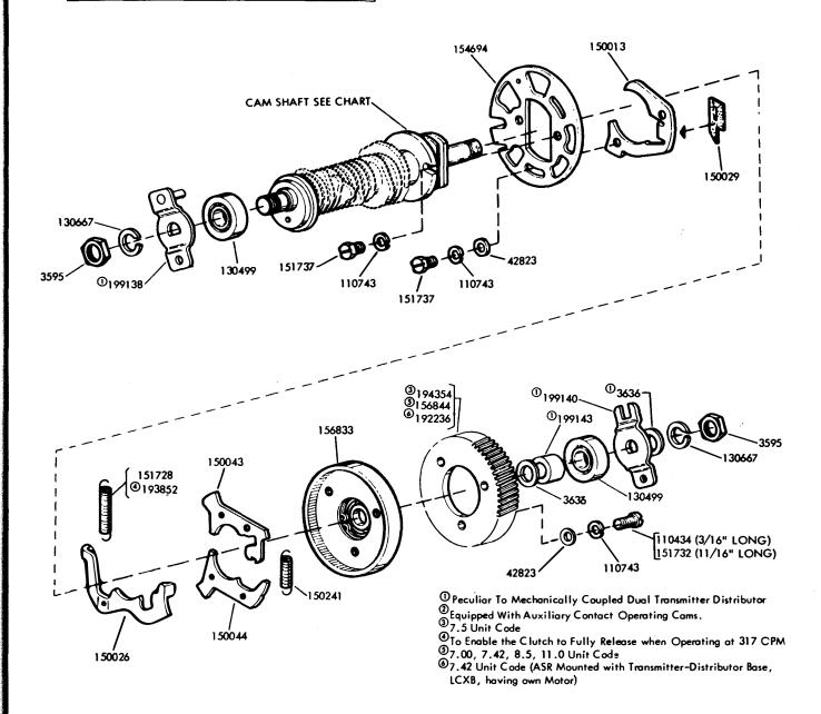
Figure 7-13. Main Shaft Mechanism (One-Cycle)
