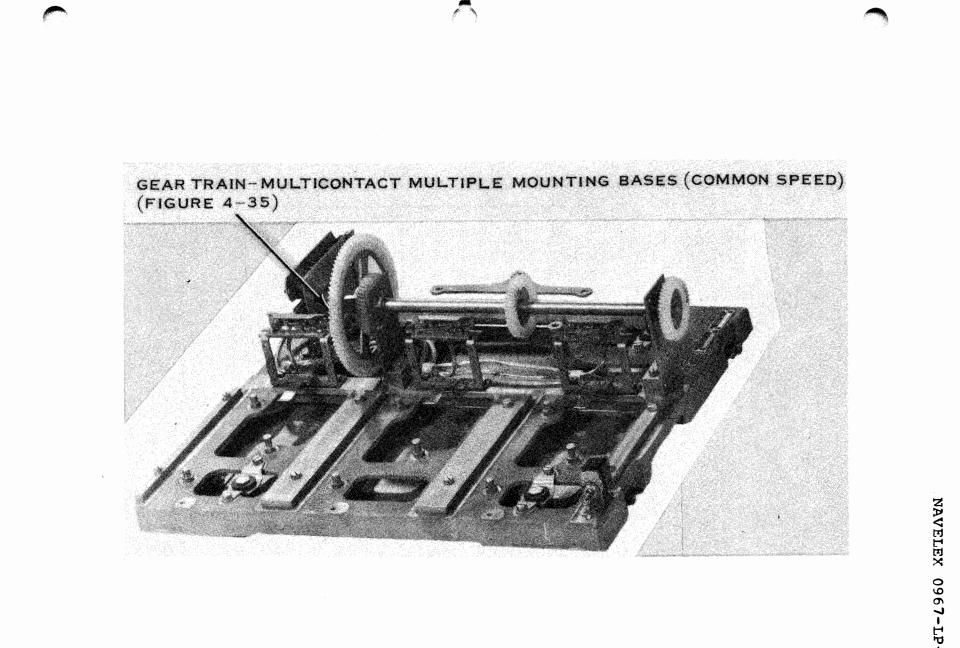
Figure 4-34. Multicontact Multiple Mounting Bases (Common Speed)
