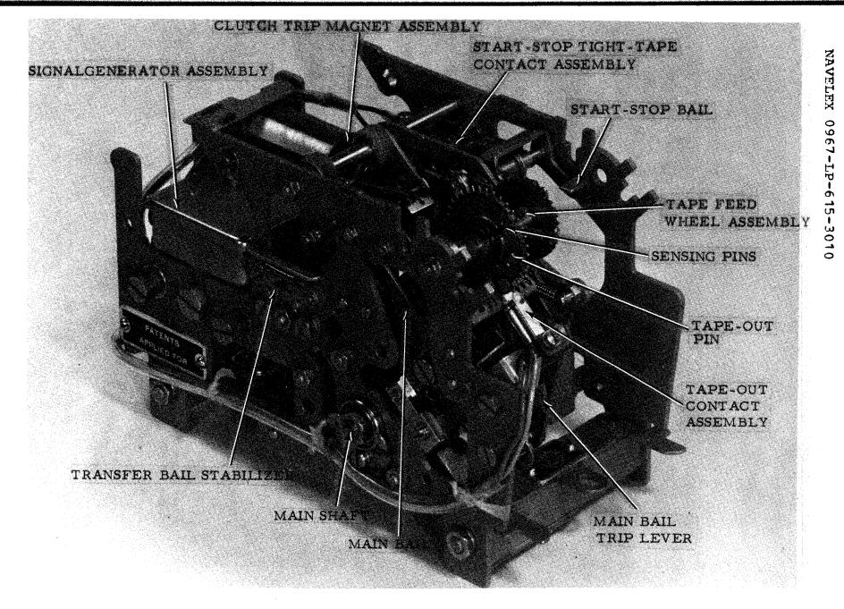
Figure 3-4. Transmitter Distributor Unit (Cover Plate, Top Plate and Tape Guideplate Removed)
