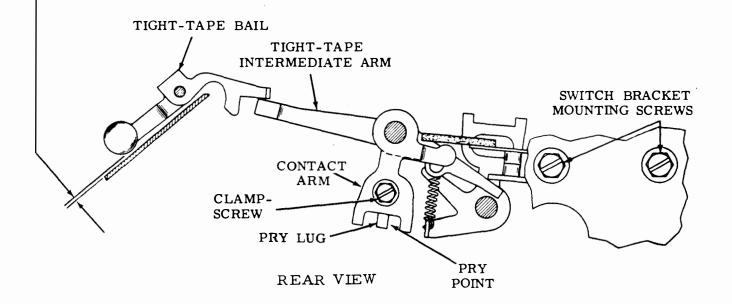
Figure 6-20. Start-Stop Switch Bracket (for Units Equipped with Tape Lid Sensing Lever)
