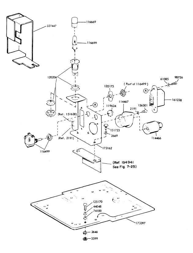
Figure 7-27. Miniature Base and Electrical Components (Sheet 2 of 2)
