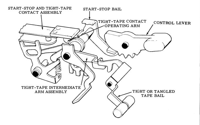
Figure 3-8. Start-Stop and Tight-Tape Switch Mechanisms
