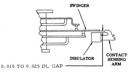
Figure 6-58. Contact Swinger - Sensing Arm Clearance
