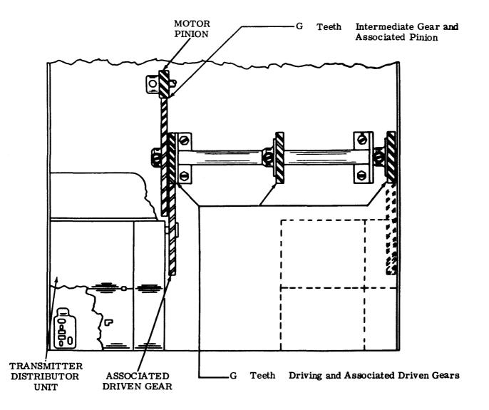
Figure 4-35. Gear Train - Multicontact Multiple Mounting Bases (Common Speed)
