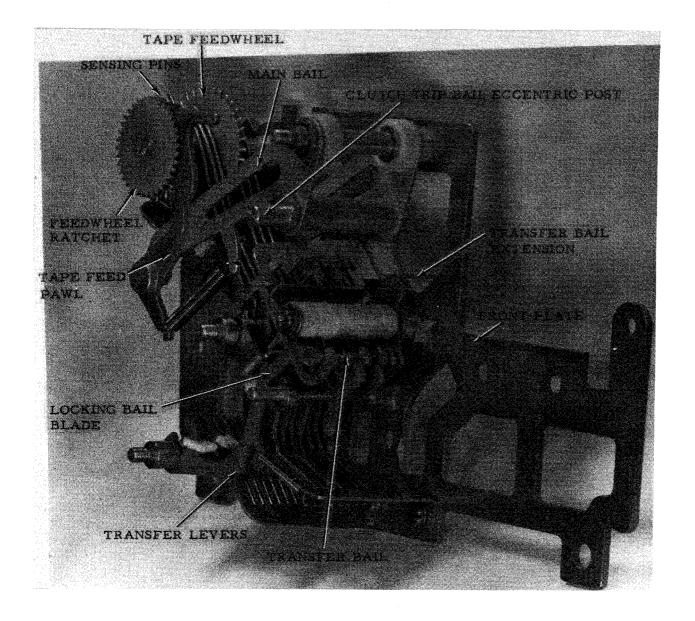
Figure 3-15. Front Plate Assembly - Pear View
