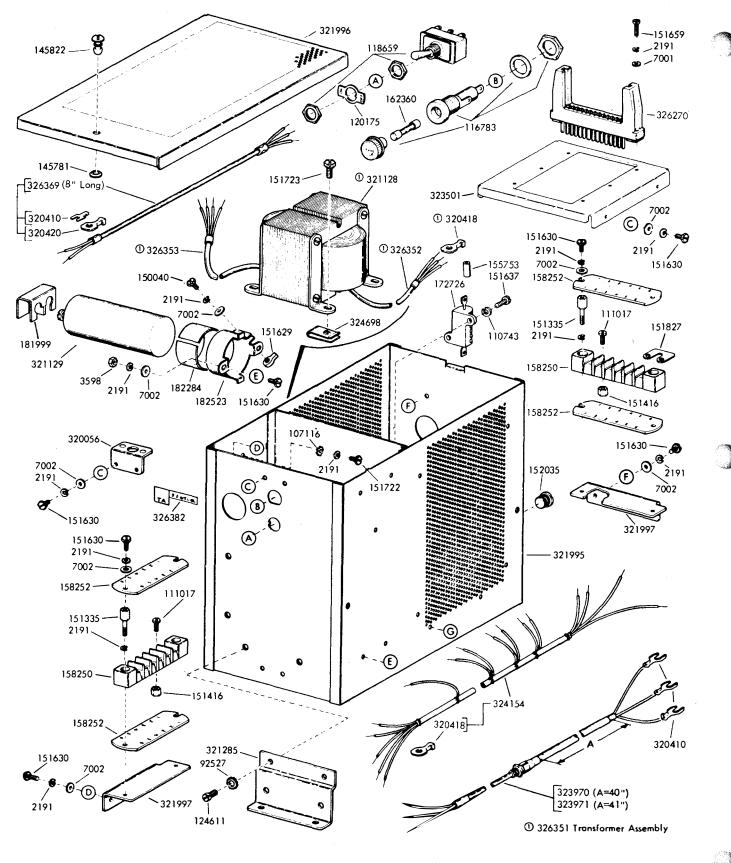
Figure 7-50. Electrical Service Assembly 326792 - Used with Mini TD Set (Sheet 1 of 2)
