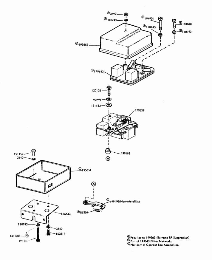
Figure 7-11. Contact Box Assemblies - 198610 (Low-Level Keyer) and 199505 (Extreme RF Suppression)
