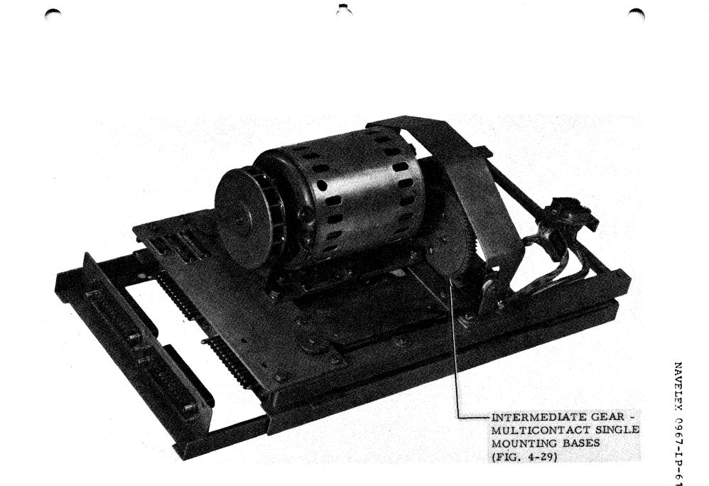
Figure 4-28. Multicontact Single Mounting Bases
