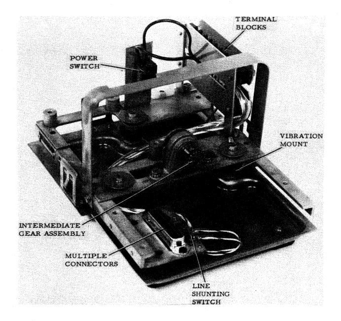
Figure 1-12. Transmitter Distributor Base - Miniaturized
