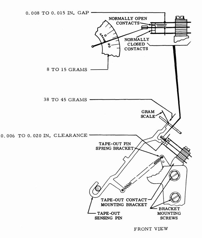
Figure 6-16. Tape-Out Contact Assembly, Tape-Out Sensing Pin Spring, and Tape-Out Contact Bracket
