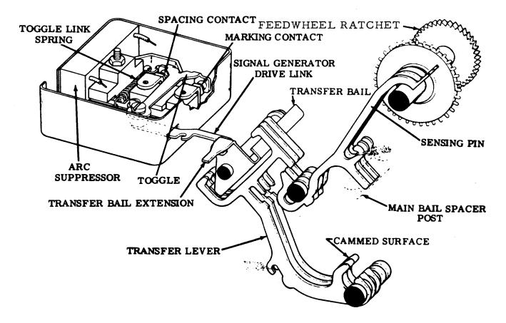
Figure 3-12. Transfer Lever and Signal Generator Mechanisms
