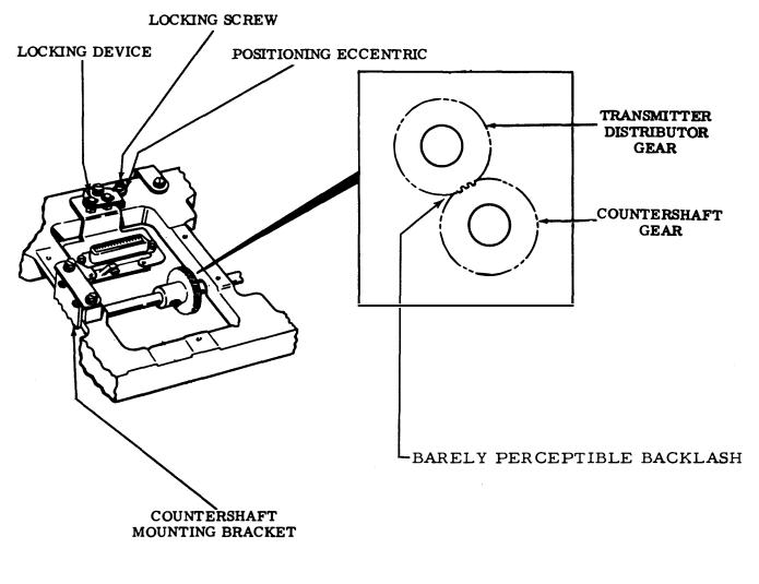
Figure 6-36. Transmitter Distributor Unit Positioning (Common Speed)
