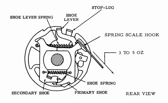
Figure 6-2. Clutch Shoe Spring
