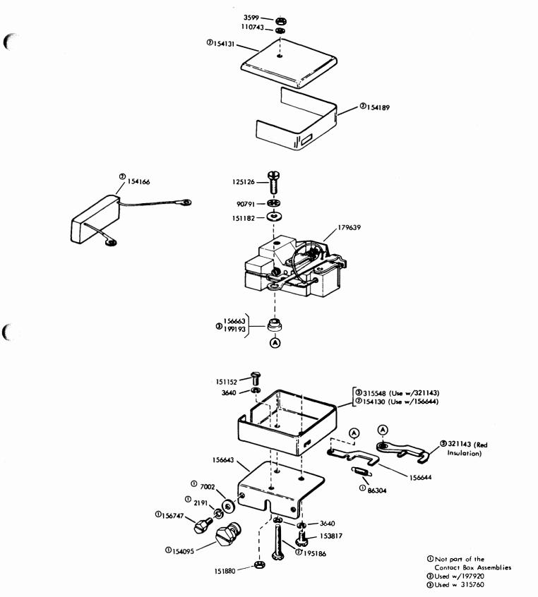
Figure 7-12. Contact Box Assemblies - 192600 (Neutral Transmission), 197920 (Neutral Transmission with Arc Suppression), 305008 (Polar Transmission), and 315760 (Polar Transmission with Insulated Drive)
