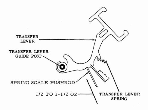
Figure 6-27. Transfer Lever Spring
