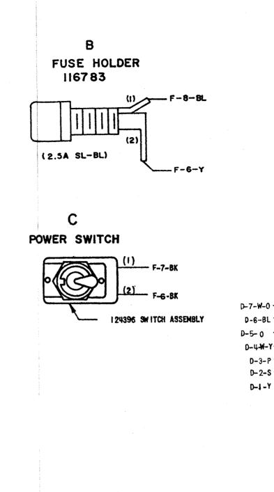
Figure 5-8. Transmitter Distributor Base LXDB19 Wiring Diagram
