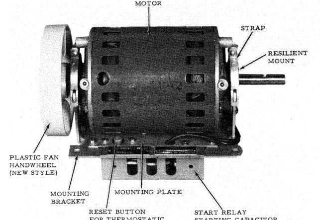
RESET BUTTON FOR THERMOSTATIC CUTOUT SWITCH START RELAY STARTING CAPACITOR THERMOSTATIC CUTOUT SWITCH
