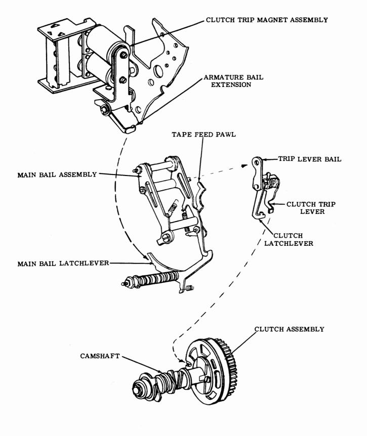
Figure 3-9. Function Control Mechanism
