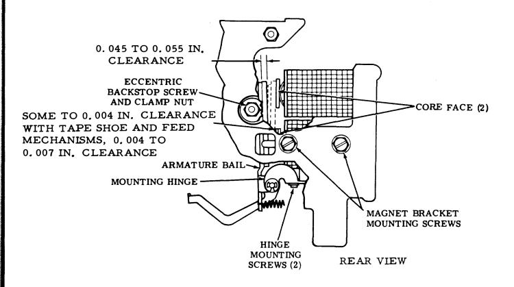
Figure 6-5. Clutch Magnet Assembly (Preliminary) (Core Clearance and Armature Bail Clearance)
