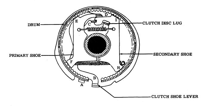
Figure 3-17. Clutch Engaged
