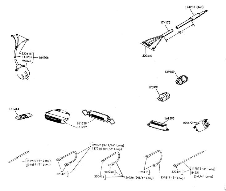
Figure 7-32. Cable Components
