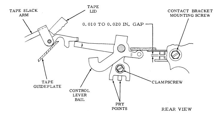
Figure 6-71. Tape Slack Contacts
