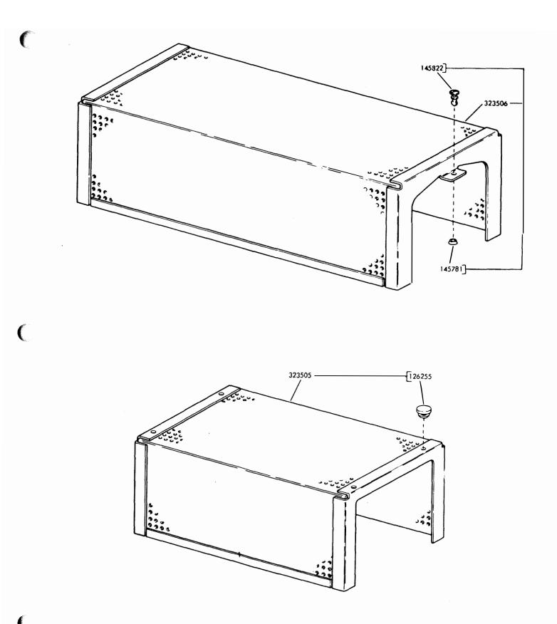
Figure 7-49. Electrical Service Assembly Covers (Sheet 2 of 2)
