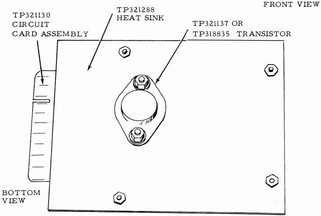
Figure 3-24. Power Supply (0.5 Ampere) TP321290
