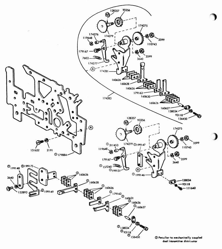
Figure 7-5. Front Plate Mechanism (With Tape Feed Assurance Contact)
