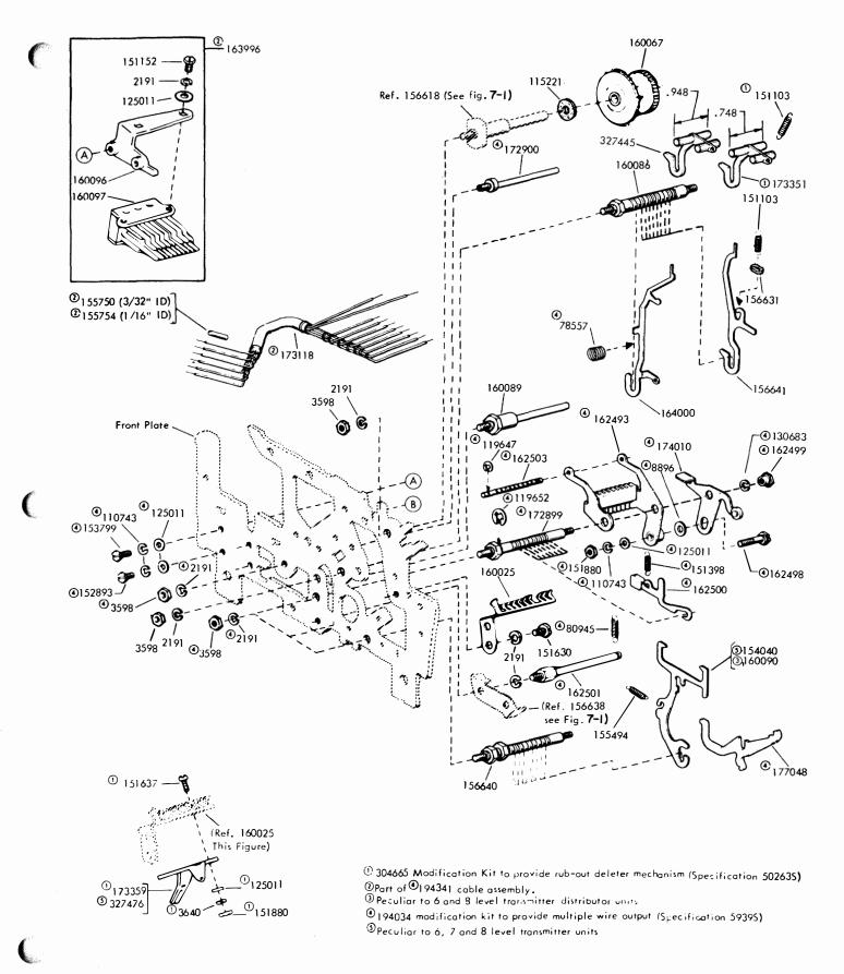
Figure 7-4. Front Plate Mechanism (6, 7, and 8 Level Units)
