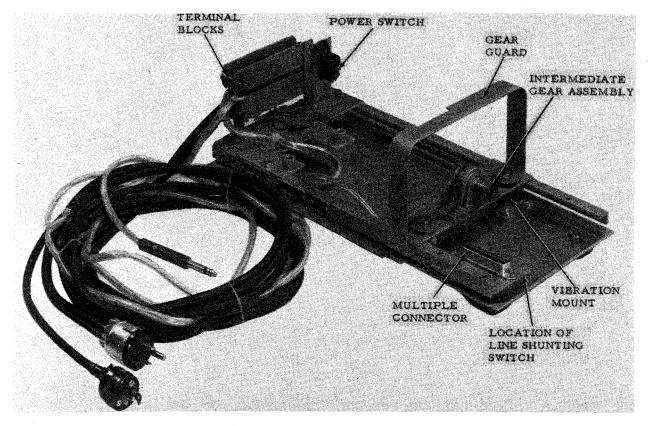
Figure 1-8. Transmitter Distributor Base - Single Contact, Single Mounting
