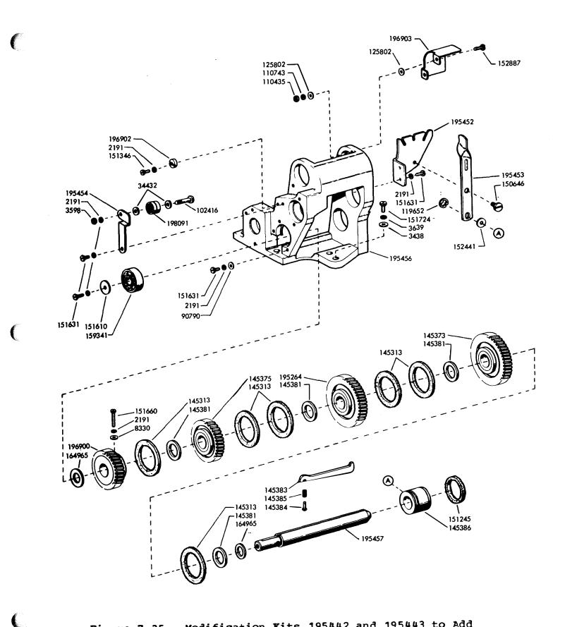
Figure 7-35. Modification Kits 195442 and 195443 to Add Three-Speed Gearshift Assemblies (Sheet 2 of 3)
