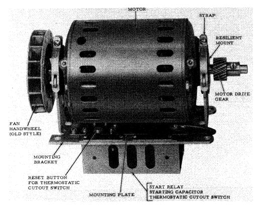
Figure 1-18. Typical Standard or Heavy Duty Synchronouss Motor Unit
