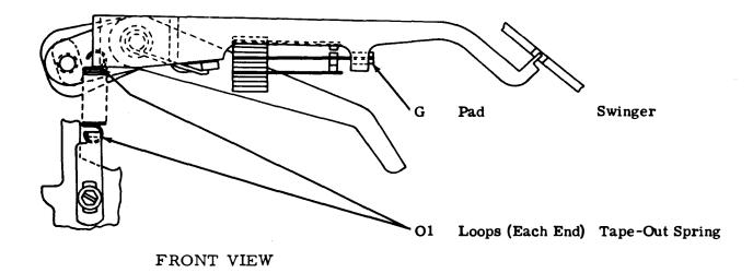
Figure 4-17. Tape-Out Sensing Mechanism (Variable Features)
