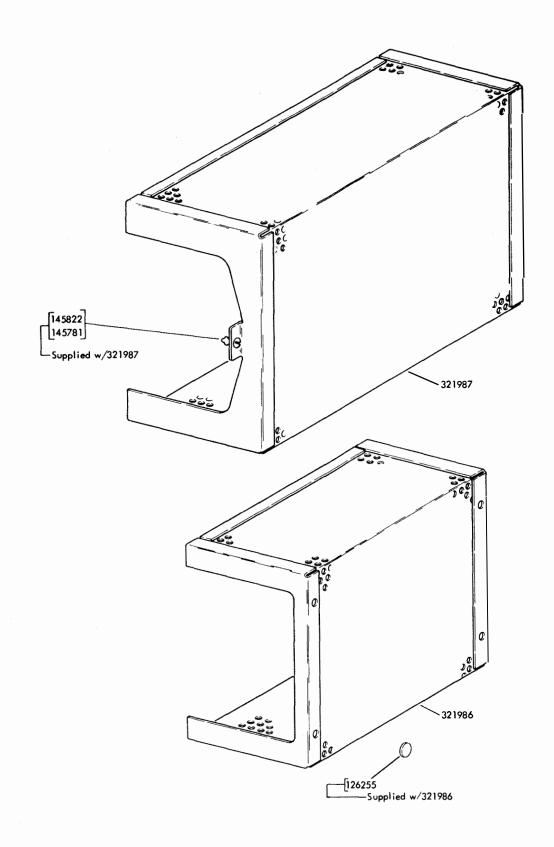
Figure 7-48. Electrical Service Assembly Covers (Sheet 1 of 2)
