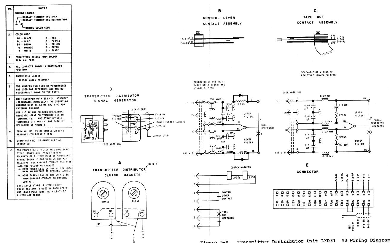
Figure 5-4. Transmitter Distributor Unit LXD31 43 Wiring Diagram
