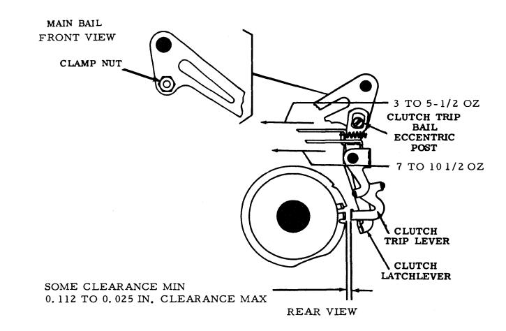
Figure 6-4. Clutch Trip Lever, Clutch Trip Lever Spring, and Clutch Latchlever Spring
