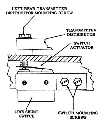
Figure 6-42. Line Shunt Switch TP172847
