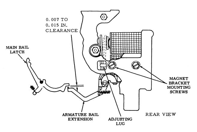
Figure 6-6. Clutch Magnet Assembly (Preliminary) (Main Bail Clearance)
