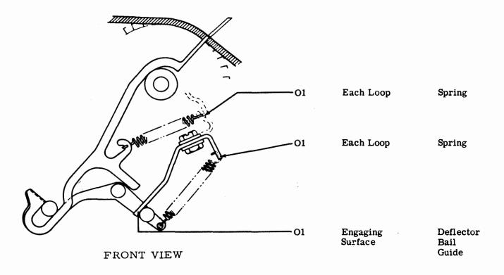
Figure 4-22. Rub-Out Deleter (Variable Features)
