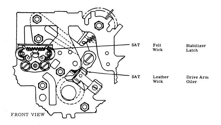
Figure 4-13. Front Plate Assembly
