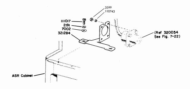
Figure 7-23. Mounting Components for Contact Box Cable - RFI Suppression Features for Low-Level Sets
