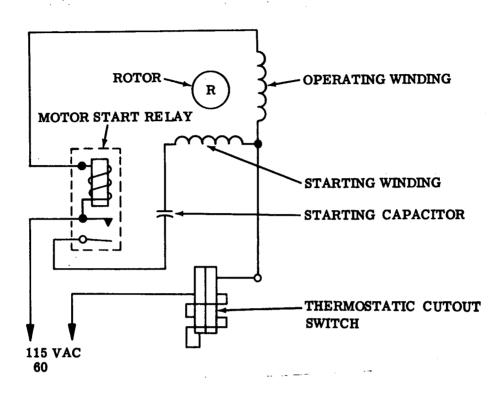
The stator of the motor has two windings: a starting winding and an operating (or run) winding. The starting winding, starting capacitor, and the normally-open contacts of the starting relay are connected in series. The coil of the starting relay is connected in series with the operating winding.
