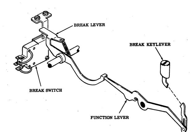
depressing BREAK KEY LEVER pivots FUNCTION LEVER pivots BREAK LEVER operates BREAK SWITCH opens SIGNAL LINE circuit
