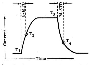
If the S-MTD is equal to the M-STD, the pulse as seen by the selector would be undistorted.
