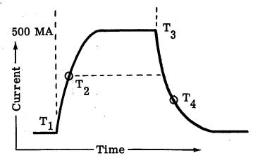
When, at the end of the transmitted pulse, the current again starts towards  $\mathcal{O}$  ma, the selector armature should, theoretically, fall away at T3. The trailing edge of the impulse, however, also slopes, consequently, a definite time will have elapsed before the armature will drop away (T4). Notice that T2 and T4 are not identical current values. The de-energization point will be of lower value due to residual magnetism in the coils.
