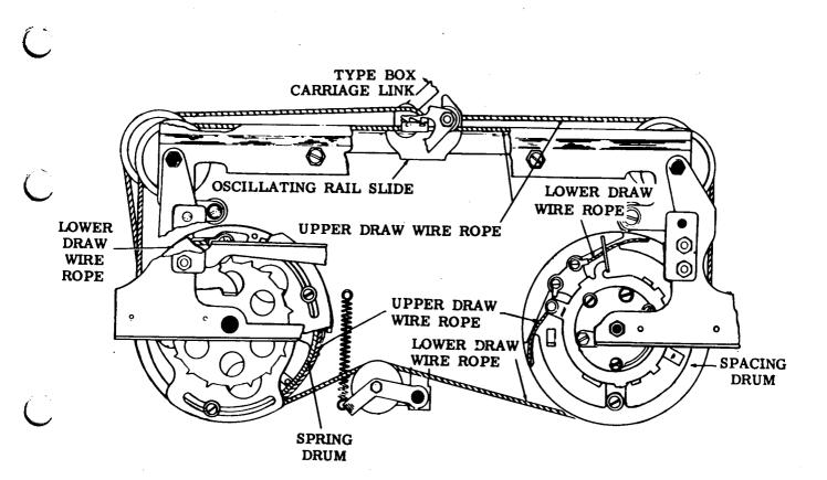
UPPER DRAW WIRE ROPE connected to SPACING DRUM and SPRING DRUM TYPE BOX CARRIAGE LINK and OSCILLATING RAIL SLIDE clamped to UPPER DRAW WIRE ROPE, LOWER DRAW WIRE ROPE, SPACING DRUM and
