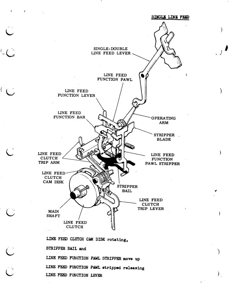
LINE FEED CLUTCH stops after one third of a revolution
