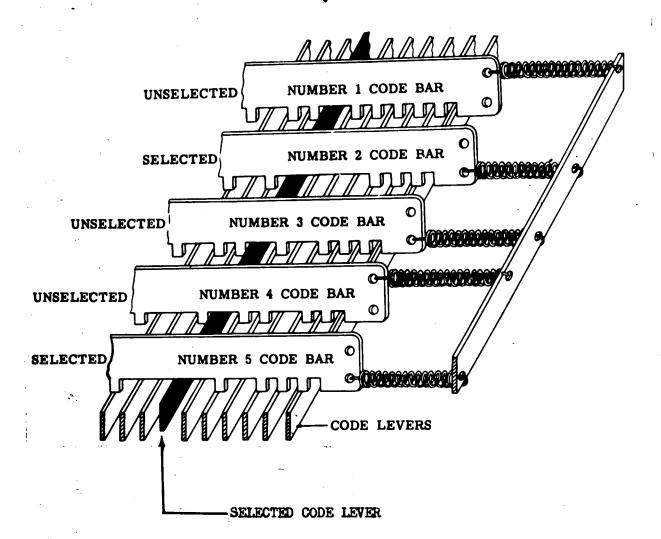
CODE BAR BAIL releases, CODE LEVER pivots SELECTED CODE BARS move (right) UNSELECTED CODE BARS blocked by CODE LEVER and TINES of code bars.
