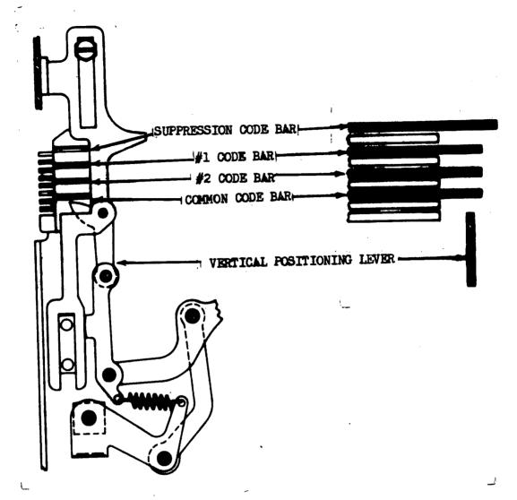
VERTICAL POSITIONING LEVER moves up until blocked by a projecting CODE BAR in a spacing (right) condition
