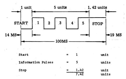
The 7.42 unit character is known as the Standard Unit Code for five-level transmission. One exception to this standard is a straight 7 unit code. An example of this is Western Union, which uses a stop pulse the same length as the start and information pulses. This unit code plus a variance in shaft speed allows for 65 wpm operation. We will discuss this a little later in this guide.
