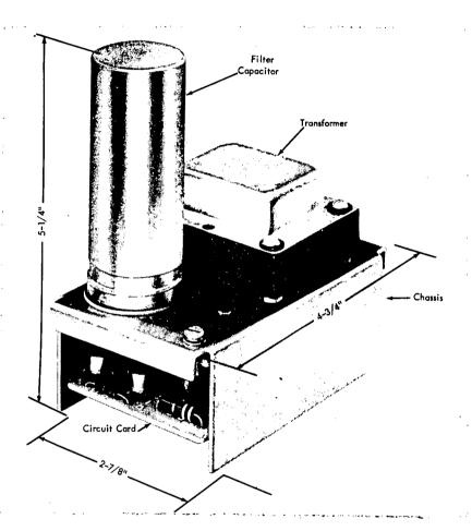
The SELECTOR MAGNET DRIVER assembly consists of a chassis mounted power supply and an etched circuit card. The power supply provides operating voltages for the various components, including five transistors, mounted on the circuit card.
