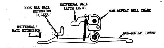
UNIVERSAL BAIL rocked to rear UNIVERSAL BAIL LATCH LEVER drops CODE BAR BAIL EXTENSION with ROLLER moves right NON-REPEAT LEVER moves up
