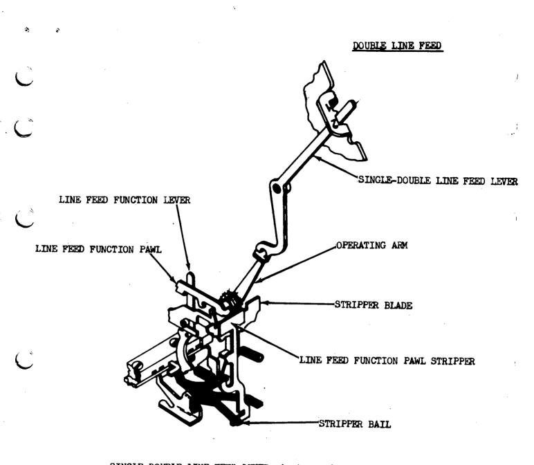
SINGLE-DOUBLE LINE FEED LEVER pivots moving OPERATING ARM moves STRIPPER BAIL out of LINE FEED FUNCTION PAWL STRIPPER STRIPPER BLADE lifts LINE FEED FUNCTION PAWL STRIPPER releasing LINE FEED FUNCTION PAWL and
