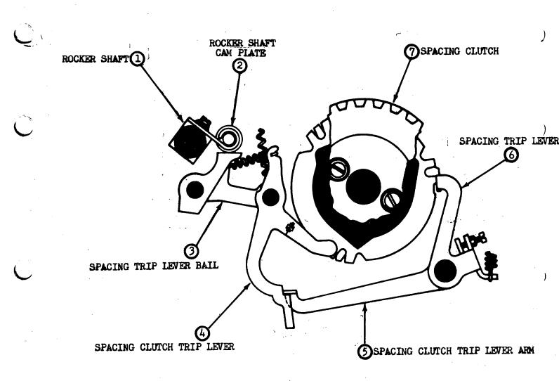
1. ROCKER SHAFT and 2. ROCKER SHAFT CAM PLATE pivot, driving SPACING TRIP LEVER BAIL and SPACING TRIP LEVER down, latching SPACING CLUTCH TRIP LEVER ARM
