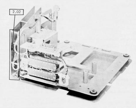
2.02 Low-Tape Alarm Switch Mechanism (Right-side View)
