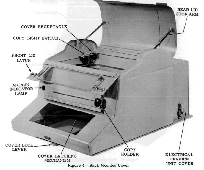
2.11 All external signal and power connections are made through terminal boards in the electrical service unit. A receptacle is provided in the cover for connection with the electrical service unit.
