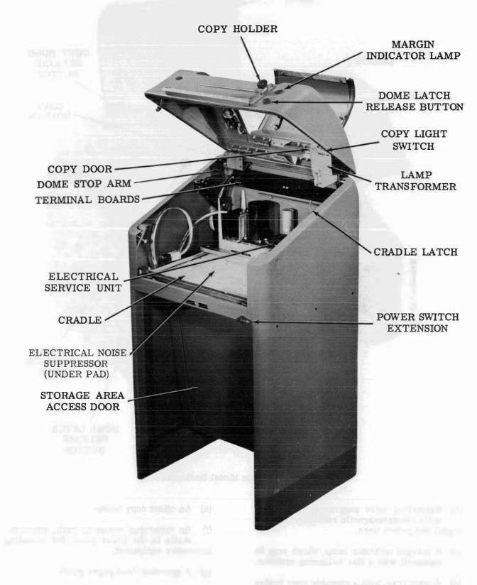
Figure 2 - Floor Model Enclosure (with Electrical Service Unit)
