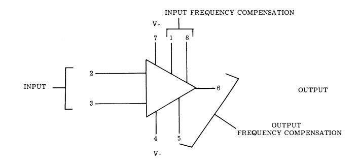
Figure 22 - Operational Amplifier (Op Amp)
