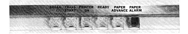
Figure 5 - Operator Controls (At Front of Cover)
