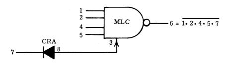
NAND Gate With Diode to Provide Additional Input
