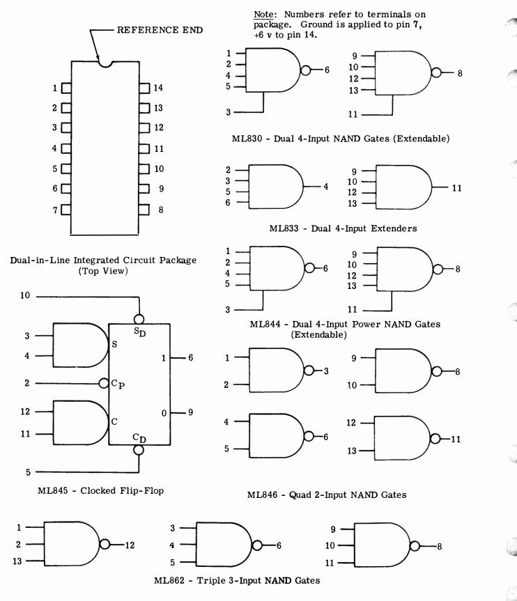
Figure 23 - Package and Configurations for Digital Integrated Circuits
