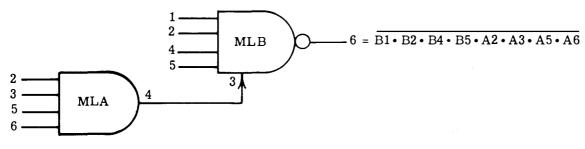
NAND Gate With Extender to Provide Four Additional Inputs
