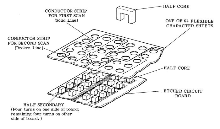
Figure 9 - Core Arrangement and Conductor Routing on Character Sheets
