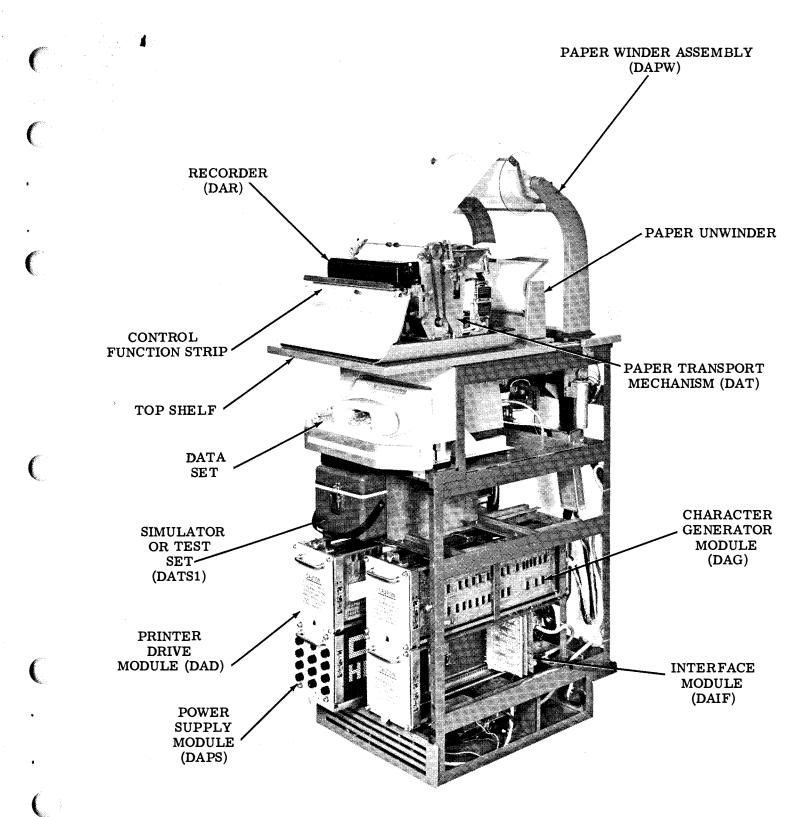
Figure 3 - DATASPEED Printer With Cabinet Panels and Cover Removed and Top Shelf and Modules Extended connected to an external data set in a DATA-SPEED sender or receiver. The data set is not furnished with the printer in either case. Sets used with a serial interface operate at 1050 or 1200 wpm, and those with a parallel interface operate at 750 wpm.
