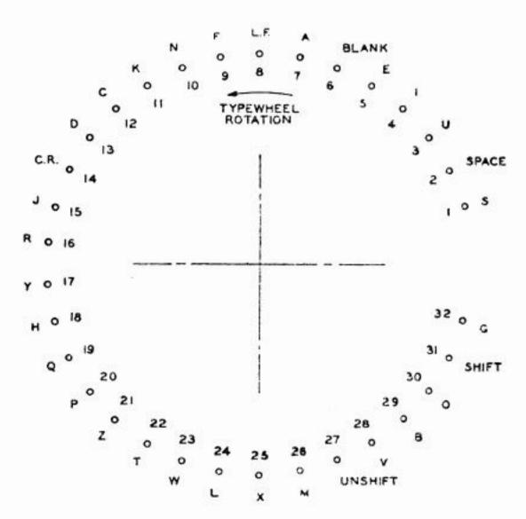
NOTE THE ABOVE ALSO REPRESENTS THE ARRANGEMENT OF CHARACTERS WHEN LOOKING AT THE UNDERSIDE OF THE TYPEWHEEL.
