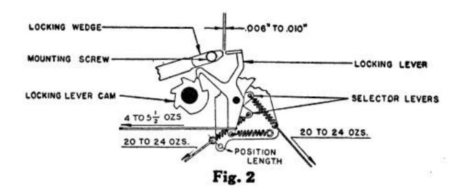
4.07 Locking lever spring shall have a tension of Min. 4 ozs. (115 gms.), Max. 5-1/2 ozs. (155 gms.) measured as in Fig. 2 when lever starts to move from high part of cam.
