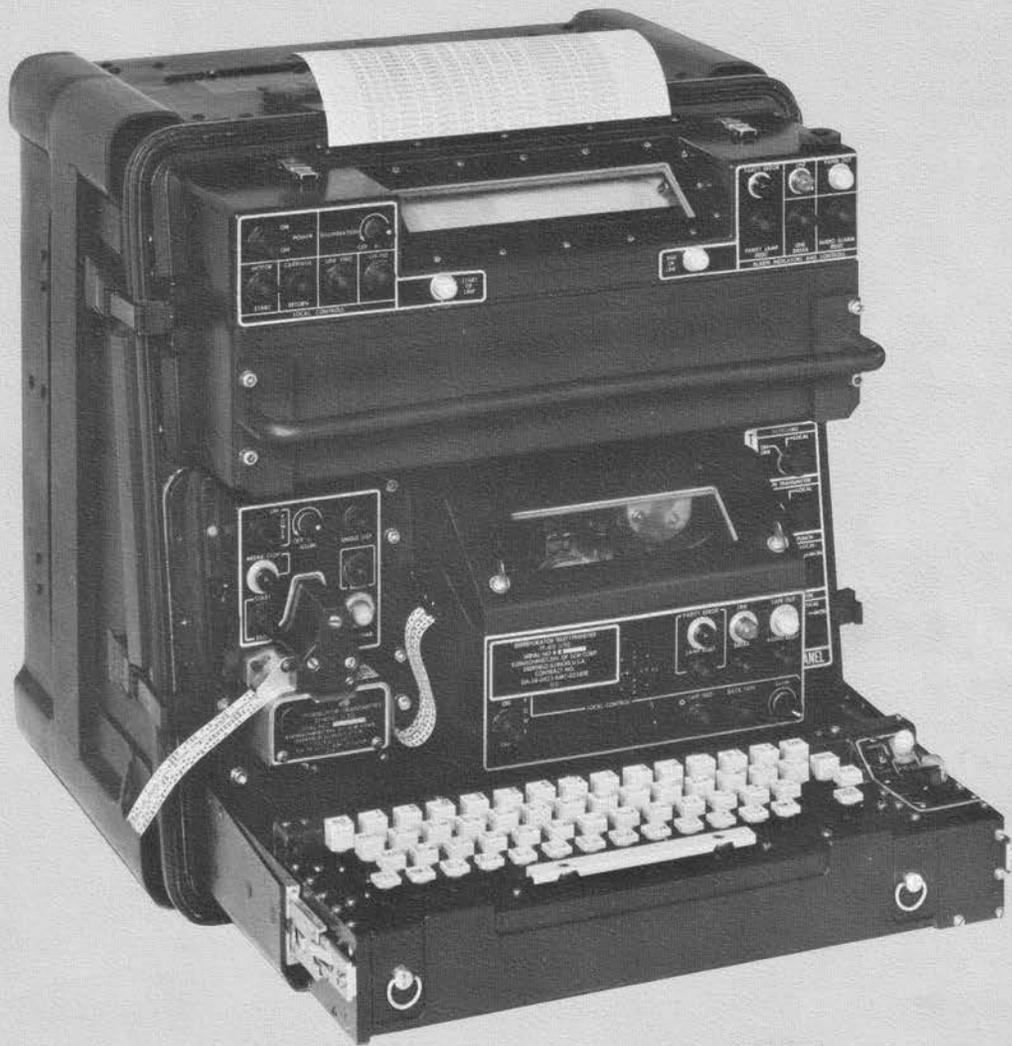
This is an automatic send-receive set, comprising a keyboard transmitter, tape transmitter, typing reperforator and page printer. It includes transmit battery and electrical interface. The set can be used on and off line to prepare or edit tapes, to transmit from either tape or keyboard and to receive on page copy and/or paper tape. In a full duplex system, the distributor transmitter takes precedence over the keyboard, inhibiting keyboard opera-
