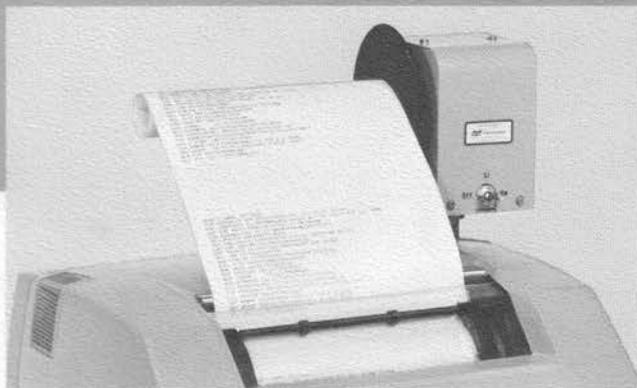
Reeling Machine RL-236/UG is a self-contained paper winder, designed for unattended and continuous operation in conjunction with a teletypewriter page printer. Its compact size and light weight makes it suitable for installation on the page printer dust cover. In operation, the reeling machine maintains a slight, yet steady tension on the printed copy issuing from the page printer as shown.
