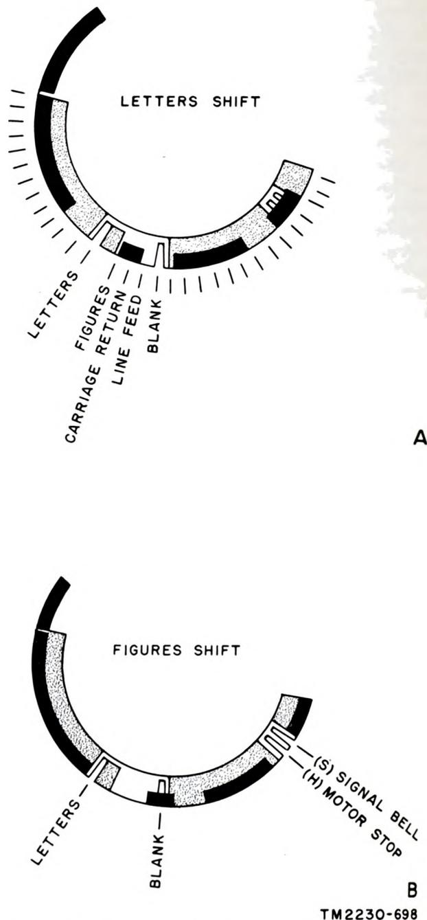
Figure 54. Location of function selecting arm positions, showing aperture gate in blocked and unblocked positions.
