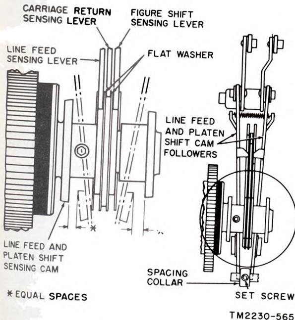
Figure 160. Cam followers and spacing collar adjustment.
