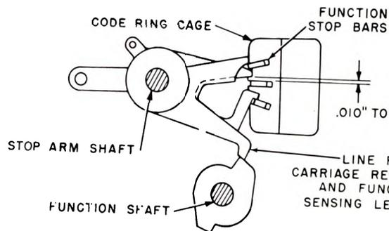
Figure 161. Code ring cage adjustment.
