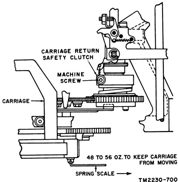
Figure 223. Carriage return safety friction clutch adjustment.
