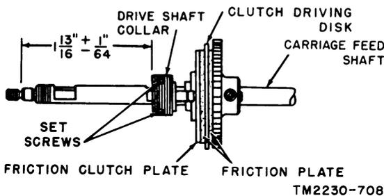
Figure 220. Carriage feed shaft drive shaft collar adjustment.
