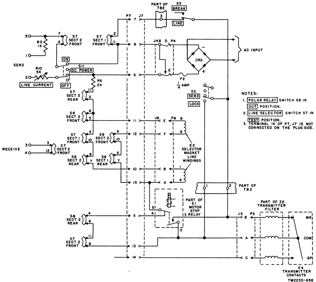
Figure 78. Test circuit without relay, simplified schematic.
