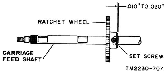
Figure 219. Carriage feed shaft ratchet wheel adjustment.
