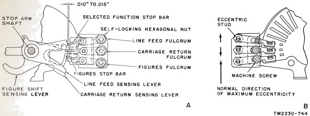
Figure 170. Stop bar adjustable fulcrum adjustment.
