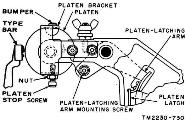
Figure 214. Letters shift position adjustment.
