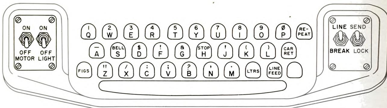
Figure 17. Standard communications keyboard.
