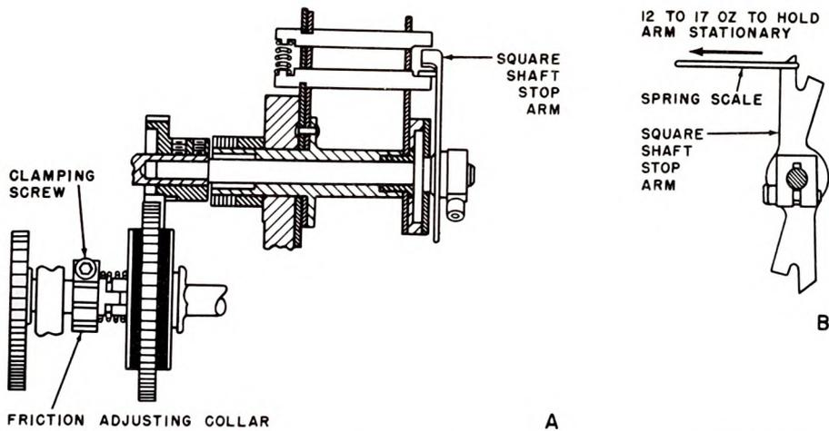
Figure 184. Square shaft stop arm torque adjustments.
