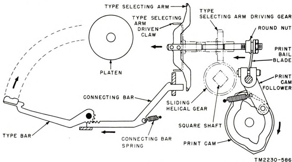
Figure 50. Cross section of teleprinter, showing operation of printing mechanism.
