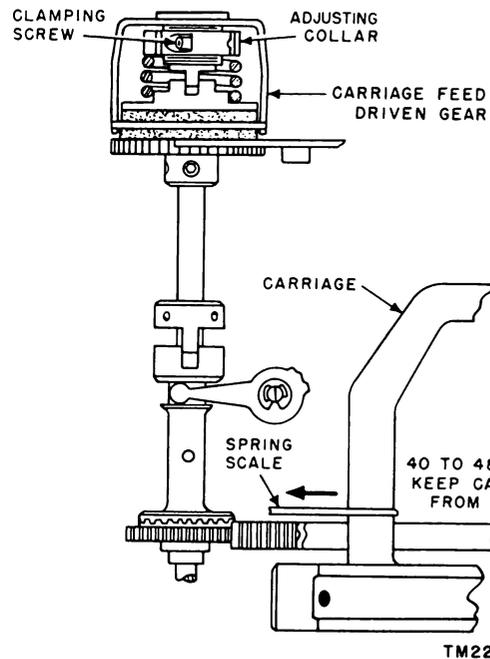
Figure 222. Carriage feed friction clutch adjustment.
