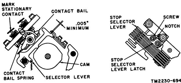
Figure 238. Stop selector lever latch and transmitter contact adjustment.
