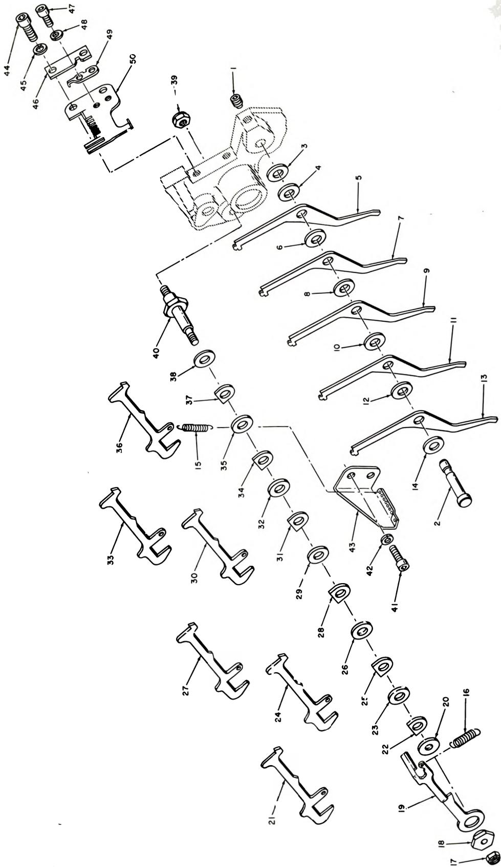
Figure 102. Keyboard-transmitter sensing and selector levers, exploded view.
