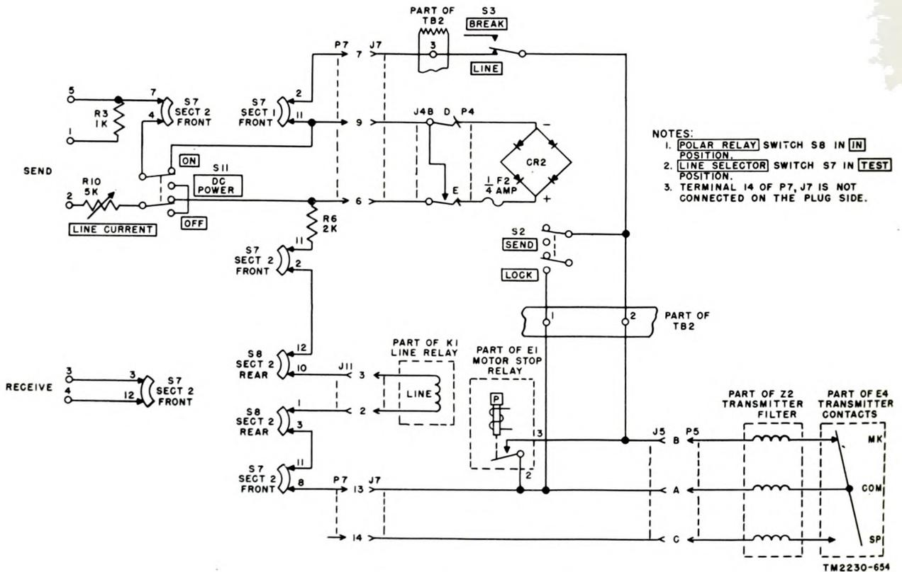
Figure 79. Test circuit with line relay, simplified schematic.
