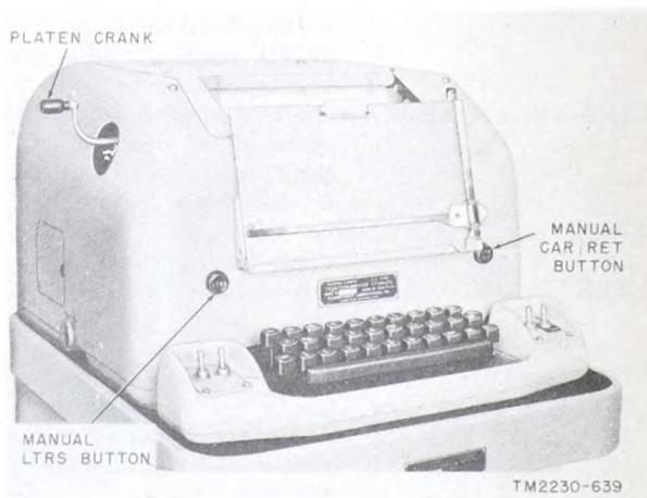
Figure 19. Teleprinter controls.
