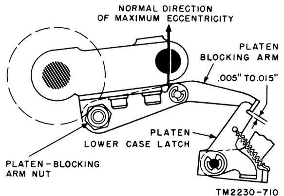
Figure 216. Platen blocking arm adjustment.
