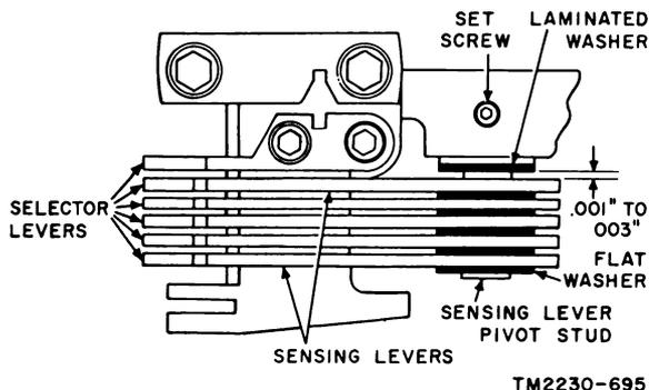
Figure 236. Sensing levers clearance alinement adjustment.
