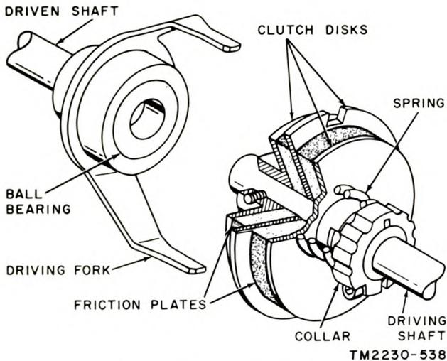
Figure 33. Friction clutch.
