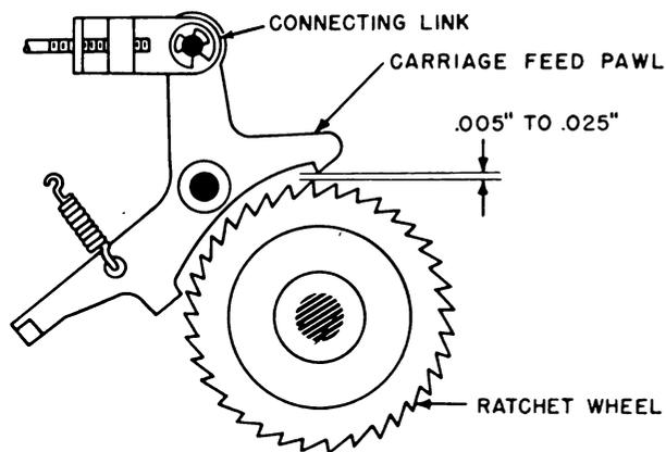
Figure 202. Carriage feed pawl adjustment.
