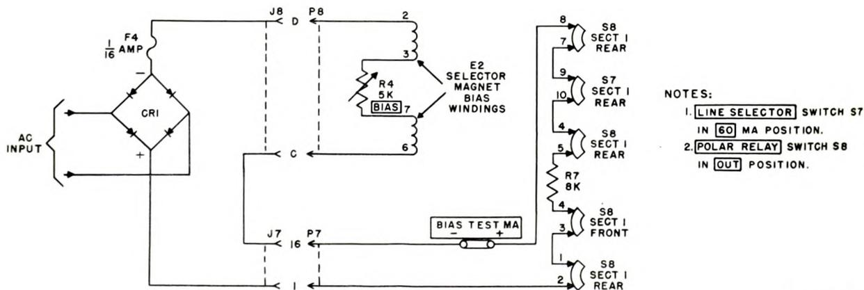
Figure 81. Selector magnet bias (60-ma) circuit, without relay, simplified schematic.
