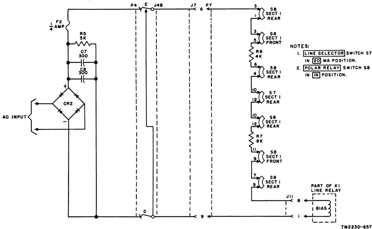
Figure 82. Line relay bias (20-ma) circuit, simplified schematic.
