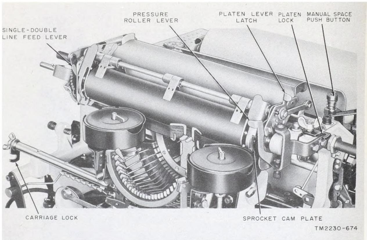
Figure 14. Teleprinter, dust cover removed, showing platen and carriage locks.
