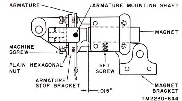
Figure 172. Armature stop bracket and bar magnet preliminary clearance.
