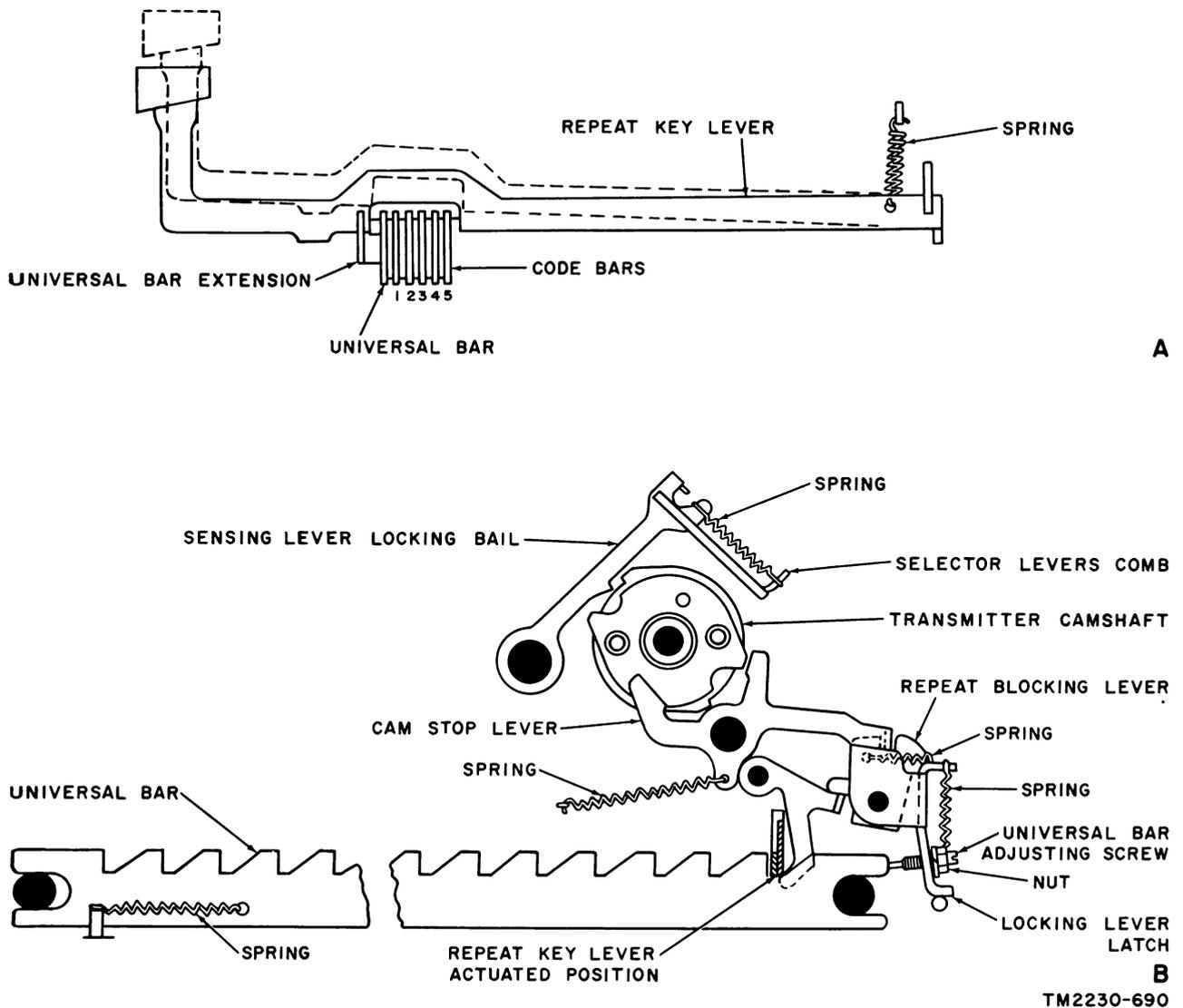
Figure 35. Transmitter camshaft control mechanism.
