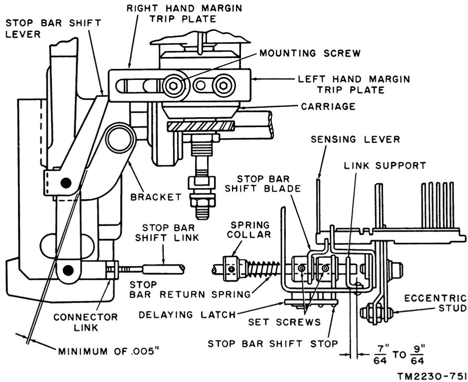
Figure 229. Automatic carriage return, shift link adjustment.
