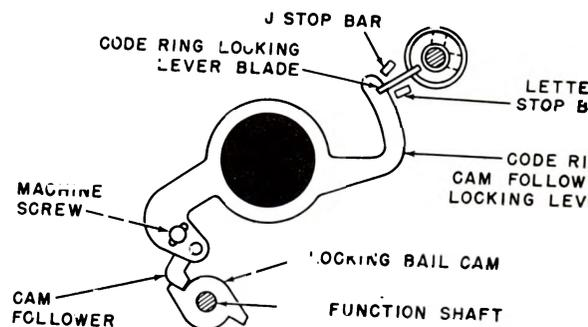
Figure 162. Code ring locking bail cam follower adjustment.
