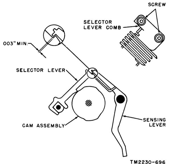
Figure 237. Selector levers and sensing levers adjustment.
