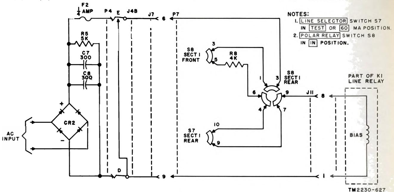
Figure 83. Line relay bias (60-ma) circuit, simplified schematic.
