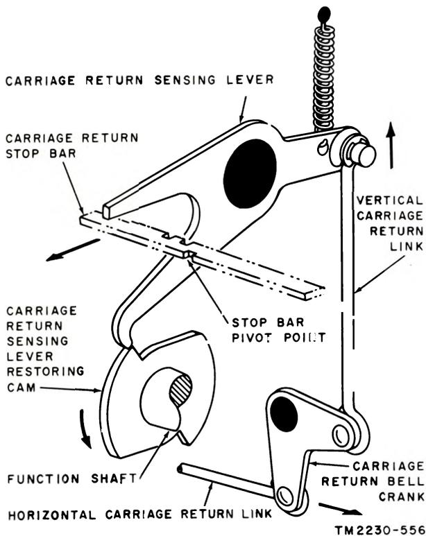
Figure 59. Carriage return operating mechanism as seen from the rear of the teleprinter.
