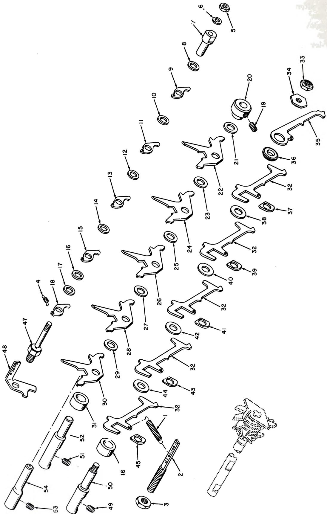
Figure 121. Selector levers and Y-levers, exploded view.
