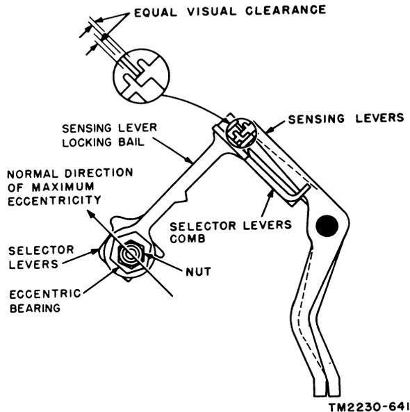
Figure 239. Sensing lever locking bail adjustment.
