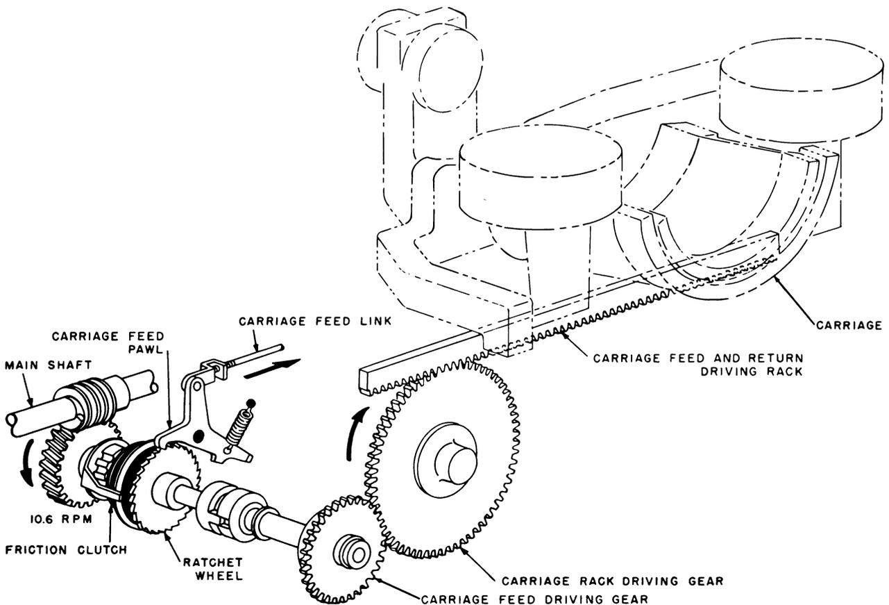
Figure 55. Carriage feed mechanism.
