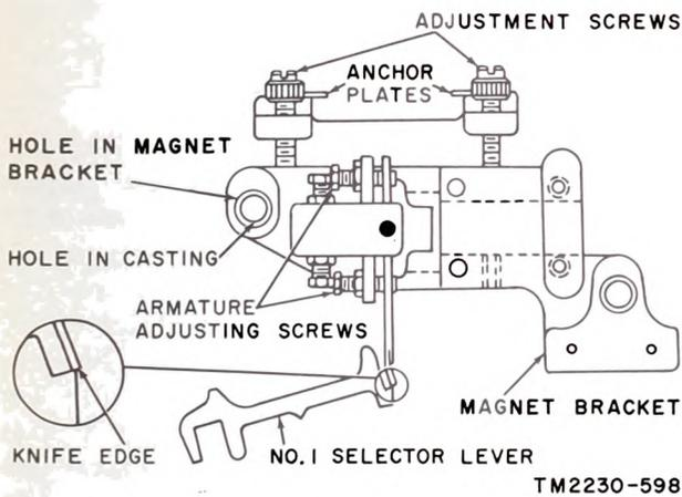
Figure 171. Armature and selector magnet bracket alignment.
