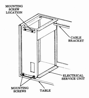
Figure 24 - ESU Mounted in Table
