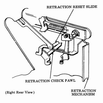
Figure 7 - Retraction Slide and Check Pawl
