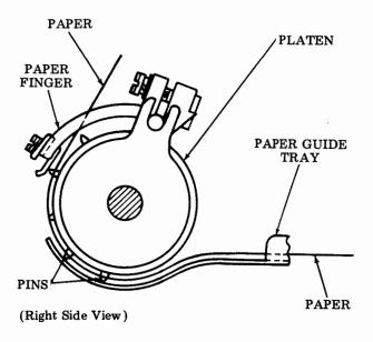
Figure 17 - Paper Routing Assembly — Sprocket Feed
