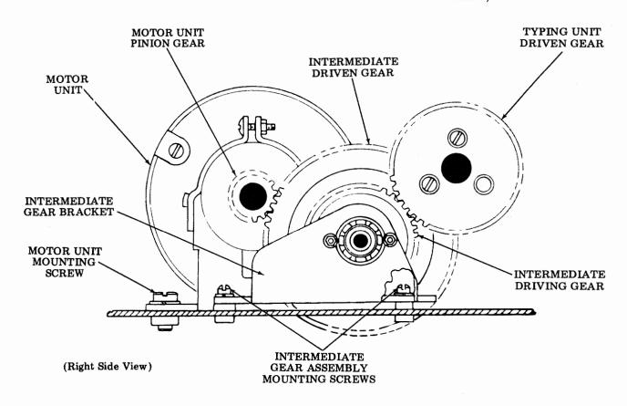
Figure 12 - Intermediate Gear Assembly
