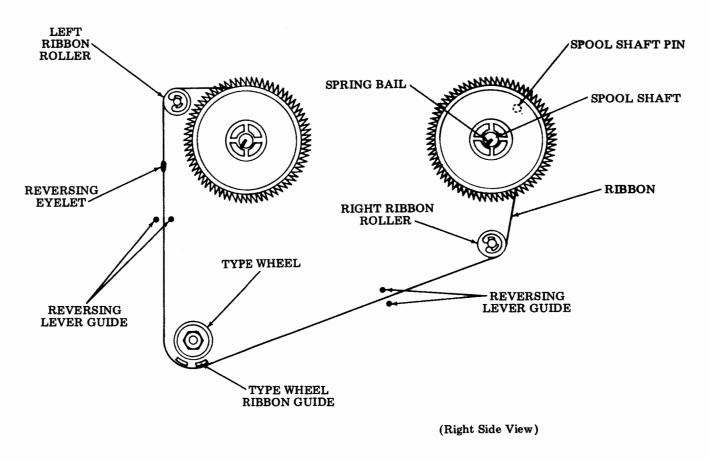
Figure 21 - Reperforator Ribbon Routing
