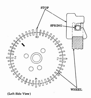
Figure 18 - Form-Out Positioning
