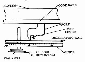
Figure 6 - Codebar Fork and Clutch Trip Lever Alignment
