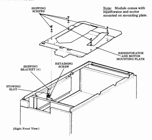
Figure 9 - Disabling Shipping Brackets — RT Module
