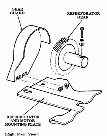
Figure 19 - Gear and Gear Guard Installation
