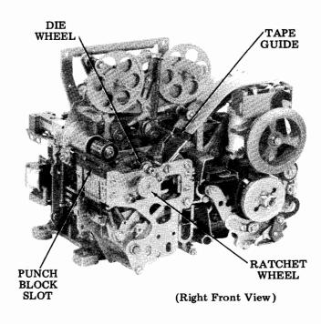
Figure 22 - 37 Typing Reperforator
