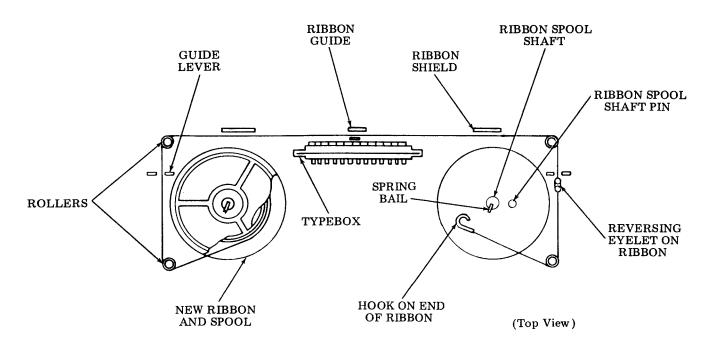
Figure 14 - Ribbon Routing
