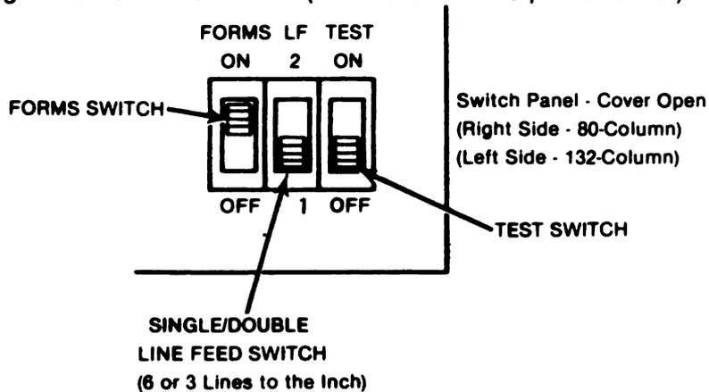
(a) **FORMS switch On** - Enables the printer to form feed on receipt of FF and stop at the start of the next form. Characters will not print during the on-line form feed operation.
