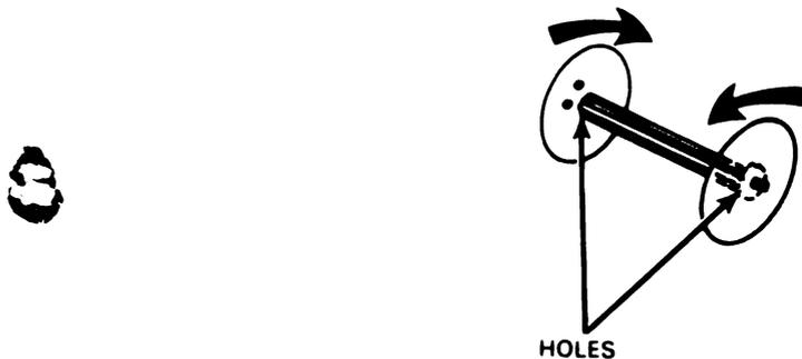
(8) To reassemble, line up pins in holes (both ends), press together and twist clockwise to secure.
