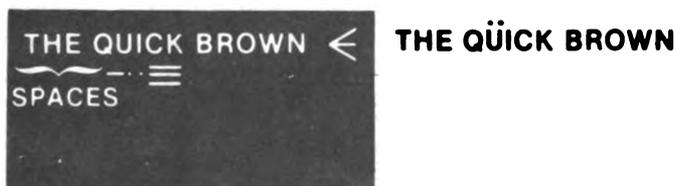
(6) To underline and accent characters at the same time: End first line of data with CARRIAGE RETURN ( ← ). Prepare a third line with accent character(s) beneath characters to be accented and terminate this line with NEW LINE ( ≡ ). Printer will copy as shown below.
