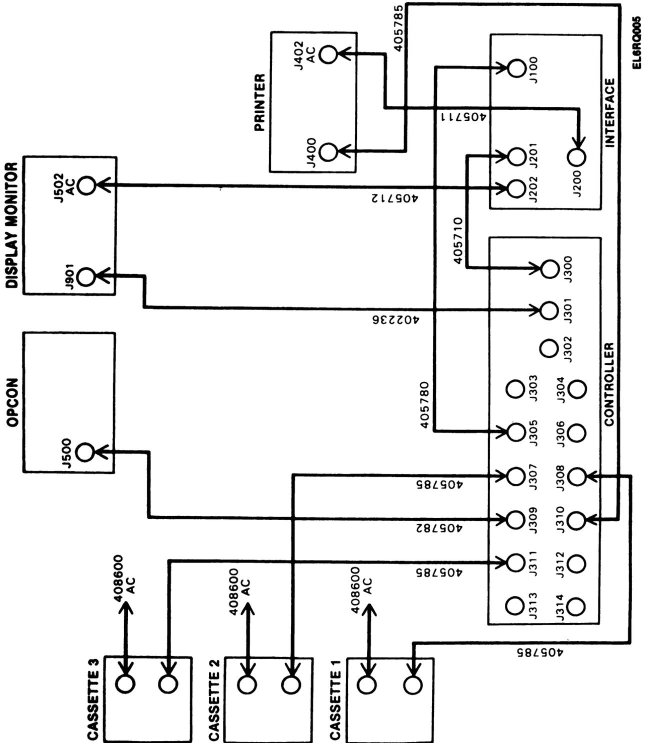
Figure 2-2. Cabling for KD, KP, KDP, KDPM Configurations
