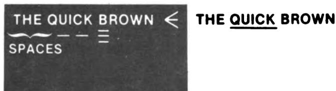
(5) To accent characters: Follow same procedure as for underscoring. End first line of data with CARRIAGE RETURN ( ← ). On next line insert the accent marks below the character to be accented. Terminate this line with NEW LINE ( ≡ ). Printer will copy as shown below.
