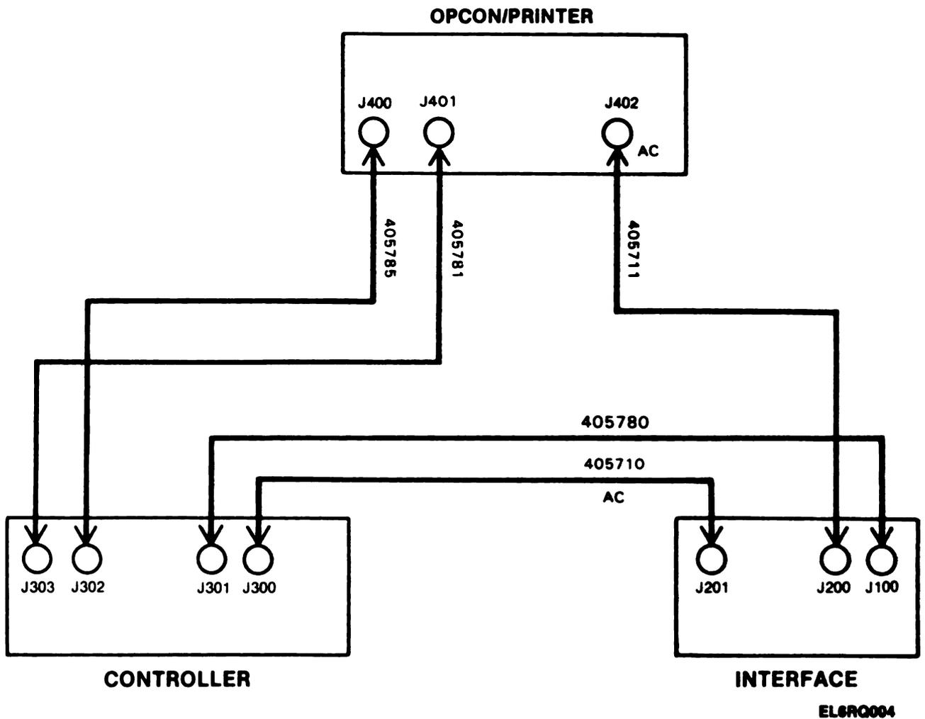
Figure 2-1. Cabling for ROP Configuration
