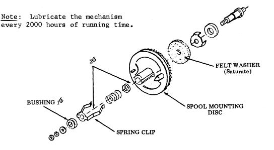
4.03 Saturate each ribbon feed felt washer with oil. The oil may be applied to felt washer through the hole in each spool mounting disc and through the two rectangular holes next to each spindle.
