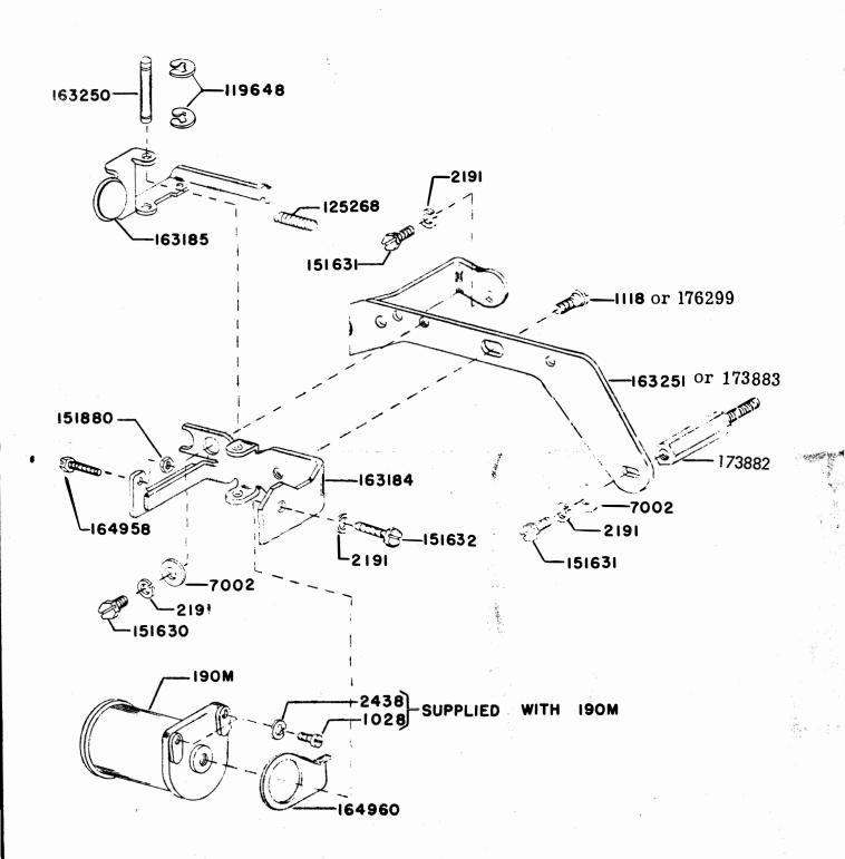
163183 MODIFICATION KIT TO EQUIP A TYPING UNIT WITH D.C. MAGNET OPERATED PRINT SUPPRESSION
