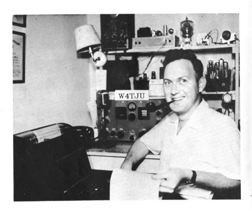
The rig is an 813, 225 watts with 811 modulators fone and the VFO is right behind me in the picture. The receiver is a surplus Super Pro (and a good one) and the chassis on the upper deck by the scope is the RTTY TU. I use the scope for tuning in the conventional way and also on the upper right hand corner of the chassis you can see a 6AL7GT staring at you which also makes
