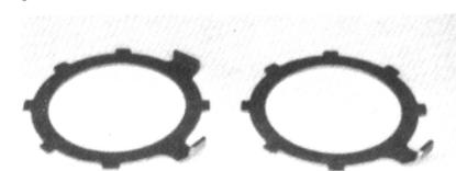
Figure 17...Showing the rear ring needed on the spacing drum for auto CR-LF. The new 154626 is on the left, the old 154625 on the right. Note the new one has an extra tab, which engages the bellcrank to move the "Zero" code bar.
