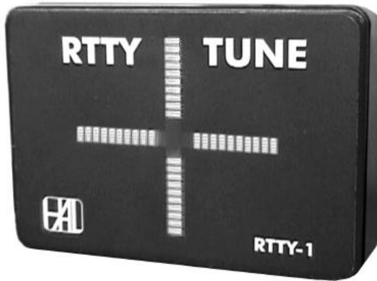
The HAL **RTTY-1** is an easy to use and very accurate tuning indicator. It may be used with virtually *any* FSK modem, TNC, multi-mode controller, demodulator, and receiver or transceiver. The crossed LED bars show correct tuning for all popular FSK modes including Baudot Teletype (RTTY), ASCII Teletype, AMTOR, SITOR, P-Mode\*, and even HF Packet Radio. Just hook it to your receiver's audio output and you're in business, even with modems that do not include "scope" output connectors.
