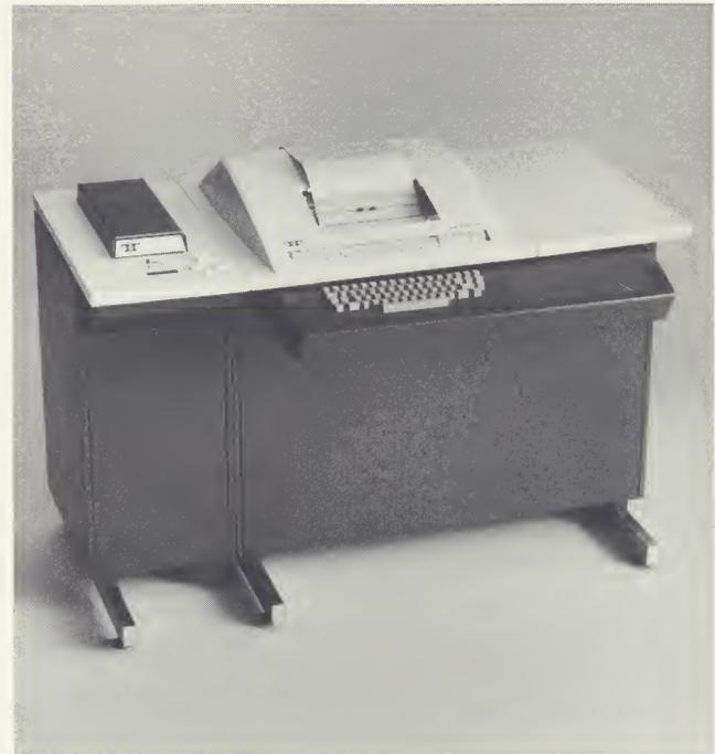
Adds "ASR" versatility to the Inktronic terminal at speeds up to 1200 wpm.
