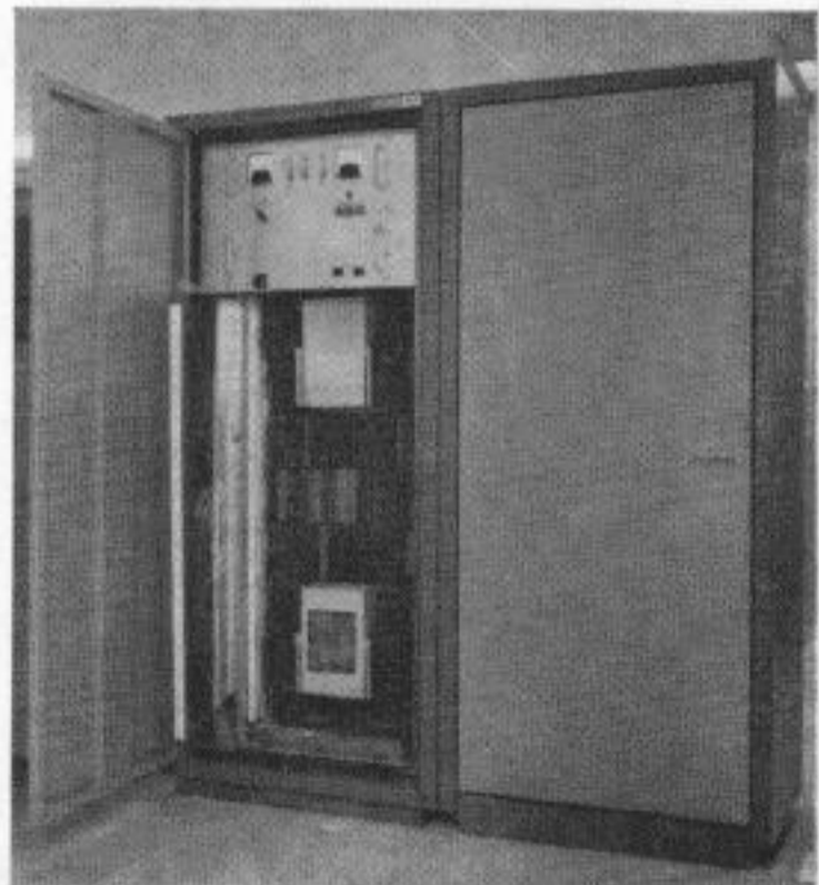
Figure 5a. Memory Bank showing Core Storage Unit at Bottom—(an enlarged view of the core storage unit is shown on the opposite page)
