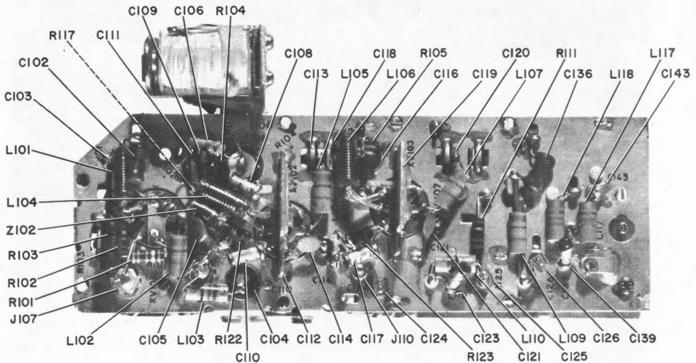
Figure 5-26. RF and PA Amplifier Assembly, Bottom View
