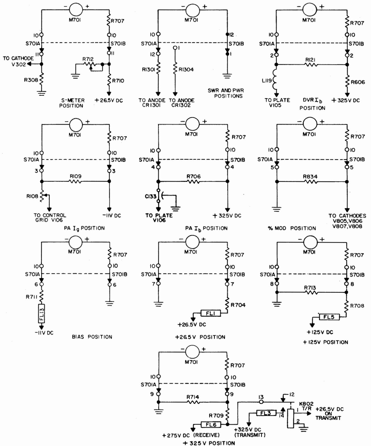
Figure 3-10. Metering Circuits, Simplified Schematic Diagram
