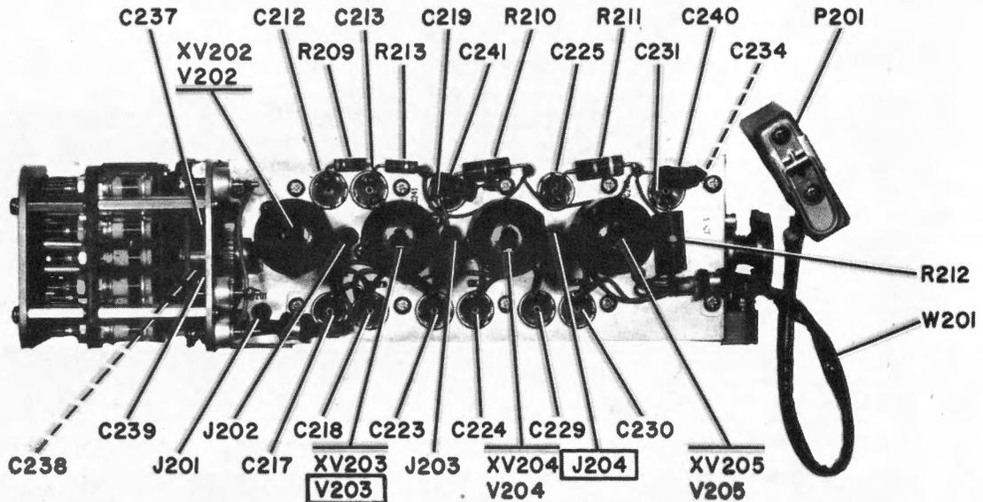
Figure 5-33. Frequency Multiplier-Oscillator, Disassembly Points (B)
