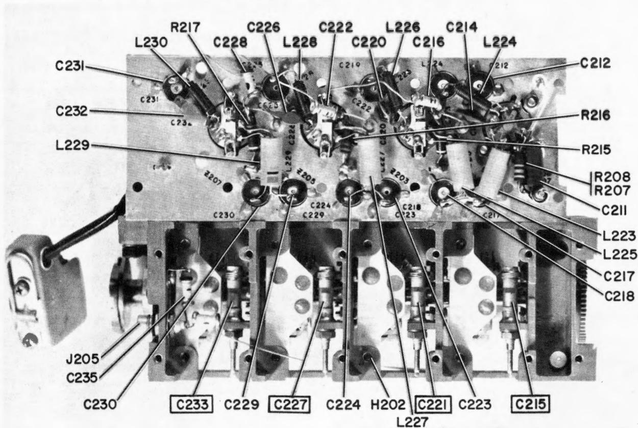
Figure 5-36. Frequency Multiplier-Oscillator, Chassis, Bottom View
