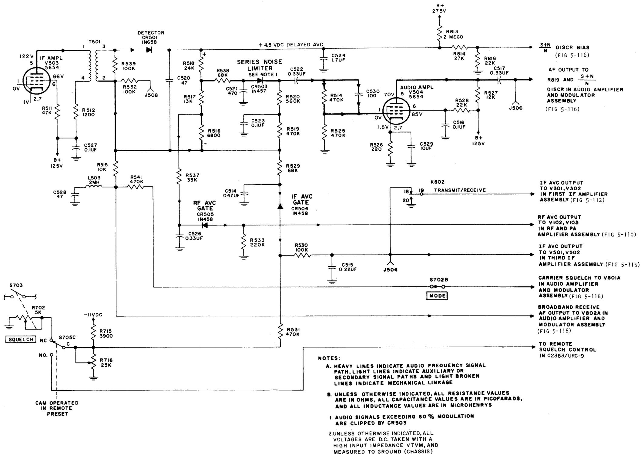
Figure 3-8. Radio Set AN/URC-9( ), Detector, Noise Limiter, and AVC Circuits, Simplified Schematic Diagram
