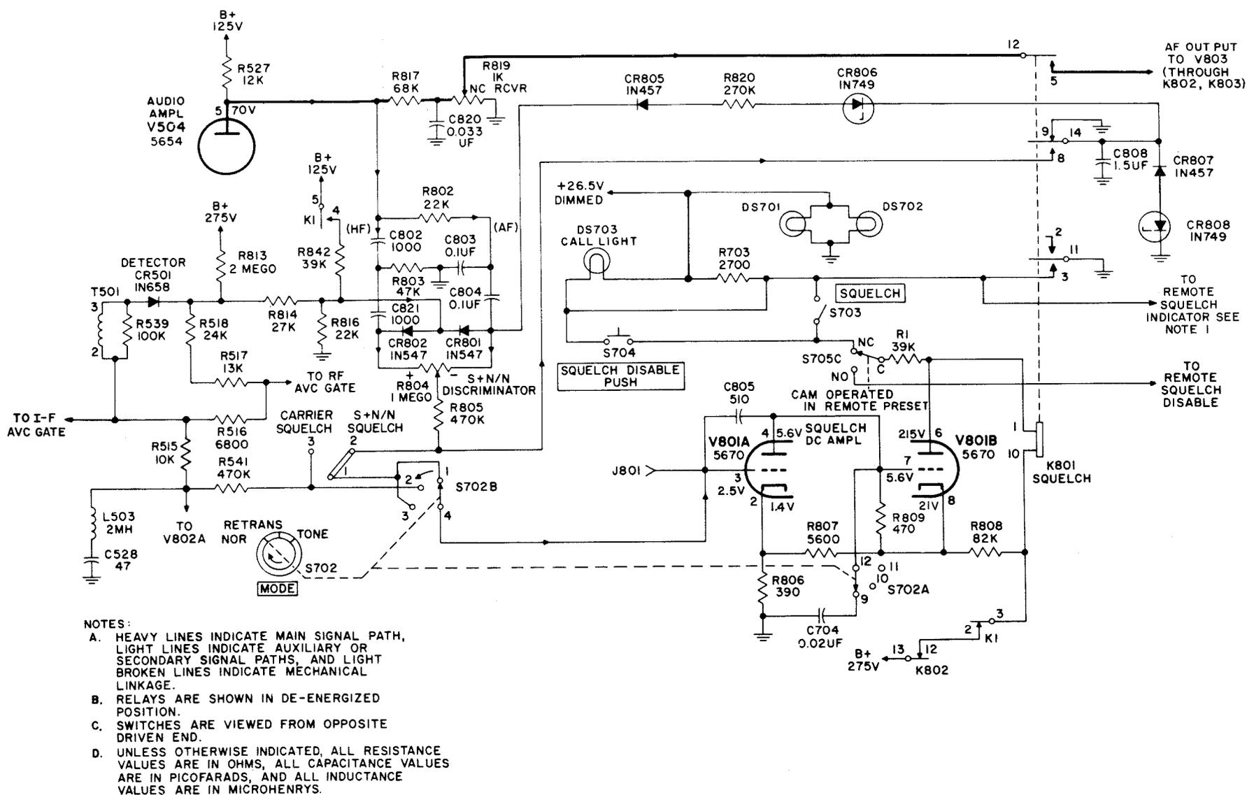
Figure 3-9. Radio Set AN/URC-9( ), Squelch Amplifier and Signal-Plus-Noise to Noise Discriminator, Simplified Schematic Diagram
