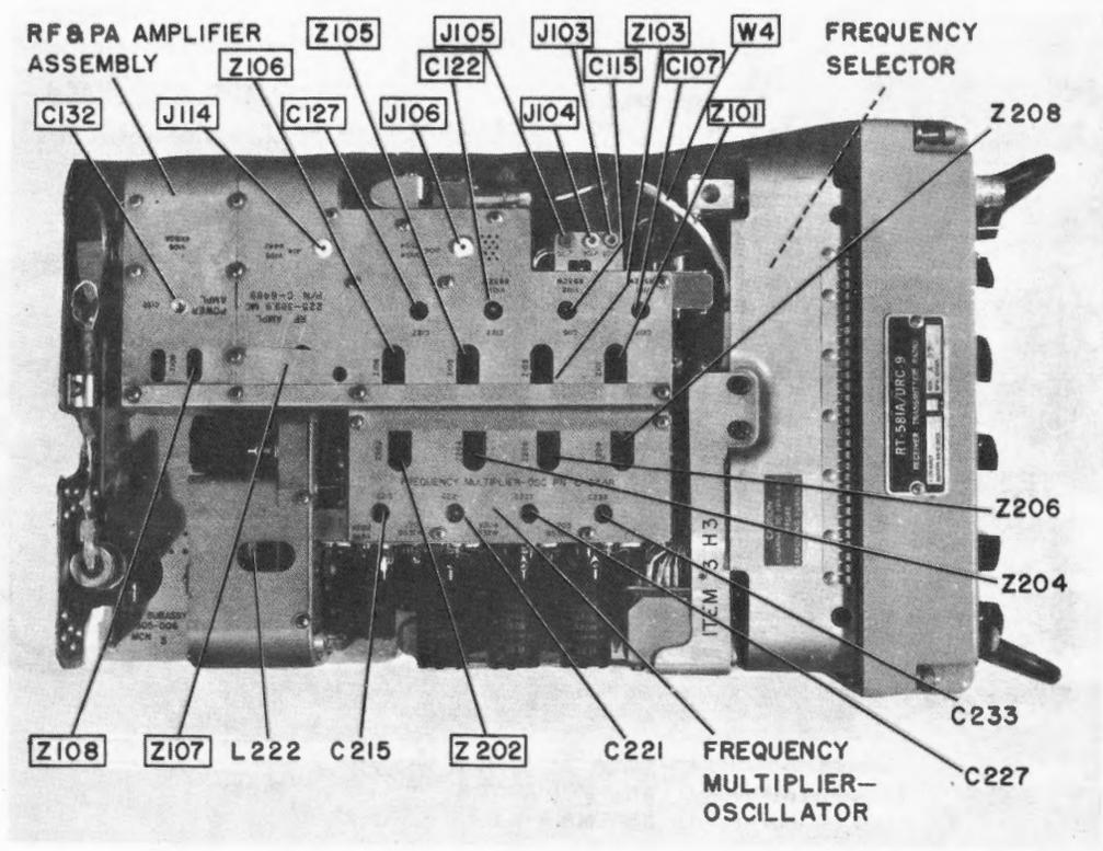
Figure 5-11. Receiver Transmitter RT-581( )/URC-9, Top View
