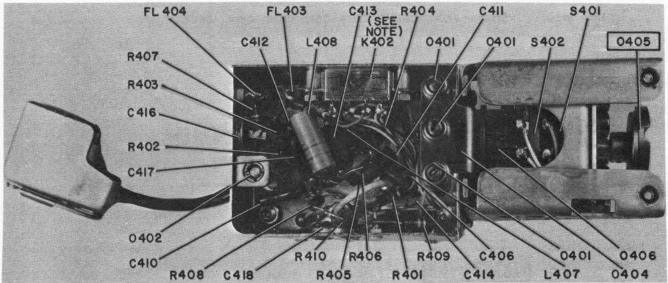
Figure 5-45. Second IF Amplifier, Bottom View
