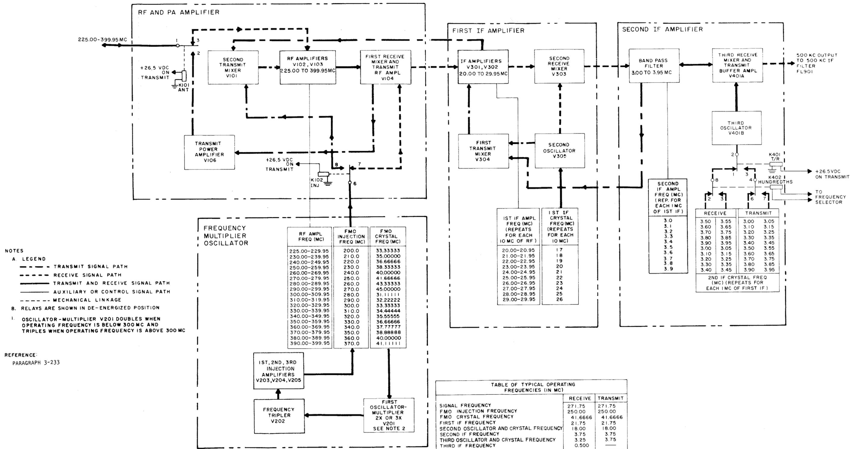
Figure 3-13. Radio Set AN/URC-9A Frequency Conversion System, Functional Block Diagram
