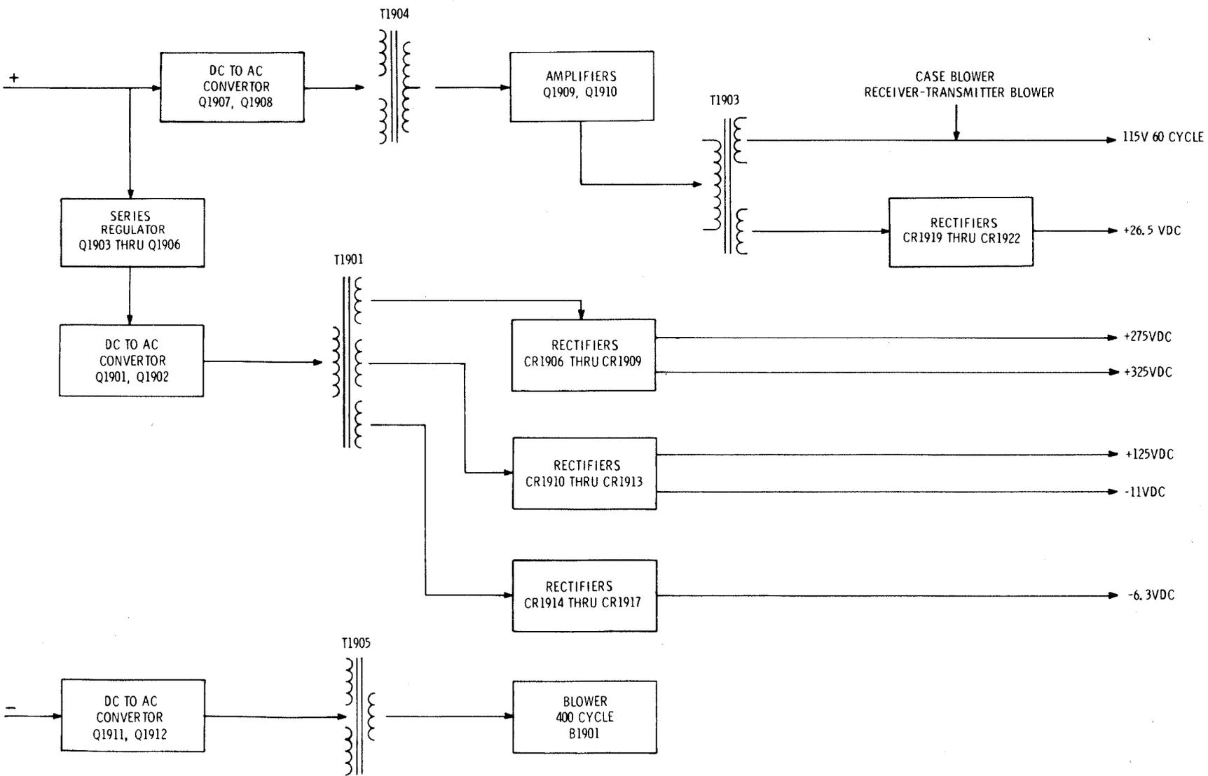
Figure 3-12. Power Supply PP-4706A/URC-9Y, Block Diagram
