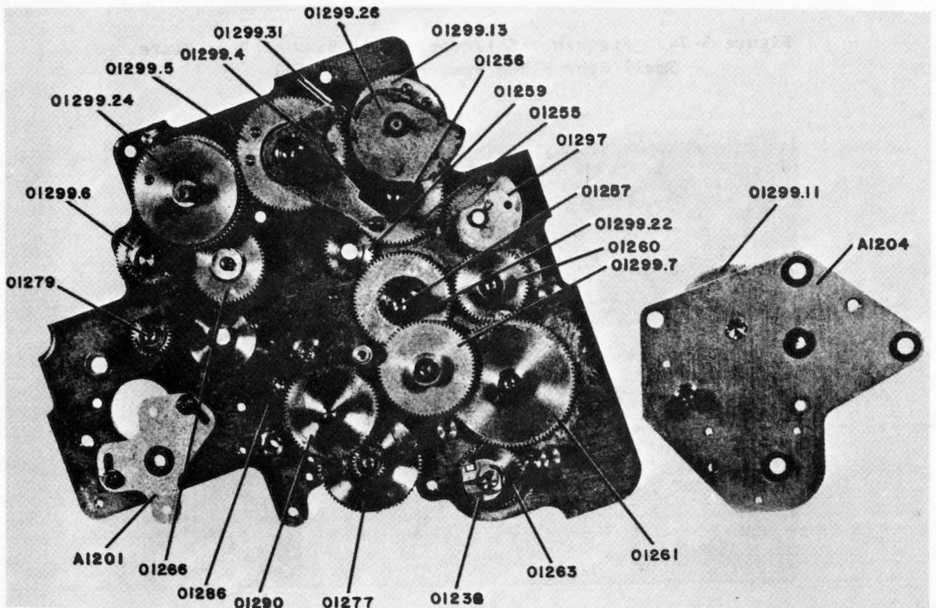
Figure 5-73. Frequency Selector, Front View of Rear Plate, Small Gear Plate Removed (AN/URC-9, -9Y, -9AY)
