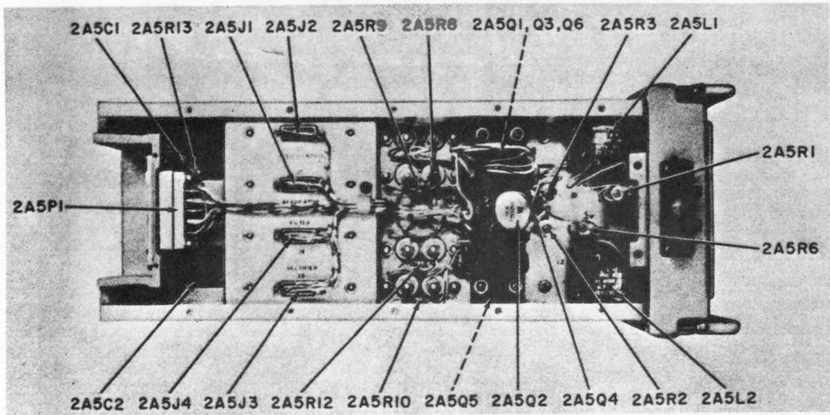
Figure 5-86. Power Supply PP-4706/URC-9Y, Bottom View
