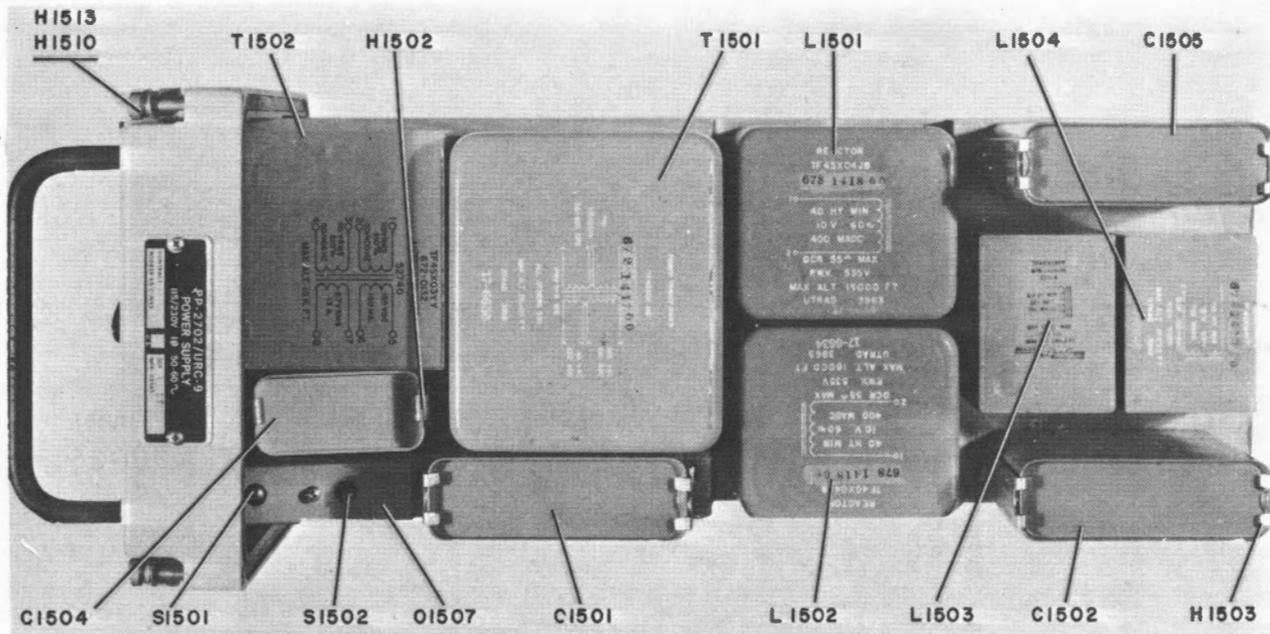
Figure 5-81. Power Supply PP-2702/URC-9, Top View
