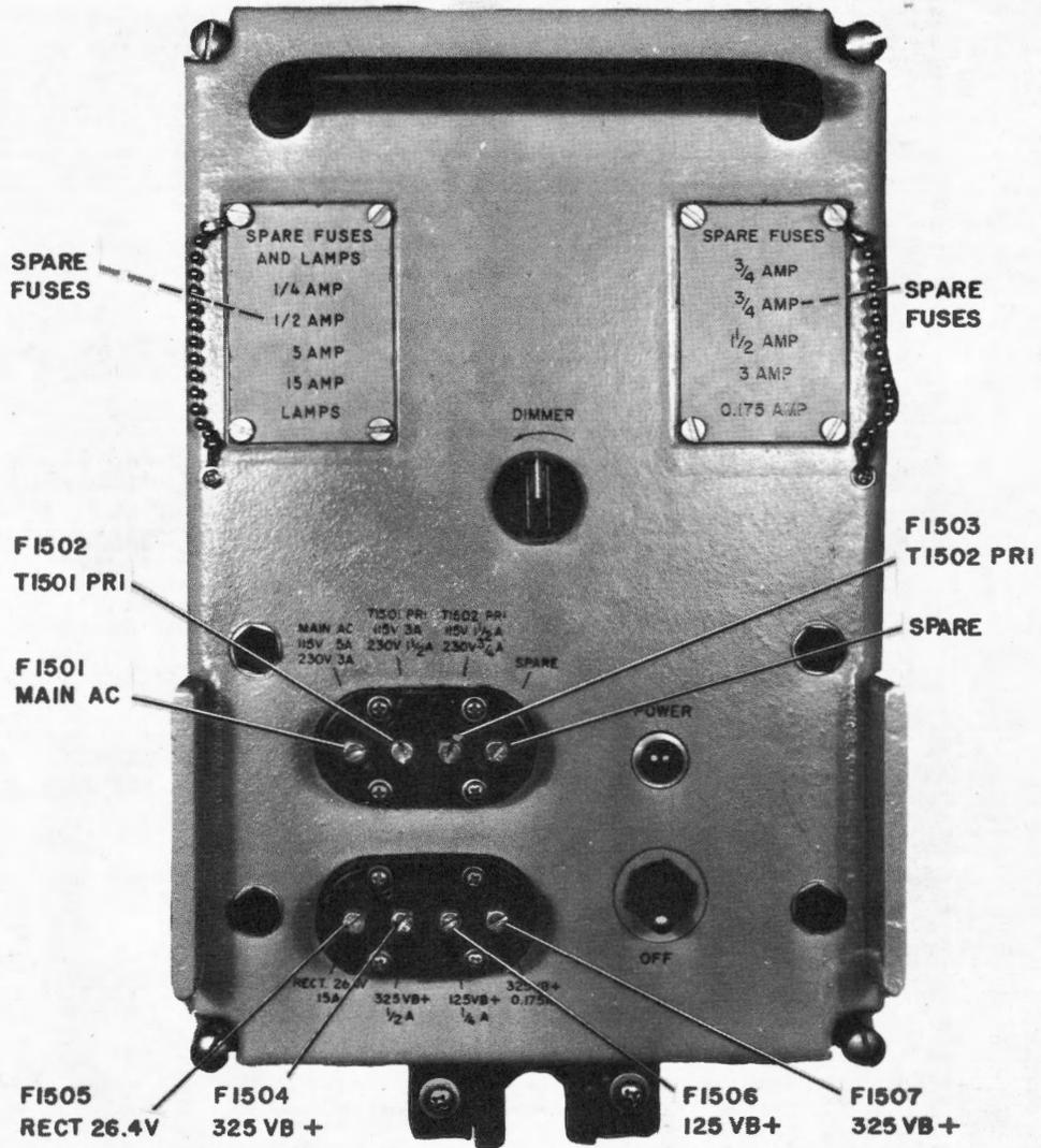
Figure 2-6. Radio Sets AN/URC-9 and 9A, Fuse Location
