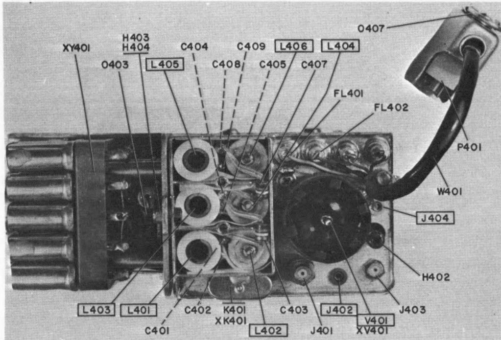
Figure 5-44. Second IF Amplifier, Top View
