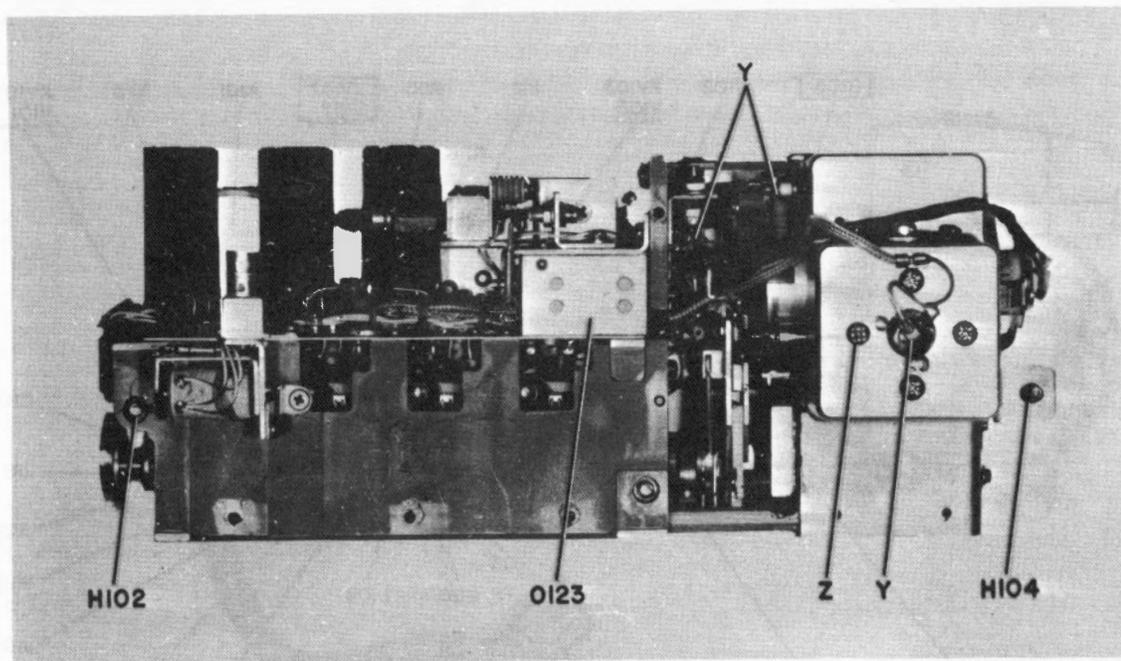
Figure 5-20. RF and PA Amplifier Assembly, Right Side, Disassembly Points
