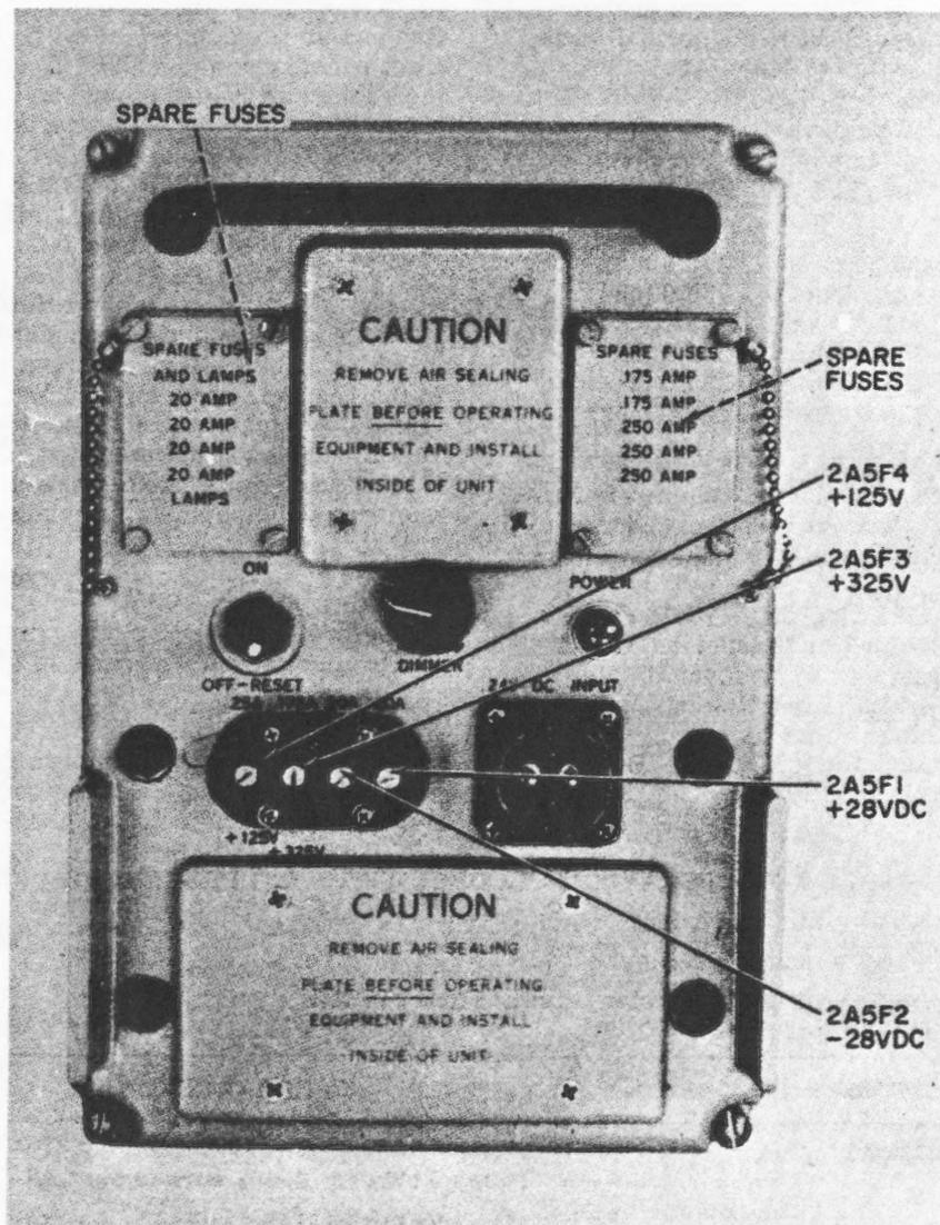
Figure 2-7. Radio Set AN/URC-9Y, Fuse Location
