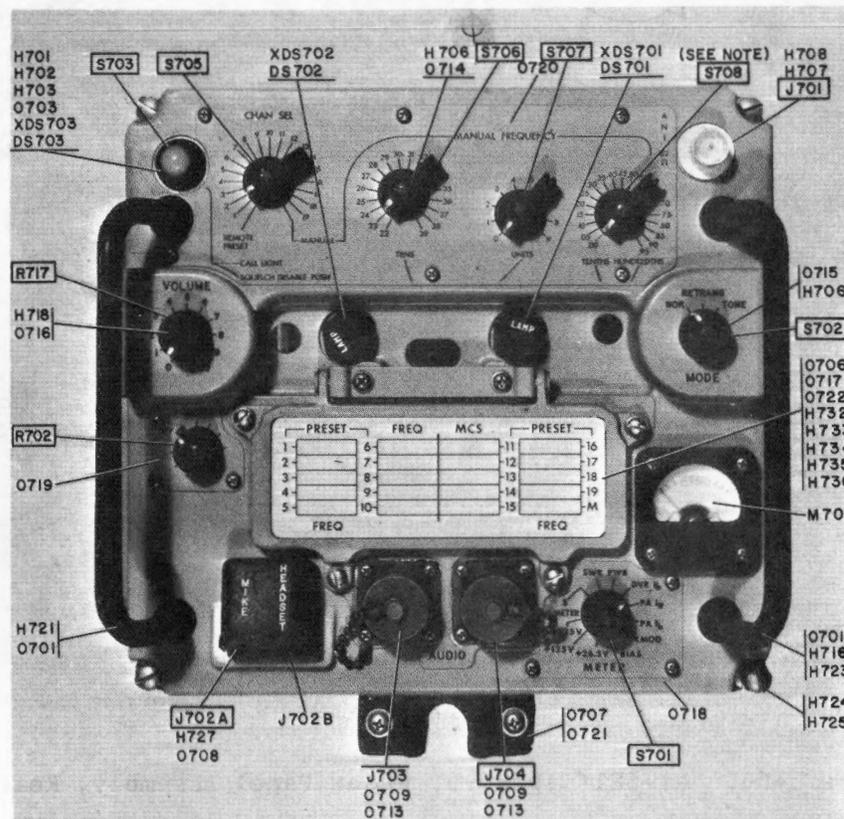
NOTE: .1 MHz increments on AN/URC-9, 9Y, and 9AY
