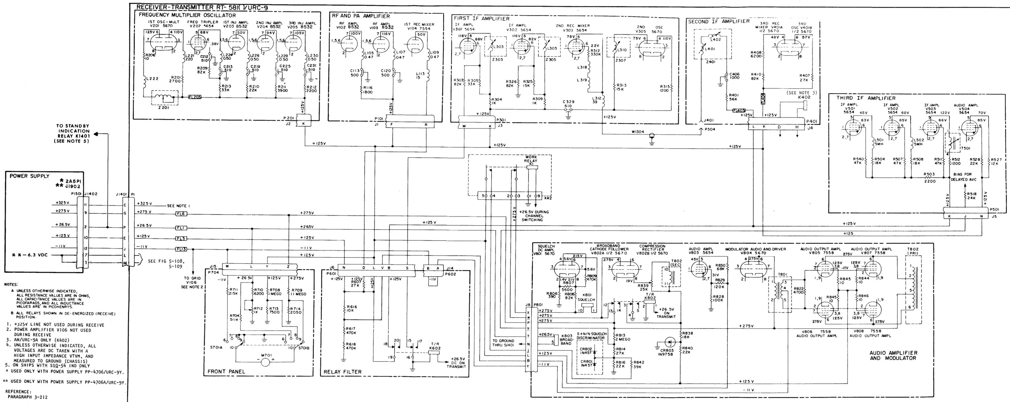
Figure 5-99. DC Power Distribution, Receive Function, Schematic Diagram
