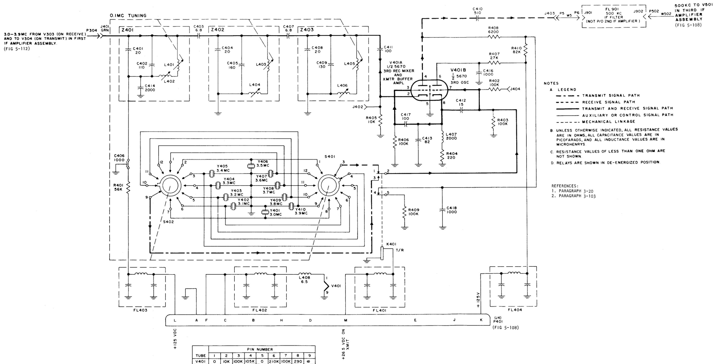
Figure 5-113. Second IF Amplifier Assembly, Schematic Diagram (AN/URC-9, -9Y, -9AY)
