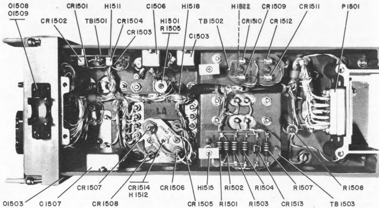
Figure 5-82. Power Supply PP-2702/URC-9, Bottom View
