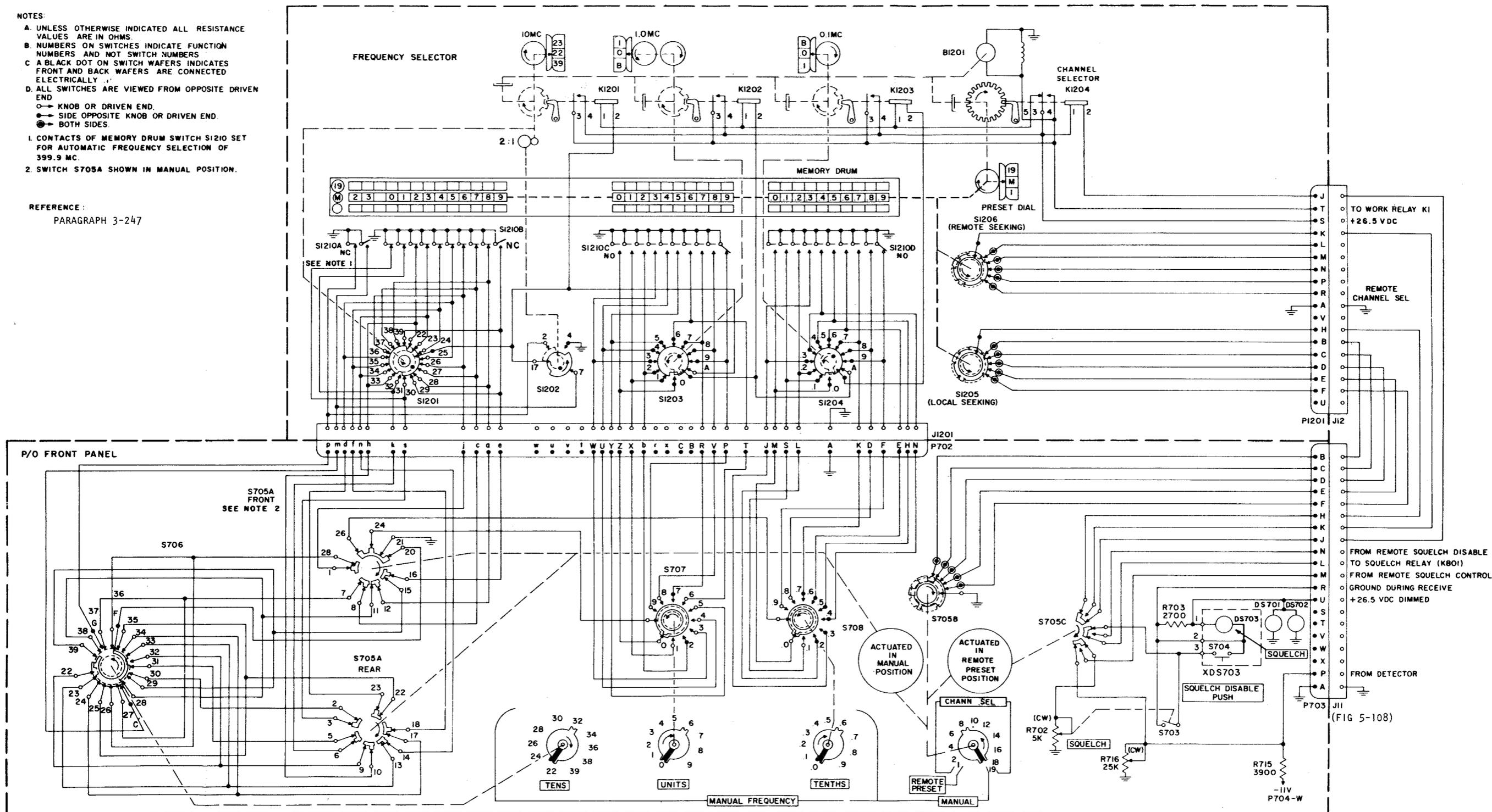
Figure 5-120. Part of Front Panel Assembly and Frequency Selector Assembly, Schematic Diagram (AN/URC-9, -9Y, -9AY)
