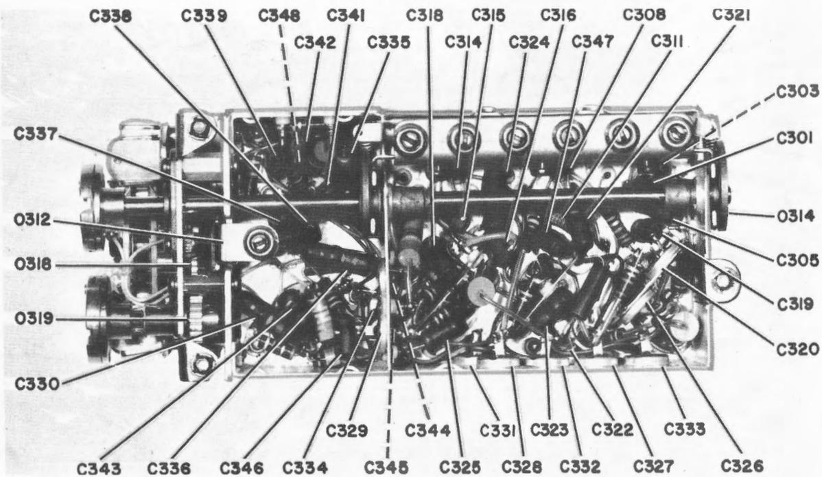
Figure 5-41. First IF Amplifier, Bottom View (B)
