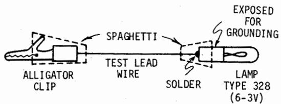
Connect Alligator clip to FL 201 on FMO Assembly. Ground side of lamp on Assembly being inspected. This Trouble Shooting light is used to illuminate the internal parts of each assembly while aligning the RT-581
