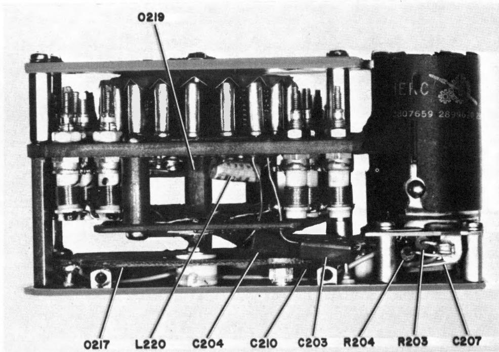
Figure 5-37. Frequency Multiplier-Oscillator,
