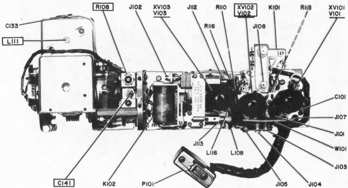
Figure 5-22. RF and PA Amplifier Assembly, Top View
