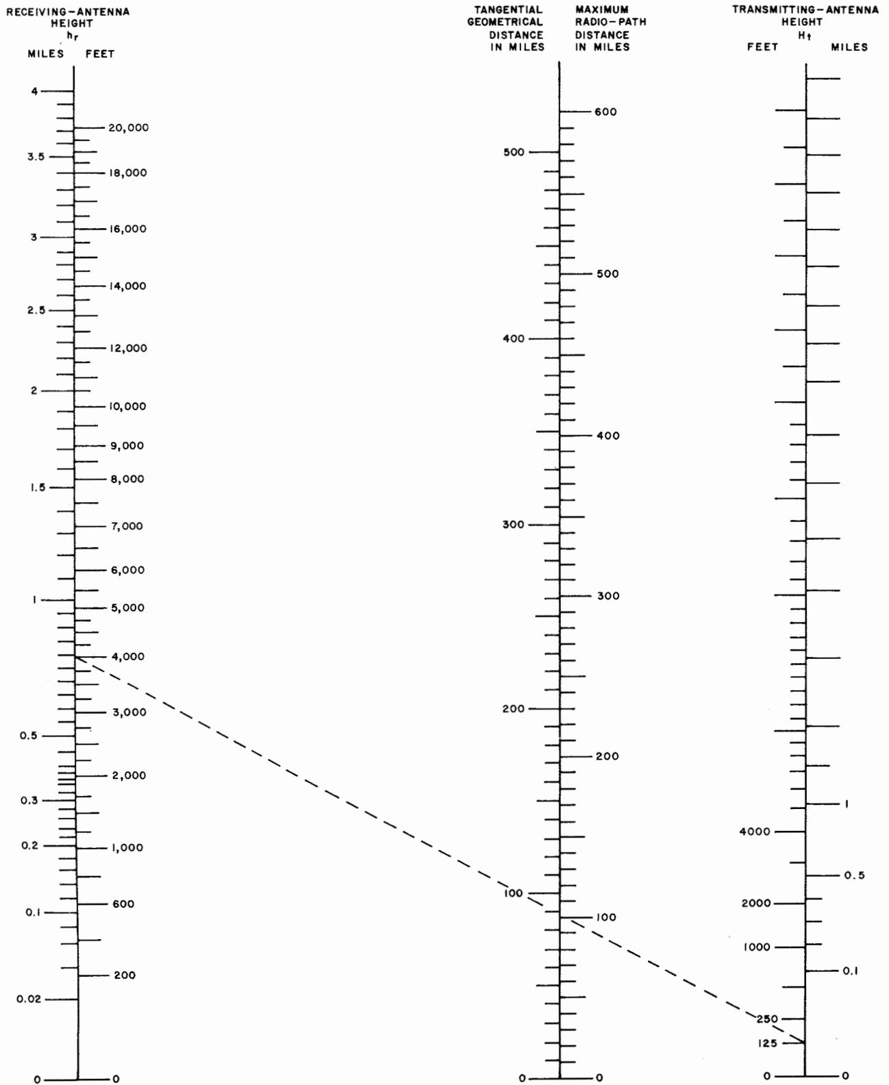
EXAMPLE SHOWN: HEIGHT OF RECEIVING-ANTENNA AIRPLANE 4000 FEET (0.76 MILES), HEIGHT OF TRANSMITTING-ANTENNA 125 FEET (0.02);
