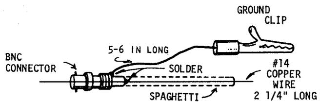
FOR USE WITH USM-207 COUNTER TO PROBE HARD TO REACH TEST JACKS.
