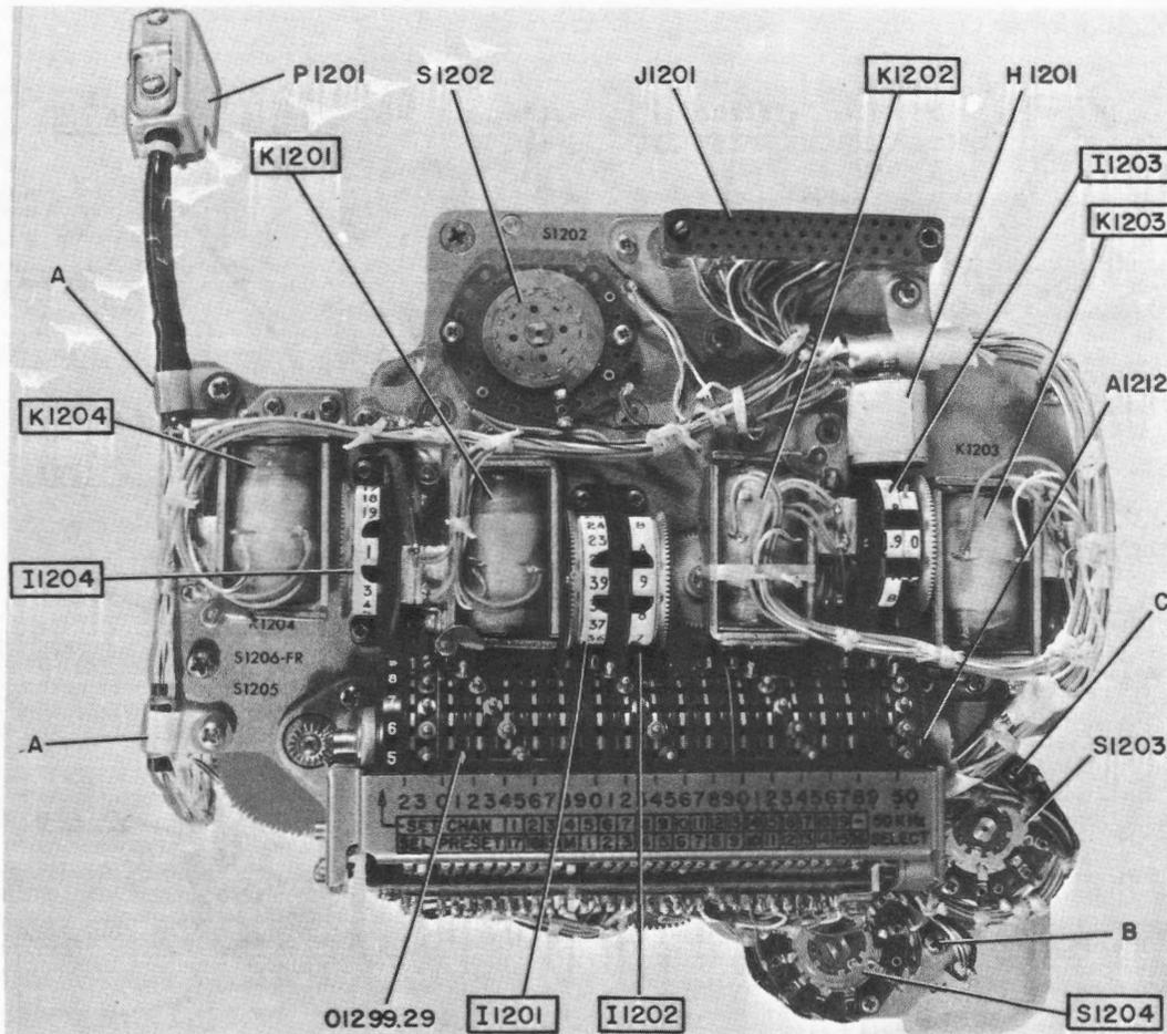
Figure 5-68. Frequency Selector, Front View (AN/URC-9A)
