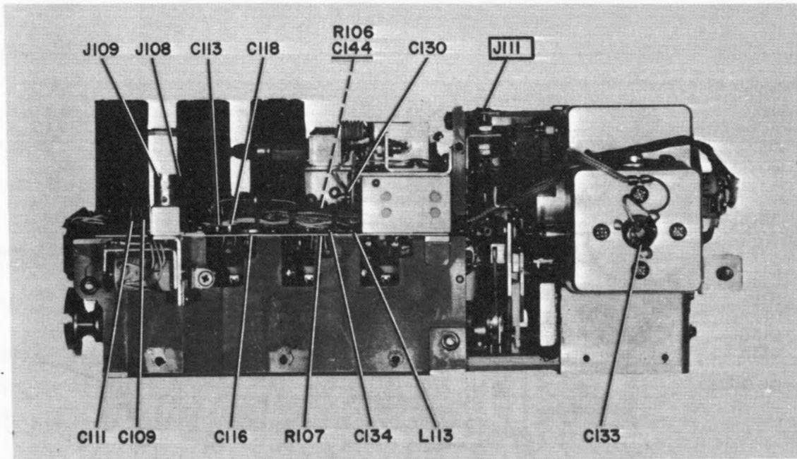
Figure 5-23. RF and PA Amplifier Assembly, Right Side
