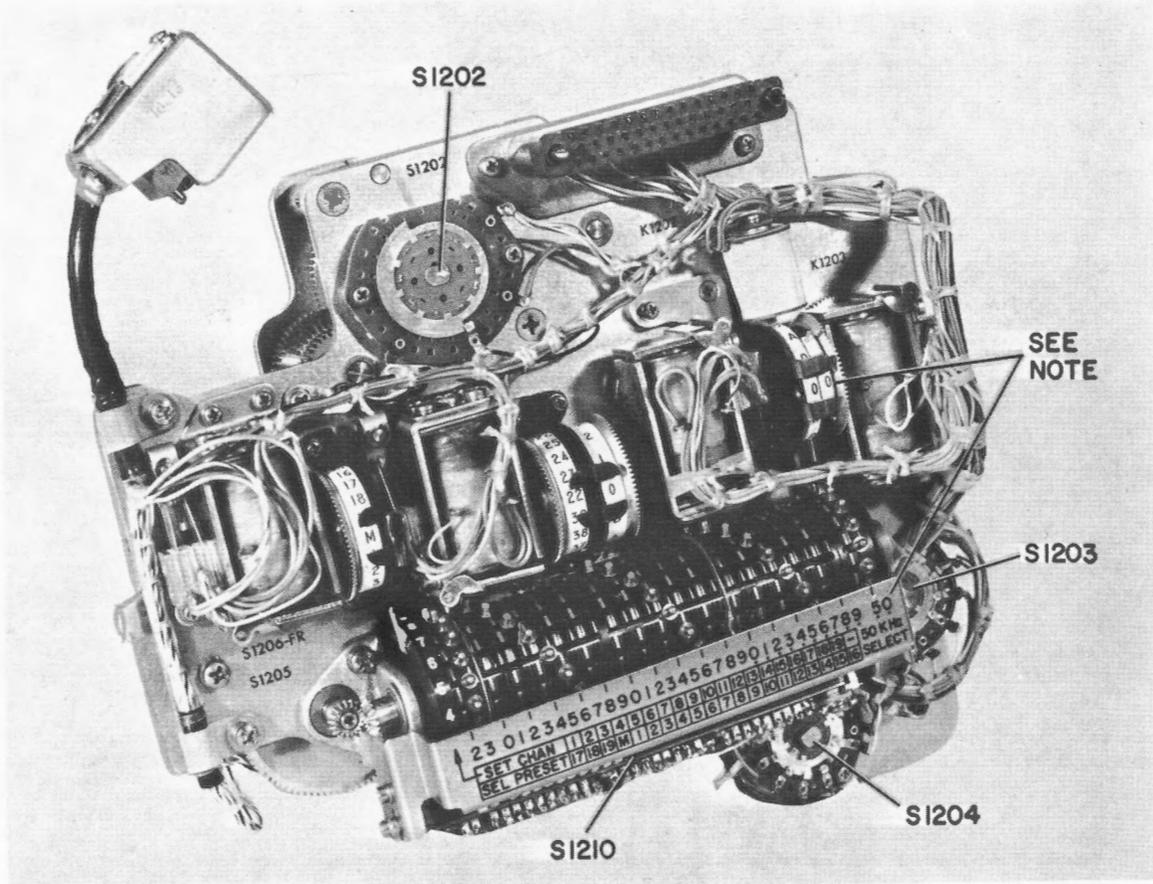
NOTE: Graduated in .1 MHz increments on AN/URC-9, 9Y, and 9AY
