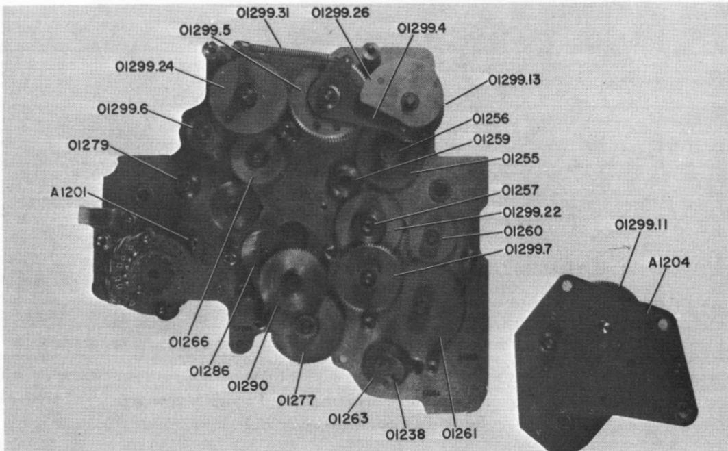
Figure 5-74. Frequency Selector, Front View of Rear Plate, Small Gear Plate Removed (AN/URC-9A)
