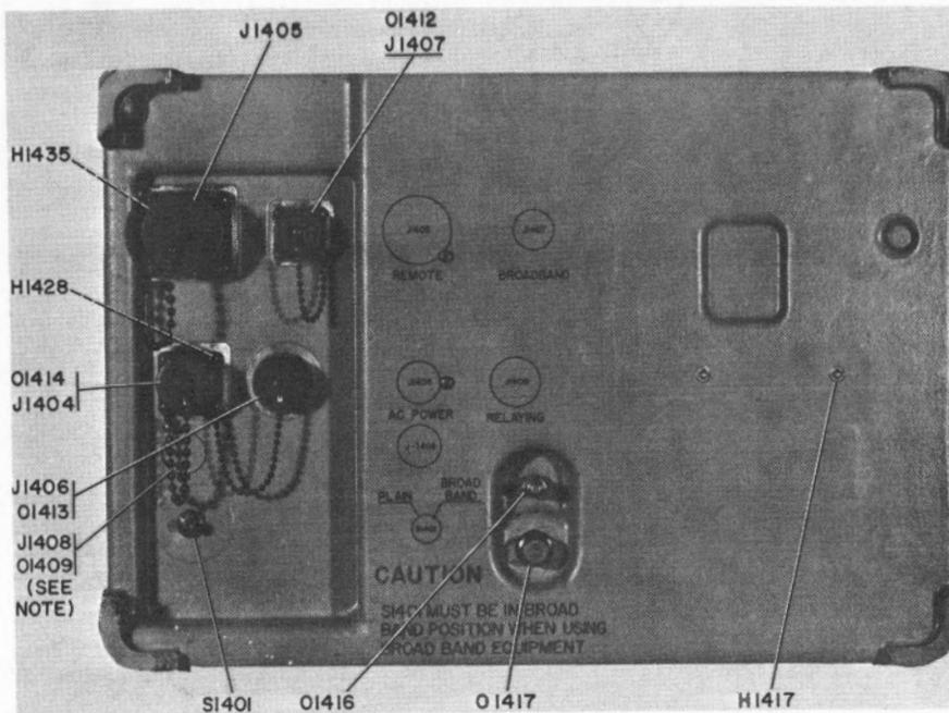
Figure 5-61. Receiver-Transmitter Case CY-2959/URC-9, Rear View
