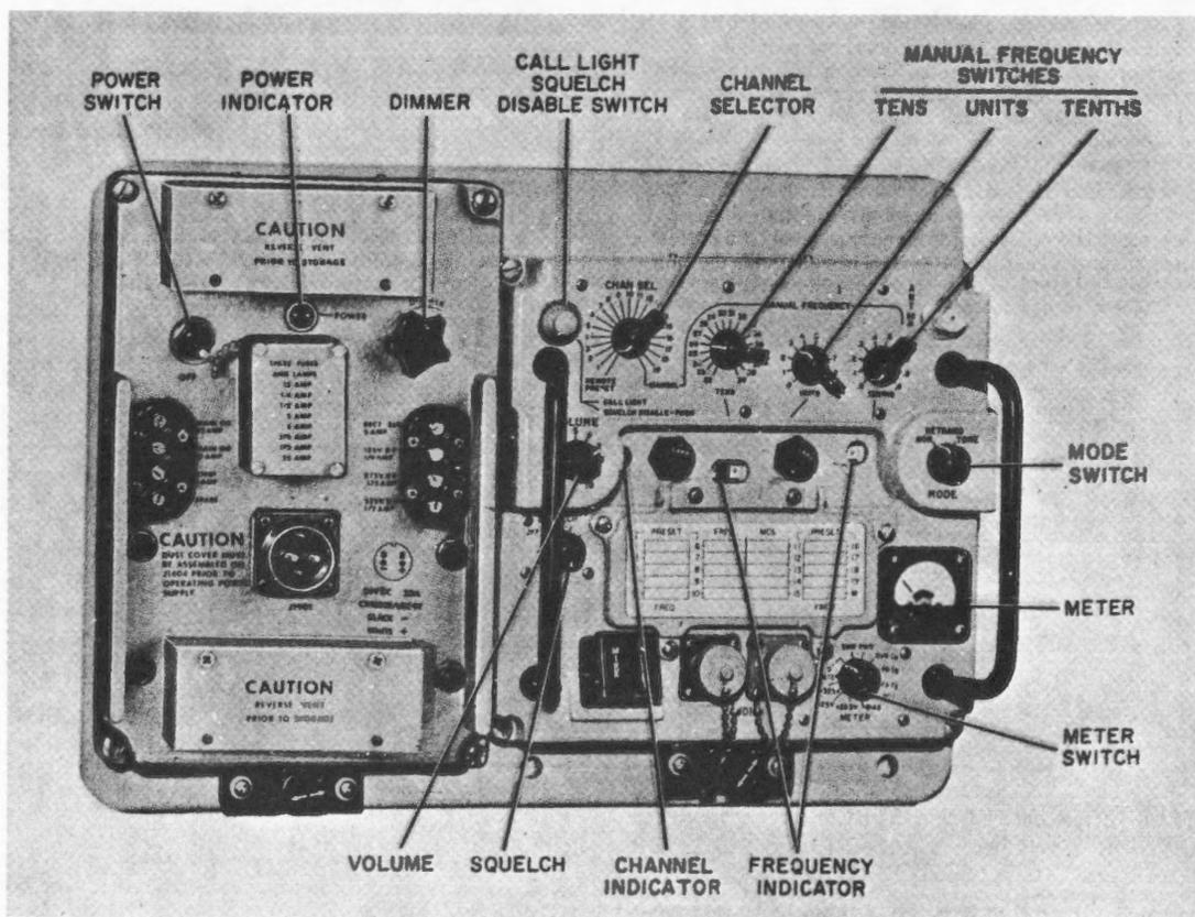
Figure 2-3. Radio Set AN/URC-9AY, Controls and Indicators
