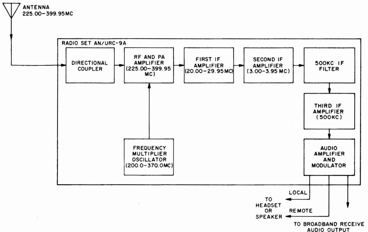
NOTE: Frequencies shown are for AN/URC-9A. Frequencies for AN/URC-9, 9Y, and 9AY are the same less the hundredths position.
