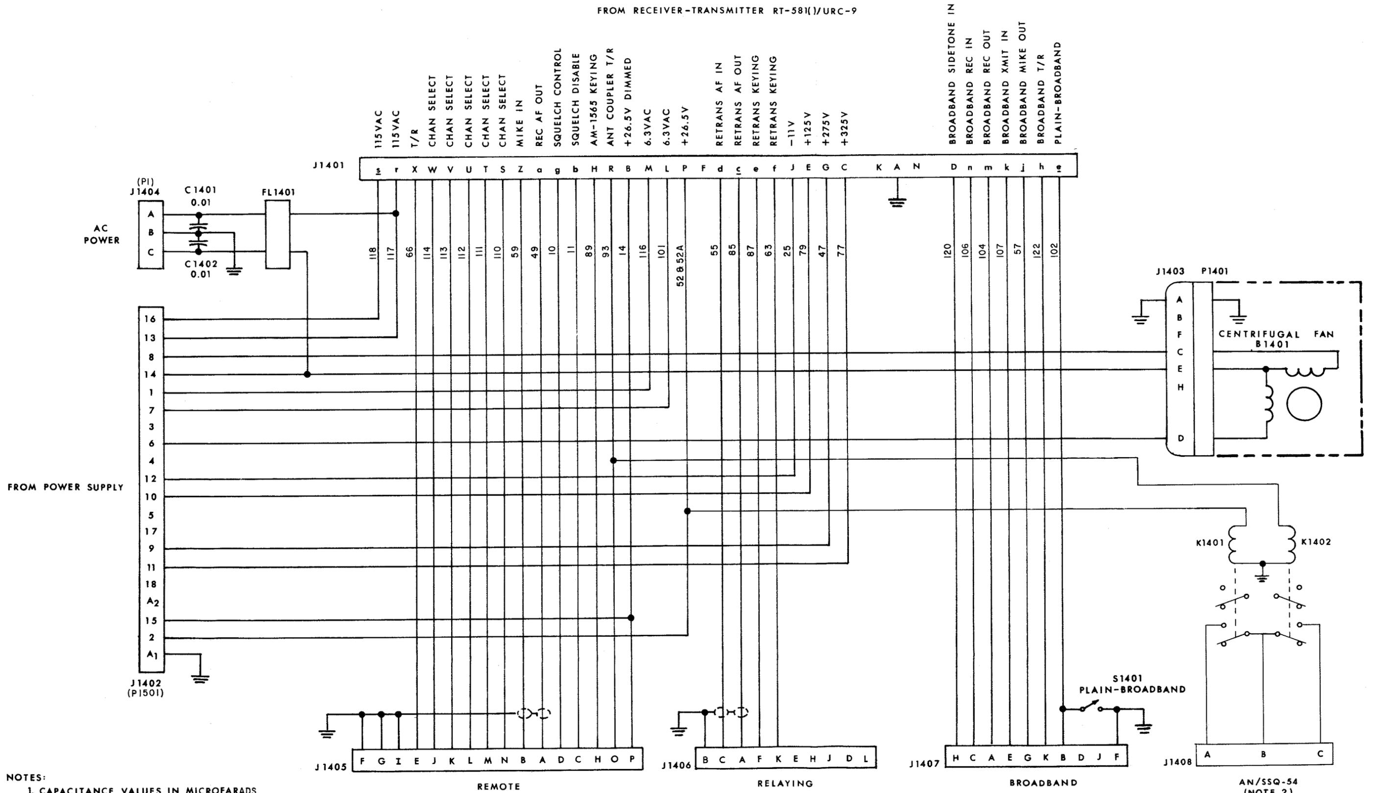
Figure 5-107. Receiver-Transmitter Case CY-2959/URC-9, Schematic Diagram
