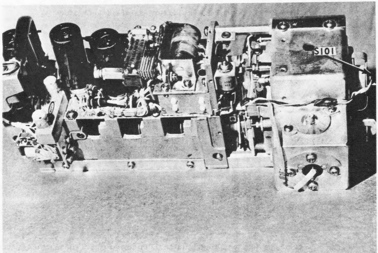
Figure 5-24. RF and PA Amplifier Assembly, Side View Showing Thermal Sensor
