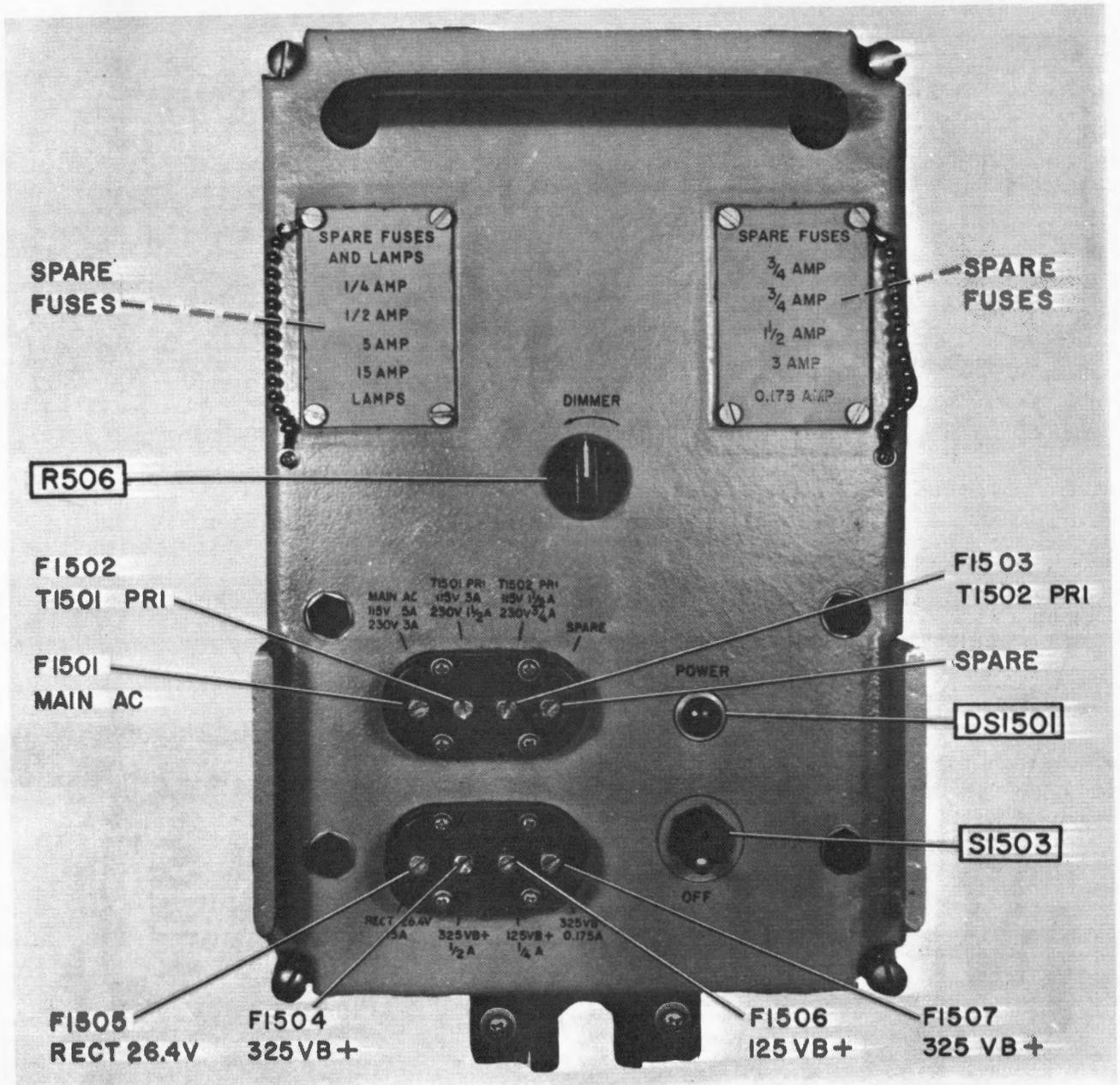
Figure 5-80. Power Supply PP-2702/URC-9, Front View
