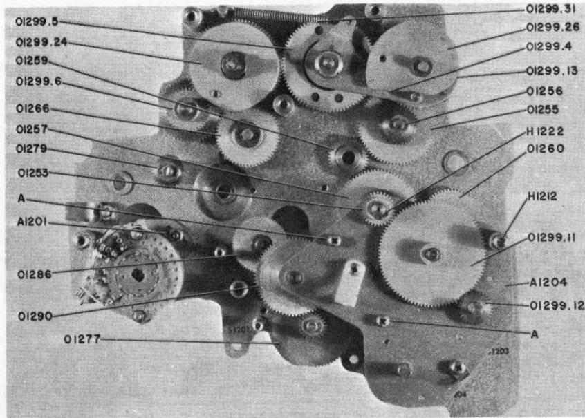
Figure 5-72. Frequency Selector, Front View of Rear Plate (AN/URC-9A)
