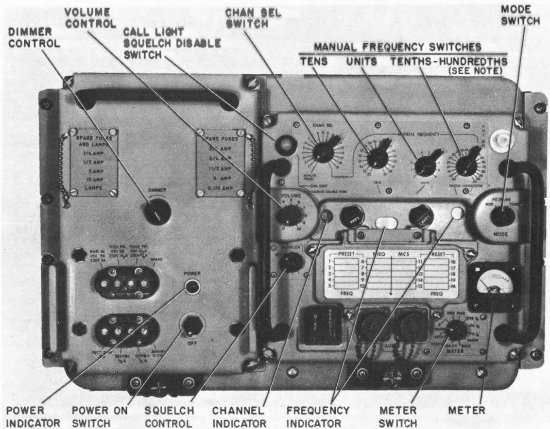
NOTE: Graduated in .1 MHz increments on AN/URC-9
