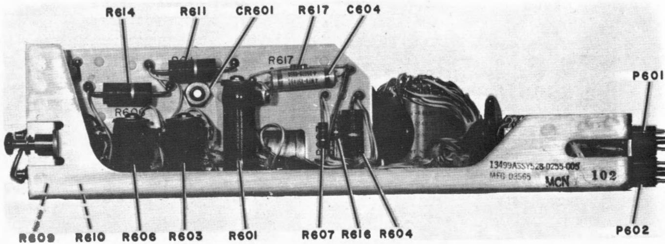
Figure 5-54. Relay-Filter Assembly, Right Side
