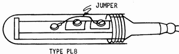
This Transmitter Key Plug is used to key the RT-581 During the Trouble Shooting and Alignment Procedures.
