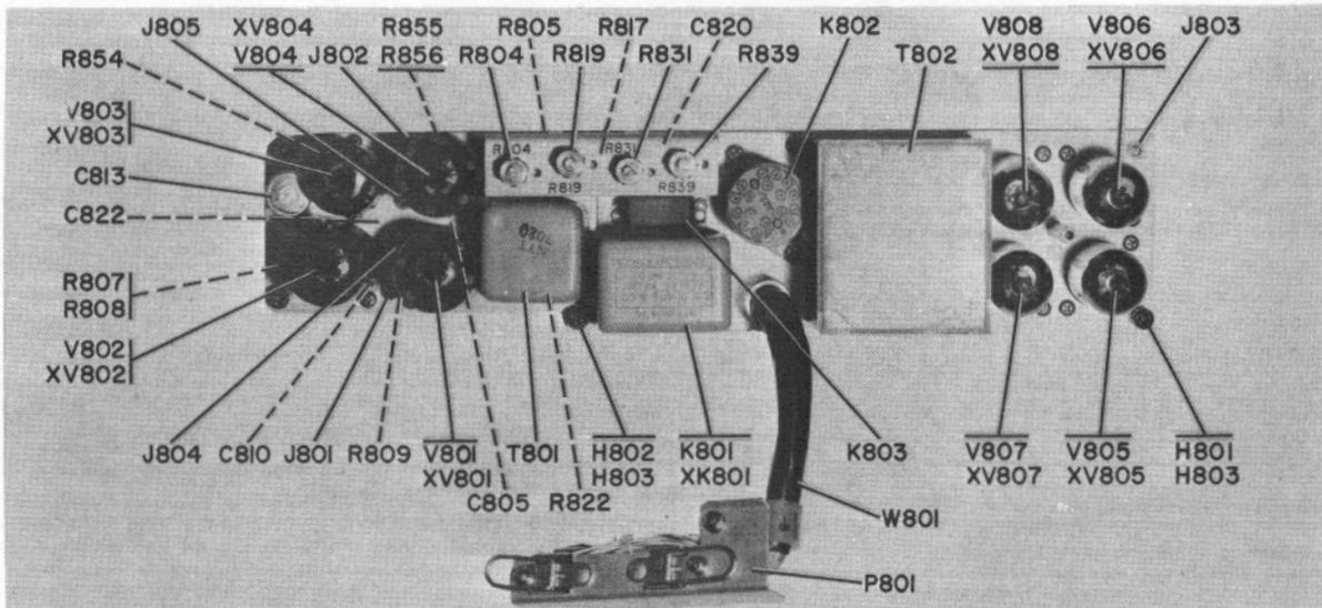
Figure 5-50. Audio Frequency Amplifier and Modulator Assembly, Top View
