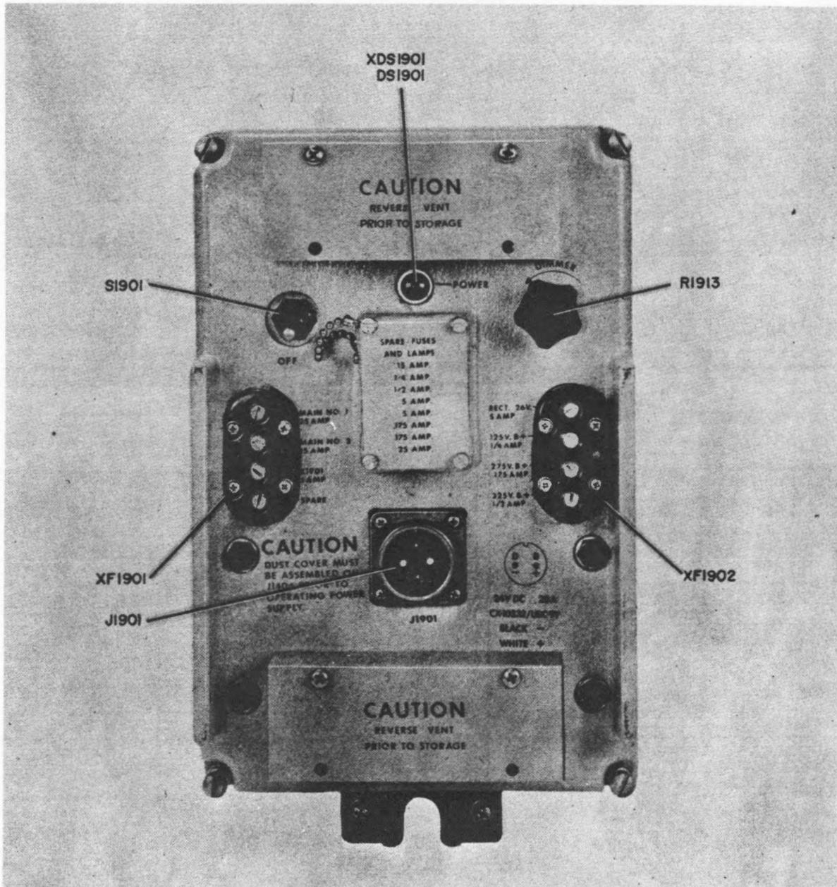
Figure 5-91. Power Supply PP-4706A/URC-9Y, Front View
