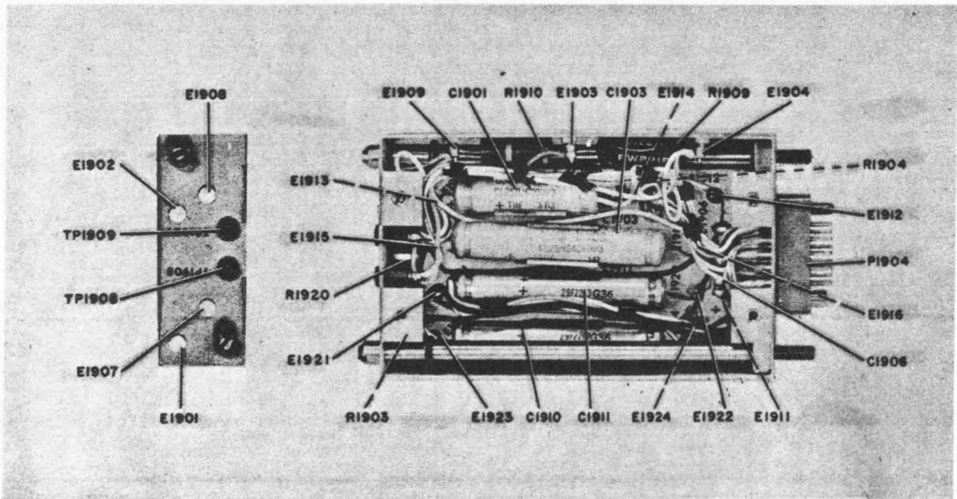
Figure 5-95. Power Supply PP-4706A/URC-9Y, Resistor
