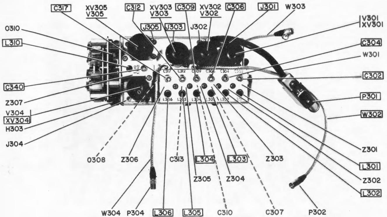
Figure 5-39. First IF Amplifier, Top View
