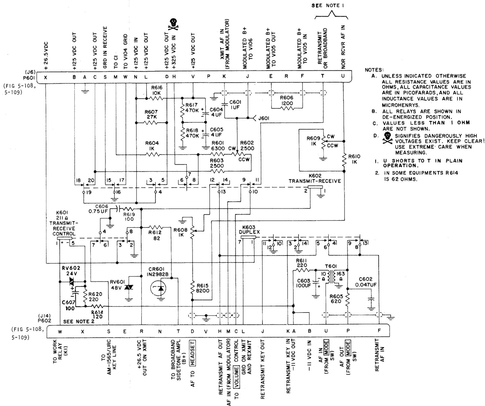
Figure 5-118. Relay-Filter Assembly, Schematic Diagram
