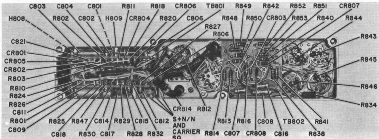
Figure 5-51. Audio Frequency Amplifier and Modulator Assembly, Bottom View
