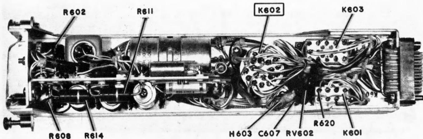
Figure 5-52. Relay-Filter Assembly, Top View
