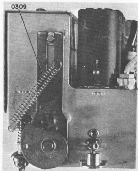
Figure 5-43. First IF Amplifier, Synchronization
