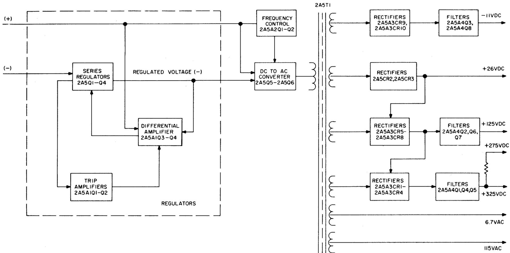
Figure 3-11. Power Supply PP-4706/URC-9Y, Block Diagram
