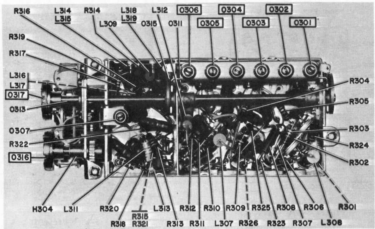
Figure 5-40. First IF Amplifier, Bottom View (A)
