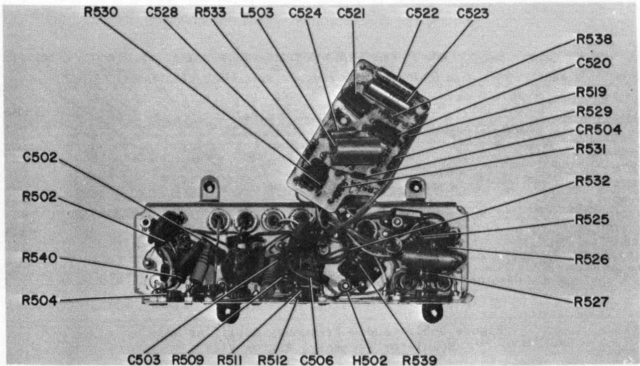
Figure 5-49. Third IF Amplifier, Bottom View (B)
