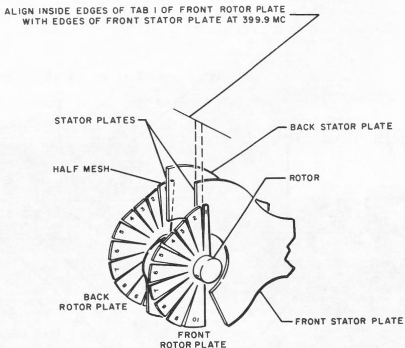
FMO, RF AND PA ASSEMBLIES TUNER CAPACITOR PLATES
