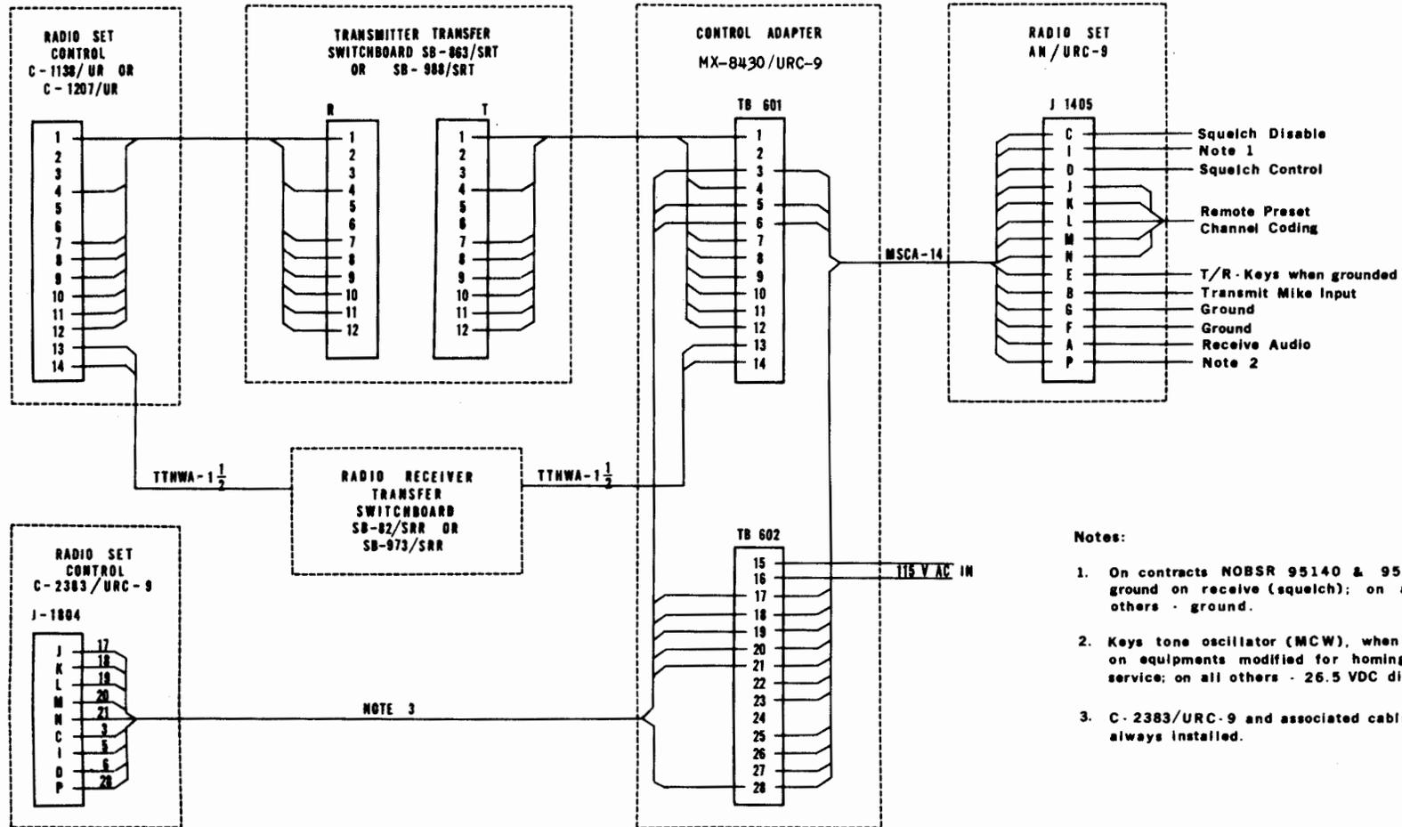
Figure 2-4. Basic Communications Systems Interconnection Wiring Diagram
