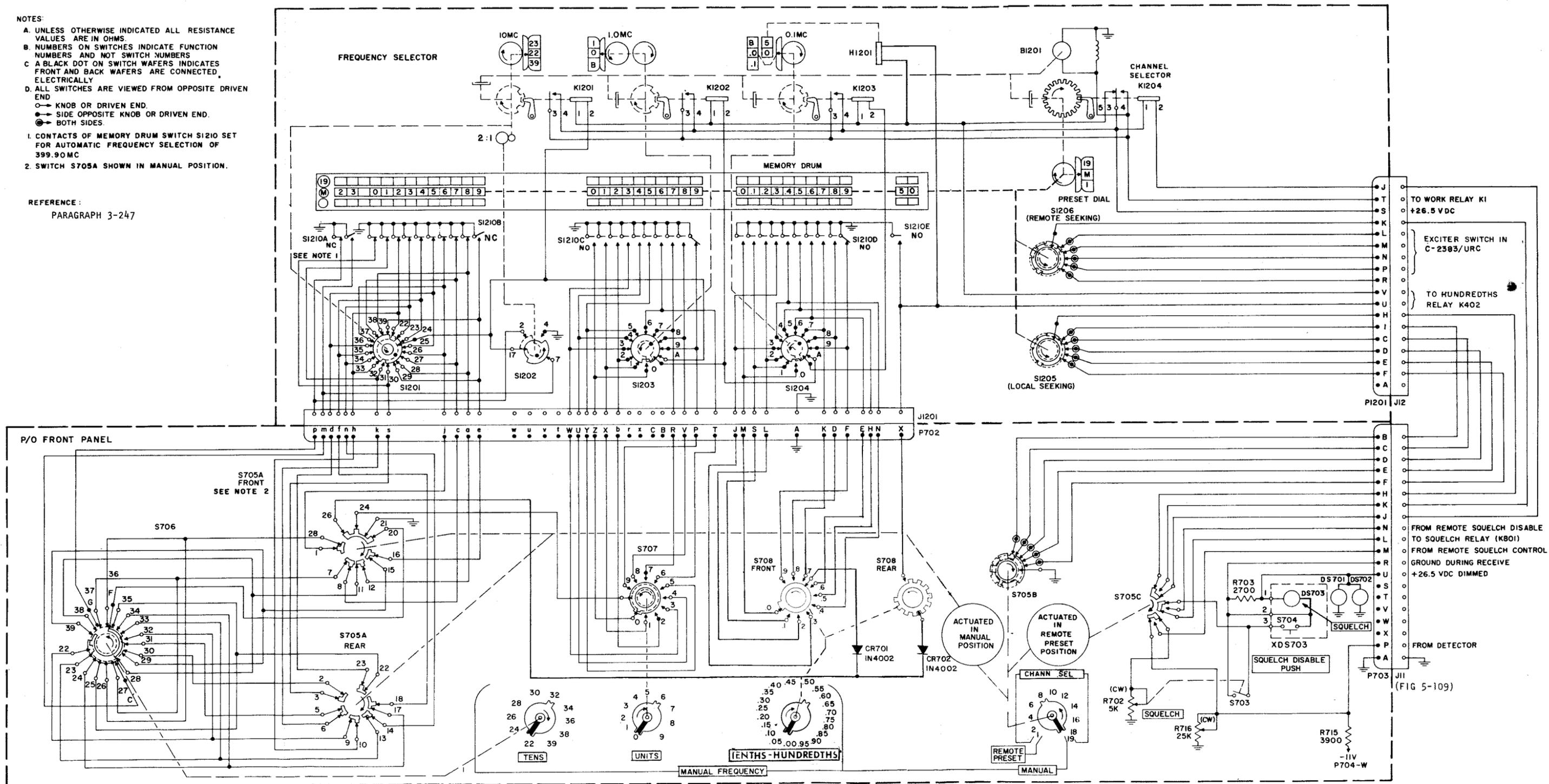
Figure 5-121. Part of Front Panel Assembly and Frequency Selector Assembly, Schematic Diagram (AN/URC-9A)
