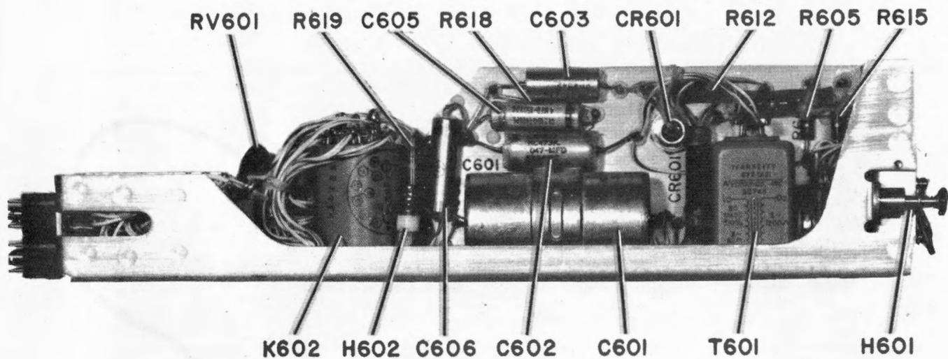
Figure 5-53. Relay-Filter Assembly, Left Side
