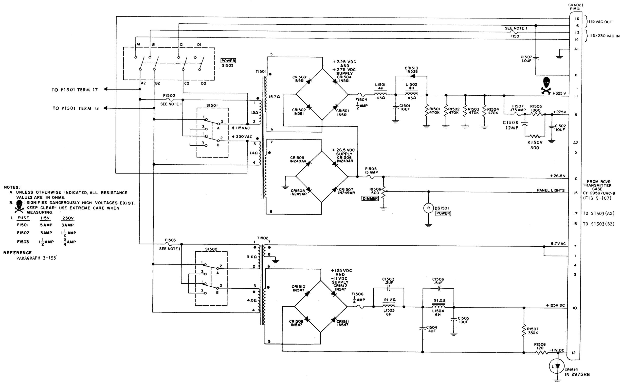
Figure 5-106. Power Supply PP-2702/URC-9, Schematic Diagram
