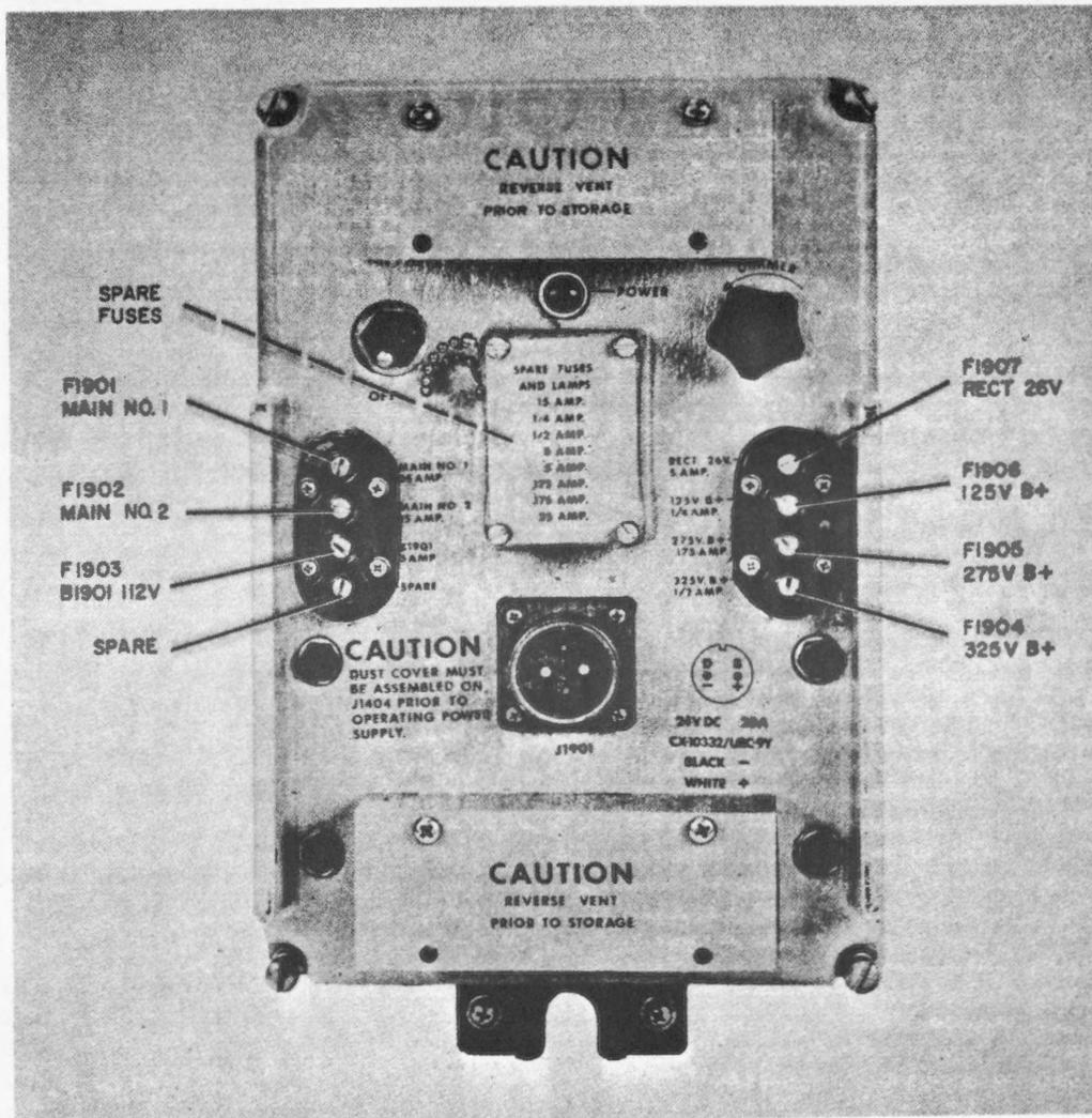
Figure 2-8, Radio Set AN/URC-9AY, Fuse Location
