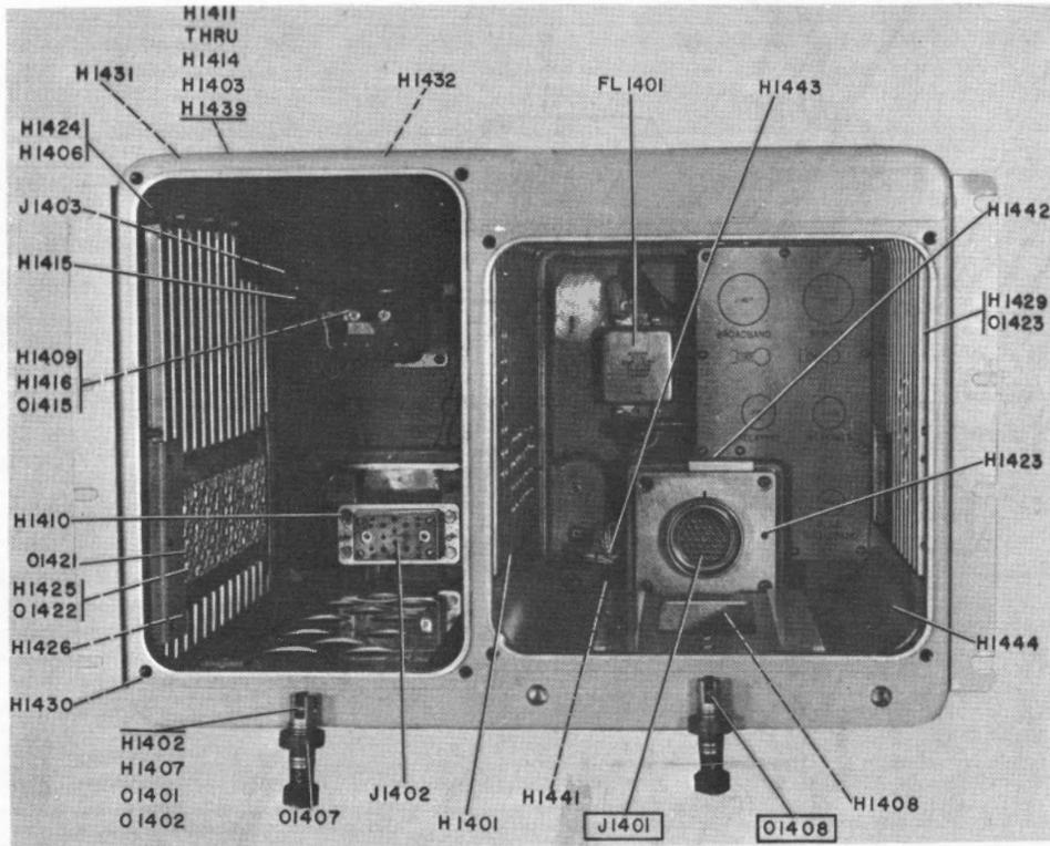
Figure 5-60. Receiver-Transmitter Case CY-2959/URC-9, Front View
