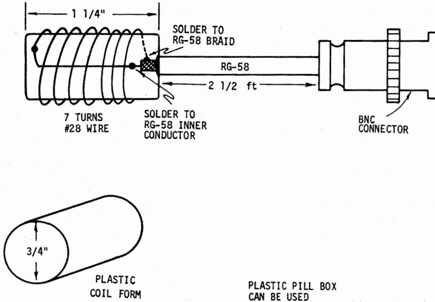
This pick-up loop is used with electronic frequency counters to verify various frequencies generated in RT-581. It is particularly useful for coupling RF from V201 into AN/USM 207 frequency counter.
