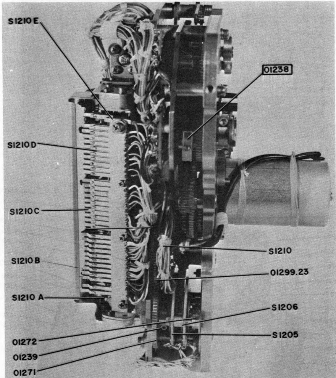
Figure 5-69. Frequency Selector, Bottom View
