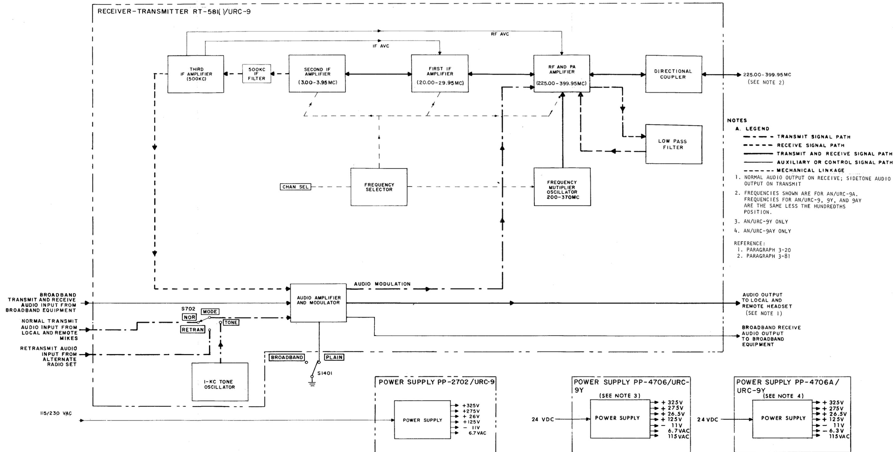
Figure 3-3. Radio Set AN/URC-9( ), Functional Block Diagram
