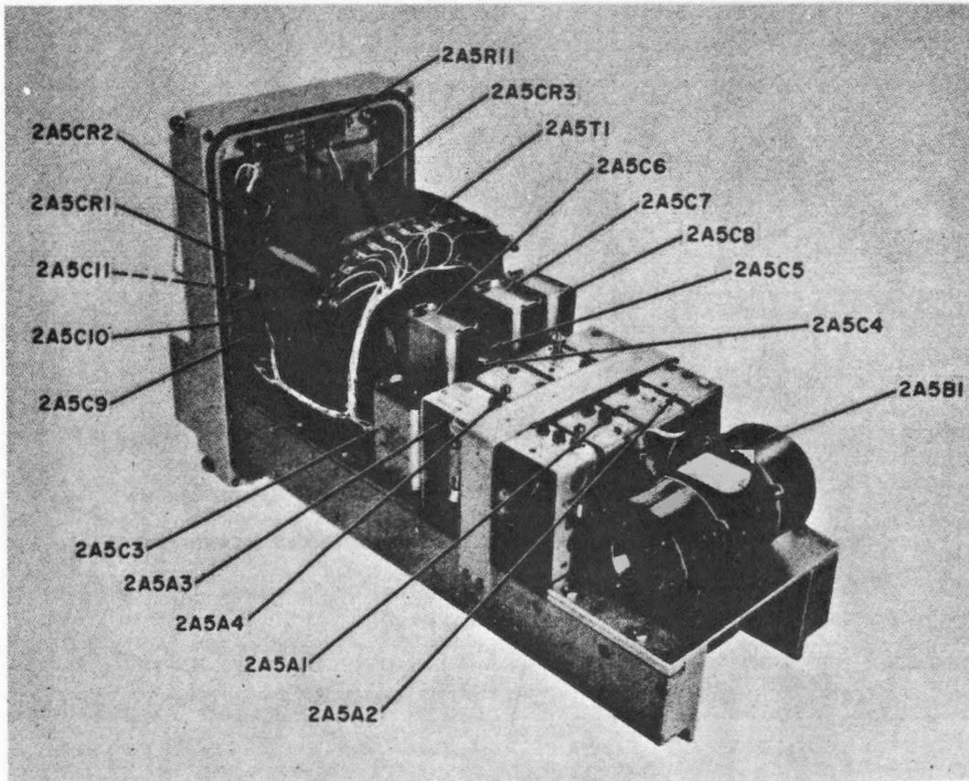
Figure 5-85. Power Supply PP-4706/URC-9Y, Top View
