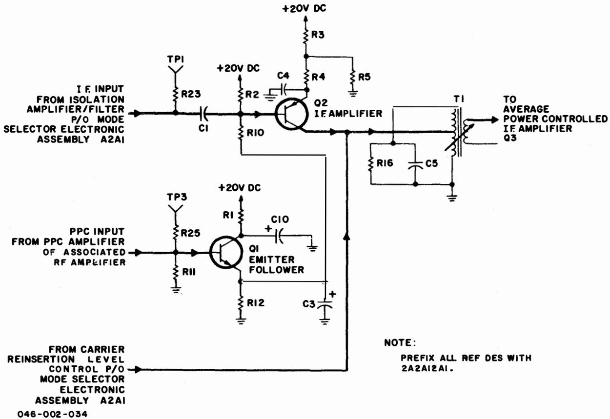
Figure 3-21. T-827B/URT, Peak-Power-Controlled IF. Amplifier, Simplified Schematic Diagram
