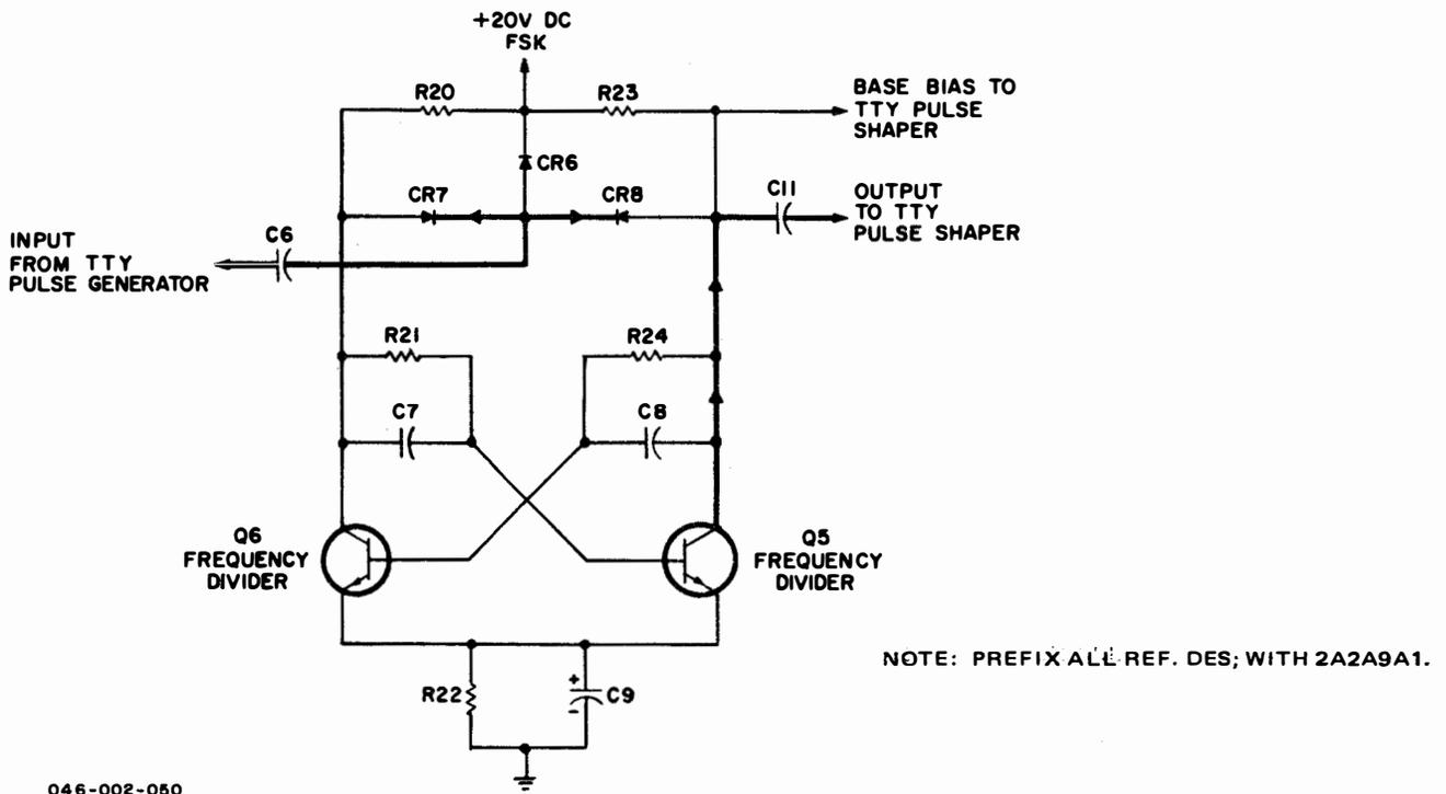
Figure 3-32. T-827B/URT, TTY Frequency Divider, Simplified Schematic Diagram
