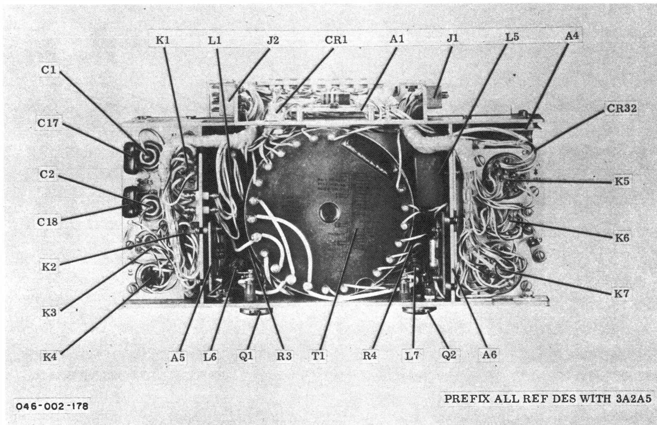
Figure 5-76. DC-to-DC Converter Assembly 3A2A5
