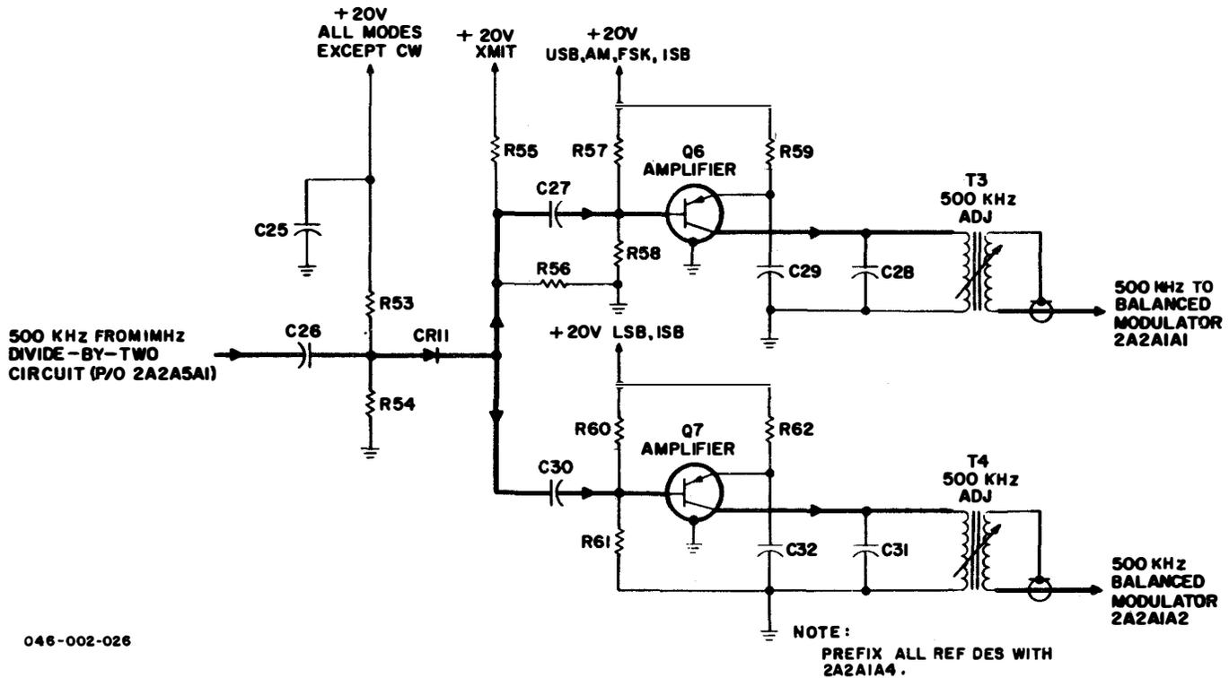
Figure 3-13. T-827B/URT, 500-kHz Amplifiers, Simplified Schematic Diagram
