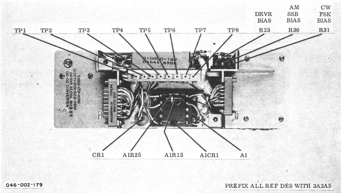
Figure 5-77. DC-to-DC Converter Assembly 3A2A5
