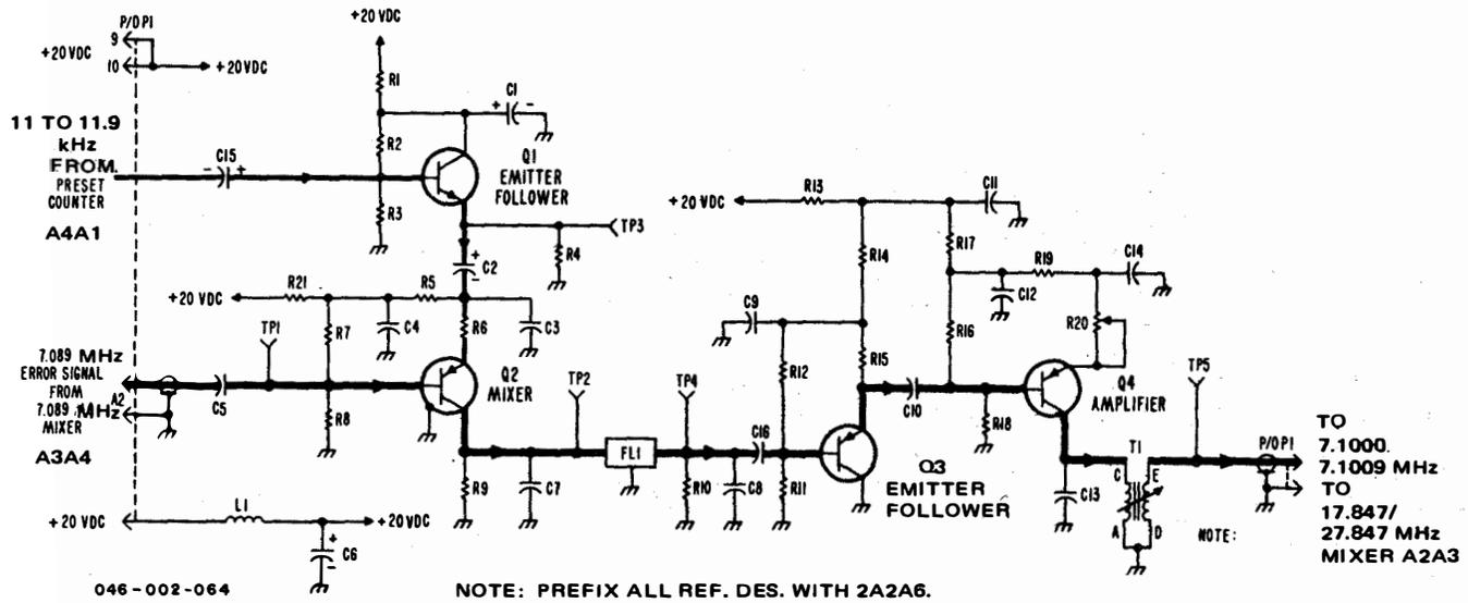
Figure 3-48. T-827B/URT, 7.1-MHz Mixer, Simplified Schematic Diagram
