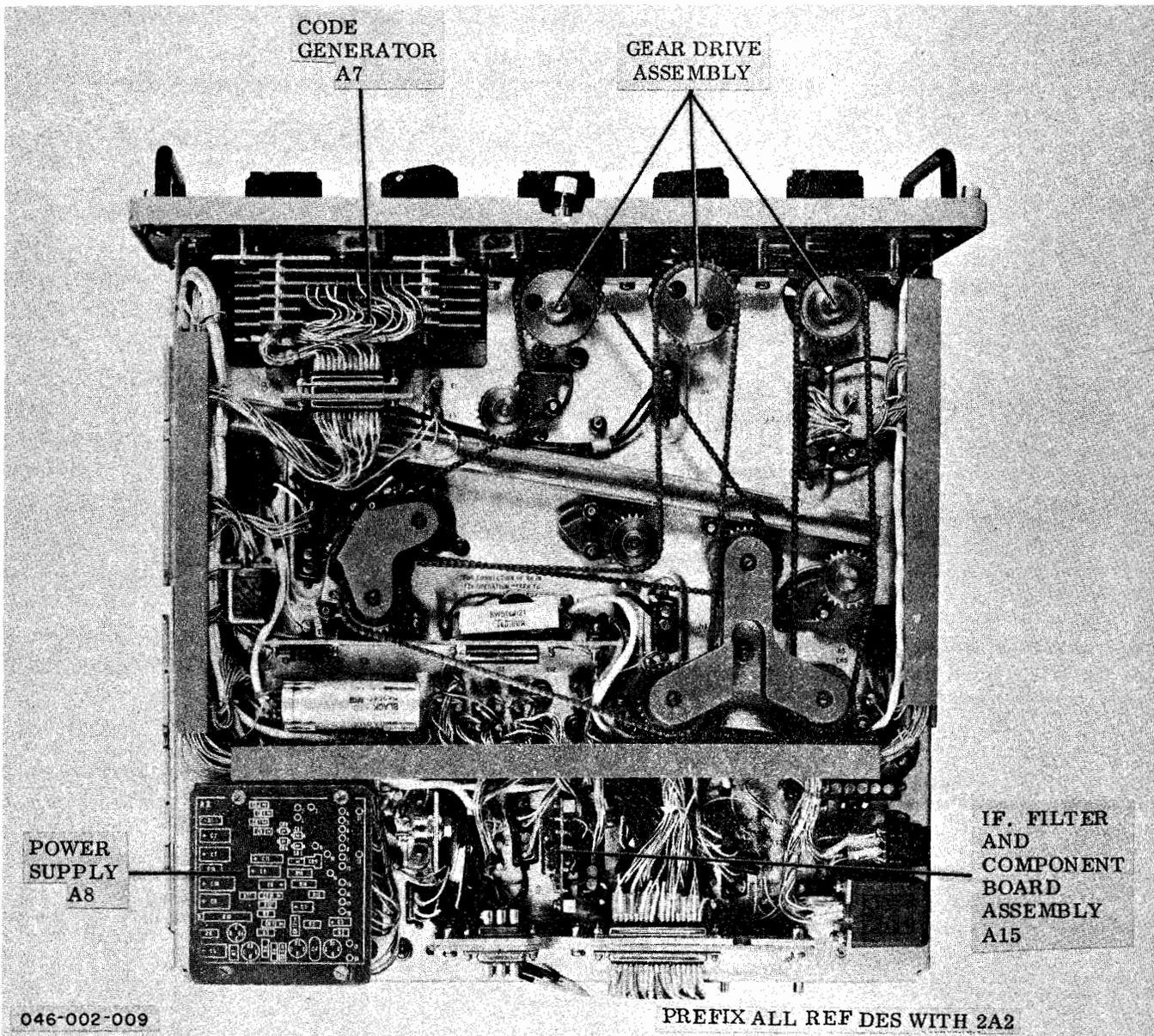
Figure 1-6. Radio Transmitter T-827B/URT, Bottom View, Case Removed
