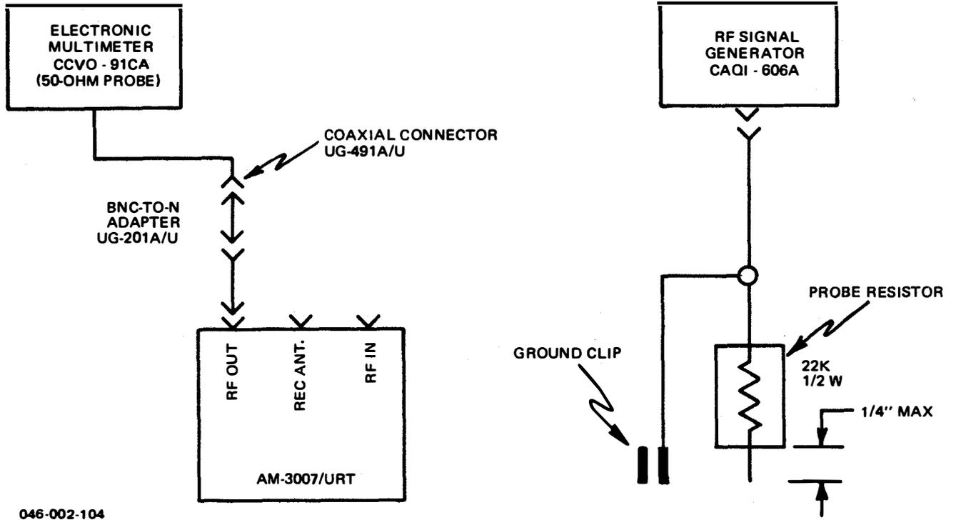
Figure 5-2. AM-3007/URT Secondary Capacitance Adjustment, Test Setup
