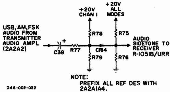
Figure 3-19. T-827B/URT, Sidetone Gate, Simplified Schematic Diagram
