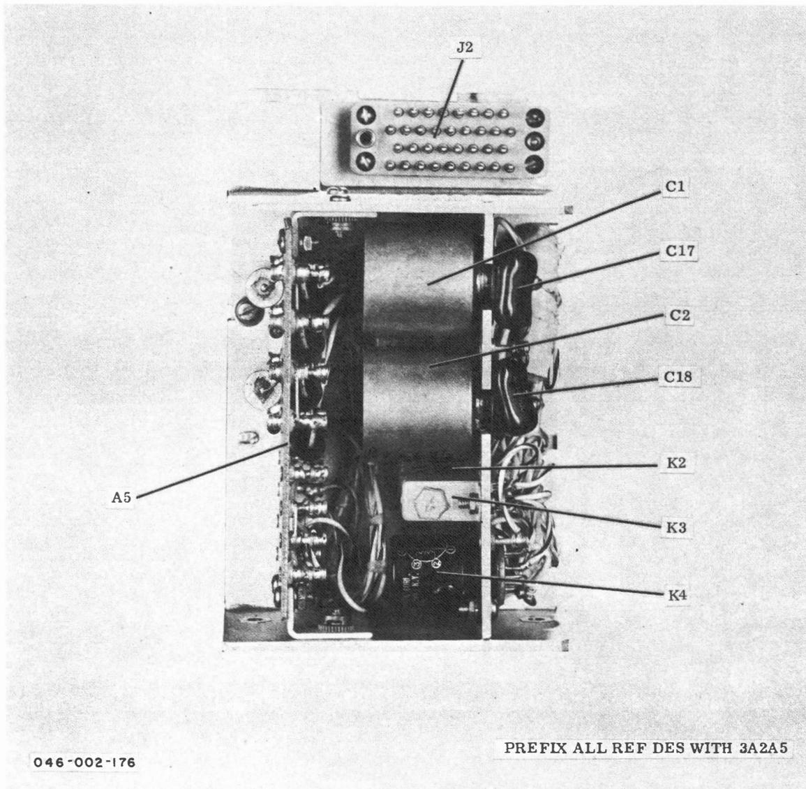
Figure 5-74. DC-to-DC Converter Assembly 3A2A5
