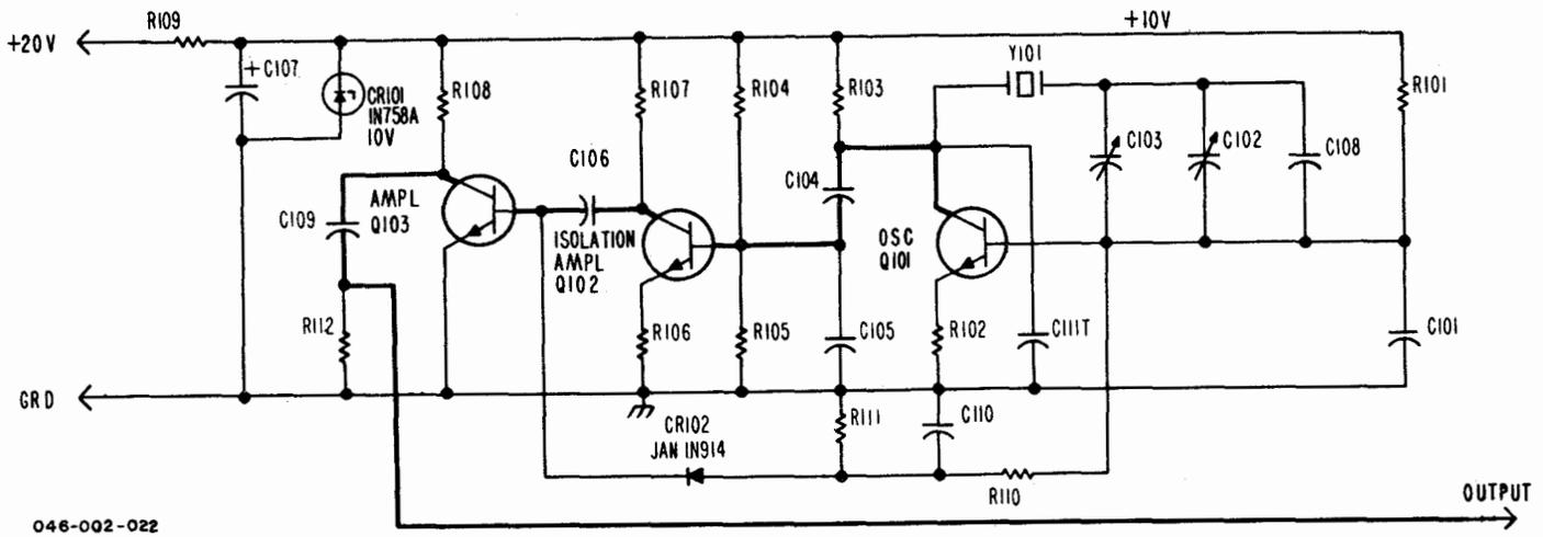
Figure 3-9. T-827B/URT, Typical 5-MHz Oscillator, Simplified Schematic Diagram
