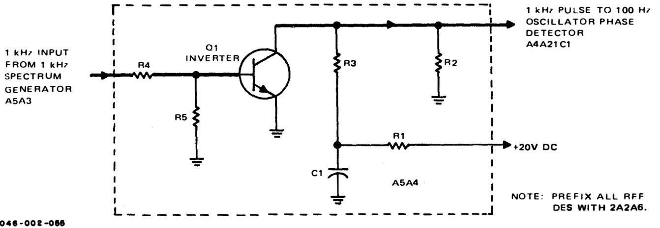
Figure 3-37. T-827B/URT, 1-kHz Pulse Inverter, Simplified Schematic Diagram
