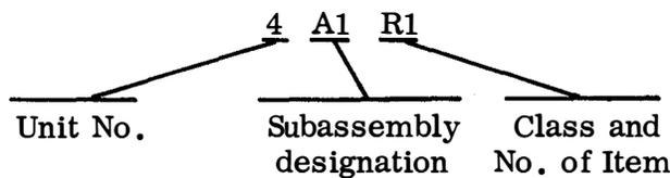
Read as: First (1) resistor (R) of first (1) subassembly (A) of fourth (4) unit.
