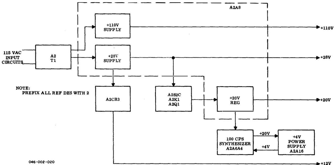
Figure 3-7. T-827/URT, DC Power Supply, Simplified Block Diagram
