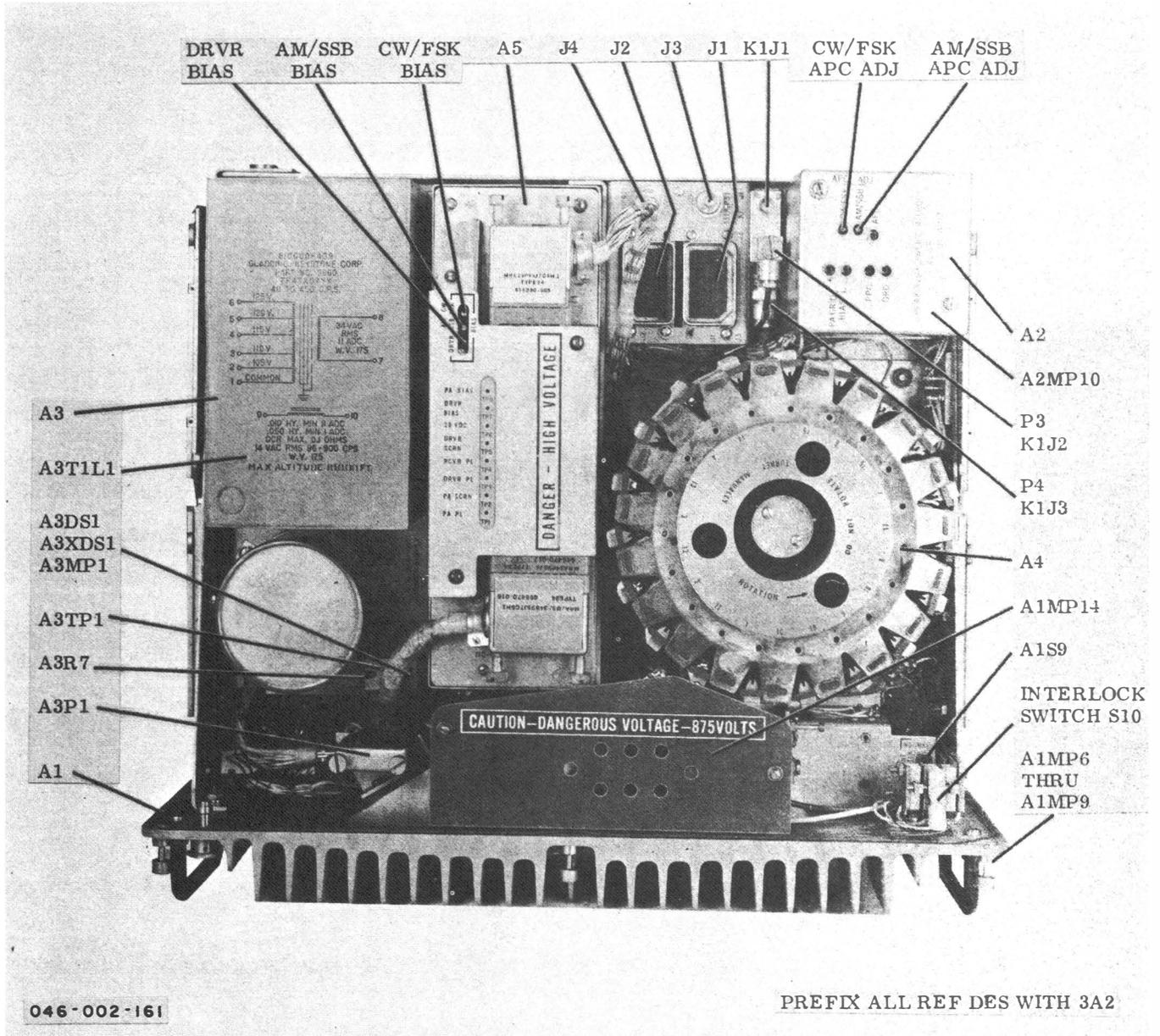
Figure 5-59. AM-3007/URT Chassis, Top View, Component Location
