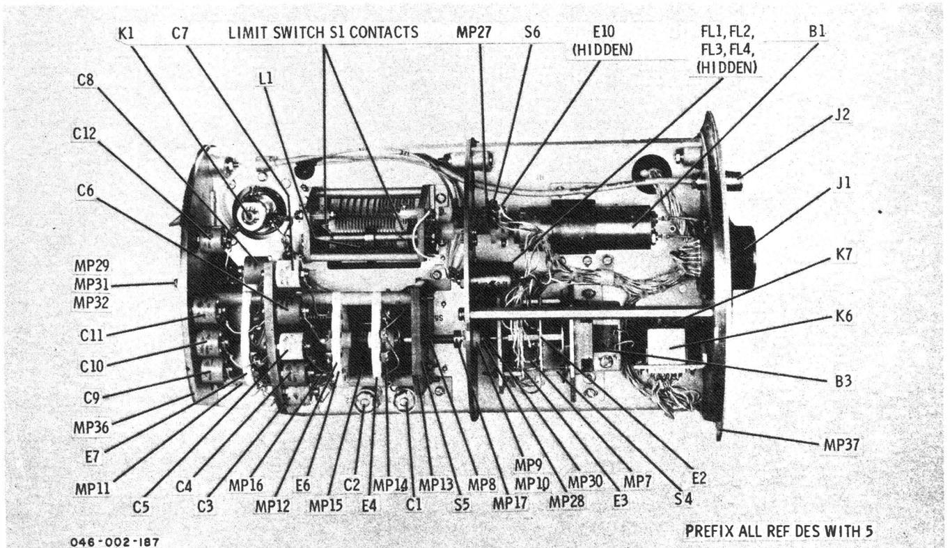
Figure 5-86. Antenna Coupler CU-937/UR Left Side, Component Location
