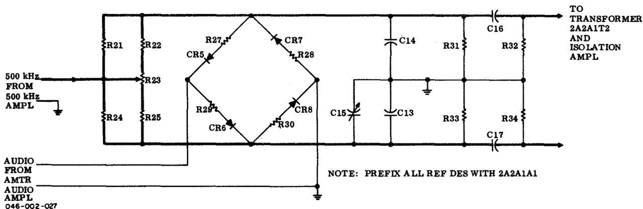
Figure 3-14. T-827B/URT, Balanced Modulator, Simplified Schematic Diagram
