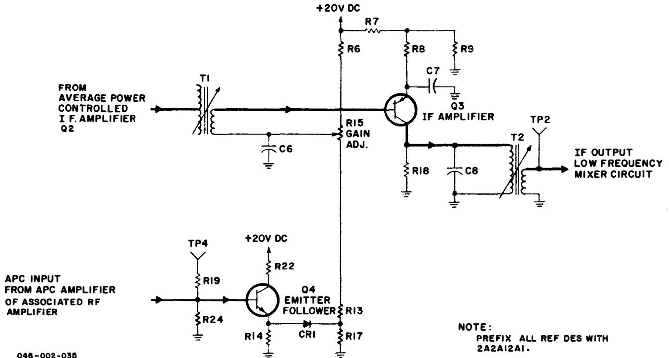
Figure 3-22. T-827B/URT, Average-Power-Controlled IF. Amplifier, Simplified Schematic Diagram
