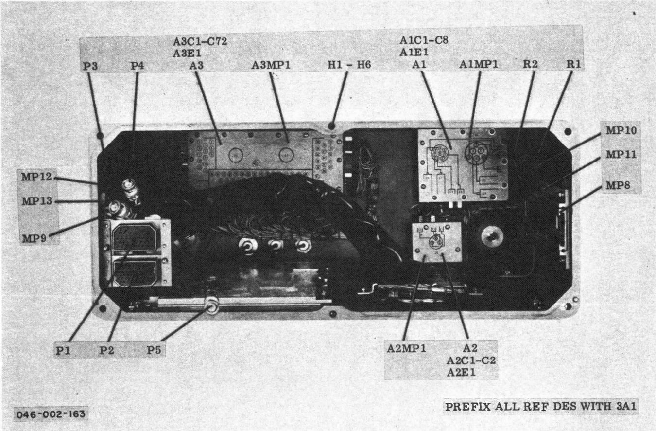
Figure 5-61. AM-3007/URT Case, Inside View, Component Location
