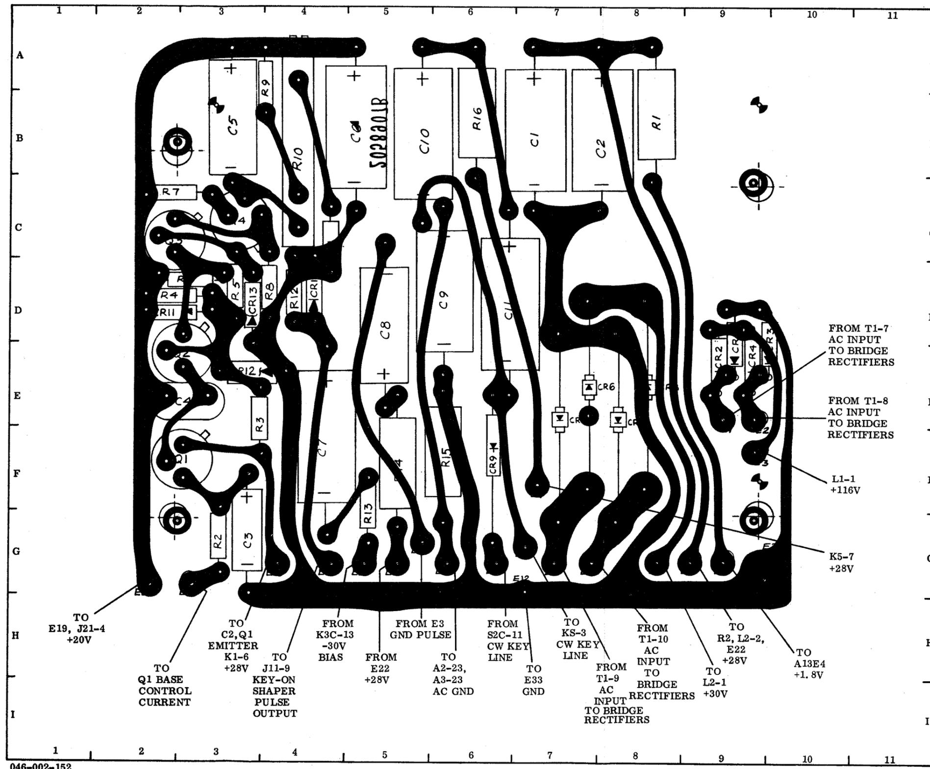
Figure 5-50. Power Supply PCB (P/O 2A2A8), Component Location
