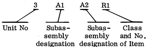
Read as: First (1) resistor (R) of second (2) subassembly (A) of first (1) subassembly (A) of third (3) unit.
