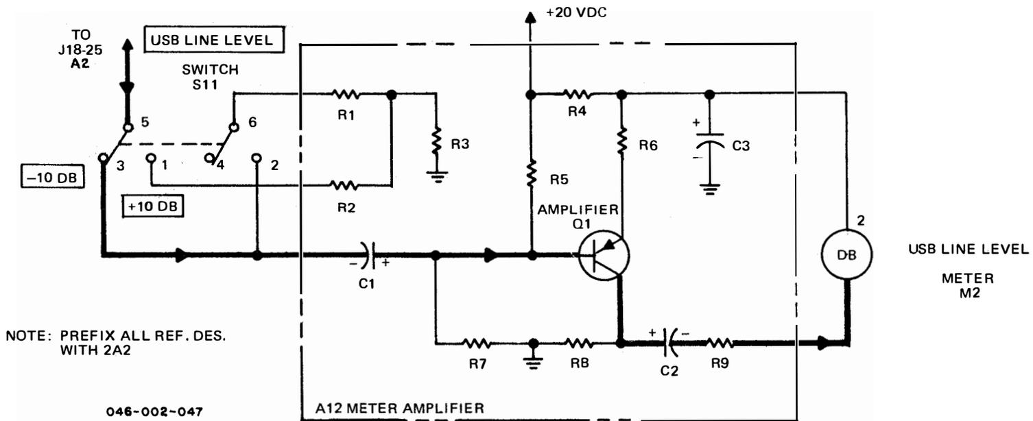
Figure 3-29. T-827B/URT, USB Audio Line Level Meter Circuit, Simplified Schematic Diagram
