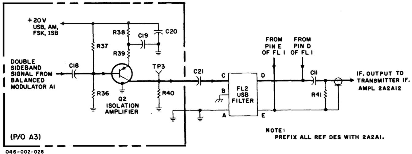
Figure 3-15. T-827B/URT, Isolation Amplifier/Filter, Simplified Schematic Diagram
