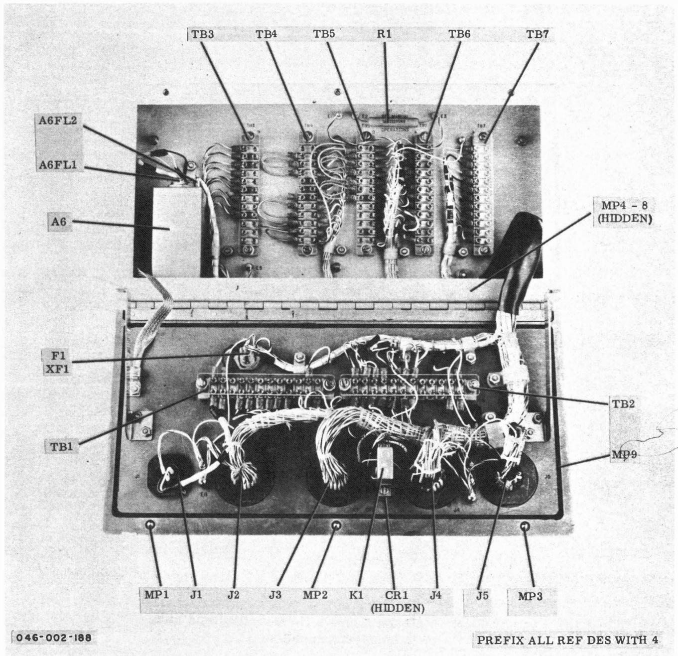
Figure 5-84. Interconnection Box J-1265/U, Cover Open, Component Location
