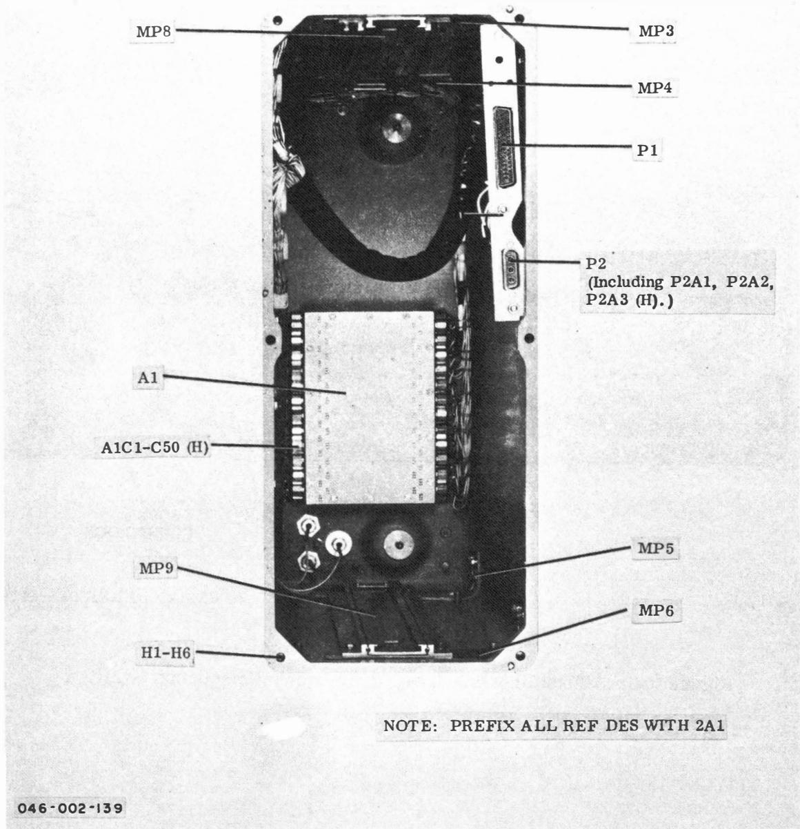
Figure 5-37. T-827B/URT Case, Inside View, Component Location
