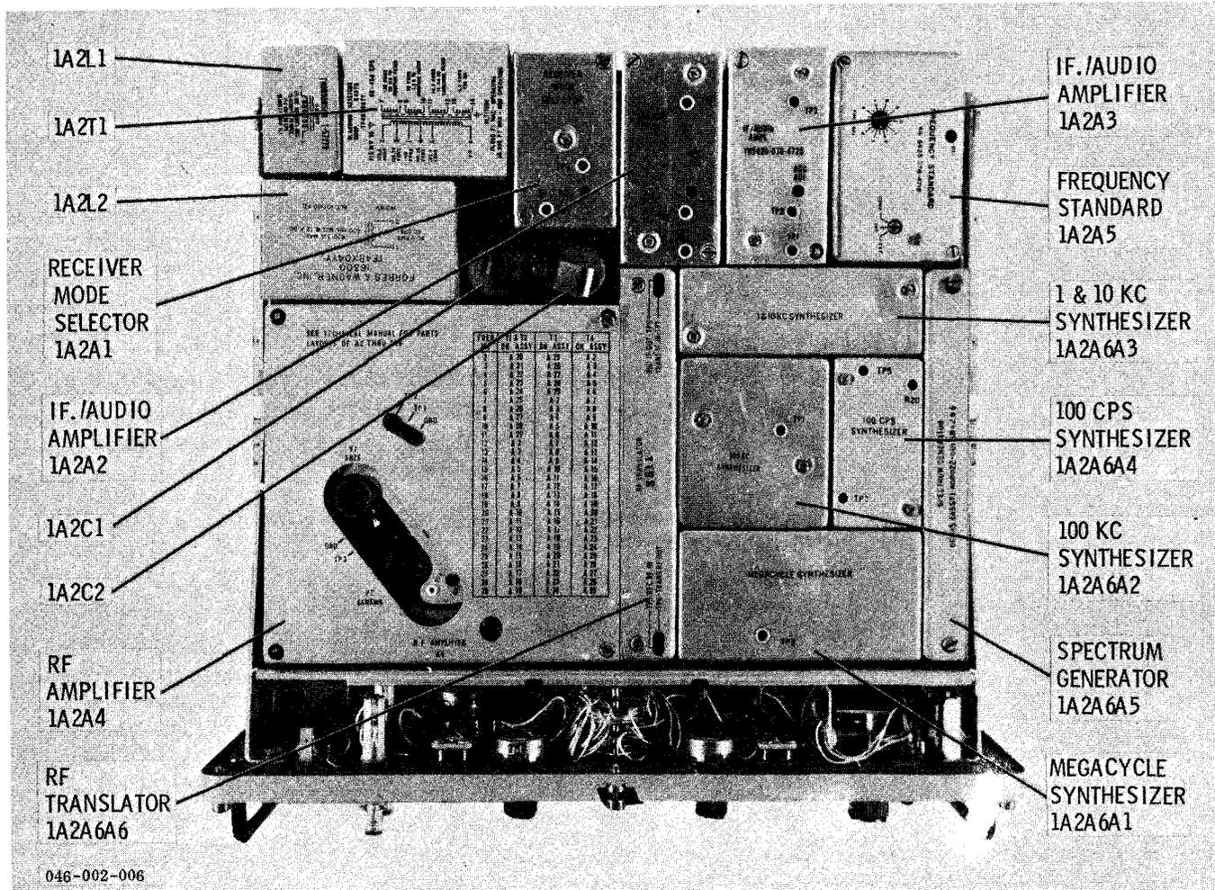
Figure 1-3. Radio Receiver R-1051B/URR, Top View, Case Removed
