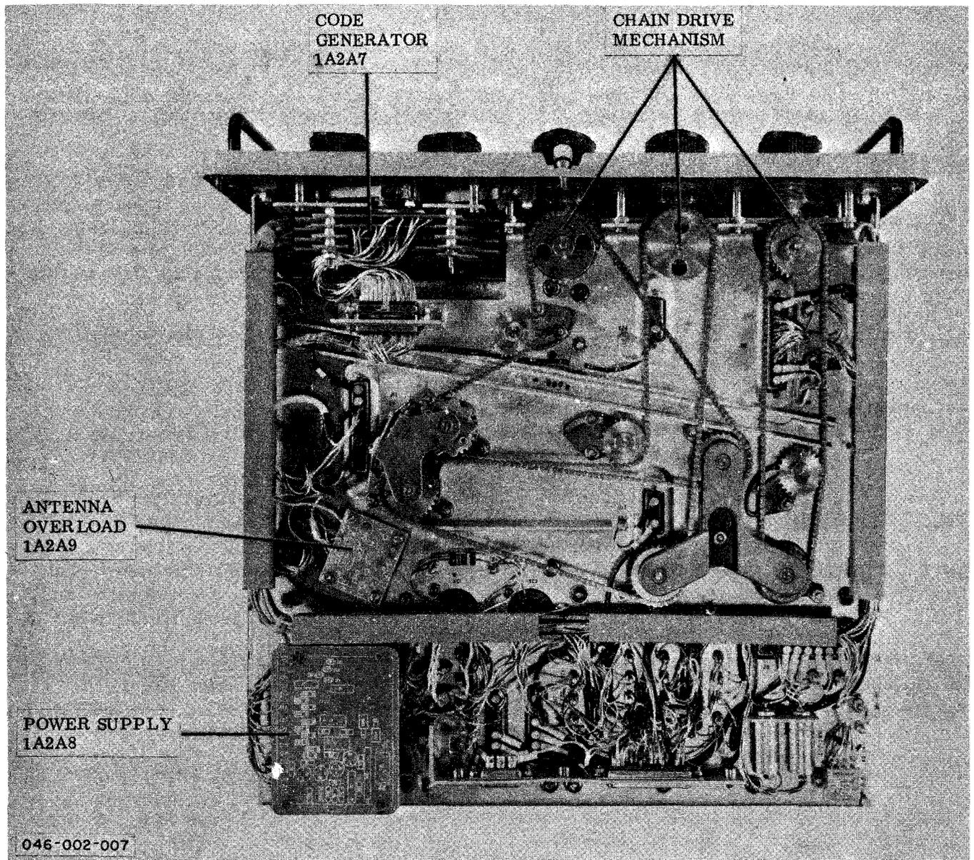
Figure 1-4. Radio Receiver R-1051B/URR, Bottom View, Case Removed
