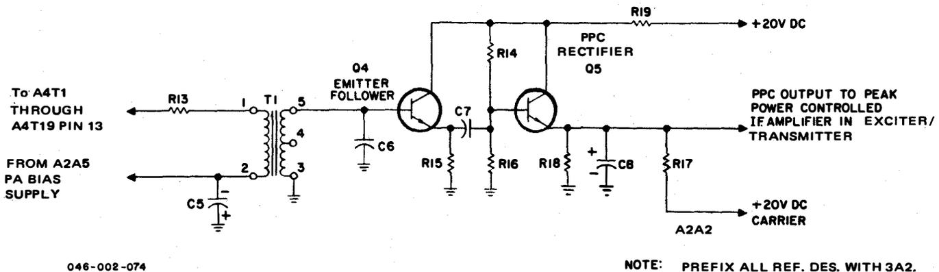
Figure 3-57. AM-3007/URT, PPC Amplifier, Simplified Schematic Diagram
