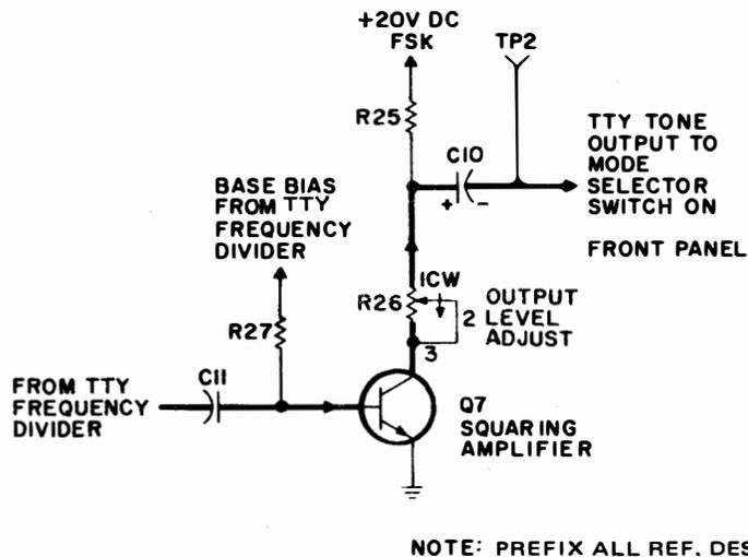
Figure 3-33. T-827B/URT, TTY Pulse Shaper, Simplified Schematic Diagram
