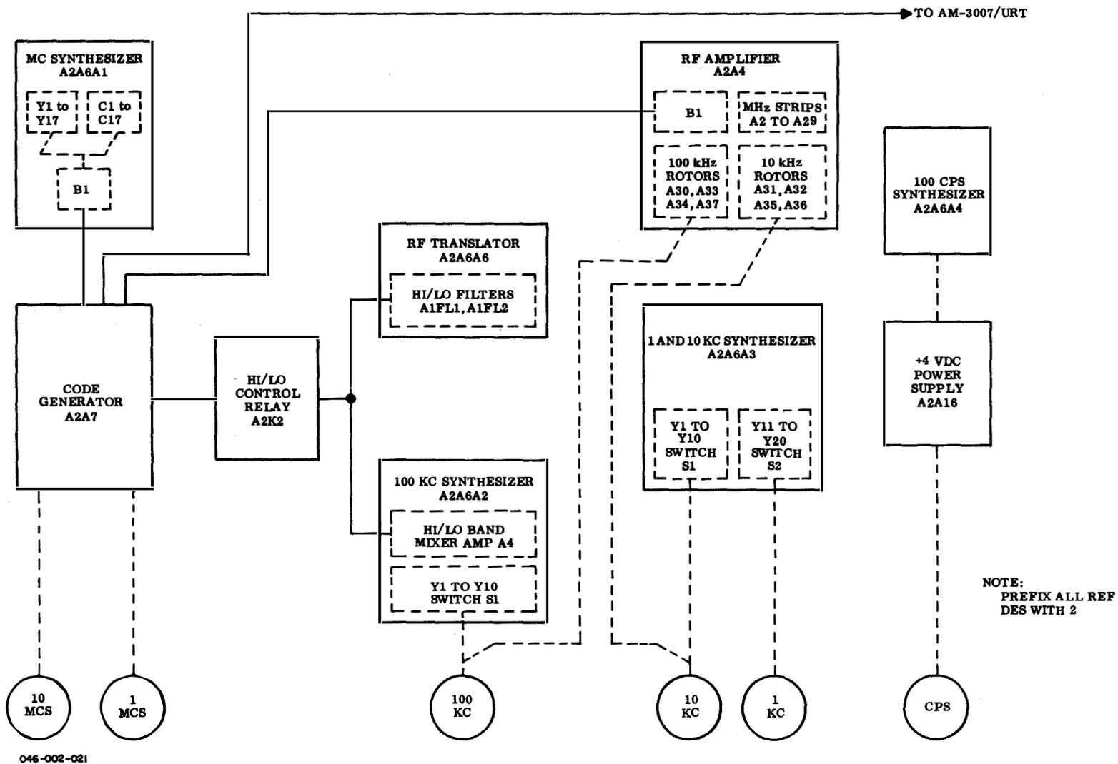
Figure 3-8. T-827B/URT, Digital Tuning, Simplified Block Diagram
