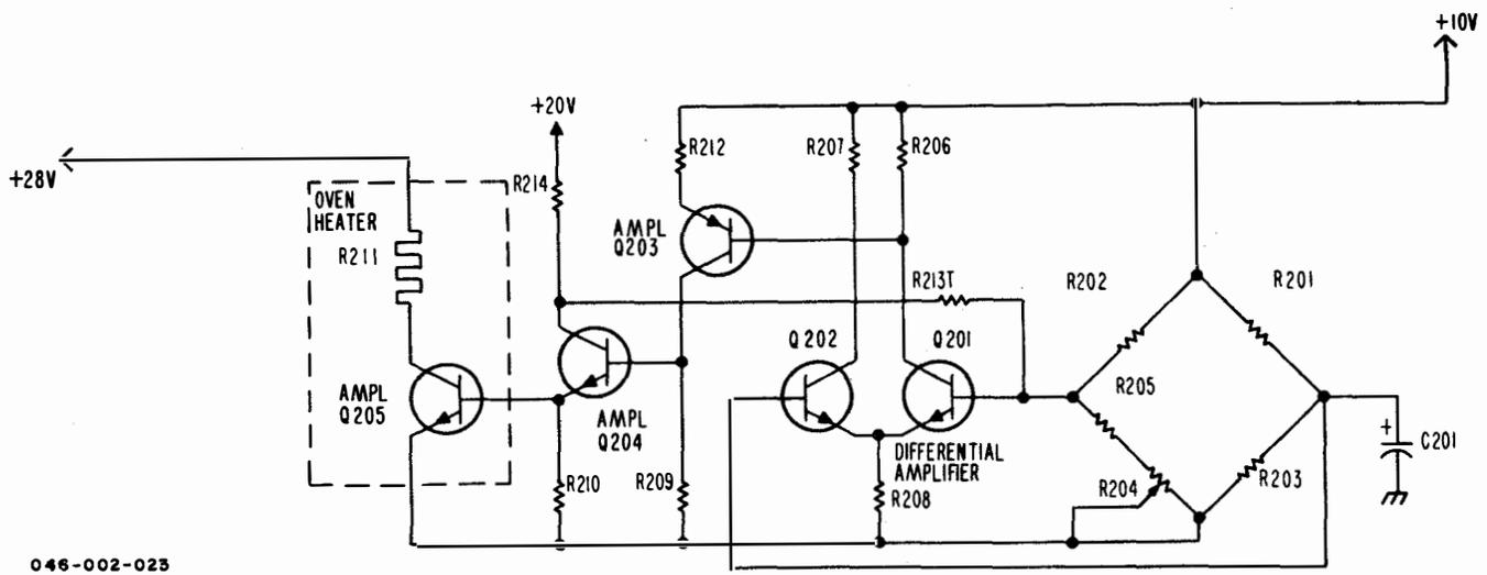
Figure 3-10. T-827B/URT, Typical Oven Control, Simplified Schematic Diagram
