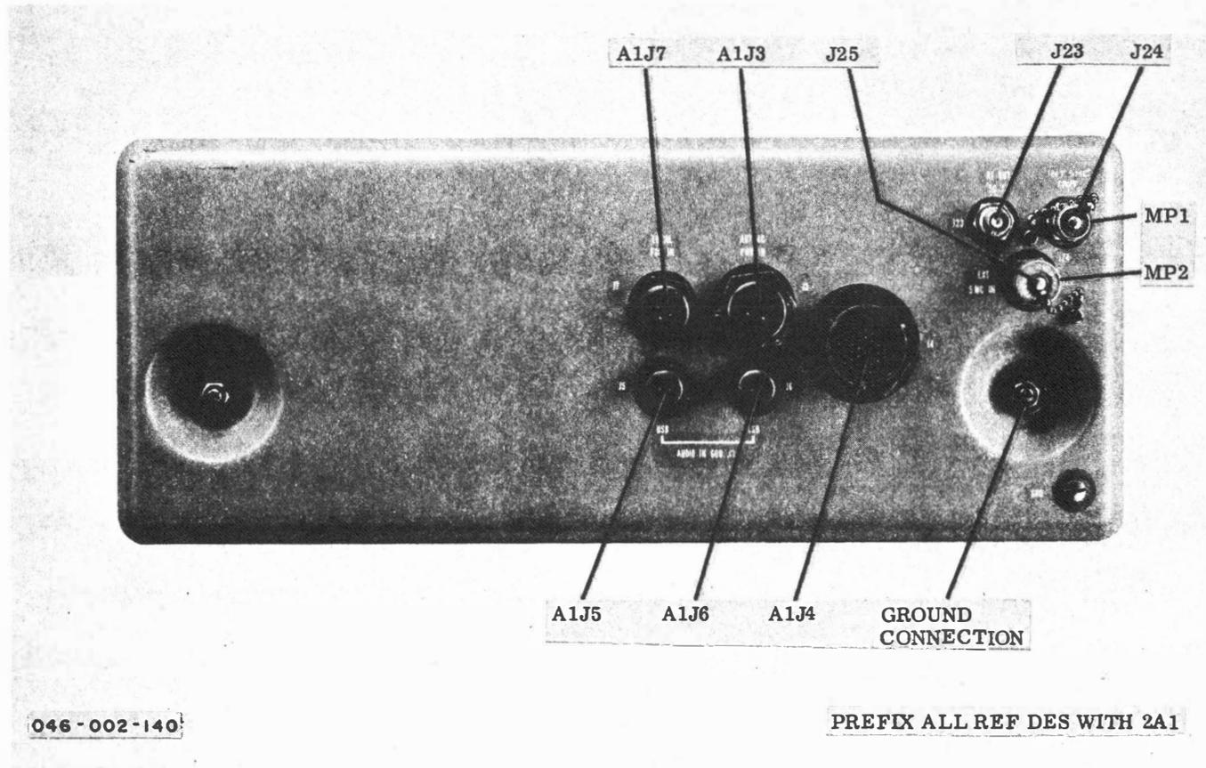
Figure 5-38. T-827B/URT Case, Rear View, Component Location
