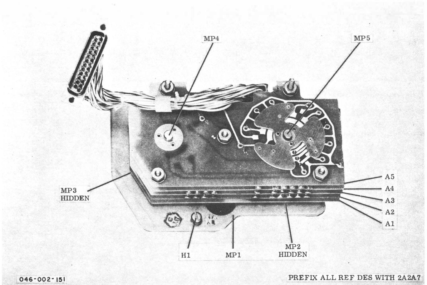
Figure 5-49. Code Generator Assembly 2A2A7,
