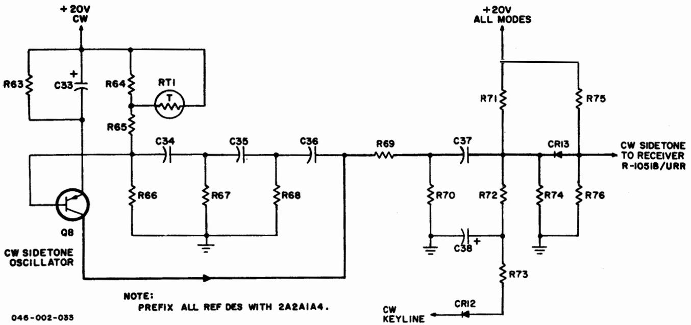
Figure 3-20. T-827B/URT, CW Sidetone Oscillator/Gate, Simplified Schematic Diagram
