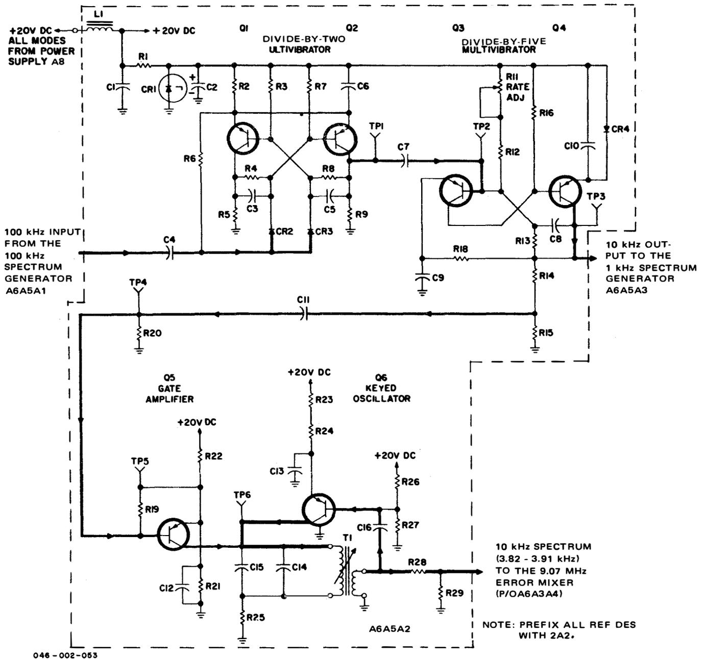
Figure 3-35. T-827B/URT, 10-kHz Spectrum Generator, Simplified Schematic Diagram
