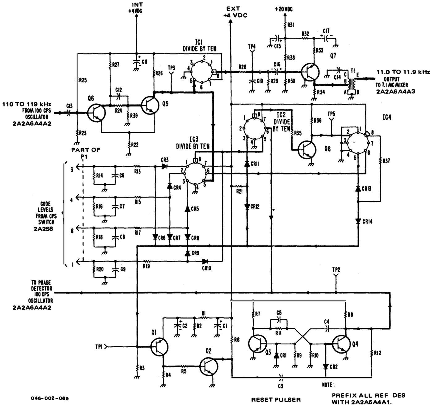
Figure 3-47. T-827B/URT, Preset Counter, Simplified Schematic Diagram
