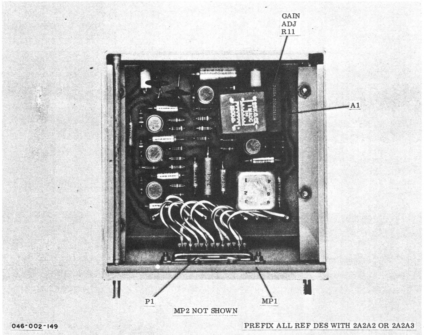
Figure 5-47. Transmitter Audio Amplifier Assembly 2A2A2 or 2A2A3,
