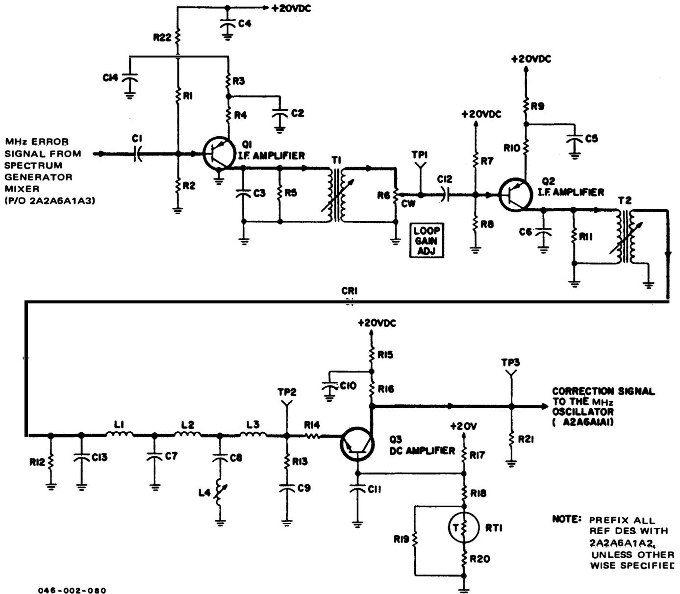
Figure 3-44. T-827B/URT, MHz Oscillator AGC, Simplified Schematic Diagram
