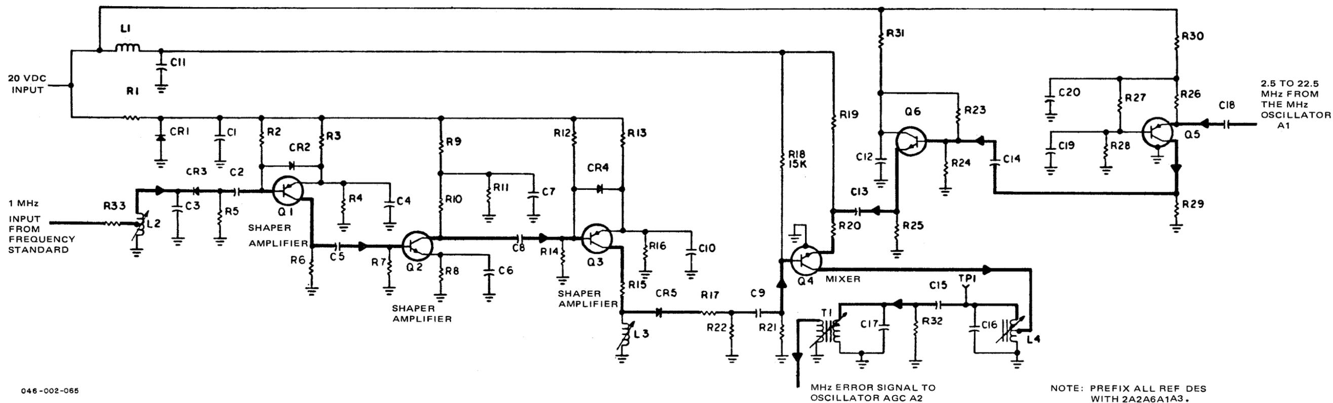
Figure 3-43. T-827B/URT, Spectrum Generator/Mixer, Simplified Schematic Diagram
