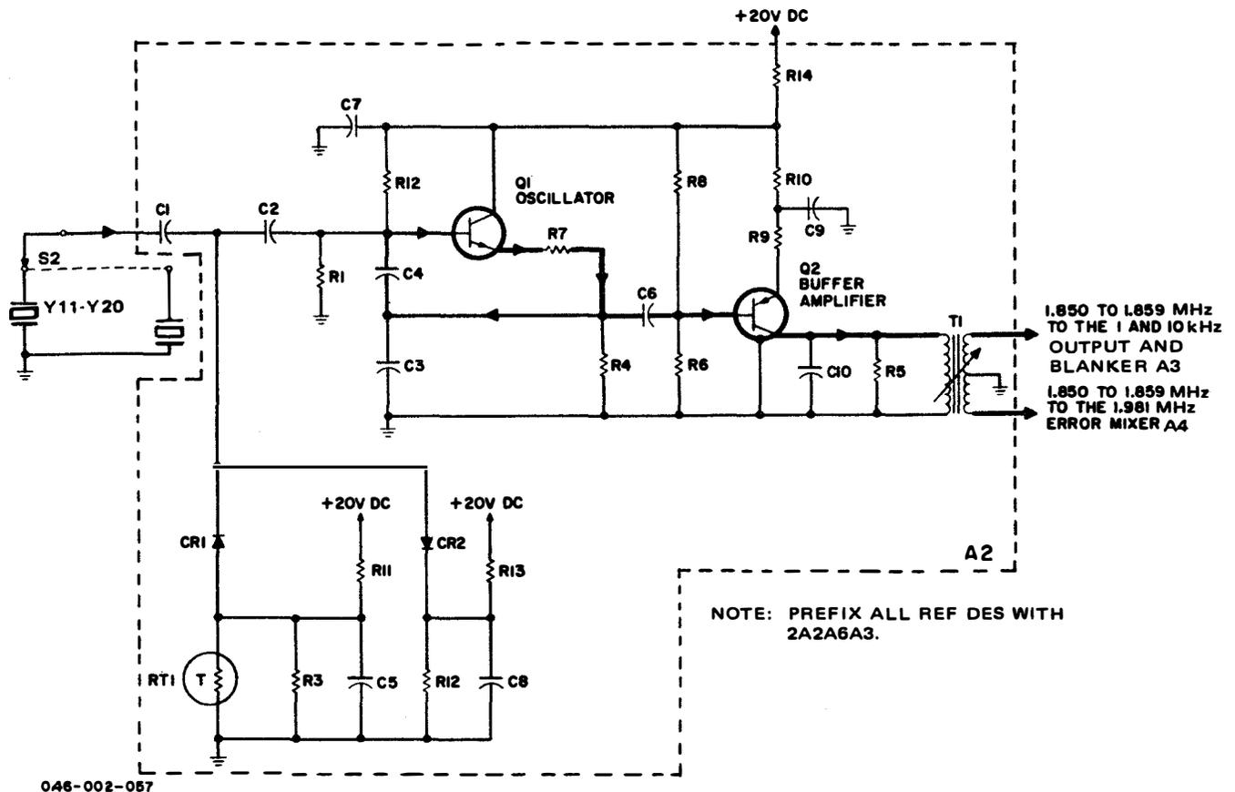
Figure 3-39. T-827B/URT, 1.850- to 1.859-MHz Oscillator, Simplified Schematic Diagram
