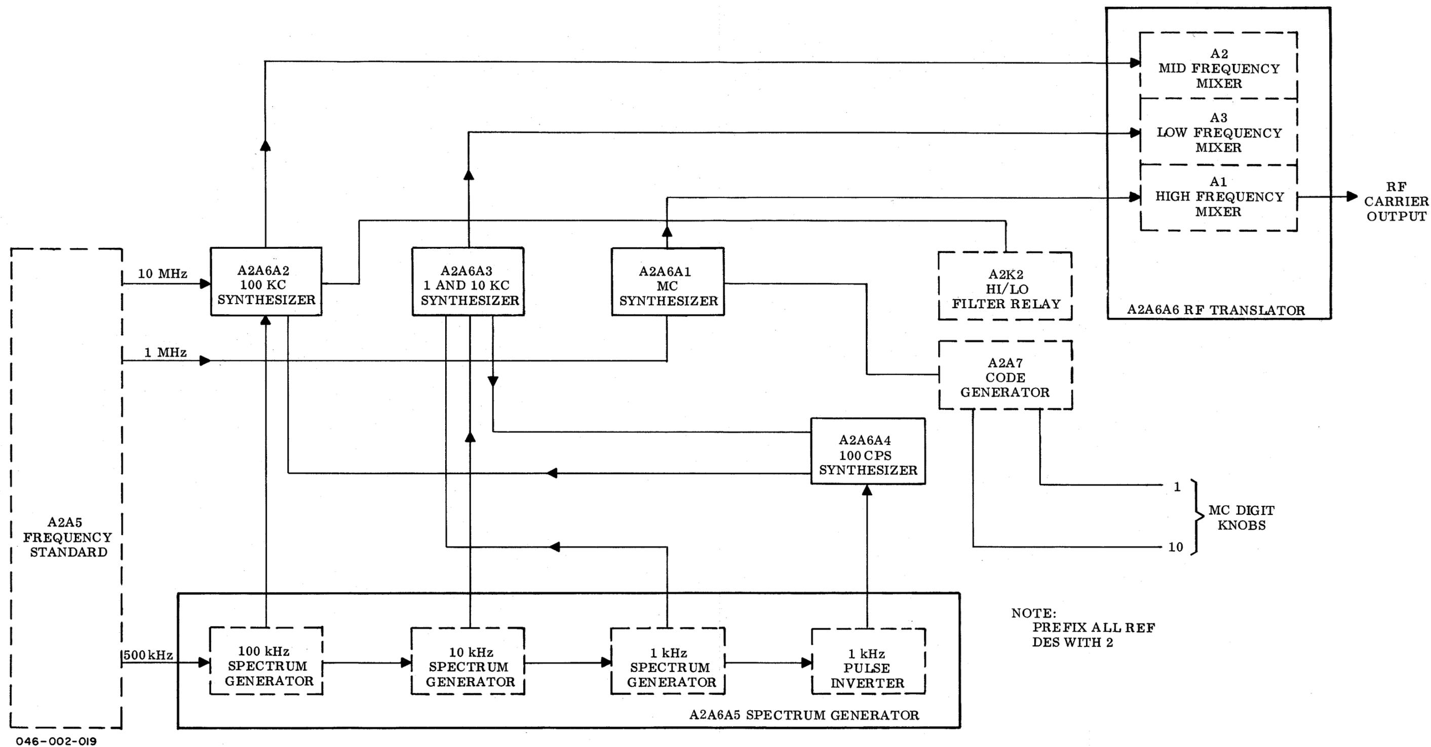
Figure 3-6. T-827B/URT, Frequency Synthesization Section, Simplified Block Diagram
