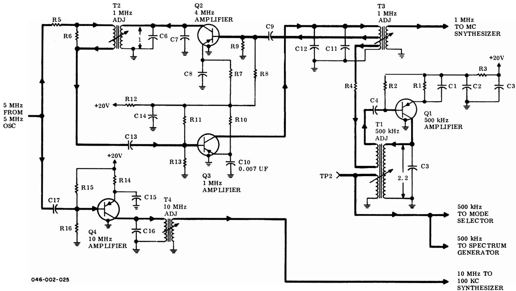
Figure 3-12. T-827B/URT, Typical Multiplier-Divider, Simplified Schematic Diagram
