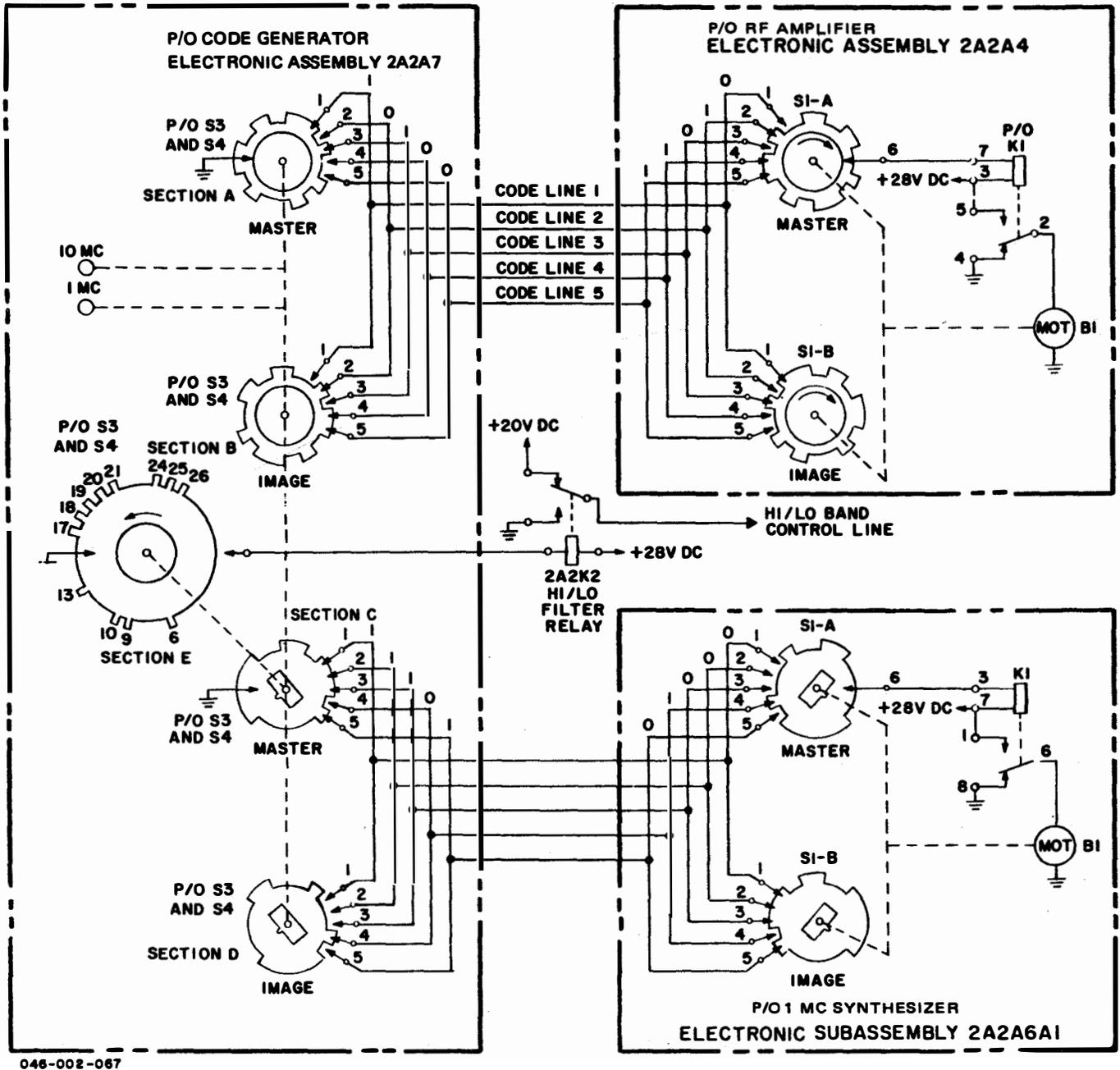
Figure 3-50. T-827B/URT, MCS Tuning Circuit, Simplified Schematic Diagram
