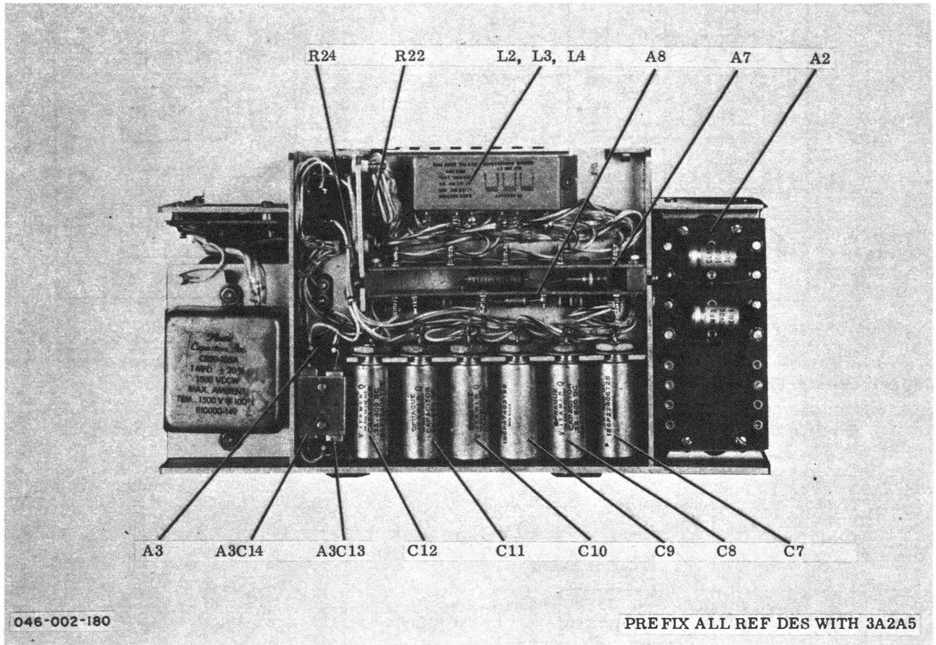
Figure 5-78. DC-to-DC Converter Assembly 3A2A5
