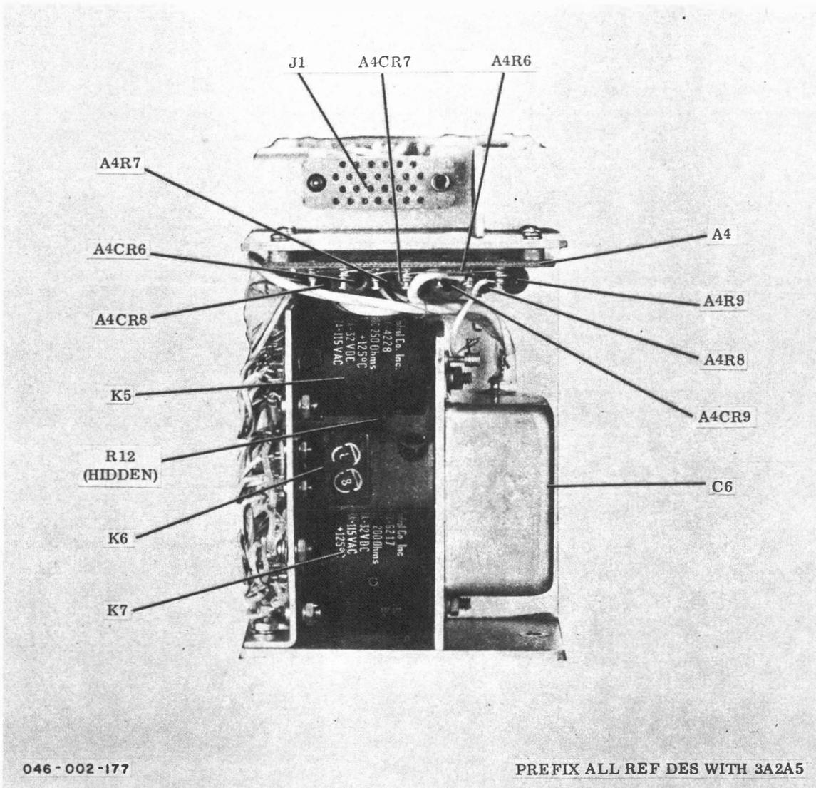
Figure 5-75. DC-to-DC Converter Assembly 3A2A5
