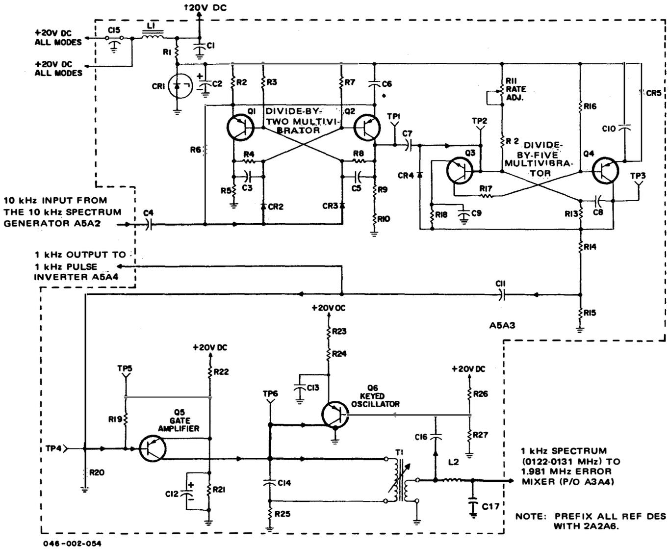
Figure 3-36. T-827B/URT, 1-kHz Spectrum Generator, Simplified Schematic Diagram
