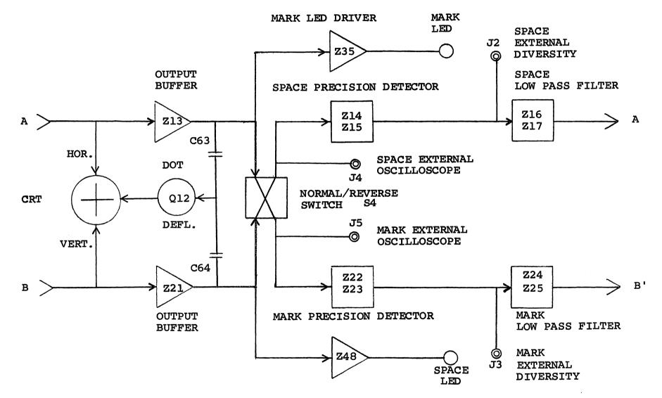
THE EXTERNAL SCOPE AND EXTERNAL DIVERSITY CONNECTORS AT THE REAR PANEL MAY BE USED FOR CONVENIENT TEST POINTS FOR TROUBLE SHOOTING OF THE VARIOUS STAGES. BLOCK DIAGRAM & VARIABLE FEATURES PAGE TWO OF FIVE.
