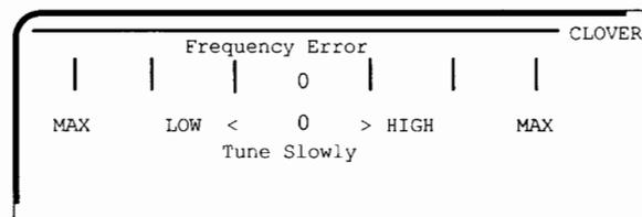
This display is a single scale that indicates the relative frequency difference between you and the station you are listening to and the direction (high or low) of the error. This bar may be used to refine the tuning done using the Amplitude Tuning Bars. The display scale is  $\pm 30$  Hz.
