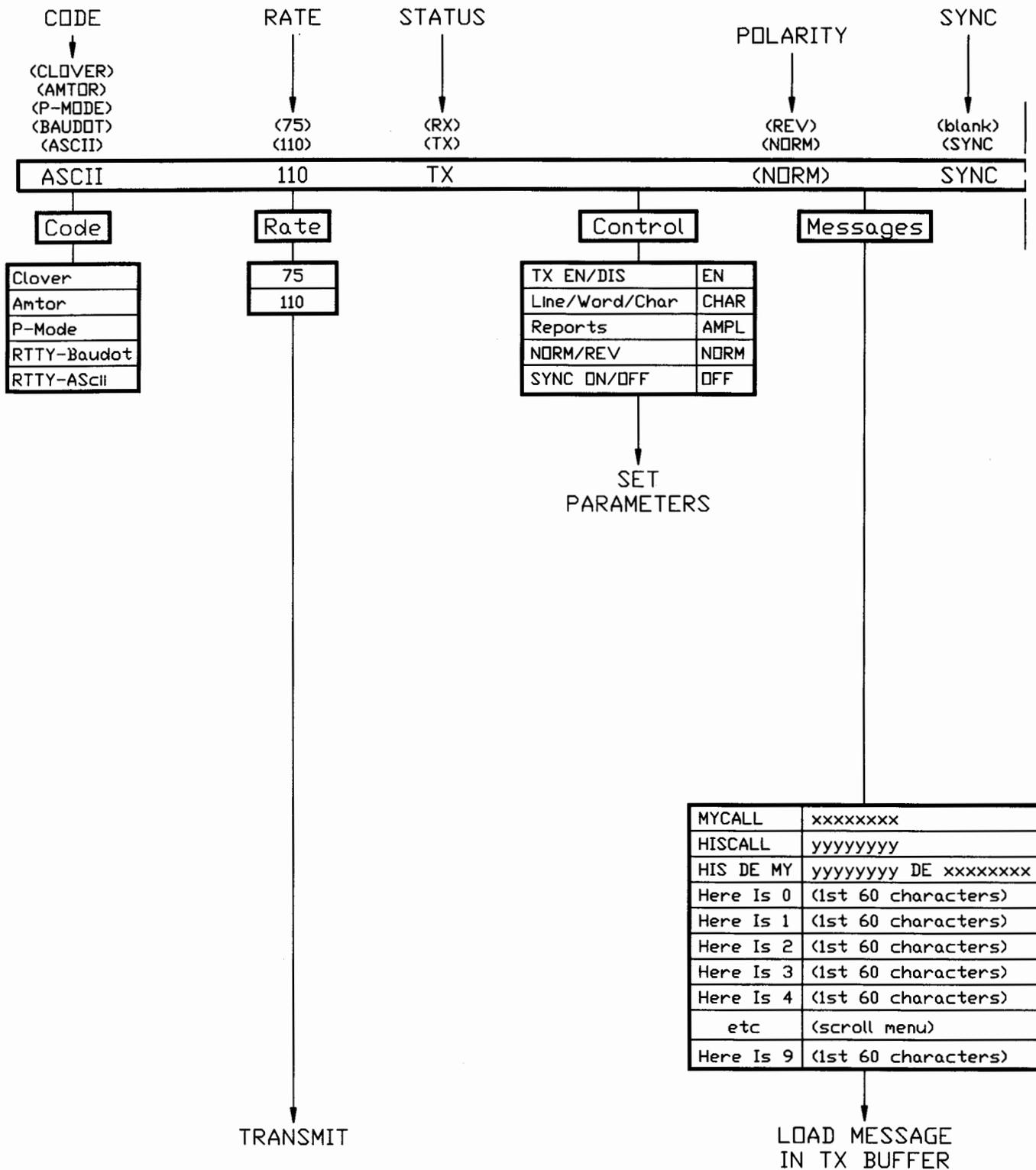
Figure 4.5 Main Menu Tree for ASCII RTTY (left side)
