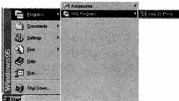
An opening WELCOME message will appear with a window requesting that you provide the correct COM Port setting for the DXP38. You may wish to save this setting in your configuration file (see section 4.5.4 Options Menu) after DXPWin has found the DXP38 modem.
