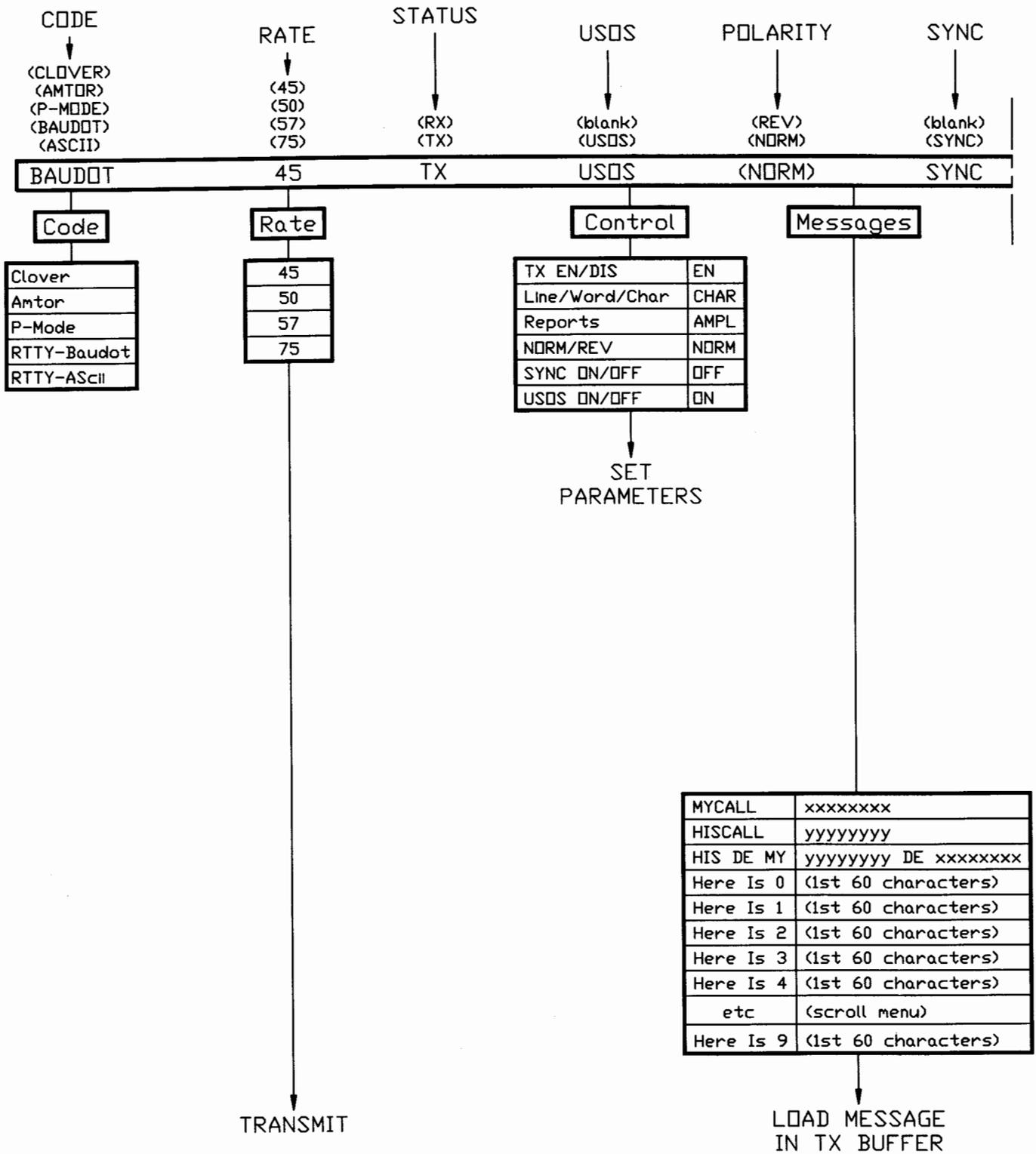
Figure 4.4 Main Menu Tree for Baudot RTTY (left side)
