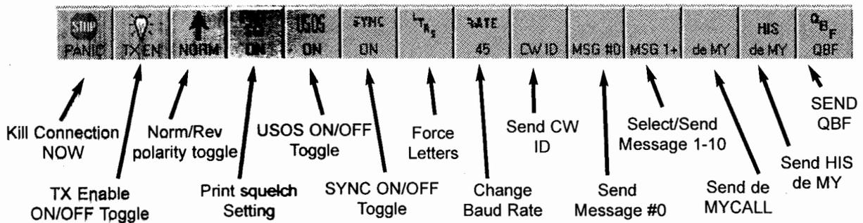
**TX Enable ON/OFF Toggle:** This option controls the state of the transmit buffer and the PTT transmit/receive control signal. In disabled state, the transmitter will not be turned ON and text typed into the transmit buffer will be held until this control is set to enabled. Disabled is the normal receive state. This control changes from disabled to enabled each time this option is selected.
