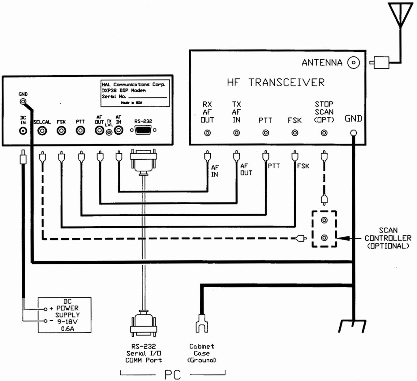
Figure 2.2 Radio System Connections
