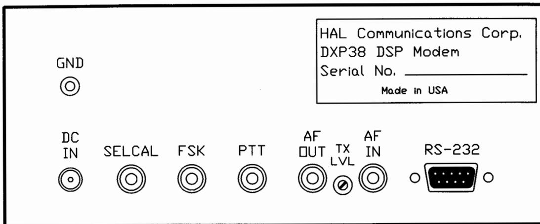
**Figure 2.1 DXP38 Rear Panel Connections**
