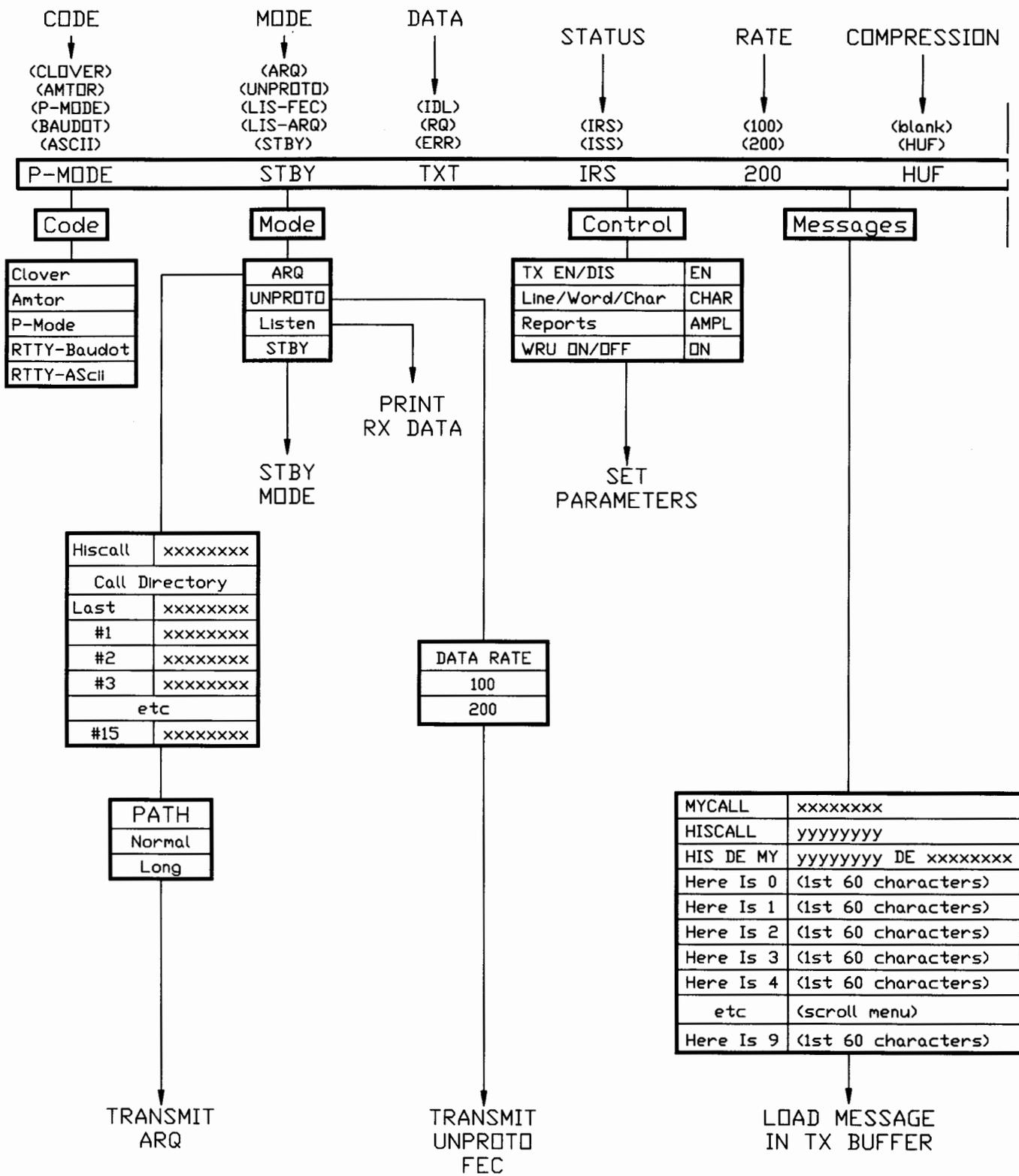
Figure 4.7 Main Menu Tree for P-Mode (left side)
