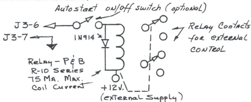
Fig. 3 Suggested Autostart Wiring
