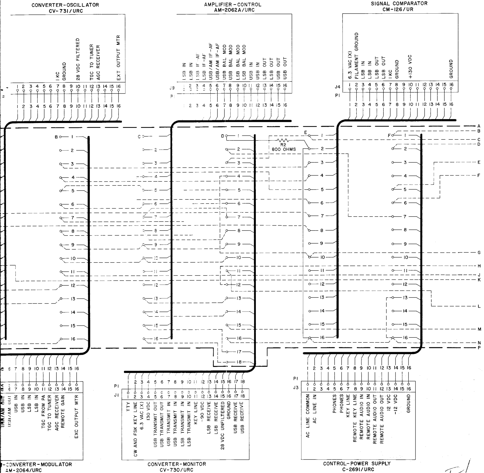
Figure 5-96. Interconnecting Box J-1007/U, Interconnecting Wiring Diagram (Sheet 1 of 2)
