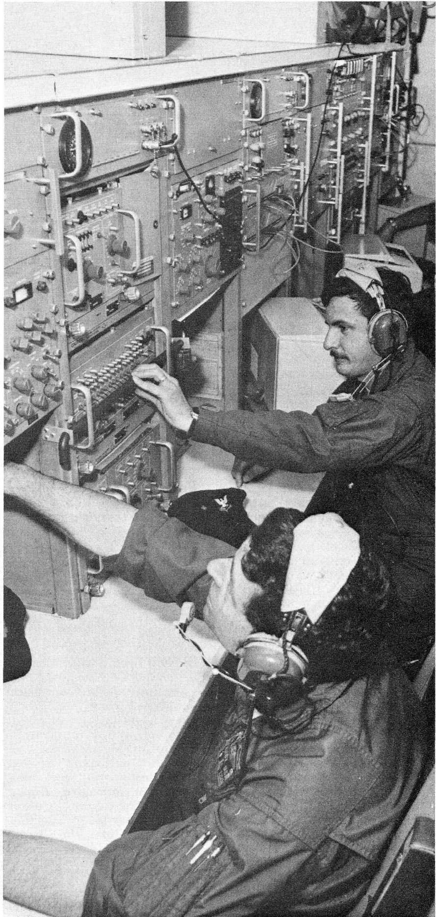
TACAMO crew members in the Communications Central receive, analyze, process and transmit messages over the frequency range from VLF to UHF.
