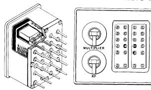
The ten crystals controlling the basic frequency generated in the oscillator section of V504 are grouped and mounted in the compact unit shown in the illustration. The crystals are of the hermetically sealed miniature type CR-7E/U and the terminal pins of the individual crystal holders fit into jacks inside the unit that connect to pins on the rear of the unit. The cover may be removed from the unit for the replacement or installation of individual crystal holders.
